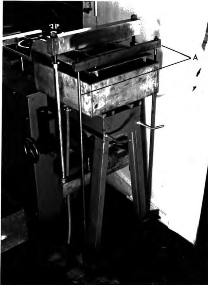
Plate III. 2. 12-inch direct shear-box with framework (A) attached to prevent vertical movement of the upper shear-box half.
