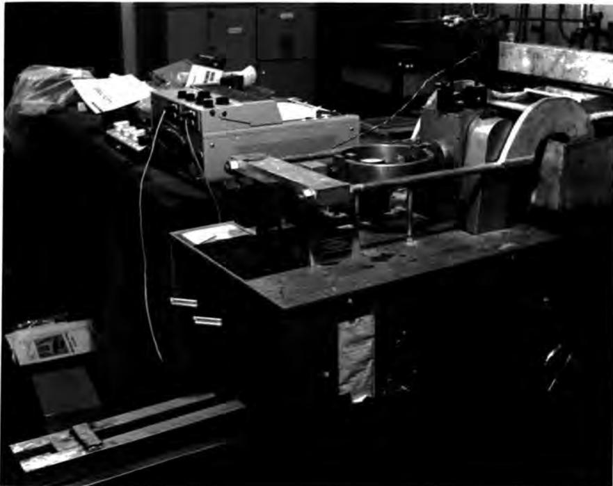
Plate III. 1. Retaining bracket attached to the rear of the shear-box to prevent movement of the upper half of the shear-box during reverse shear.
