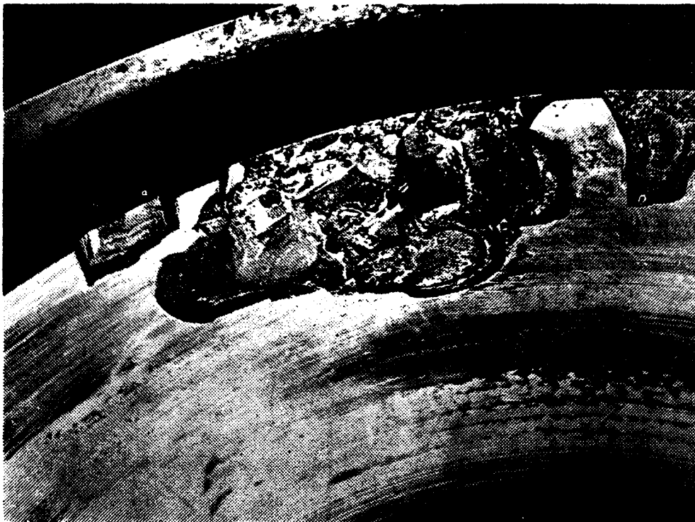
-Distressed area of bearing
