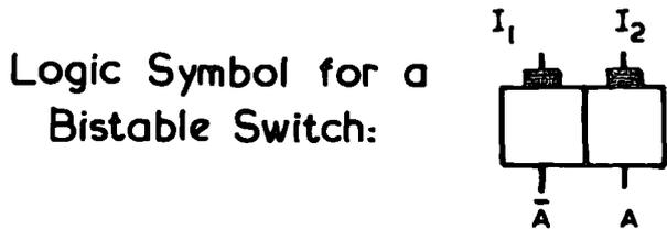
This circuit will change states as pulses are applied alternately to the two inputs.
