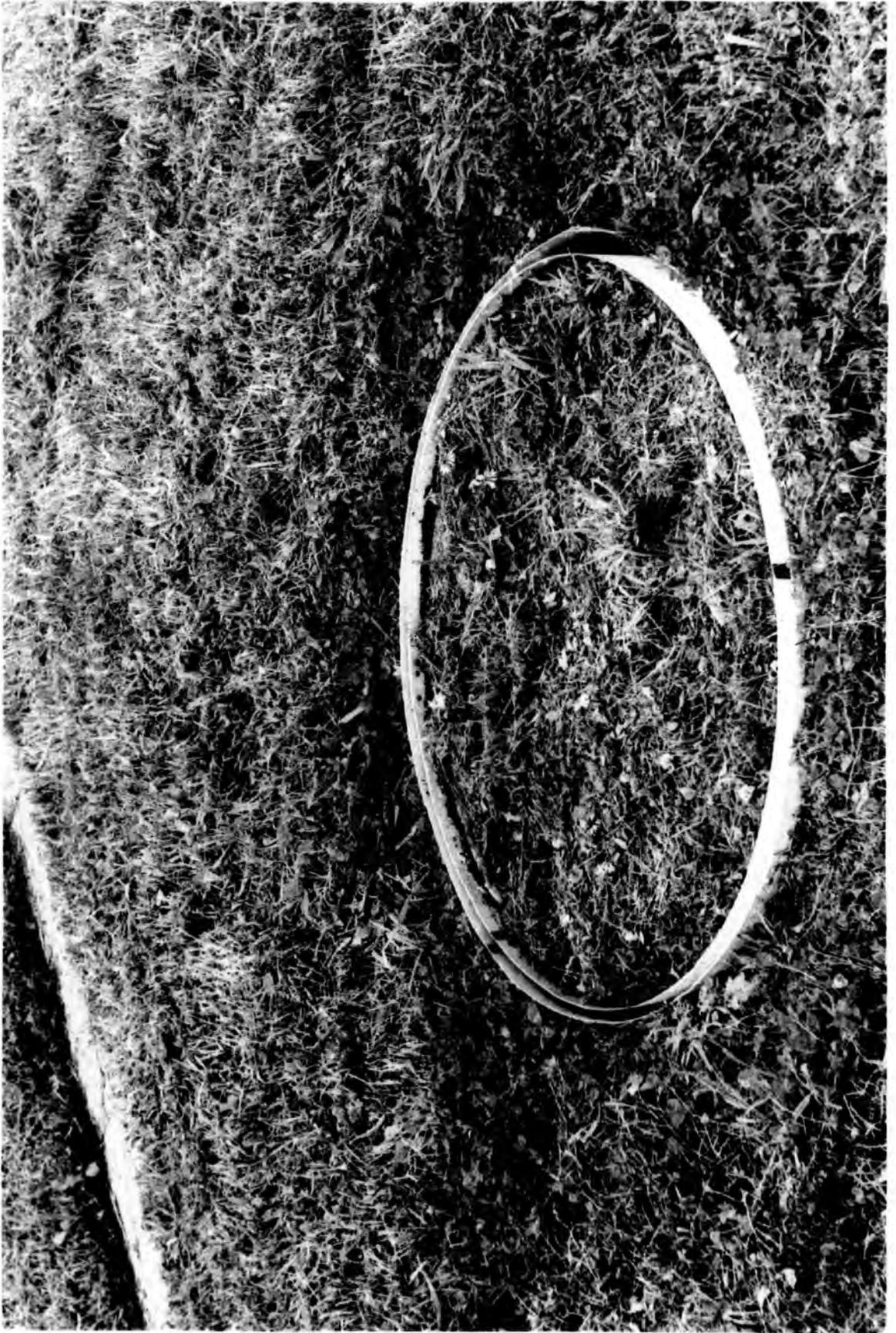
Fig. 4.3 The air-earth current collector
