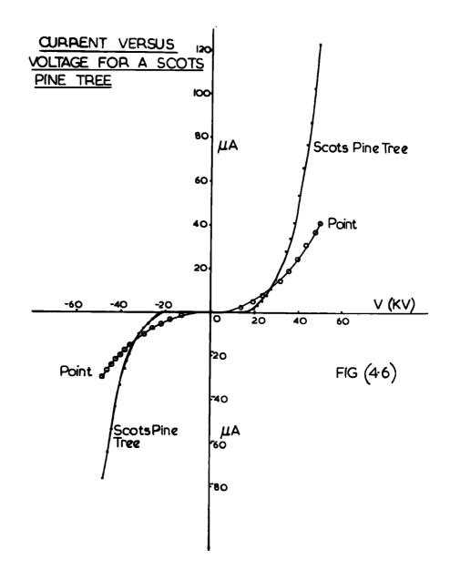
The measurements were also made of the point discharge current through a metal point of the same height as that of the tree. The experiments were finally repeated for the other two trees i.e. the Sycamore and Cryptomeria Japonica. Some of the results for the Scots Pine tree, with the positive and negative potentials on the plate, are shown in fig. (4.6). The results are similar for the other two trees.
