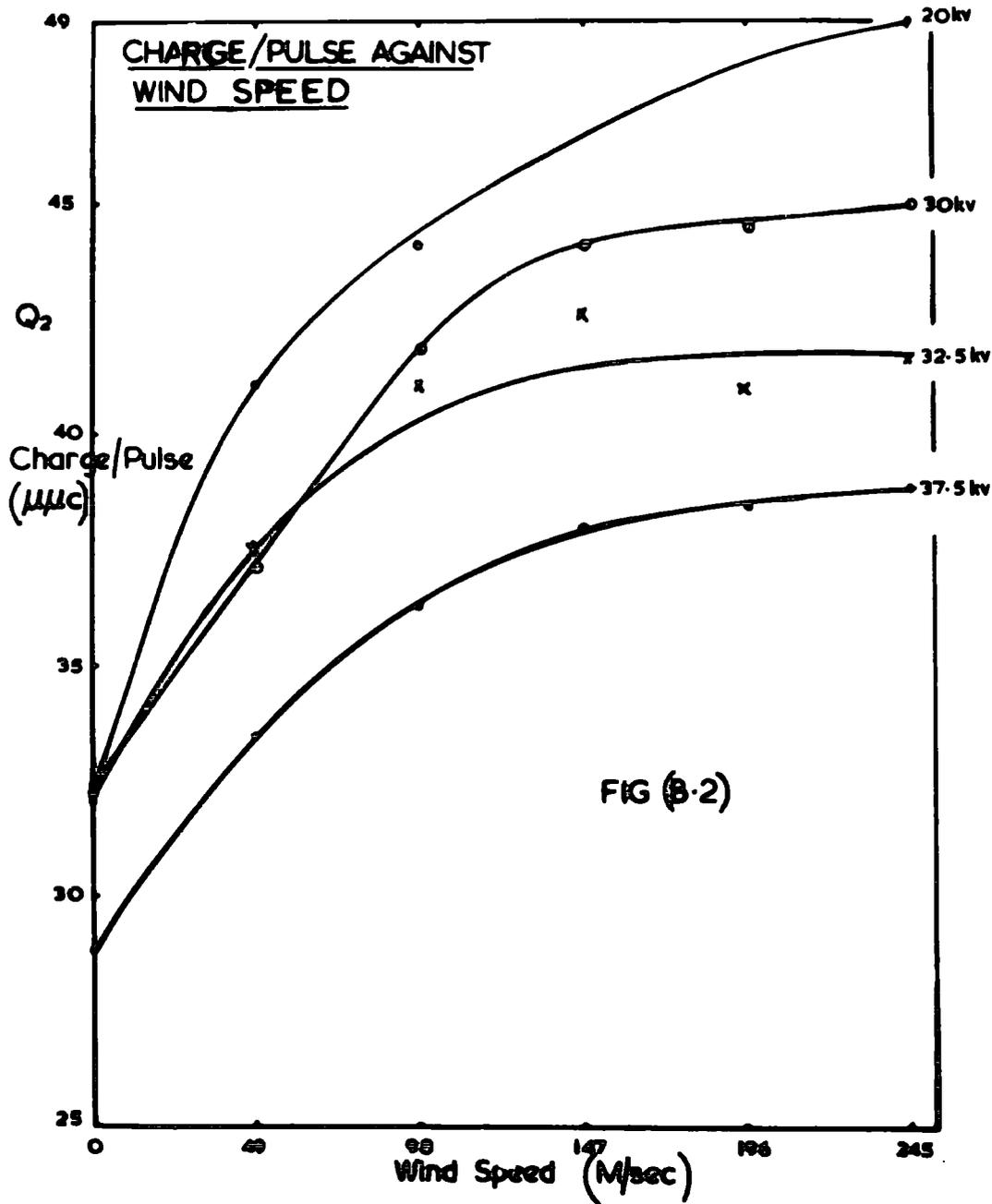
speed increases, the amplitude of the pulses increases, the frequency decreases, giving a corresponding increase in charge per pulse. A similar type of plateau occurs at about 147 m/s, as was observed by NYGAARD (1966b).
