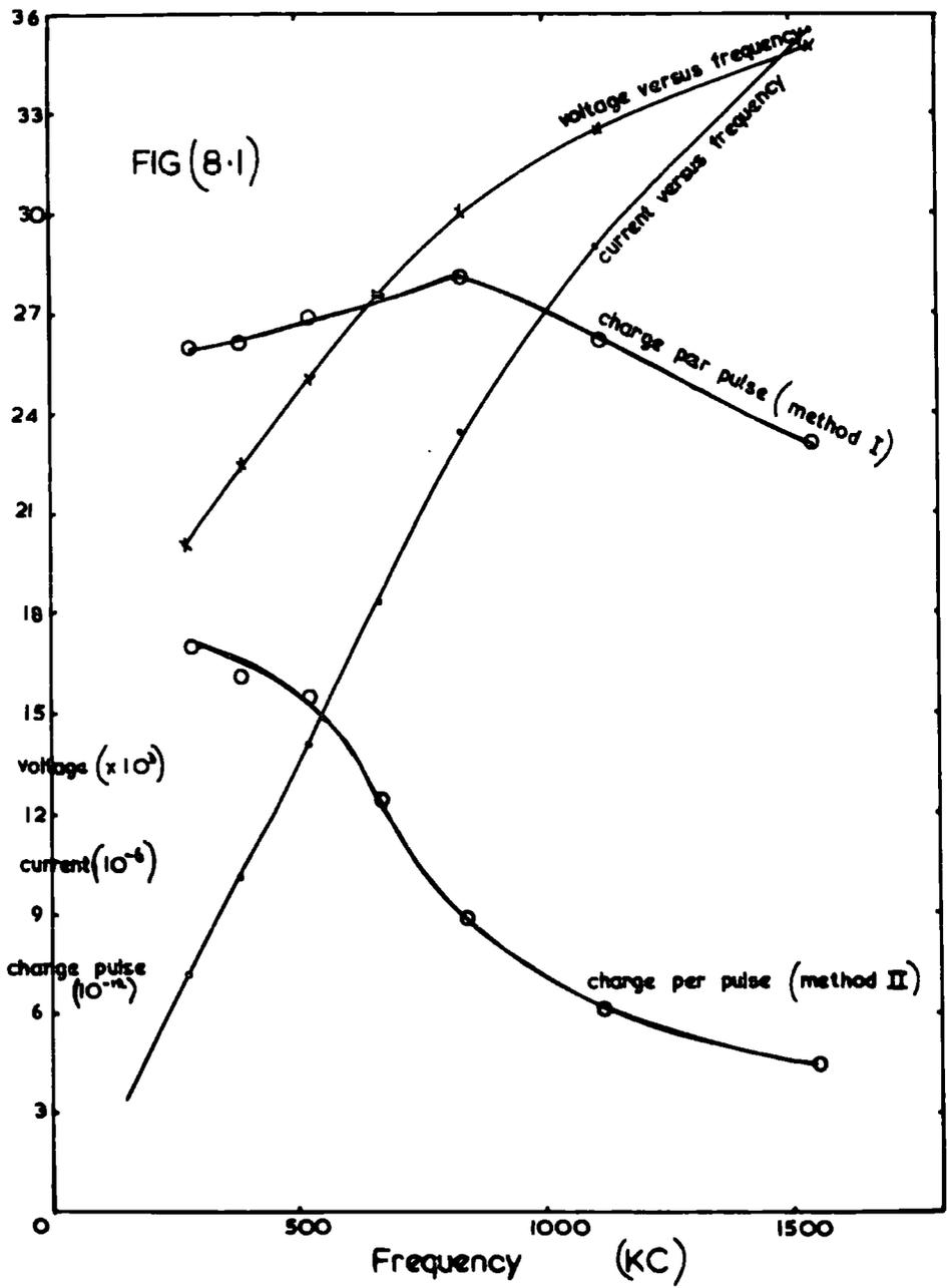
Fig. (8.1) shows the variation of current, voltage and charge per pulse (as evaluated by both the methods) against frequency.
