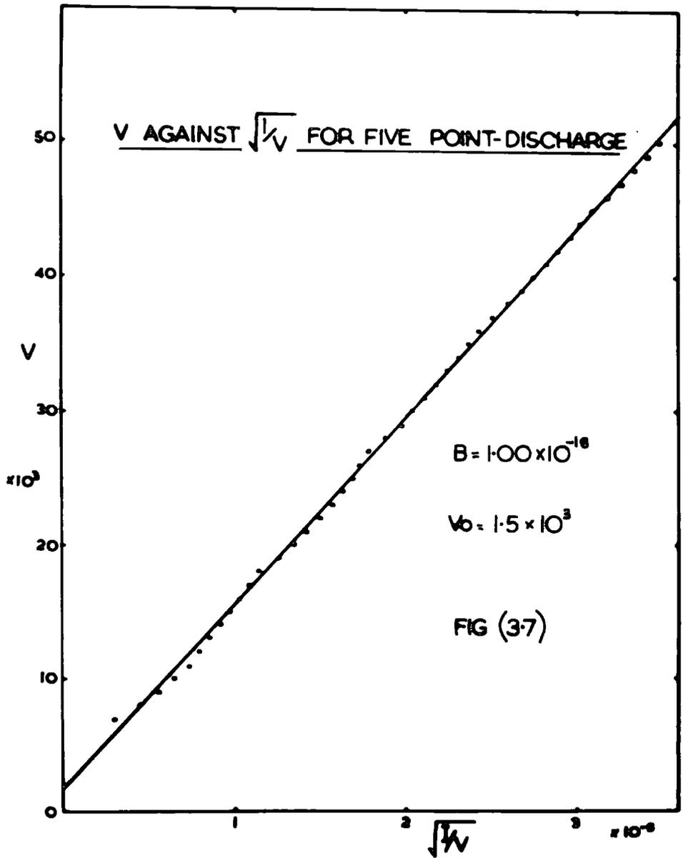
Finally the fig. (3.7) shows that the total point-discharge current through these five points, having different starting voltages, obey a cube law of the form:
