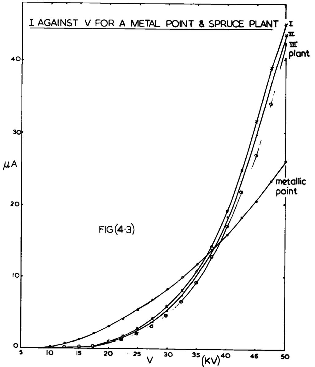
the latter began to decay and settled down to a fairly steady value after a few minutes. So the readings of the mean point discharge current were taken on the average of about quarter of an hour intervals, as the voltage on the upper plate was increased in steps.
