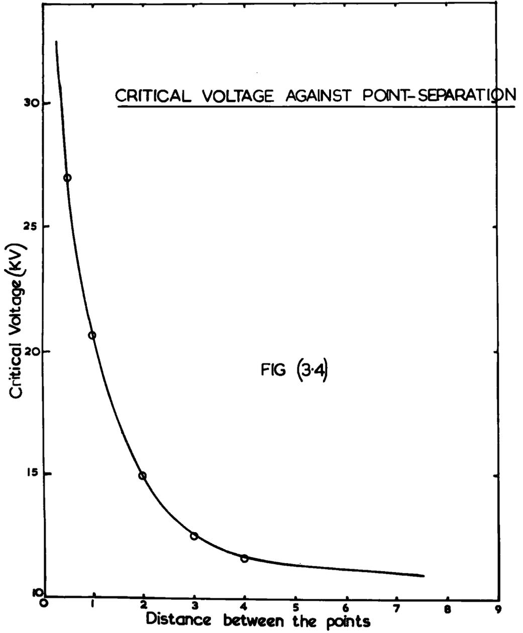
observed by CHIPLONKAR (1940) and CHALMERS and MAPLESON (1955). On the other hand for greater distances between the points, the critical voltage is very low, so even for lower fields (above the critical voltage), the multiple point-discharge current is always more than through a single point and agrees with what was observed by SIVARAMAKRISHNAN (1957) and BELIN (1948).
