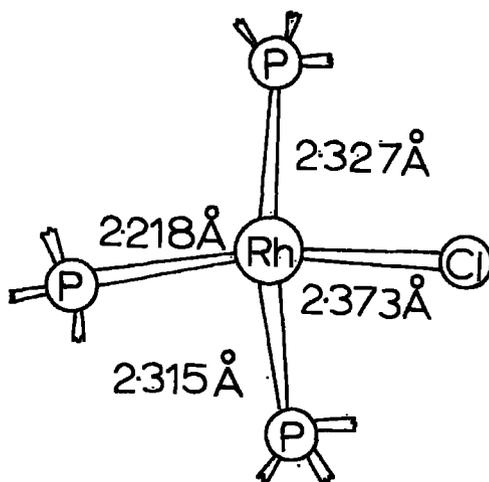
Fig. 5 Bond lengths in  $(\text{Ph}_3\text{P})_3\text{RhCl}$
