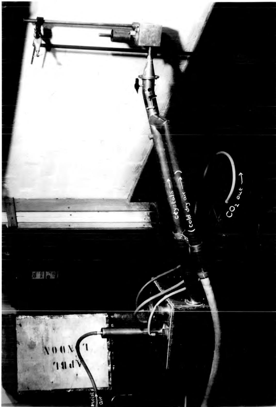
Fig. 14. Ice System for growing ice crystals.
