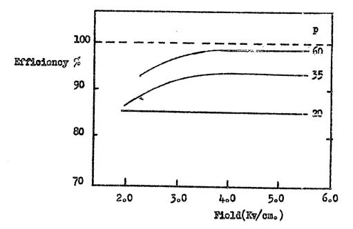
Fig. 2.6(a) The efficiency, field characteristics, with gas pressure (cm.Hg) as parameter. Tp=3.2 $\mu$  sec, TR= 0.5 $\mu$  sec,  $\tau = 4 \mu$  sec.
