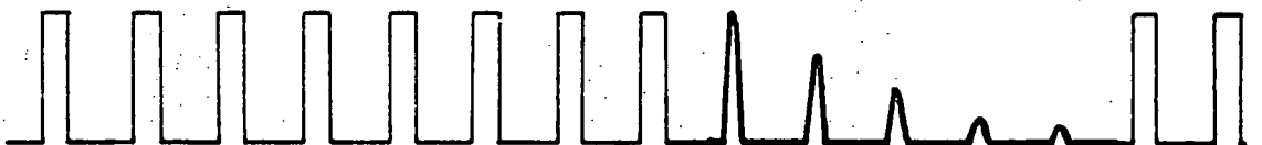
FIGURE 5.21: Pulse superposition : omission of RF pulses from input train to allow observation of maximum.
