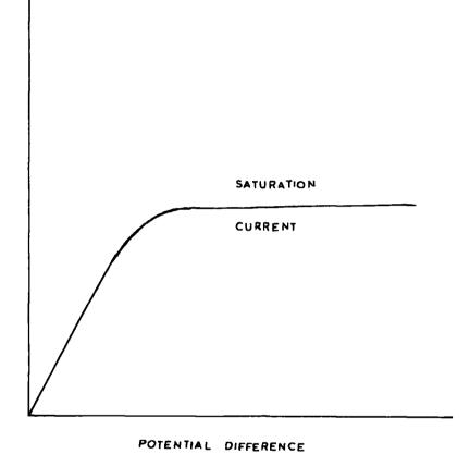
FIG. 1. IONIC AND SATURATION CURRENT
