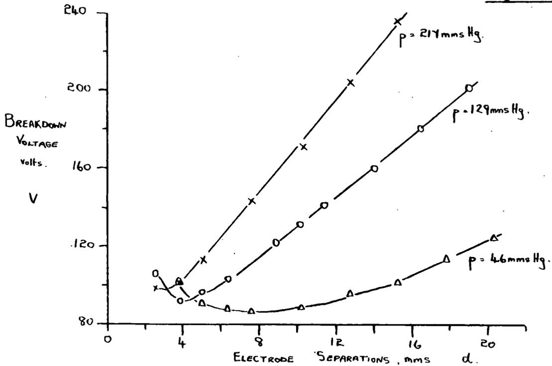
Fig. 40. Neon. Variation of Breakdown Stress with Gas Pressure.
