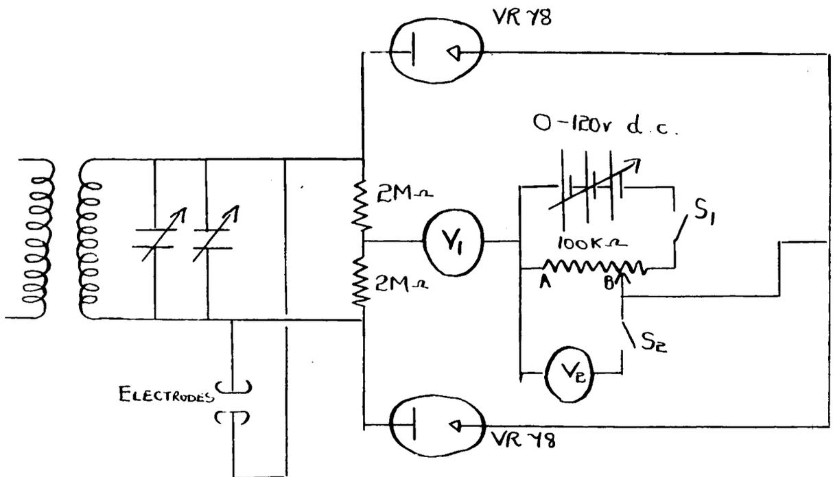
(iii) Pye Scalalamp electrostatic voltmeter (high range)
