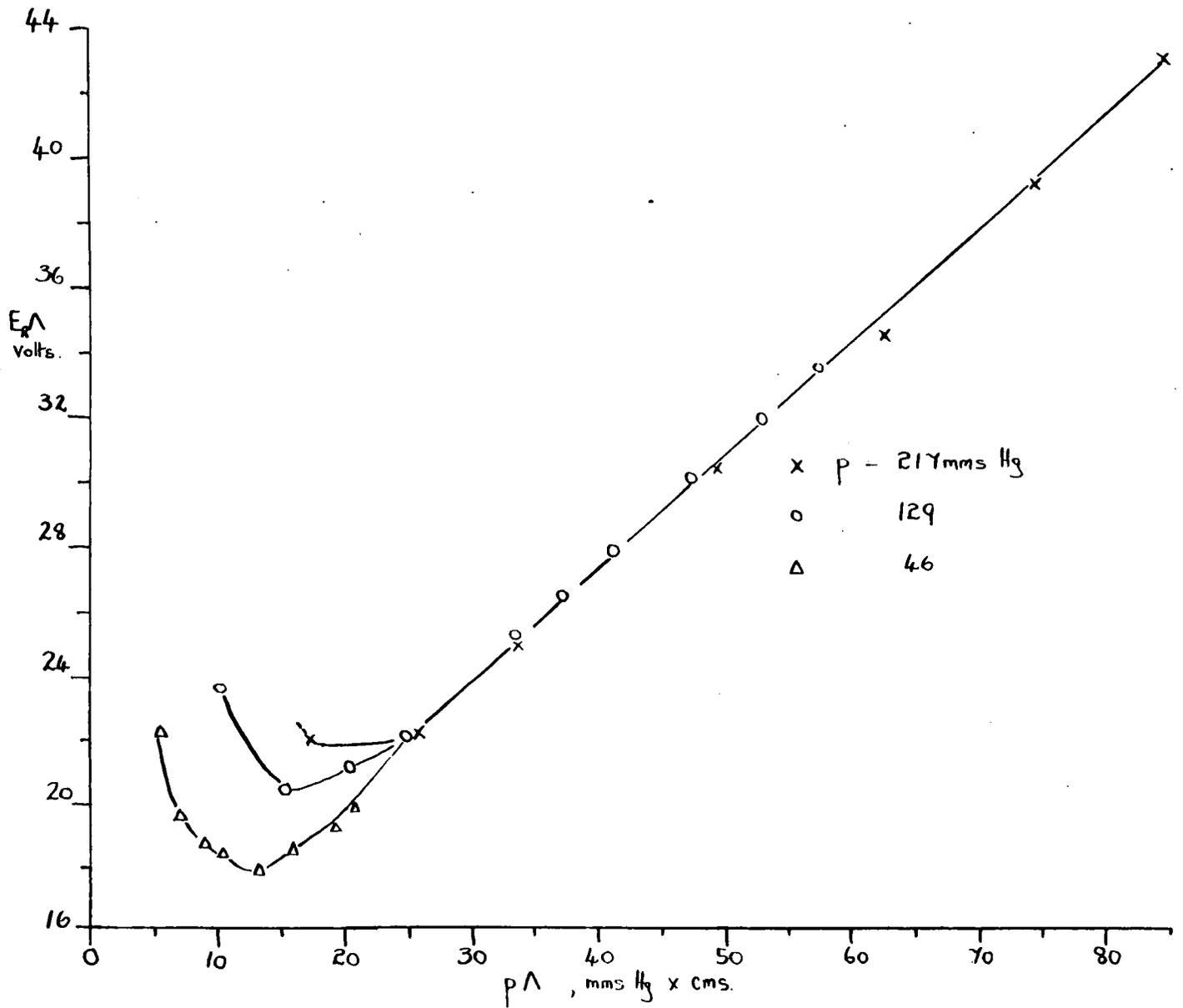
measurements, using values of  $\Lambda$  determined on the assumption that the mean life of an electron within the gap is limited by diffusion processes alone. Since "A"-type Rogowski electrodes were used in all the neon measurements, values of  $\Lambda$  in terms of the electrode separation were calculable directly from Fig. 20.
