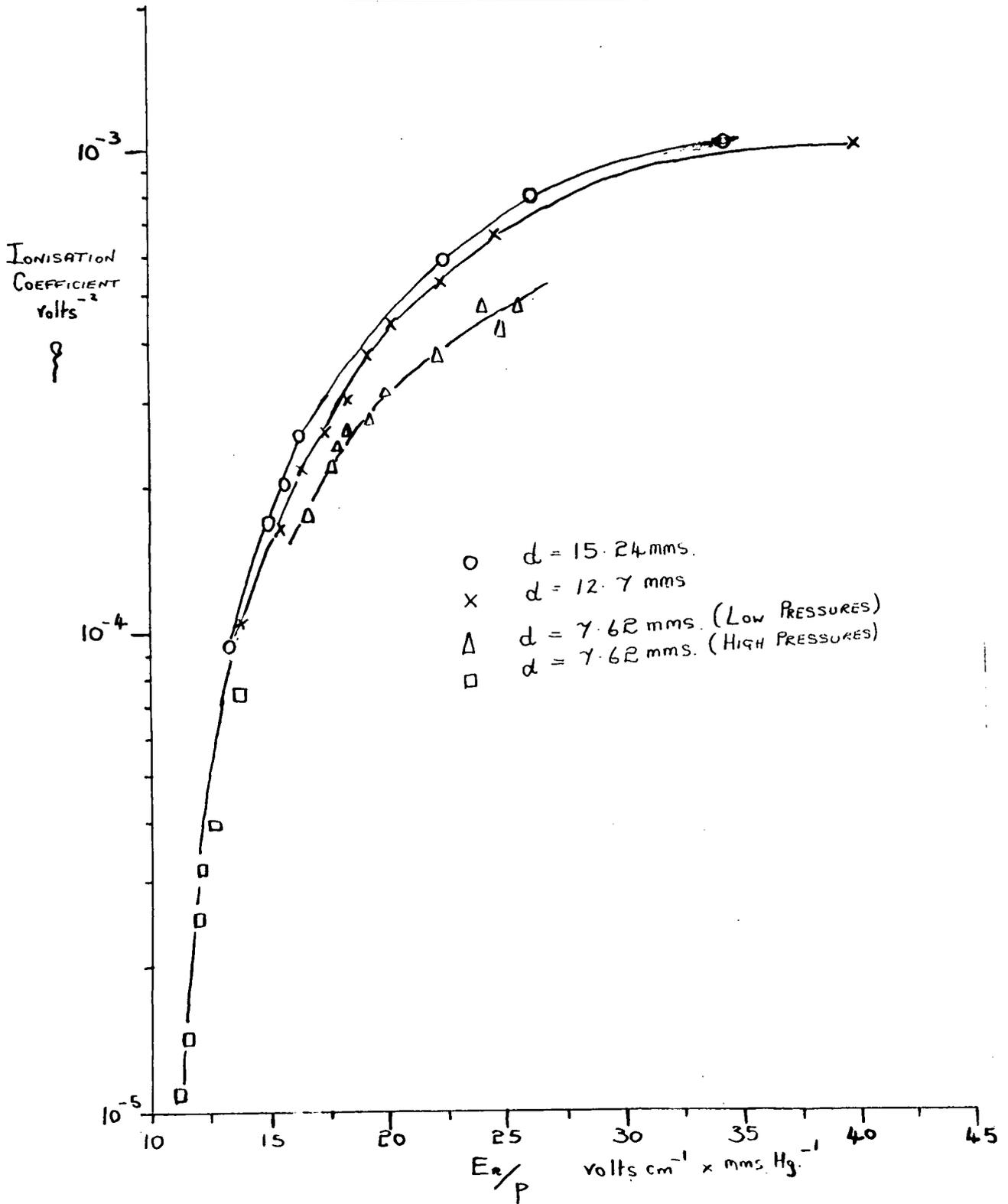
Under u.h.f. conditions, the drift velocity of electrons is produced by diffusion instead of mobility motion, and a 'high frequency' ionisation coefficient may be introduced (Brown 1951), analogous to the first Townsend coefficient; 3 .
