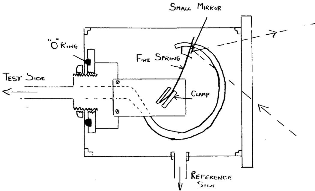
Fig. 9(b) Moving Bellows Gauge
