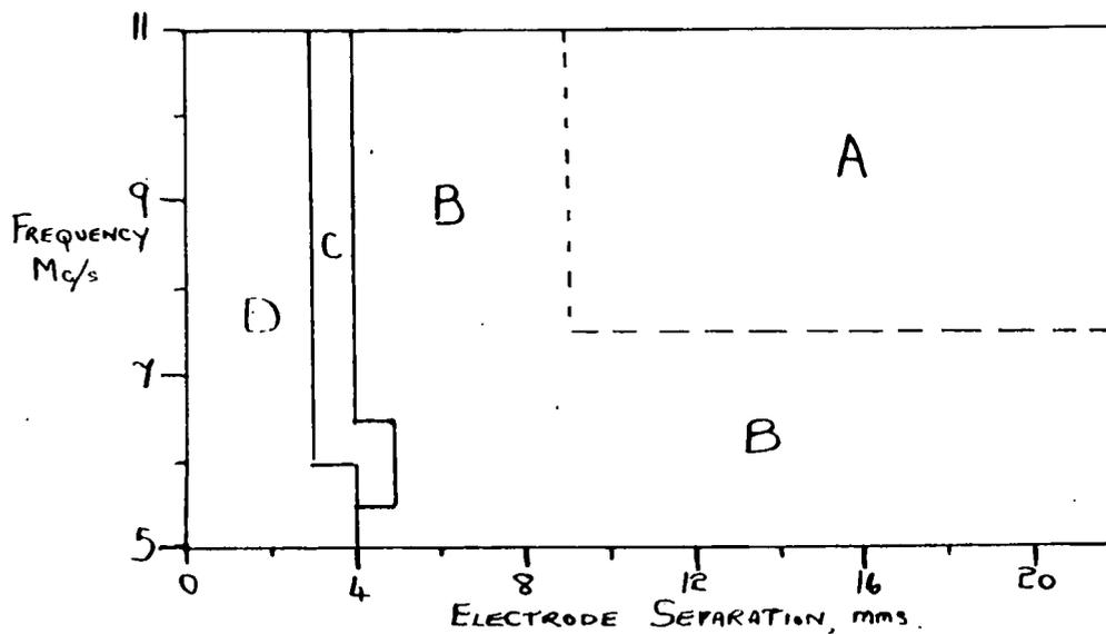
A record was kept, for each of the several hundred discharge measurements in hydrogen, of the form of the discharge; the mode appearing under a given set of conditions was found to be a function of gas pressure, electrode separation and frequency.
