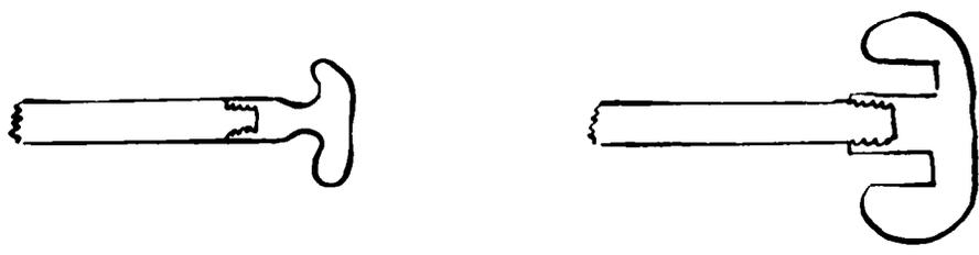
surface on to a distant screen upon which were drawn Rogowski profiles of different sizes, corresponding to the diameter of each set of electrodes required. A diagram of the apparatus is shown in Fig. 6 (a). Such factors as lens magnification, distance between lens and screen, optimum illumination, etc., were determined by a set of preliminary experiments.
