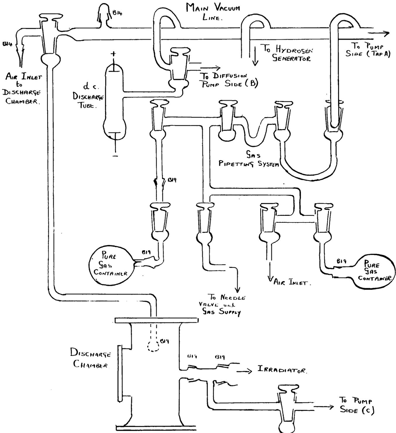
to give a rough indication of vacuum conditions in either the test or diffusion pump sides of the system, the glow discharge 'blacking out' below a pressure of about  $10^{-2}$  mms.Hg. The tube was stressed by a 7 Kv. d.c. supply, with large series resistors to limit the current.
