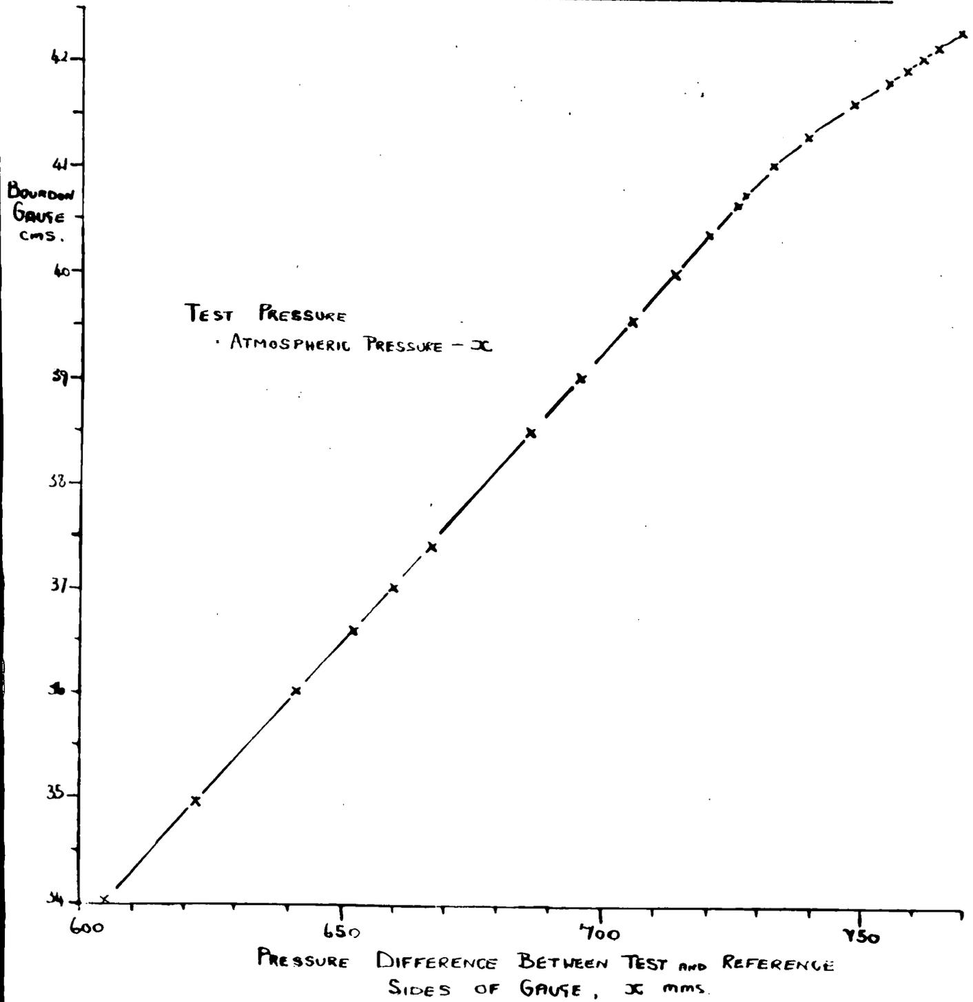
and mercury manometer. Further readings were then taken until air in the reference side reached atmospheric pressure.
