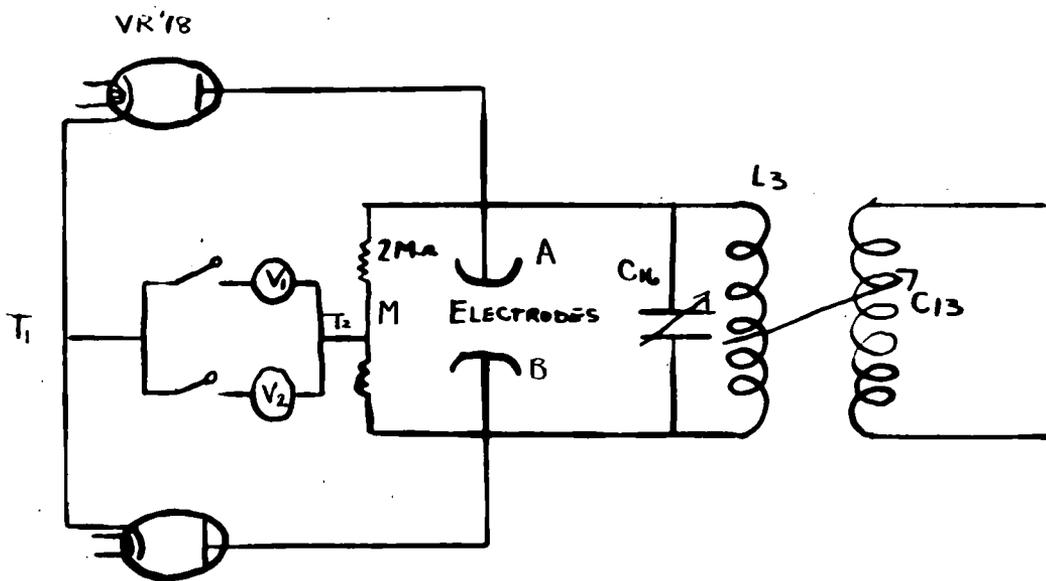
voltage required being coarsely and finely adjusted by C13 and C15 respectively. Working under these conditions, the power input associated with a given pre-breakdown voltage across the electrodes was as small as possible.
