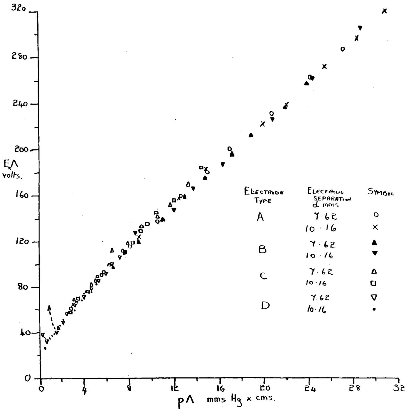
between similar electrodes separated by the different gaps shows that a smaller stress was necessary to initiate breakdown in the larger gaps. This phenomenon has already been encountered - Fig 18 - and may be explained by considering relative diffusion losses to the electrodes.
