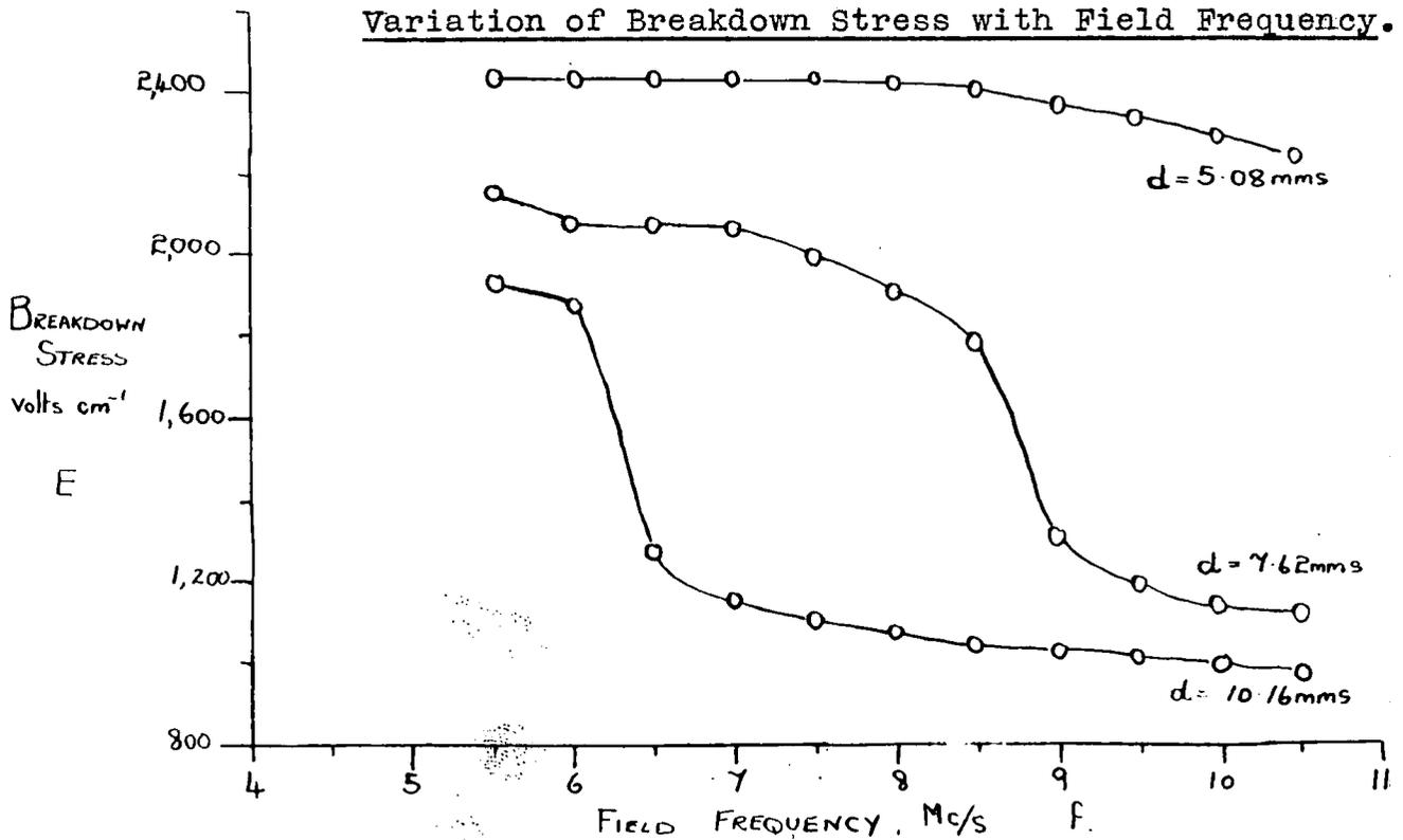
The calculations confirm that at the top of each "step" the amplitude of electron oscillation is very close to the gap spacing; at the bottom electrons are free to oscillate within the gap each half-cycle of the field. Discharges at separations exceeding this value constitute true u.h.f. breakdown.
