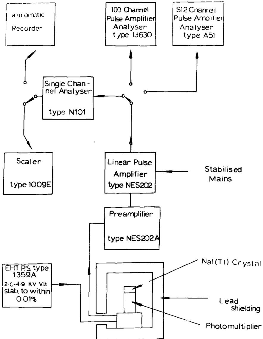
Fig. 1 Block diagram of the circuits used for scintillation counting.
