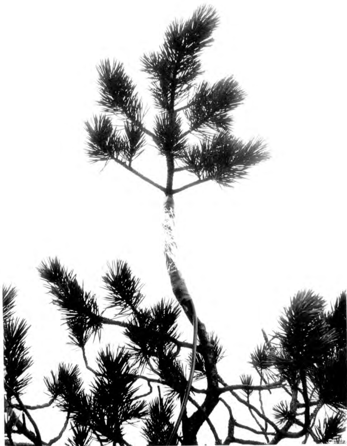
FIG. 9.6A POINT DISCHARGE PULSE DETECTOR - THE ELECTRODE.
