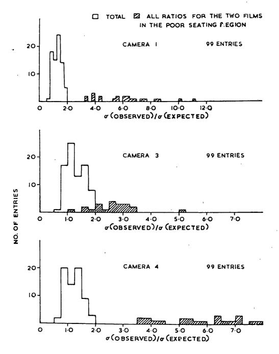
is difficult to understand since each camera was served by the same vacuum. At best the distributions for the other two cameras correspond to a standard deviation in the setting error of ~30 $\mu$  instead of the expected 5 $\mu$ .
