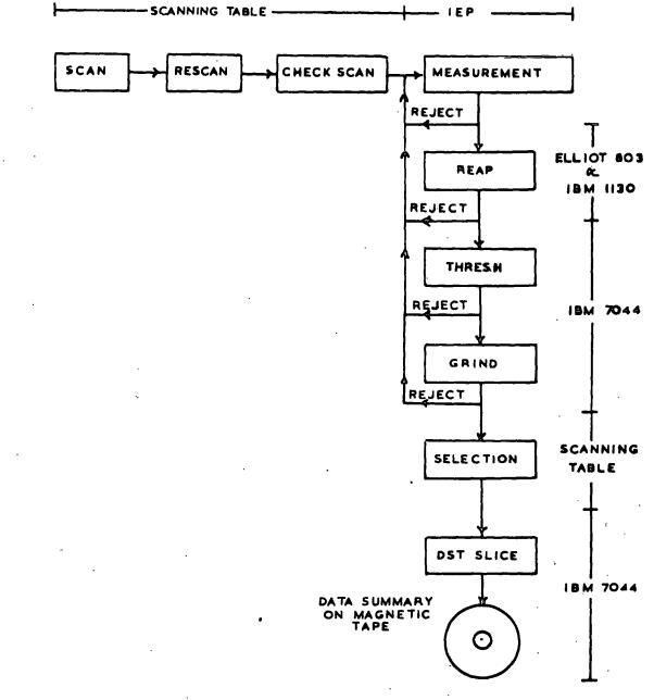
Gev/c (24 rolls) film was scanned on two Prevost machines designed to project images of the three films from the cameras onto a horizontal table with a magnification of  $\sim 14x$ . Two of the images overlapped for ease of reference where stopping or dipping tracks were concerned.
