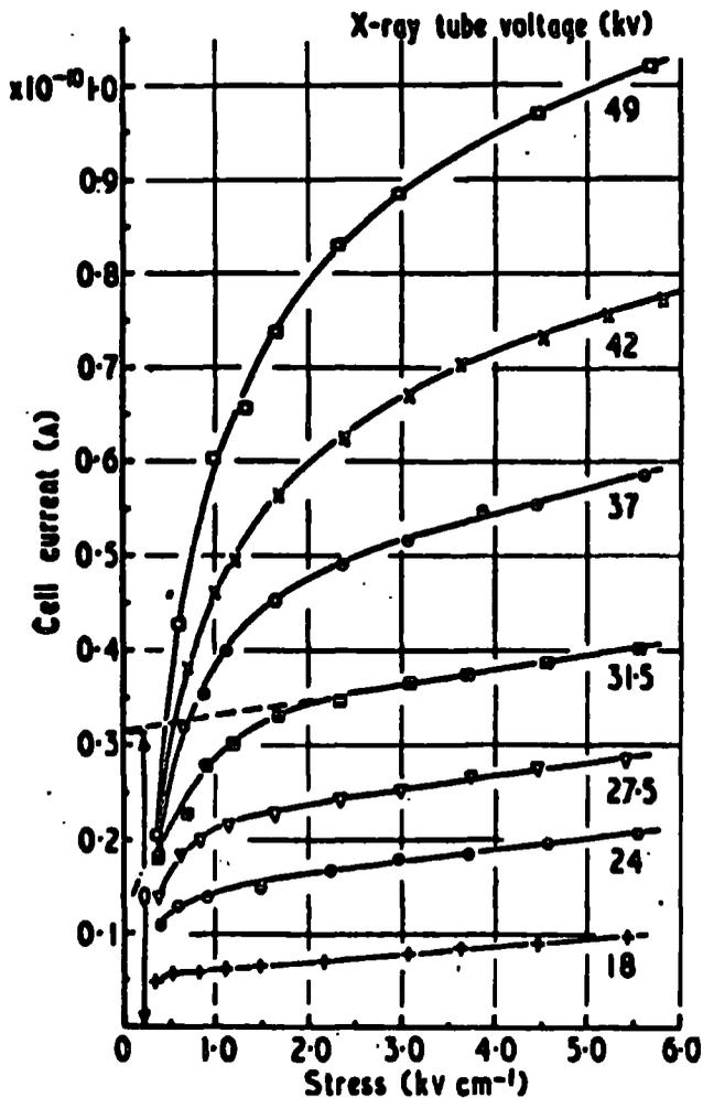
Conduction characteristics of *n*-hexane filled test cell. Molybdenum target in x-ray tube through which electron current of 2.4 mA flowed. Foil electrode negative.<sup>19</sup>
