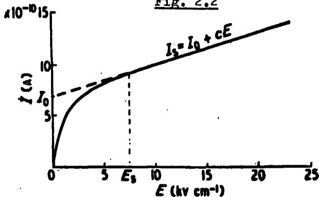
Current-voltage characteristic of induced conduction in a dielectric liquid.<sup>8</sup>
