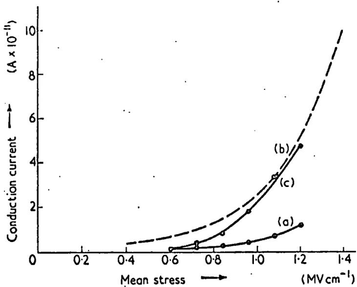
*The conduction current of liquid hexane as a function of the mean stress. (a) Purified hexane saturated with air; (b) Purified and degassed hexane; (c) Commercial hexane saturated with air.*
