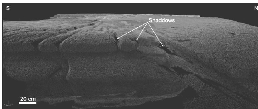
**Fig. 2.1.** A perspective view of a 3D point-cloud, acquired using TLS methods. The scan is of a faulted wave-cut-platform from Lilstock, Somerset, UK (See **Fig. 2.12**). Areas not in the direct line of sight of the scanner are left blank and shadows are cast over the outcrop. In this image multiple scan positions are combined to maximise data coverage.
