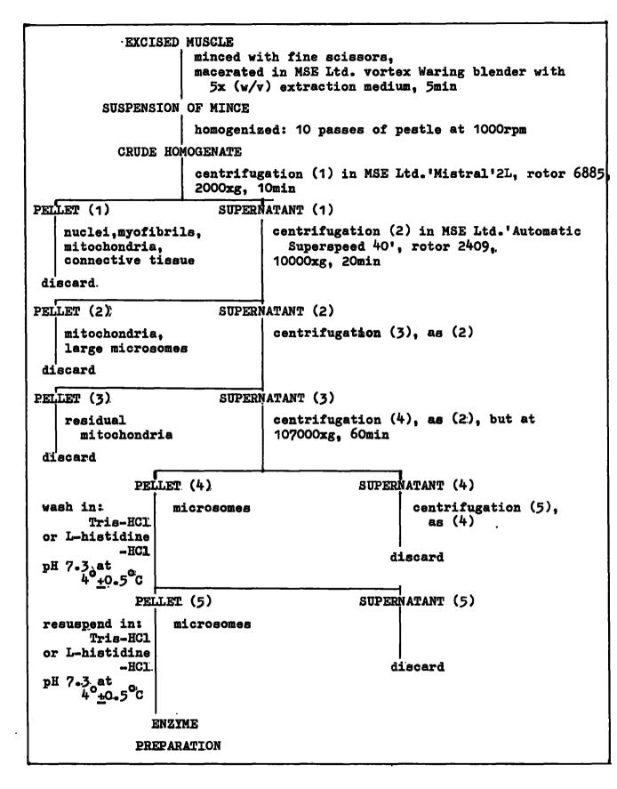
FIG. III-1. PROCEDURE FOR EXTRACTION OF SKELETAL MUSCLE MICROSOMES.
