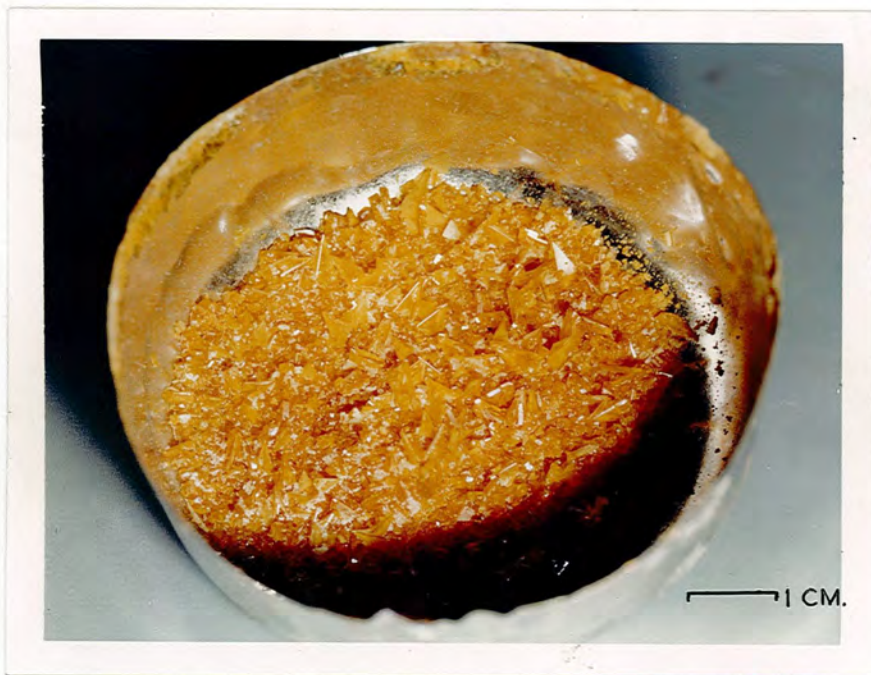
Crystals as grown before removal from crucible. (see Chapter 3)
