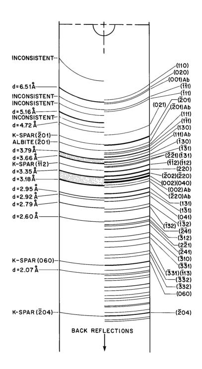
intensity by comparison with their fading, originally strong neighbours, and show slight differences in spacing from the original feldspar planes, they are interpreted as belonging to a high-pressure phase (or phases). The resulting twelve strong reflections and four uncertain lines representing onr or more high-pressure phases are listed in Table IV.5 and depicted in a schematic Debije-Scherrer pattern in Figure IV.12.
