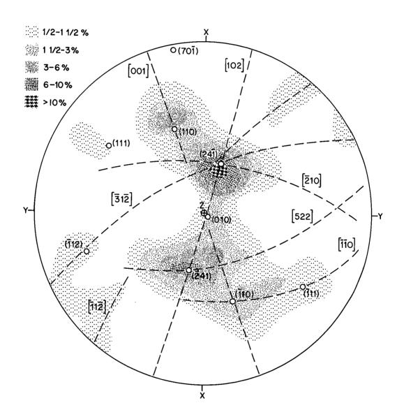
these shock-induced planes occurs in the [001] zone, 62° from (010) and near (110), although (430) is the low-index orientation nearest the focus of the planes.
