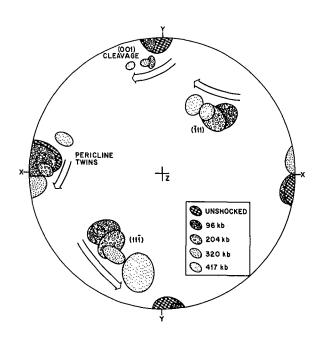
counter-clockwise migration is consistent and thus the twin-like features in the 417kb sample which plot near the rhombic section of the unshocked sample cannot be original pericline twins.
