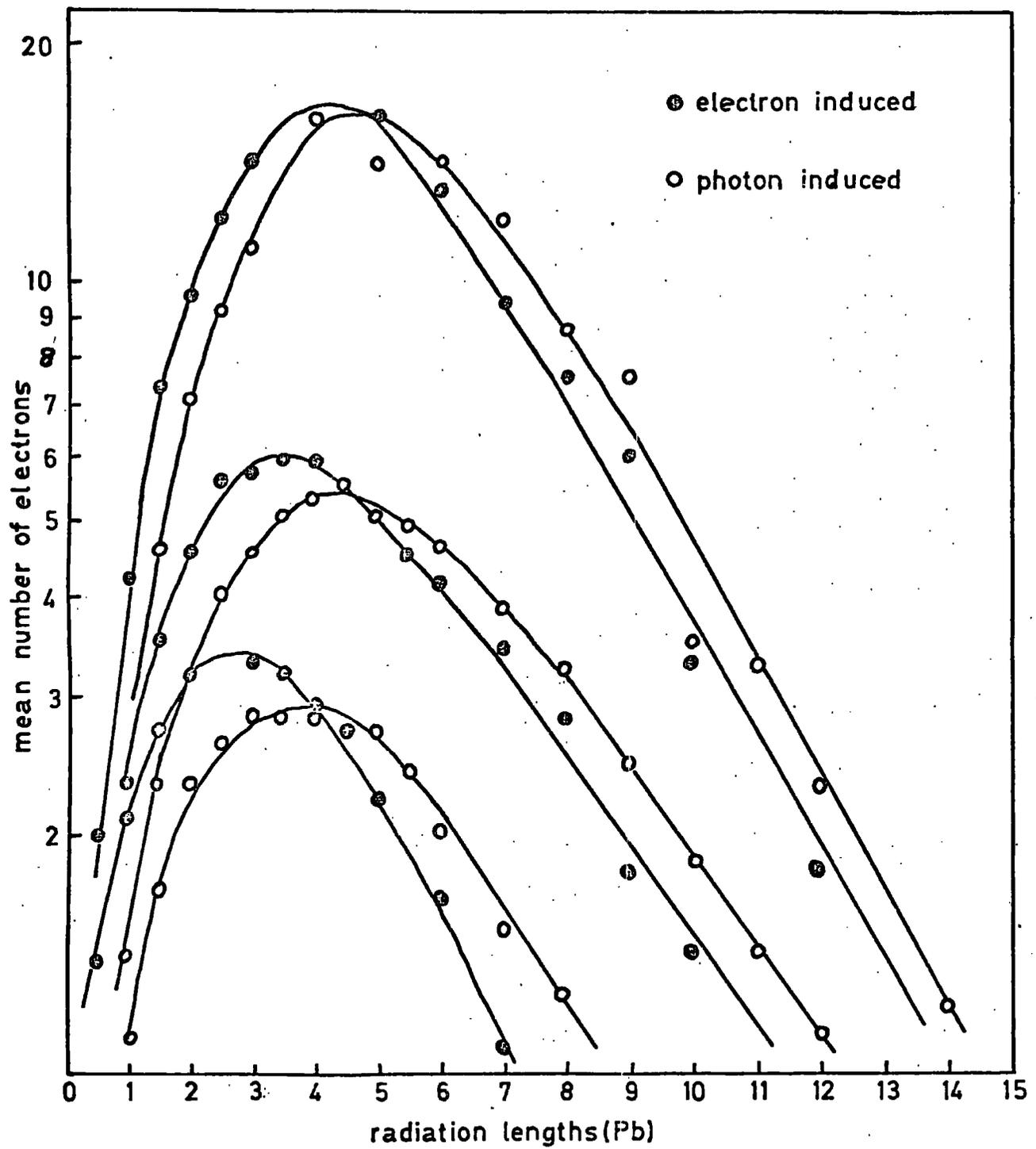
FIGURE 40 mean number of electrons produced as a function of target depth and primary energy
