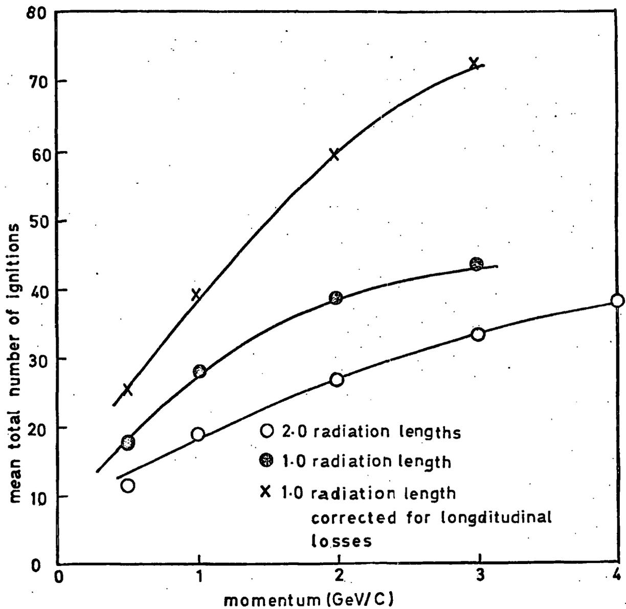
FIGURE 38 Mean total number of tubes igniting versus positron energy
