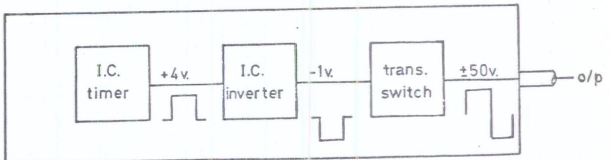
FIGURE 27 generation of square wave clearing field
