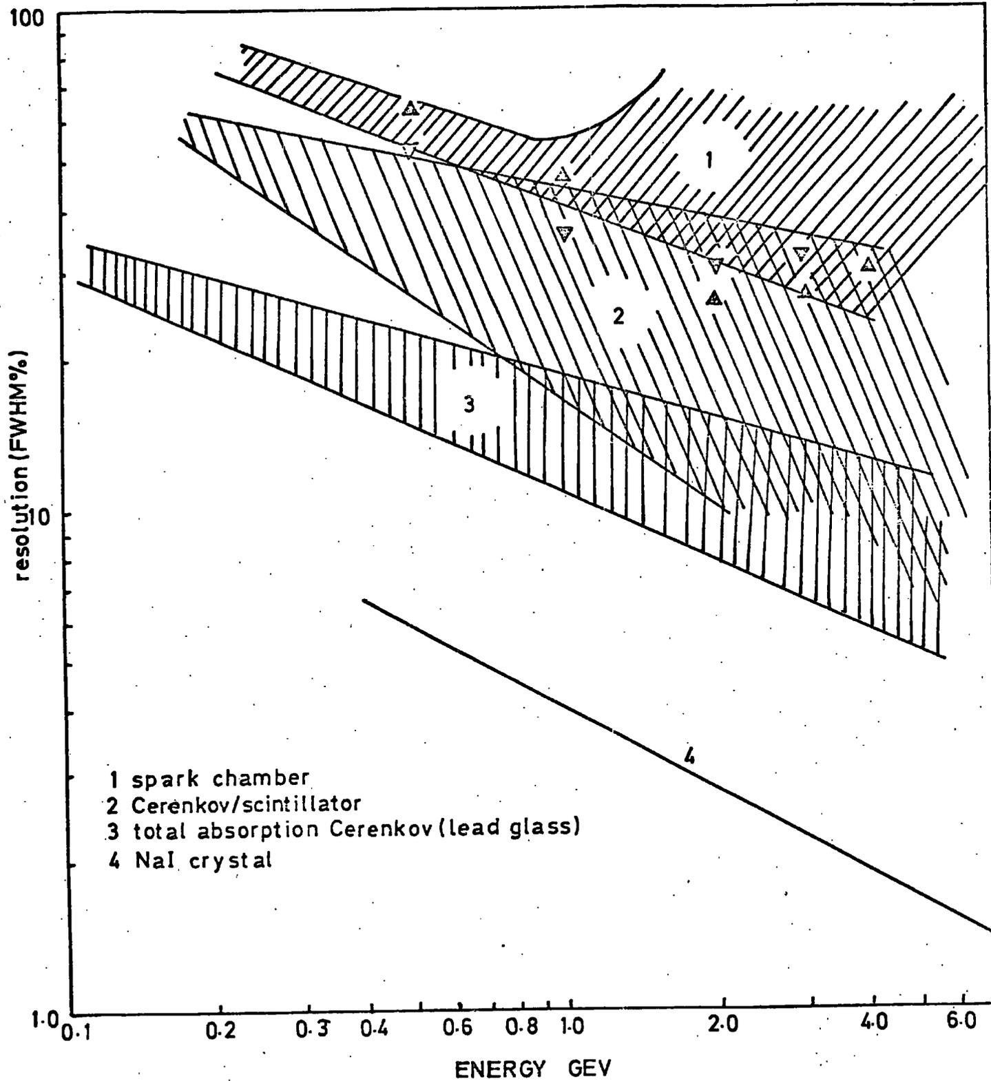
FIGURE 37 energy resolution of gamma ray detectors
