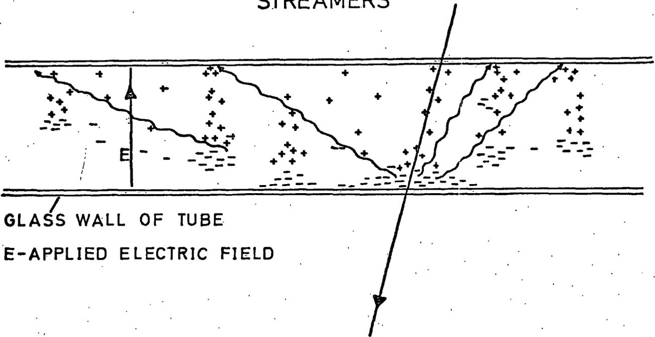
FIGURE 9 DISCHARGE WITH PRODUCTION OF STREAMERS
