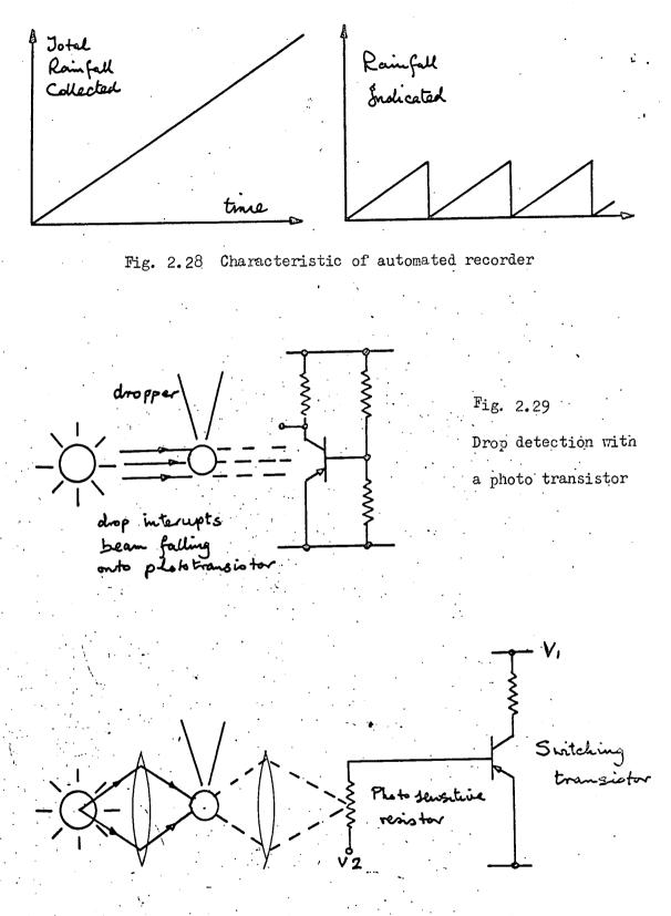
Fig. 2.30 Drop detection with a photo resistor
