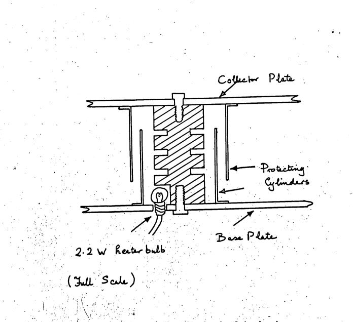
Fig. 2.5 The collector insulator housing
