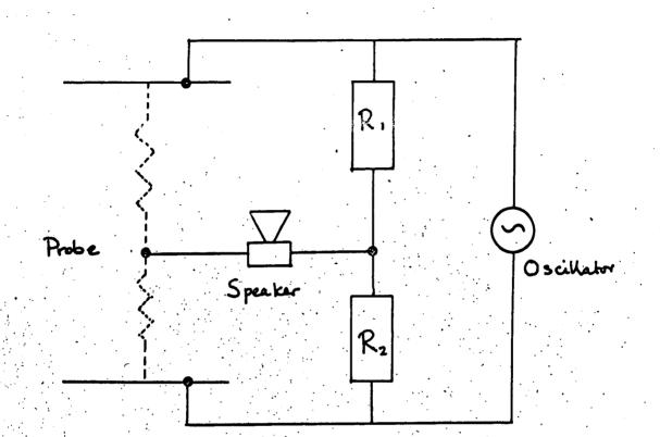
Fig. 2.7 Schematic arrangement of electrolytic tank experiments
