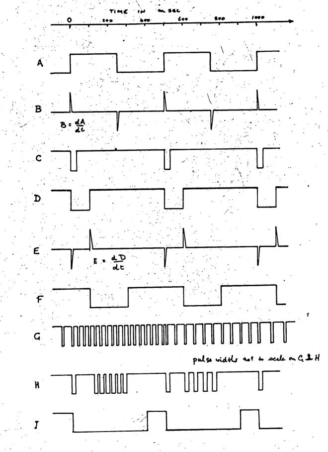
Fig. 10.1 Wave forms in automatic recording system
