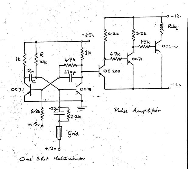
Fig. 2.27 Electronics of the rainfall recorder
