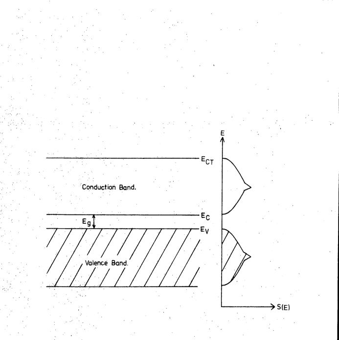
Fig.2-1. Energy Band Diagram of an Intrinsic Semiconductor.
