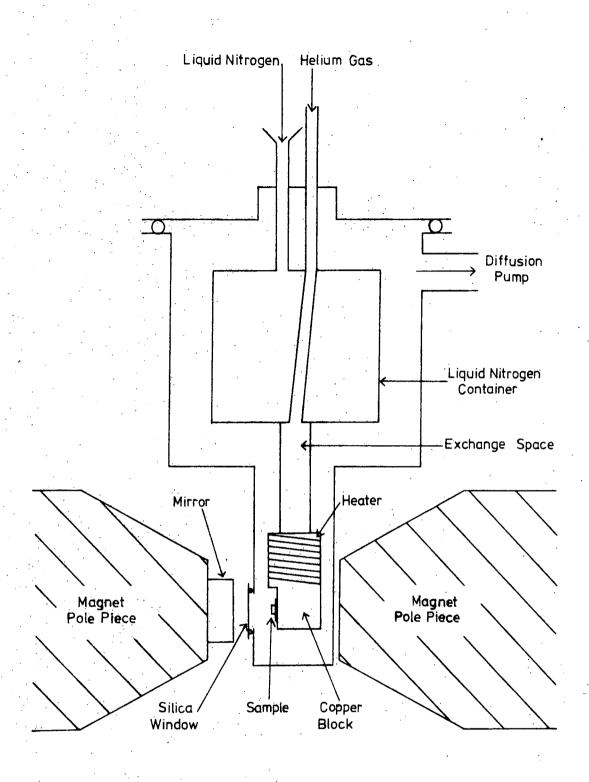
Fig.4-3. Cryostat used for Hall Effect Measurements.
