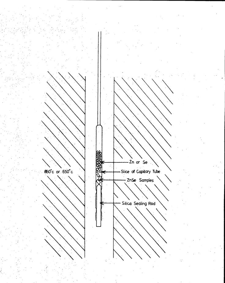
Fig. 3-4. Tube used for heating ZnSe in various molten Elements and Alloys.
