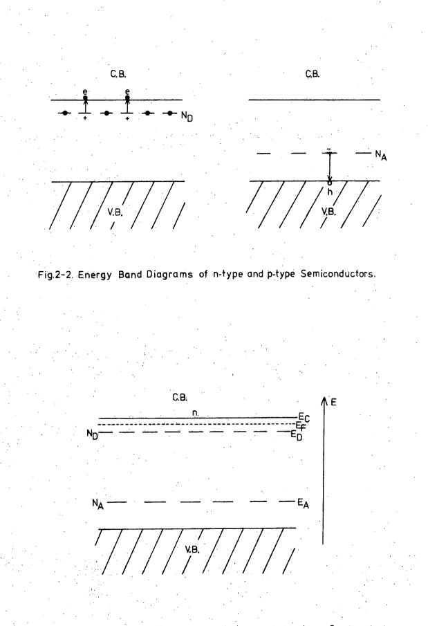
Fig.2-3. Energy Band Diagram of a Compensated n-type Semiconductor.
