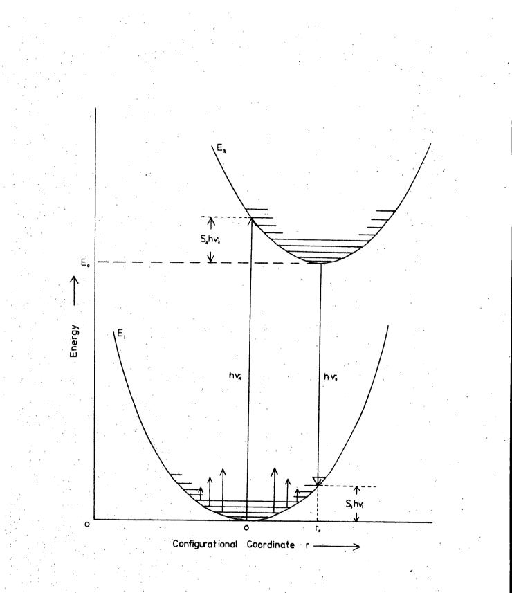
Fig 1-5 A typical Configurational Coordinate Diagram.
