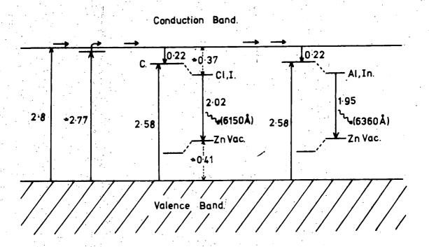
Fig. 5-36. Excitation and Emission Processes present in S.A. ZnSe at 85°K.
