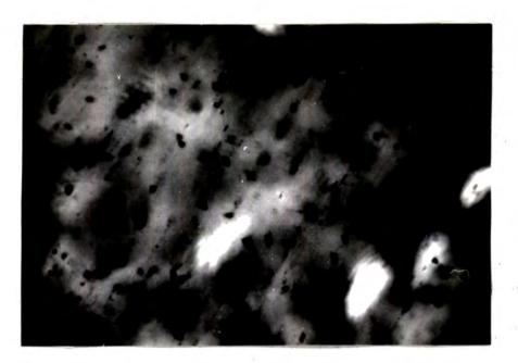
Fig. 7-11. Transmission Photomicrograph of ZnSe:In 139 heated in Zn. (×350)
