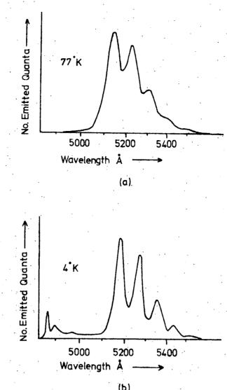
(b). Fig.1-1. Edge Emission Spectrum of CdS (C.C.Klick 1953)
