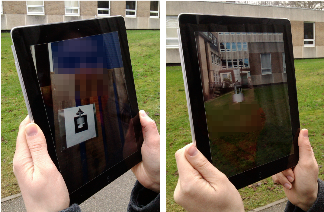
(a) Before the camera switch. The virtual object is tracked using the marker over the user's shoulder. (b) After the camera switch. The virtual object is tracked using the inertial sensors, and shown over the scene in front of the user.
