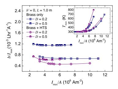
**Figure 5.12** Calculated average helium boil-off per unit current  $(b/I_{\max})$  for two vapour-cooled brass current leads and maximum temperature (inset) as a function of the ratio between maximum current and cross-sectional area  $(I_{\max}/A)$  of each lead with and without HTS tapes at x=0 m to x=0.5 m from the total length of 1.0 m. The system has no static or sample boiling.
