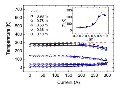
**Figure 5.14** Temperature of a 10-mm<sup>2</sup> current lead as a function of applied current ramping at 6 As<sup>-1</sup> up to 300 A. The inset shows temperature profile at the current of 300 A. Dashed lines are calculations using Equations (5.1) - (5.3) with  $m = \tilde{\rho}_{\text{liquid}}b$  from the experiment. Solid lines are calculations including the convective-like cooling effect near the top end.
