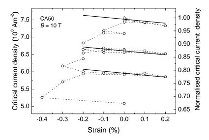
**Figure 4.14** Critical current density as a function of strain for the DI-BiSCCO CA50 tape at 4.2 K for the applied magnetic field of 10 T normal to the tape surface. The solid lines have constant gradient which is equal to the gradient in Figure 4.13. The normalisation constant is 364.0 A.
