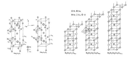
**Figure 3.3** The crystal structures of YBCO and BiSCCO. YBCO has orthorhombic perovskite structure with two CuO<sub>2</sub> planes and perpendicular CuO chains. BiSCCO family has tetragonal structure with different number of CuO<sub>2</sub> planes for different phase members [104].
