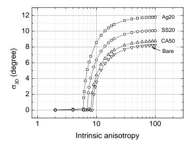
**Figure 7.9** The standard deviation of the misalignment angle ( $\sigma_{3D}$ ) versus intrinsic anisotropy for the DI-BiSCCO Ag20, SS20, CA50 and bare tapes calculated from (7.3) where the scaling function at  $\theta = 0^{\circ}$  is obtained from the experiments.
