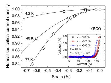
**Figure 5.24** Normalised critical current density of YBCO tapes as a function of strain at 4.2 K, 40 K and 77 K. The inset shows voltage-current characteristics of a YBCO tape at 40 K as a function of applied strain with the magnetic field applied normal to the tape surface.
