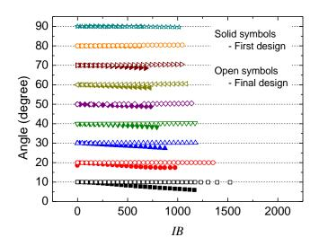
**Figure 5.3** Instantaneous angle between magnetic field and the sample's surface as a function of the product of the current and the applied magnetic field for  $J_c$  measurements on a DI-BiSCCO tape at 4.2 K at different starting angles. The applied magnetic field was 3 T for the first design and 14 T for the final design.
