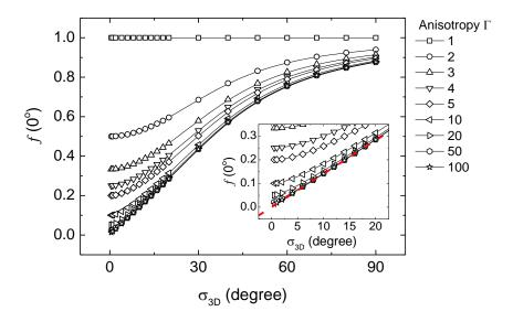
**Figure 7.8** The calculated scaling function at  $\theta = 0^{\circ}$  as a function of standard deviation of the *c*-axis misalignment angle  $(\sigma_{3D})$  for various values of the intrinsic anisotropy  $(\Gamma)$ . The inset is the same plot in a different scale. Dotted line in the inset is  $\sigma_{3D} = \sigma_{2D} = 70.9 f(0^{\circ})$  from (4.3).
