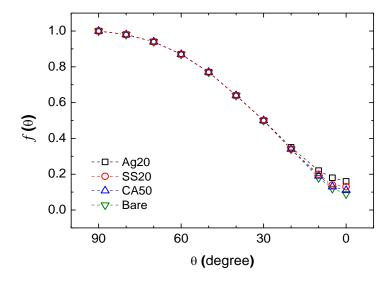
**Figure 4.10** The scaling function  $f(\theta)$  for four different types of the DI-BiSCCO tapes calculated by normalising  $B_{\perp}(\theta)$  with respect to  $B_{\perp}(90^{\circ})$ . The scaling function generally follows  $\sin\theta$  except at the low angles  $(\theta < 20^{\circ})$ .
