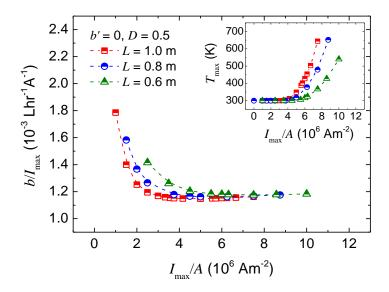
**Figure 5.9** Calculated average helium boil-off per unit current  $(b/I_{\rm max})$  for two vapour-cooled brass current leads and maximum temperature (inset) as a function of the ratio between maximum current and cross-sectional area  $(I_{\rm max}/A)$  of each lead without any static or sample boiling for the duty cycle of 0.5 and the current lead's lengths of 0.6, 0.8 and 1.0 m. The maximum current investigated was 1000 A.
