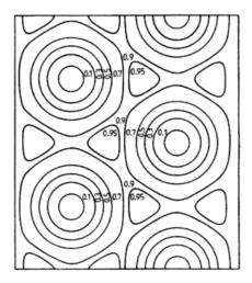
**Figure 2.3** Level surfaces of normalised  $|\psi|^2$  for the triangular vortex lattice, which also represent the lines of constant magnetic field and constant current flow [17].
