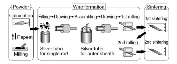
Figure 3.5 Bi-2223 wire manufacturing process with PIT technique [128].
