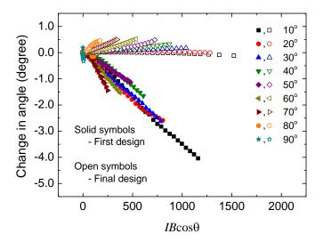
**Figure 5.4** Data from Figure 5.3 replotted as the change in the angle during the  $J_c$  measurement as a function of the product of the current (I), the applied magnetic field (B) and the cosine of the instantaneous angle between magnetic field and the sample's surface at different starting angles.
