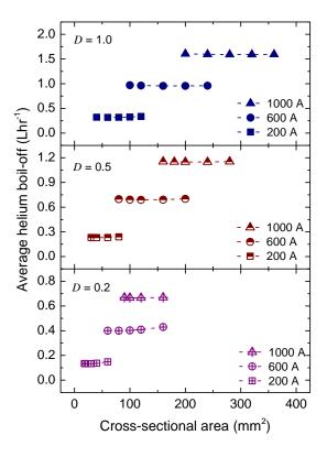
**Figure 5.8** Calculated average helium boil-off (averaged over 10 cycles) for two vapour-cooled brass current leads as a function of the cross-sectional area of each lead carrying a current up to 200, 600 and 1000 A for duty cycles of 0.2, 0.5 and 1.0. The system has no static or sample boil-off and the length of all current leads is 1.0 m.
