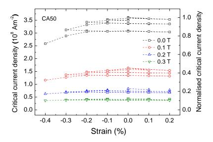
**Figure 4.12** Critical current density as a function of strain for the DI-BiSCCO CA50 tape at 77 K at different applied magnetic fields normal to the tape surface. The critical current densities were also normalised with the normalisation constant of 173.7 A.
