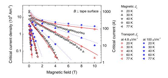
**Figure 7.11** Magnetic and transport critical current densities determined at the electric fields of 4.8  $\mu$ Vm<sup>-1</sup> and 100  $\mu$ Vm<sup>-1</sup> for the DI-BiSCCO tapes as a function of magnetic field applied normal to the tape surface at different temperatures. Solid lines are fits to the transport data at 4.8  $\mu$ Vm<sup>-1</sup> using (6.4) and (6.9). Dotted lines are fits to the data at 100  $\mu$ Vm<sup>-1</sup> using the same equations.
