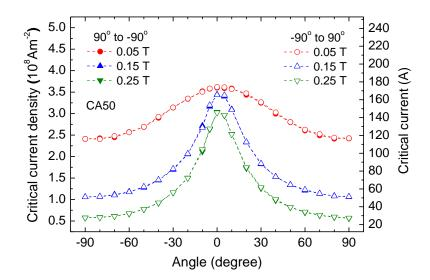
**Figure 4.8** Critical current density as a function of the angle between applied magnetic field and the surface of the DI-BiSCCO CA50 tape at 77 K at two different directions of changing the angle. No angular hysteresis was observed.
