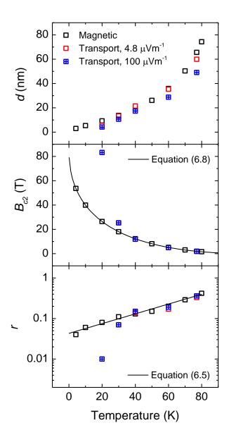
**Figure 7.12** Half-thickness (*d*) of the junction, upper critical magnetic field ( $B_{c2}$ ) and ratio (*r*) between normal state resistivities of the superconducting grains and the junctions fitted to the magnetic and the transport  $J_c$  data as a function of temperature.
