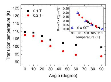
**Figure 7.5** Transition temperature at 1 % of the normal state resistance as a function of angle between magnetic field and the surface of the DI-BiSCCO bare tape for the magnetic fields of 0.1 T and 0.2 T. The inset shows data replotted as a function of  $B(\sin^2\theta + \Gamma_{\rm eff}^{-2}\cos^2\theta)^{1/2}$  where  $\Gamma_{\rm eff} = 8.5$ . Data from Figure 7.2 for fields applied normal to the tape surface are also plotted for comparison.
