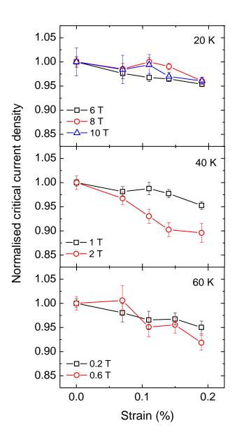
**Figure 7.14** Normalised critical current density of a DI-BiSCCO CA50 tape as a function of applied strain at 20 K, 40 K and 60 K at different magnetic fields applied normal to the tape surface. The normalising constants are values of the critical current density at zero applied strain.
