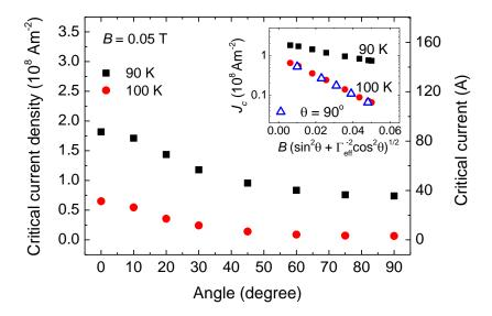
**Figure 7.13** Critical current density of a DI-BiSCCO bare tape as a function of angle between applied magnetic field and the tape surface for the magnetic field of 0.05 T at 90 K and 100 K. The inset shows data replotted as a function of  $B(\sin^2\theta + \Gamma_{\rm eff}^{-2}\cos^2\theta)^{1/2}$ . Data for fields applied normal to the tape surface at 100 K are also plotted for comparison.
