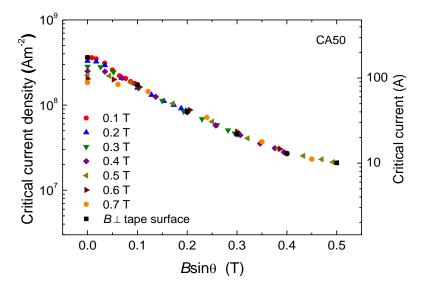
**Figure 4.7** Critical current density as a function of the field component normal to the surface  $(B\sin\theta)$  of the DI-BiSCCO CA50 tape at 77 K. Data for the field applied normal to the tape surface are made more explicit for clarity. Deviation from the universal relation occurs at low fields due to the grain misalignment.
