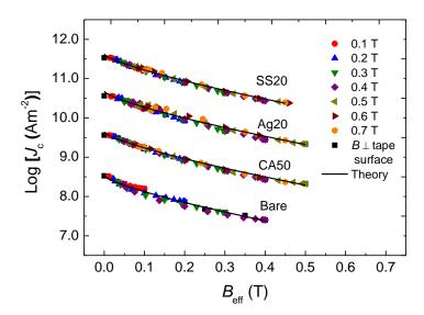
**Figure 4.11** Critical current density as a function of the effective normal magnetic field for the DI-BiSCCO tapes at 77 K. The data for each tape are increased sequentially by 1 from the bare tape for clarity. Solid lines are plots of (4.4).
