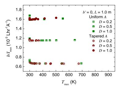
**Figure 5.10** Calculated average helium boil-off per unit current  $(b/I_{\rm max})$  for two vapour-cooled brass current leads as a function of maximum temperature with uniform cross-sectional area and tapered cross-sectional area. The system has no static or sample boiling and the length of all current leads is 1.0 m. The maximum current investigated was 1000 A.
