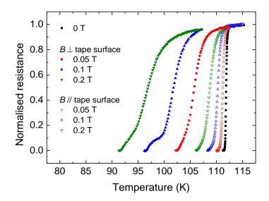
**Figure 7.2** Normalised resistance versus temperature for the DI-BiSCCO bare tape as a function of magnetic field applied normal and parallel to the tape surface. In both orientations, the magnetic field was normal to the current flow.
