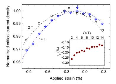
**Figure 6.7** Normalised critical current density of YBCO tape at 4.2 K as a function of applied strain for the magnetic fields of 2 T and 14 T applied normal to the tape surface. Dotted lines are guides to the eye. The arrow shows peak strain  $(\varepsilon_p)$  for each magnetic field. The inset shows  $\varepsilon_p$  versus magnetic field.
