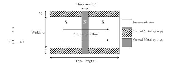
**Figure 6.1** Schematic diagram of the SNS junction model [221]. The junction consists of two superconducting components separated by a normal metal barrier that limits the current flow. This barrier represents the grain boundary in polycrystalline superconductor.
