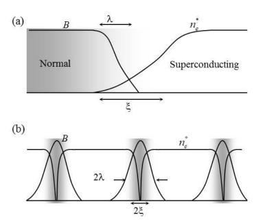
**Figure 2.4** (a) Increase in the number of superconducting electrons  $n_e^*$  and the decay of the magnetic field B at the interface of a type I superconductor. (b) Change in the number of superconducting electrons and magnetic field around three fluxons in the vortex state of type II superconductor.
