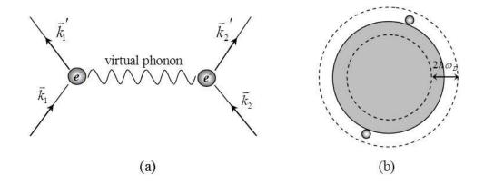
**Figure 2.6** (a) The pairing mechanism via exchange of a virtual phonon (with energy  $\hbar\omega_D$ ) - the momenta of two electrons change from  $\vec{k}_1$  and  $\vec{k}_2$  to  $\vec{k}_1'$  and  $\vec{k}_2'$  after the interaction. (b) The isotropic Fermi sphere of the electron system (the solid line shows the Fermi energy) - the new momenta  $\vec{k}_1'$  and  $\vec{k}_2'$  have to be above the Fermi surface since all orbitals below are filled.
