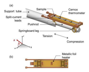
**Figure 5.18** (a) Diagram of the springboard-shaped sample holder and thermometry. (b) Metallic foil heaters underneath the sample holder.
