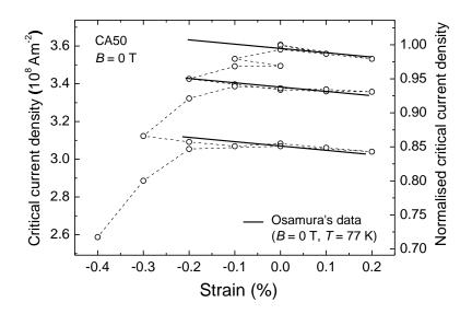
**Figure 4.13** Critical current density as a function of strain for the DI-BiSCCO CA50 tape at 77 K for zero field alone. The solid lines are similar to Osamura's data at 77 K in self-field [160]. The normalisation constant is 173.7 A.
