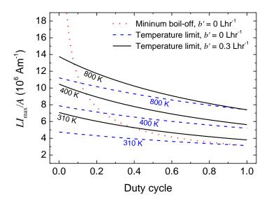
**Figure 5.13** Optimum shape factor ( $LI_{max}/A$ ) of the current lead for critical current measurements as a function of duty cycle calculated from (5.6) where the maximum temperature of the current lead is a limiting factor (dash and solid lines), in comparison with the optimum shape factor obtained at the minimum average helium boil-off for the current lead's length of 1.0 m (dotted line). For b' = 0.3 Lhr<sup>-1</sup>, the minimum boil-off gives a maximum temperature larger than 800 K.
