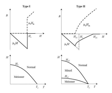
**Figure 2.2** Magnetic response in type I and type II superconductors. The Meissner state is found in type I superconductor below  $H_c$  while it is found below  $H_{c1}$  in type II superconductor before the superconductor enters the mixed state as the magnetic field increases. Eventually materials become normal when the field exceeds  $H_c$  in type I and  $H_{c2}$  in type II superconductors. These behaviours occur below  $T_c$ .
