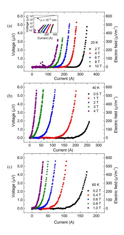
**Figure 7.10** Voltage-current characteristics of a DI-BiSCCO CA50 tape at 20 K (a), 40 K (b) and 60 K (c) for various magnetic fields normal to the tape surface. The inset in (a) is the log-log plot of the same data including the resistive curve of silver at 20 K.
