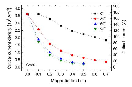
**Figure 4.4** Critical current density as a function of applied magnetic field at different orientations for the DI-BiSCCO CA50 tape at 77 K. The critical current density decreases more drastically when the fields are applied normal to the tape surface.
