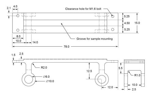
Figure 5.19 Technical drawings of the springboard-shaped sample holder.
