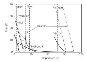
**Figure 3.1** Magnetic field versus temperature phase diagram of some common HTS in comparison with some LTS [95]. The thick solid lines show irreversible fields. The thin ones show upper critical fields.
