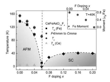
**Figure 3.4** Doping dependent phase diagram of CeFeAsO<sub>1-x</sub>F<sub>x</sub> iron-based superconductor determined from neutron measurements [107].
