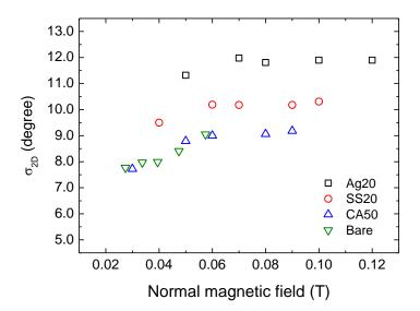
**Figure 4.9** Standard deviation of the misalignment angle as a function of magnetic field normal to the tape surface for four different types of the DI-BiSCCO tapes. To first order, the standard deviation is not dependent on magnetic field.
