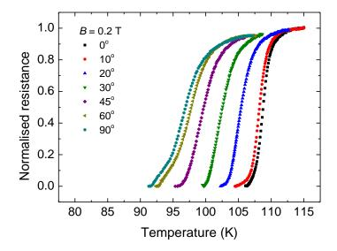
**Figure 7.3** Normalised resistance versus temperature for the DI-BiSCCO bare tape as a function of angle between magnetic field and the tape surface at 0.2 T. The magnetic field was normal to the current flow.
