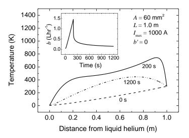
**Figure 5.7** Calculated temperature profile of a vapour-cooled brass current lead with the bottom end immersed in liquid helium while ramping current up to a maximum current of 1000 A in 200 s and then reducing the current to zero without any static or sample boiling (b' = 0). The current lead's length is 1.0 m and the cross-sectional area is 60 mm<sup>2</sup>. The inset shows calculated helium boil-off as a function of time.
