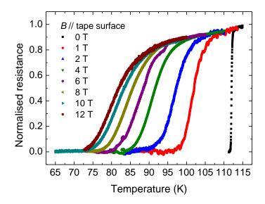
**Figure 7.1** Normalised resistance versus temperature for a DI-BiSCCO bare tape as a function of magnetic field applied parallel to the tape surface and the current flow. The applied current was 10 mA for B = 0 - 2 T and 100 mA for B = 4 - 12 T.
