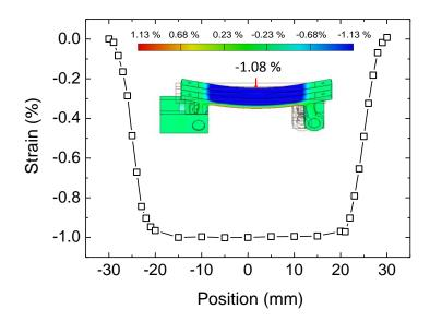
**Figure 5.20** Computational data of the strain homogeneity on the top surface of the 2.5-mm-thick springboard-shaped sample holder with an applied strain of -1.08 %. The inset shows a colour plot of the data from finite element analysis.
