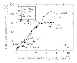
**Figure 3.7** Plot of  $T_c$  versus relaxation rate of cuprates, BKBO (solid squares), Chevrel-phase (C) and BEDT (solid star) systems based on  $\mu$ SR measurements; and of Nb and heavy fermion systems (inset) with the values of relaxation rate estimated from the bulk penetration depth measurements [140].
