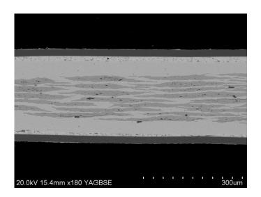
**Figure 4.1** SEM image of the transverse cross-section of a DI-BiSCCO SS20 tape. The tape consists of (in order, from outer surface) stainless steel lamination layers (dark grey), solder layers (light grey with black spots), silver/silver alloy matrix (light grey) and BiSCCO filaments.
