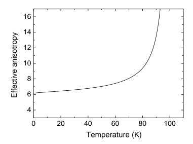
**Figure 7.7** Effective anisotropy of the DI-BiSCCO bare tape as a function of temperature calculated from  $B_{c2}(T,0^{\circ})/B_{c2}(T,90^{\circ})$  using  $B_{c2}(T)$  from (6.8) where  $T_c(90^{\circ}) = 101.6 \text{ K}$ ,  $B_{c2}(0,90^{\circ}) = 81.4 \text{ T}$ ,  $T_c(0^{\circ}) = 107.6 \text{ K}$  and  $B_{c2}(0,0^{\circ}) = 500.6 \text{ T}$  as obtained from the fits in Figure 7.6.
