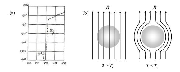
**Figure 2.1** (a) Electrical resistance of mercury as a function of temperature measured by Onnes, showing zero resistance state below  $\sim$ 4.2 K [8]. (b) Magnetic flux exclusion from superconducting material in Meissner state below  $T_c$ .
