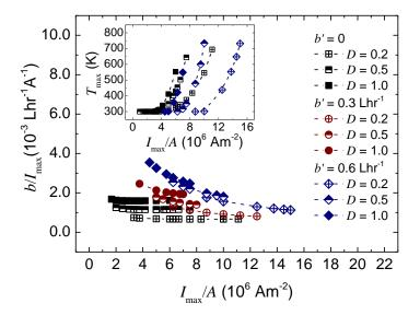
**Figure 5.11** Calculated average helium boil-off per unit current  $(b/I_{\rm max})$  for two vapour-cooled brass current leads and maximum temperature (inset) as a function of the ratio between maximum current and cross-sectional area  $(I_{\rm max}/A)$  of each lead with and without static or sample boiling. The length of all current leads is 1.0 m. The maximum current investigated was 1000 A.
