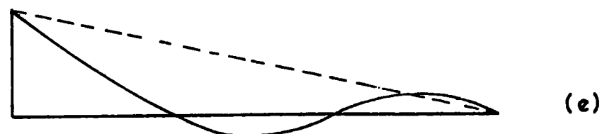
Figure 2.3 : Derivation of Shape Functions for corner nodes.
