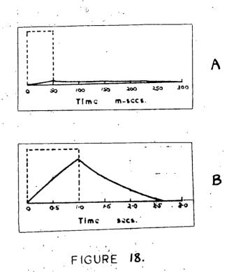
Thus with the introduction of  $R_i$  between  $C_i$  and  $C_2$ , impulses of short duration have little effect on the input circuit of the amplifier; consequently the effects of rapid field changes are suppressed. The effective time-constant of the amplifier is now 2/3 second. It is not expedient to increase  $R_i$  too much otherwise it will alter the potential of the collector considerably when large currents are received.
