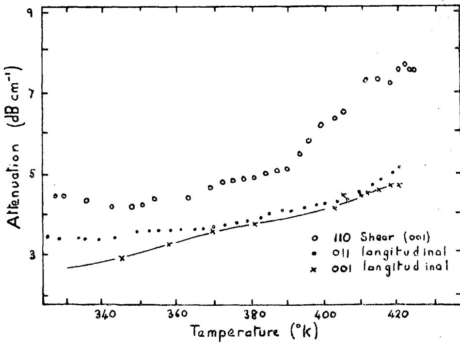
Figure 5.27(b) Ultrasonic attenuation at 14MHz in In-15 at.% Tl near to  $T_m$ .
