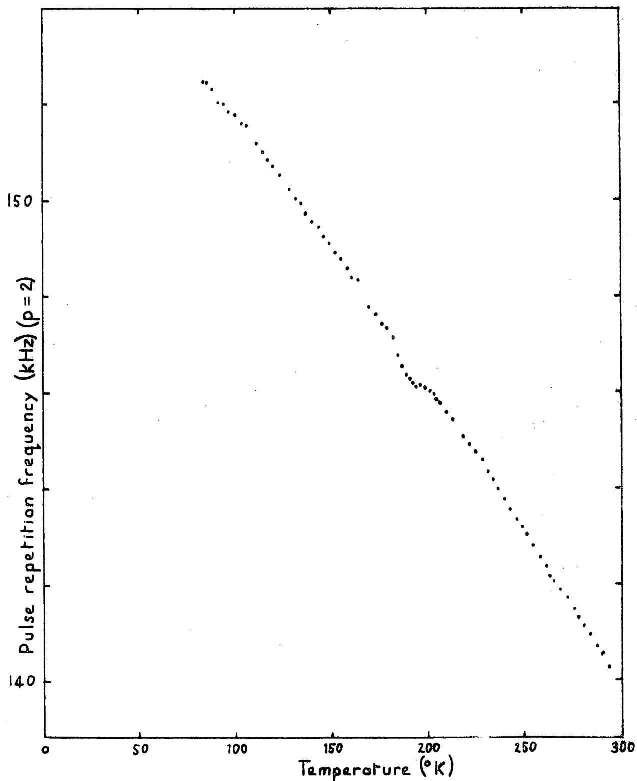
Figure 5.9 The measured PRF for wave propagation in the [110] direction of a shear wave polarised [001] at 15MHz in In-25 at.% Tl.
