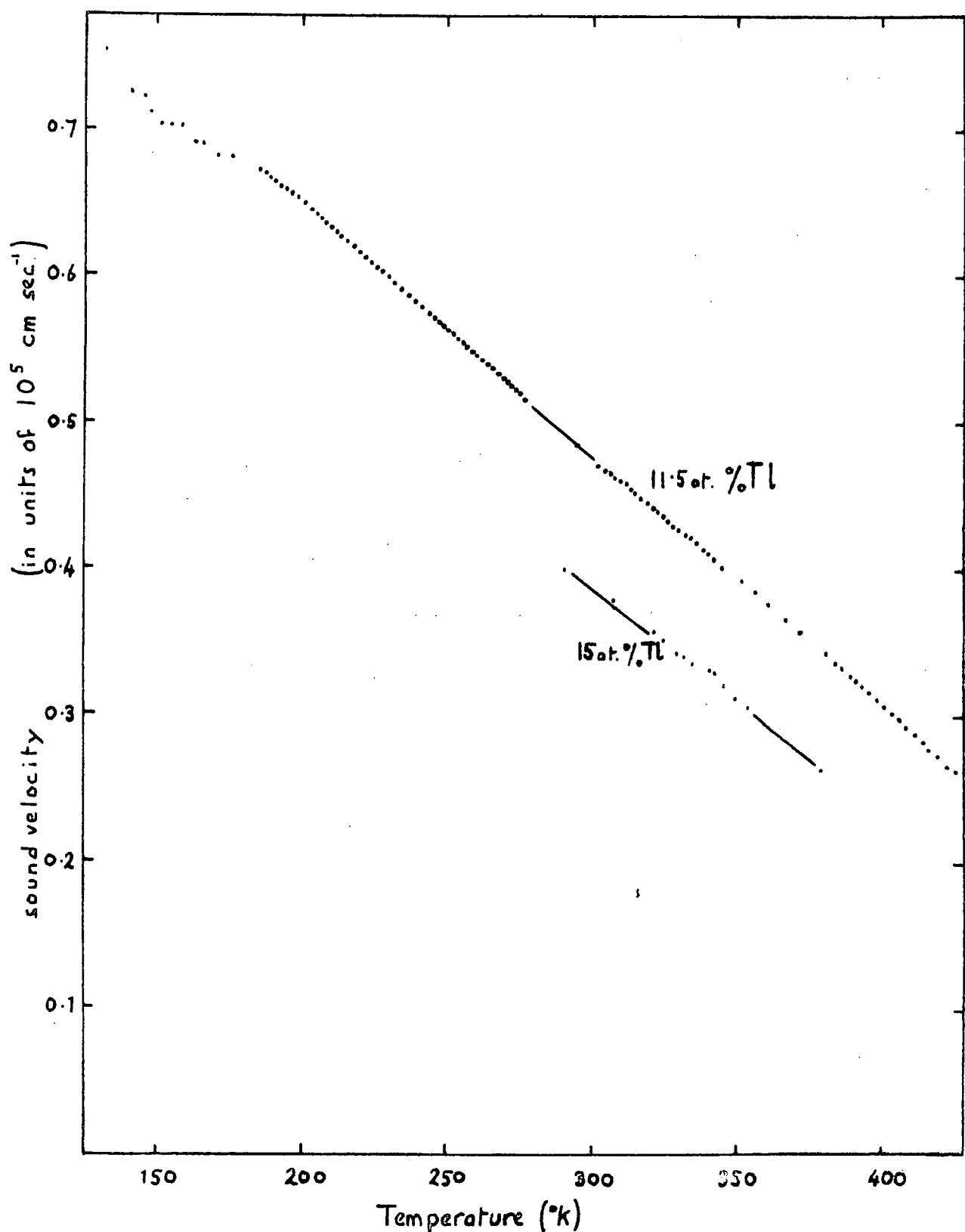
Figure 5.15 The temperature variation of the slow shear mode propagating in the [110] direction and polarised [110] for In-11.5 and 15 at.% Tl.
