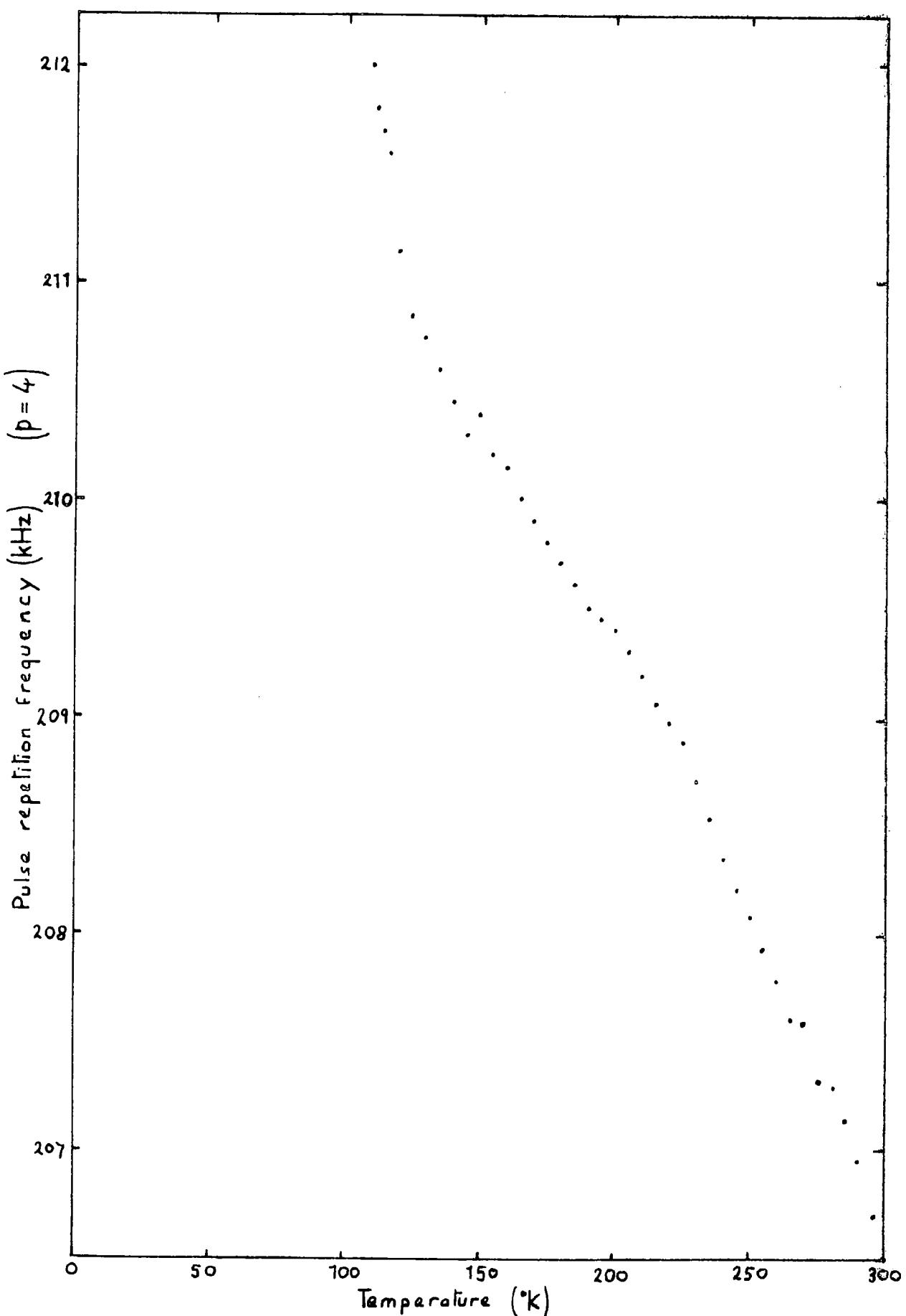
Figure 5.7 The measured PRF for propagation of longitudinal waves at 15MHz in the [100] direction in In-27at.% Ti.
