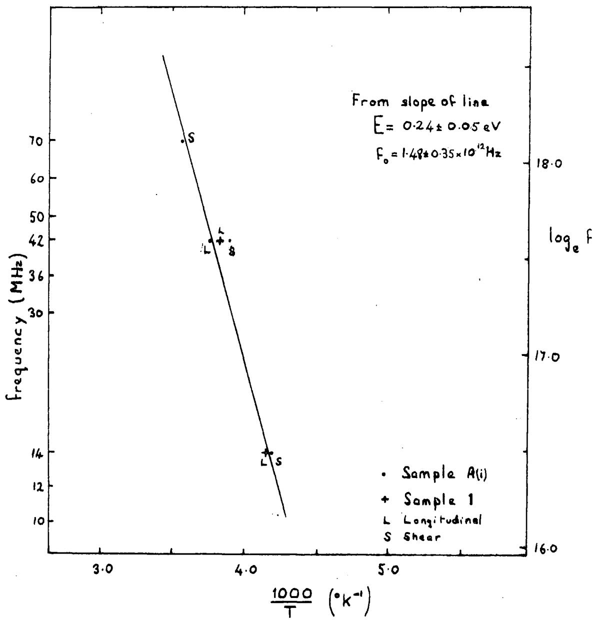
Figure 5.21 Arrhenius plot to determine activation energy and attempt frequency of Bordoni peak.
