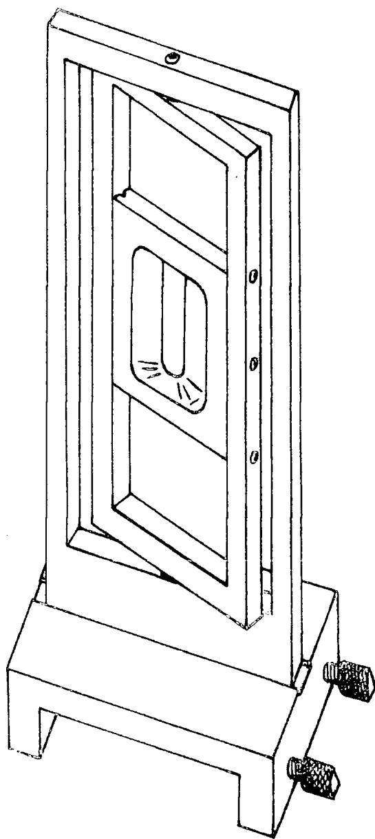
Figure 4.13 An apparatus for checking the orientation of planed faces of ultrasonic samples.
