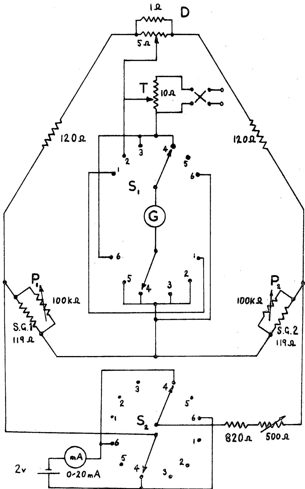
Figure 4.22 Strain gauge bridge used in measurement of thermal expansion.
