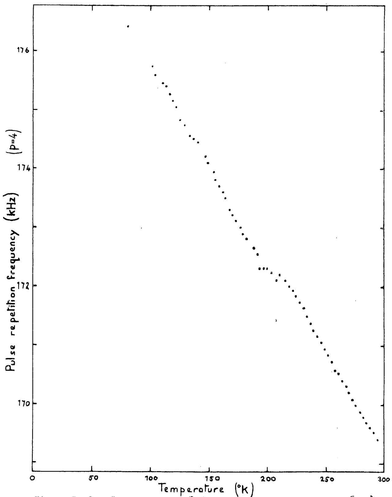
Figure 5.10 The measured PRF for wave propagation in the [110] direction of a longitudinal wave at 13.5 Ma in In-29 at.% Ti.
