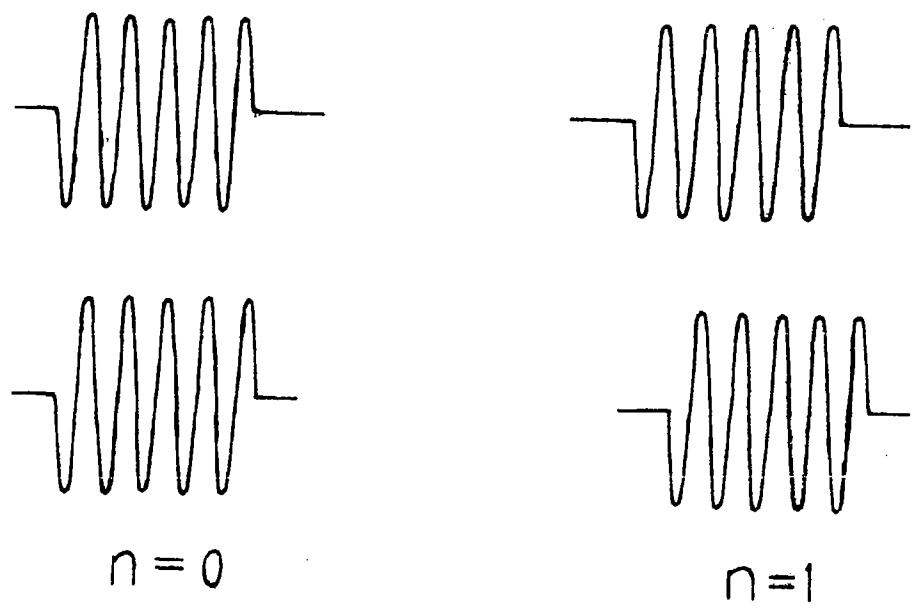
Figure 4.16 Superposition of r.f. pulses.
