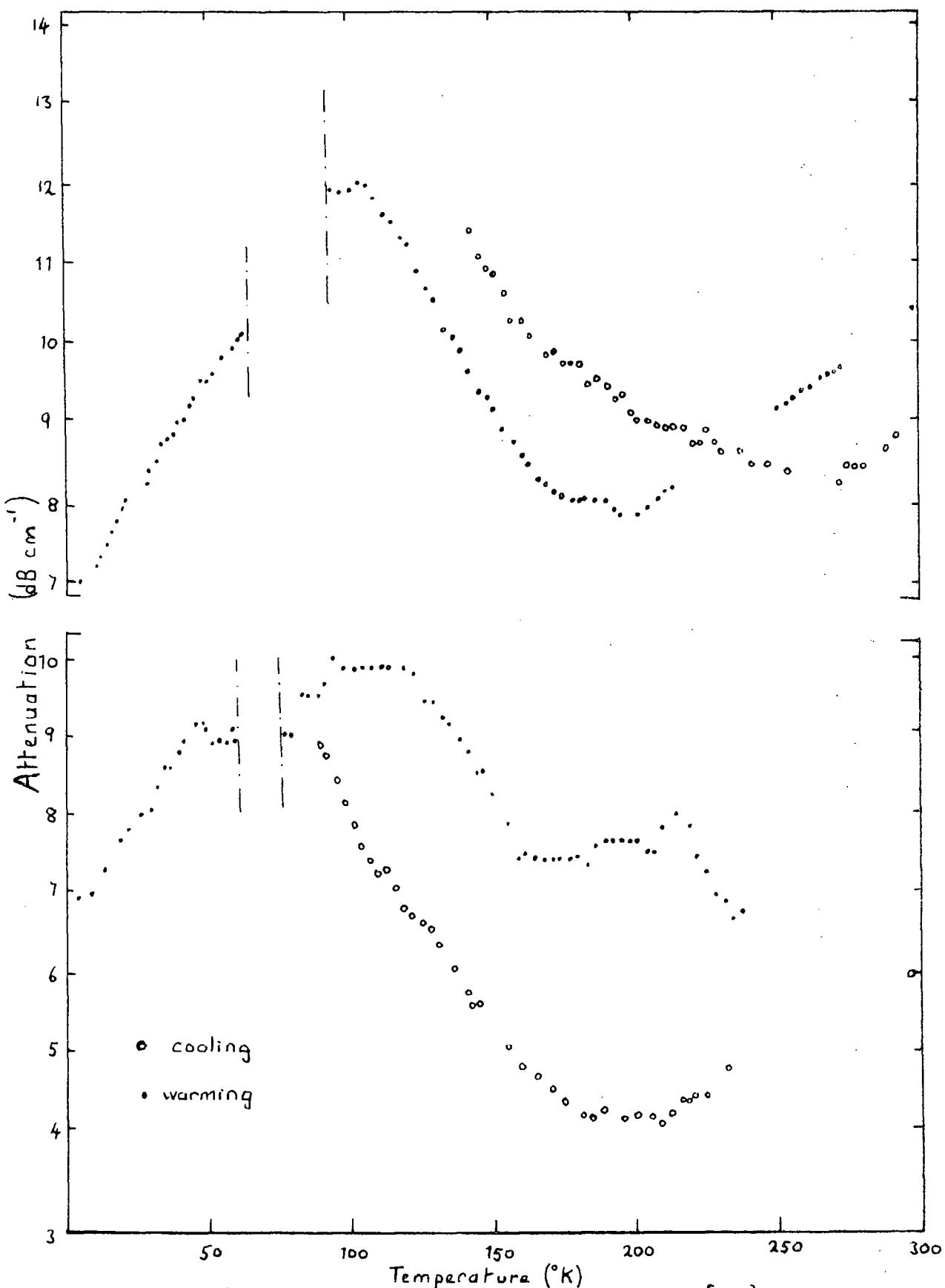
Figure 5.26 Ultrasonic attenuation at 14MHz in [110] in indium.
