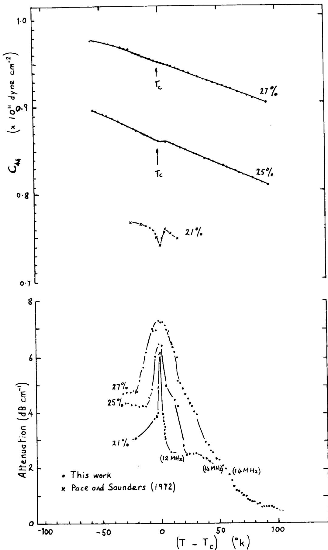
Figure 8.3 Velocity and attenuation in the vicinity of the martensitic transition in three In-Tl alloys.
