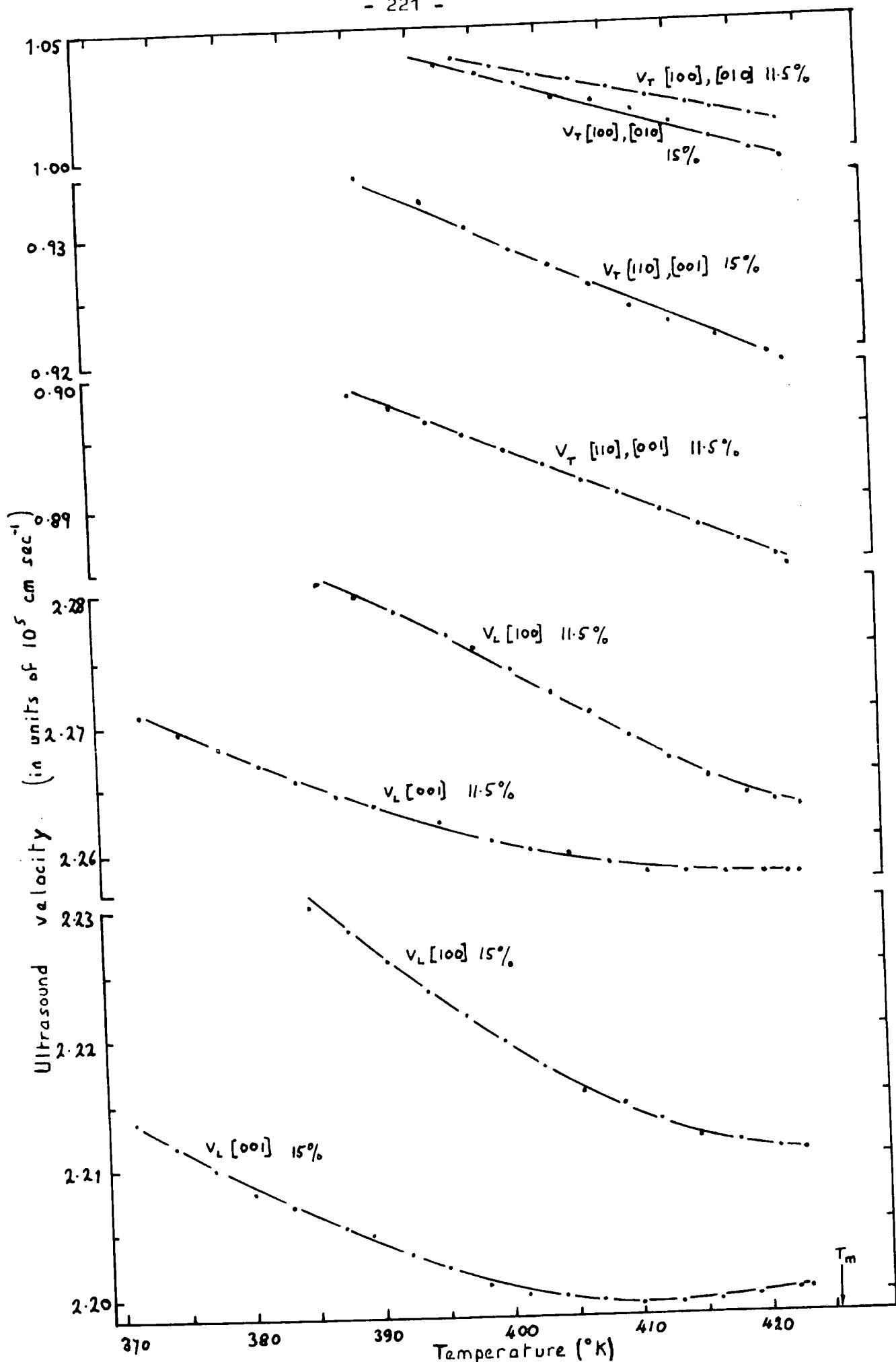
Figure 8.2 Ultrasound velocity near the melting point in In-11.5 and 15 at.% Tl.
