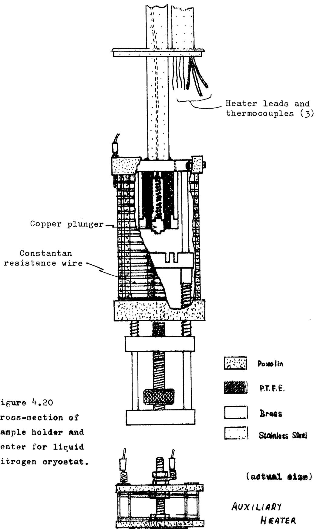
The heater was wound non-inductively on a paxolin former, and three nylon grub screws held it in position so that the sample was at its centre. Constantan wire of such a length as to give a resistance of  $300\Omega$  was used, and electrical connections were made using two small plugs. An auxiliary heater, powered by a variable a.c. supply (maximum 15 volt) was available when necessary to increase the rate of evaporation of the liquid nitrogen from beneath the sample.
