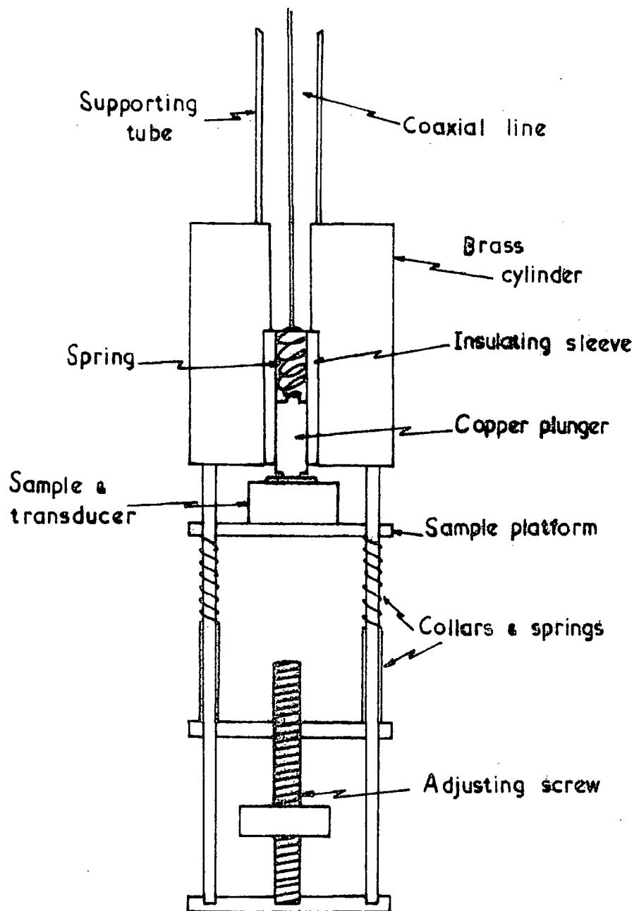
Figure 4.19 Schematic diagram of a sample holder for ultrasonic studies.
