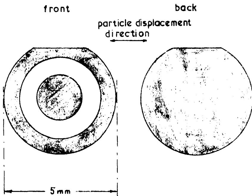
Figure 4.14(b) The dimensions and electrode configuration of the transducers used in this work. A shear transducer is shown; a longitudinal one needs no flat to indicate particle displacement direction, and is circular. The shading represents gold plating.
