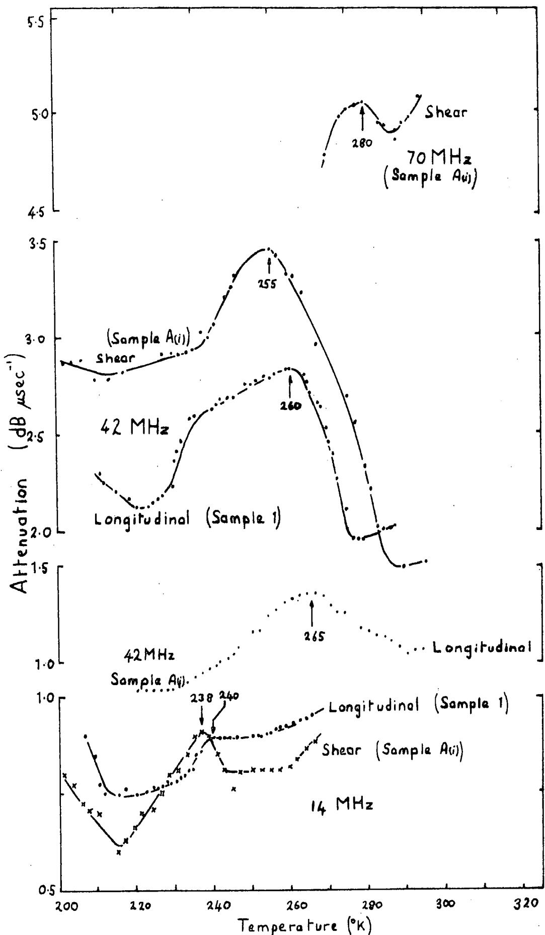
Figure 5.20 Collected data (for various samples and polarisations) of the Bordoni peak found for wave propagation in [110] in In-27 at.% Tl.
