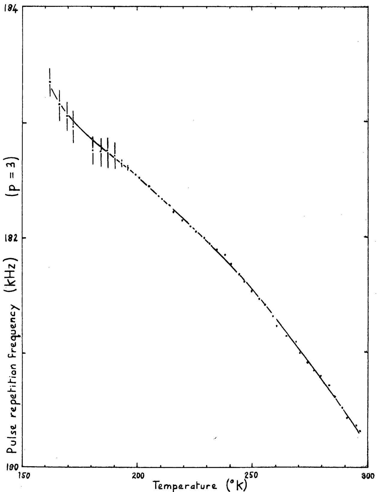
Figure 5.11 The measured PRF for wave propagation in the [100] direction of a longitudinal wave at 14MHz in In-25 at.% Tl.
