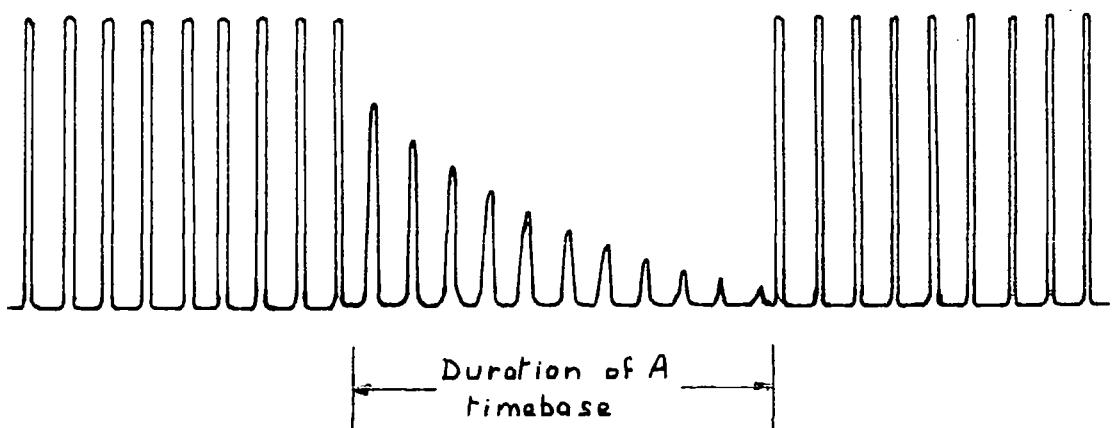
Figure 4.18 The appearance of the oscilloscope trace at or near superposition of echoes.
