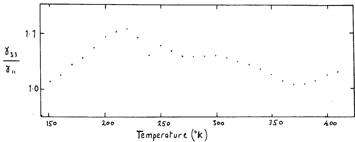
Figure 3.1 The temperature variation of  $\frac{\gamma_{11}}{\gamma_{33}}$  for an In-11.5 at.% Tl alloy.
