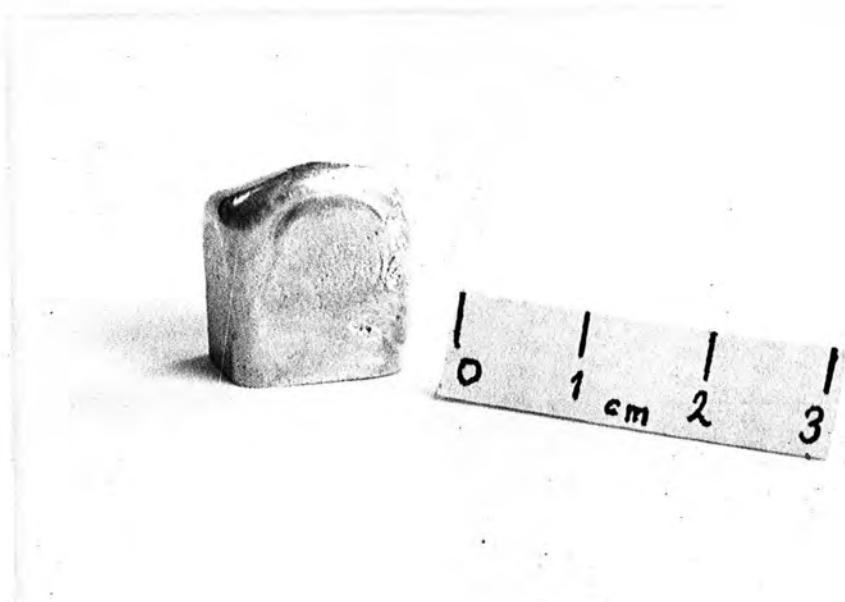
Figure 4.5 As-grown boule of an indium-thallium alloy. (Part of the boule (approx.  $\frac{1}{3}$ ) has been cut away.)
