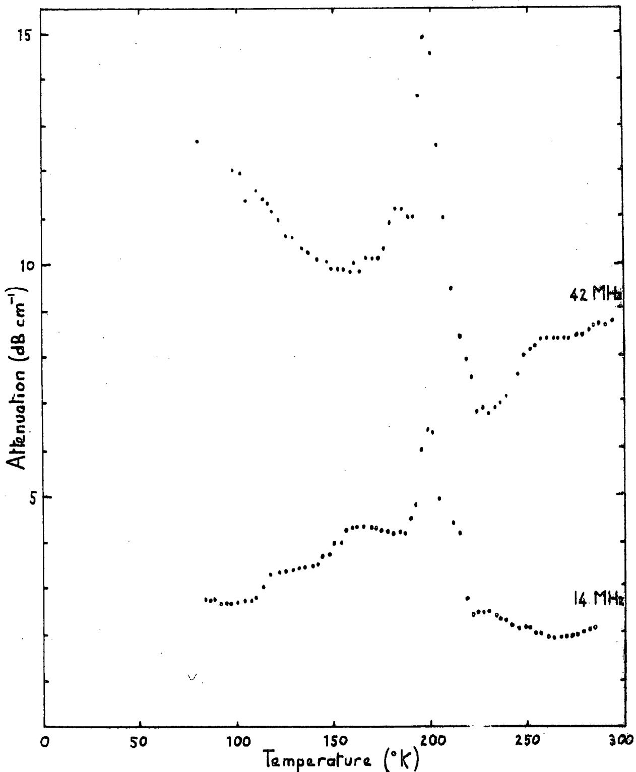
Figure 5.18 Attenuation of ultrasound in In-25 at.% Tl as a function of temperature. The measurements are for a longitudinal wave propagating [110], and were obtained on cooling.
