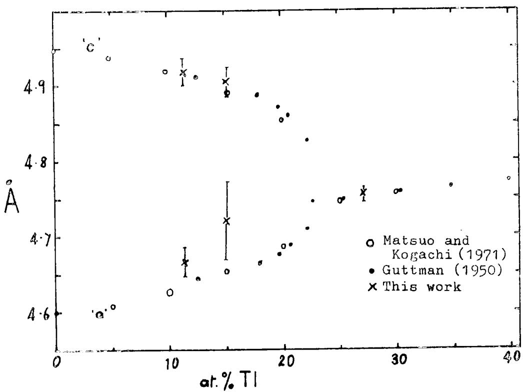
Figure 4.11 Lattice parameters of indium-thallium alloys.
