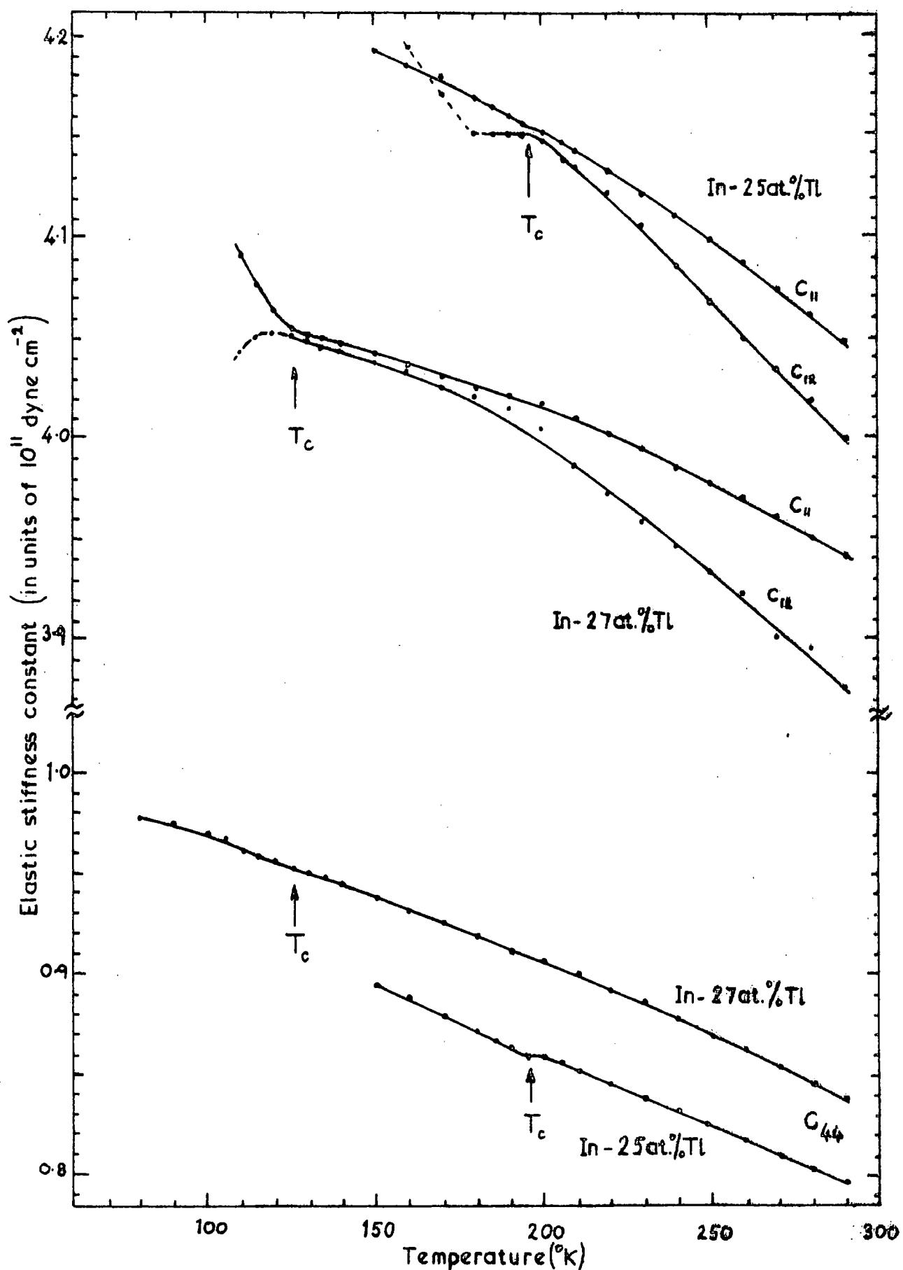
Figure 5.8 The elastic constants  $C_{11}$ ,  $C_{12}$  and  $C_{44}$  for the cubic alloys In-25 and 27 at.% Tl over a temperature range which includes their transition temperatures.
