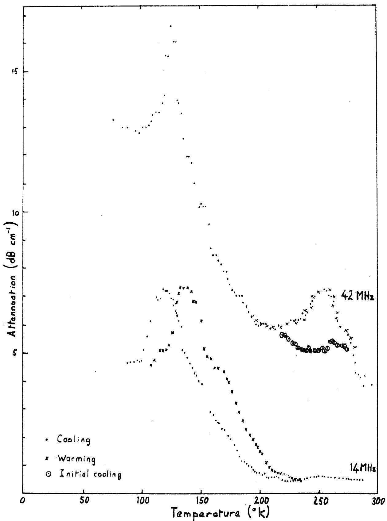
Figure 5.19 Attenuation of ultrasound in In-27 at.% Tl as a function of temperature. The 14MHz curve was for longitudinal waves, and the 42MHz one for shear waves polarised [001], both propagating in [110].
