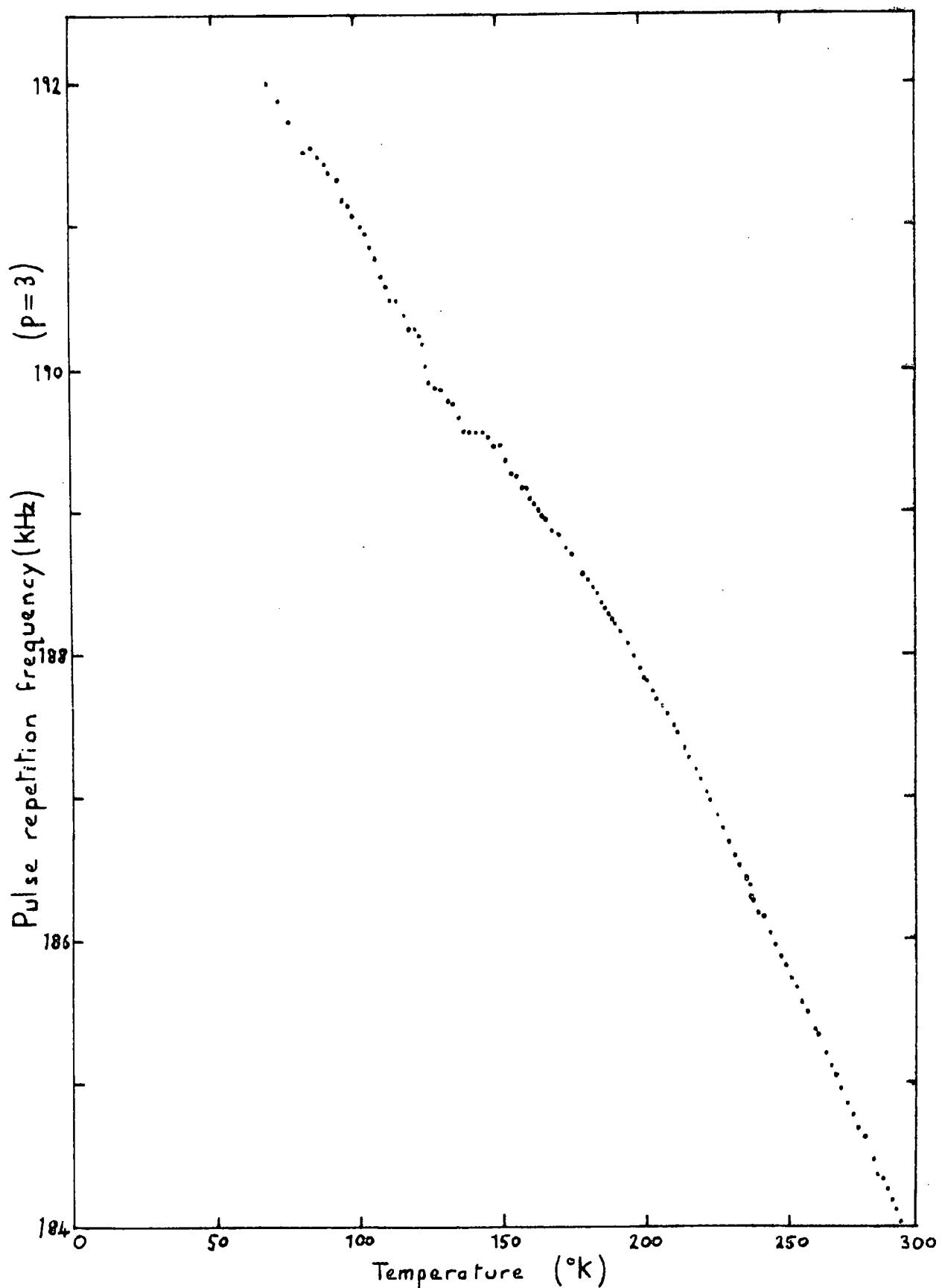
Figure 5.6 The measured PRF for propagation of longitudinal waves at 15MHz in the [110] direction in In-27at.% Ti
