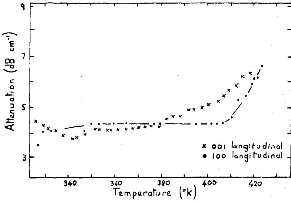
Figure 5.27(a) Ultrasonic attenuation at 14MHz in In-11.5 at.% Tl near to  $T_m$ .
