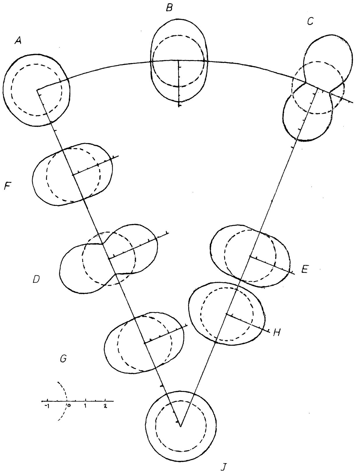
Figure 6.5 Poisson's ratio variation in In-15 at.% Tl.
