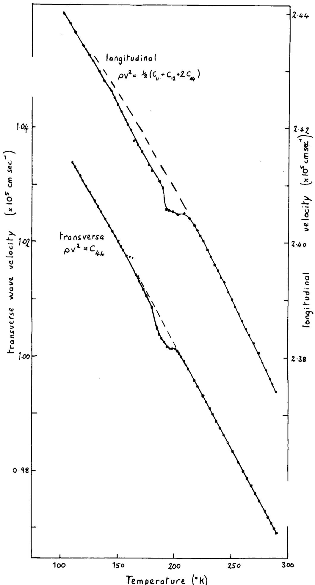
Figure 8.9 Velocities of wave propagation along [110] for In-25 at.% Tl, after a thermal expansion correction has been made.
