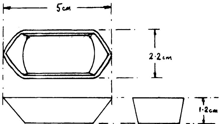
Figure 4.1 The pyrex glass boat in which crystals
