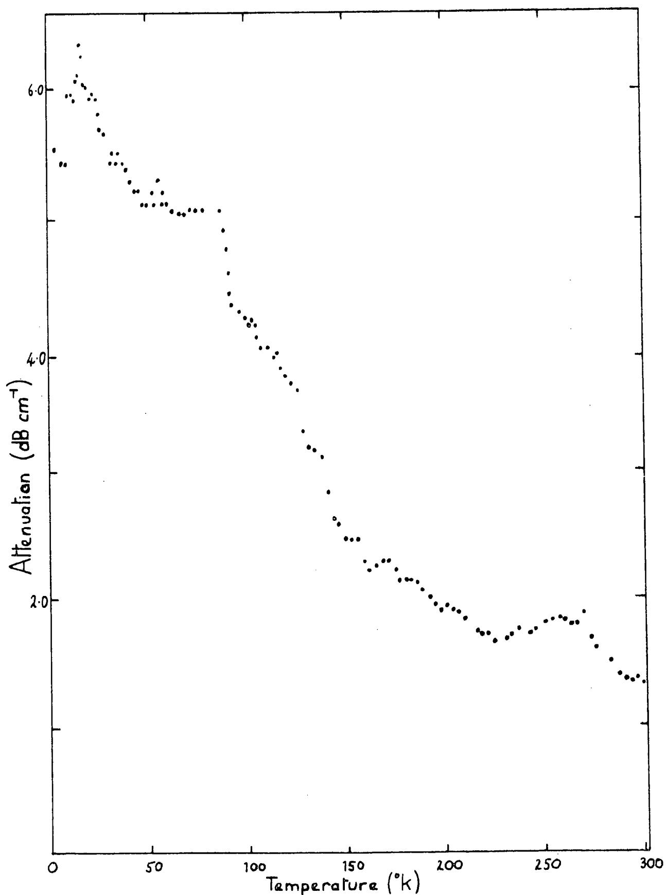
Figure 5.22 Ultrasonic attenuation at 15MHz in [110] in In-10 at.% Tl alloy (longitudinal waves).
