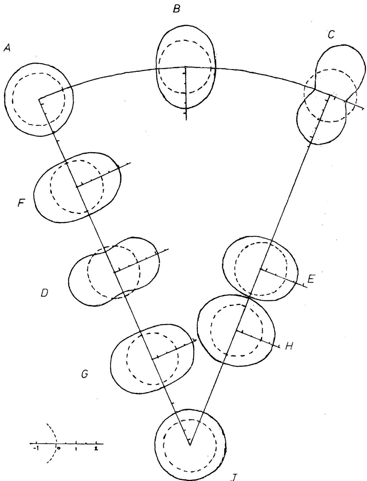
Figure 6.4 Poisson's ratio variation in In-11.5 at.% Tl.
