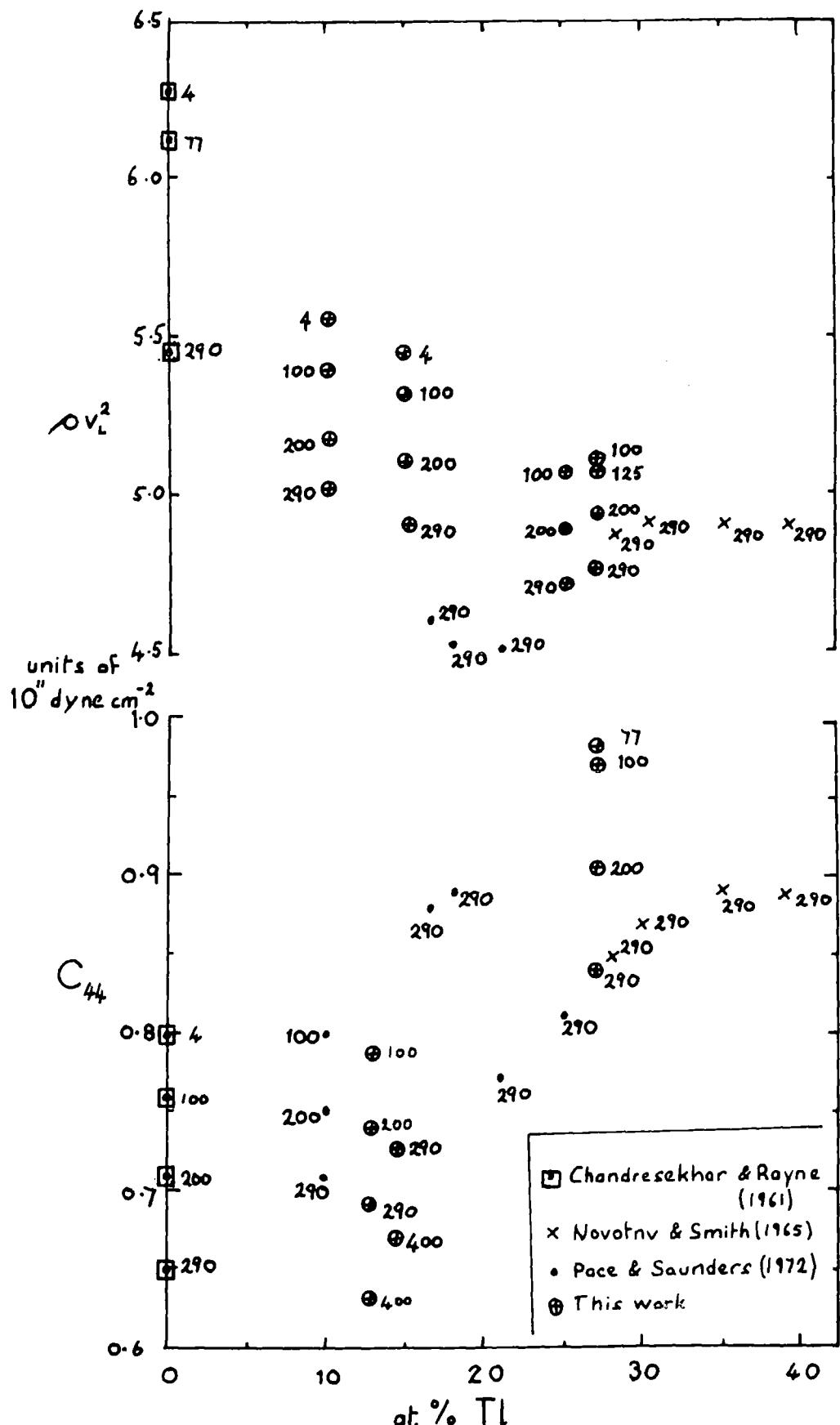
Figure 8.4 The longitudinal and one of the shear moduli for propagation in the [110] direction. The temperature corresponding to each point is shown adjacent to the point (the units are degrees Kelvin).
