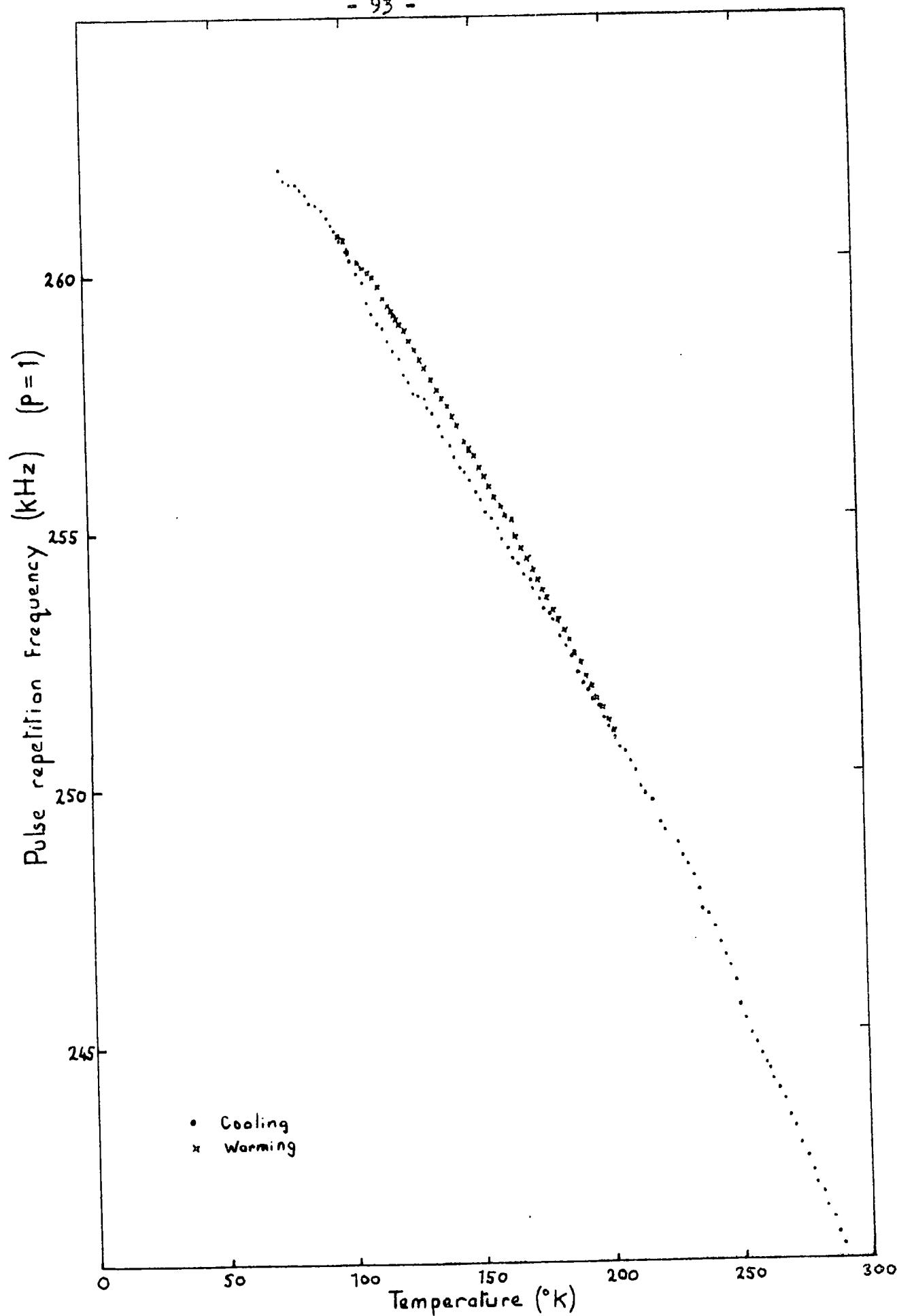
Figure 5.5 The measured PRF for propagation of [001] polarised shear waves in the [110] direction in In-27at.% Tl.
