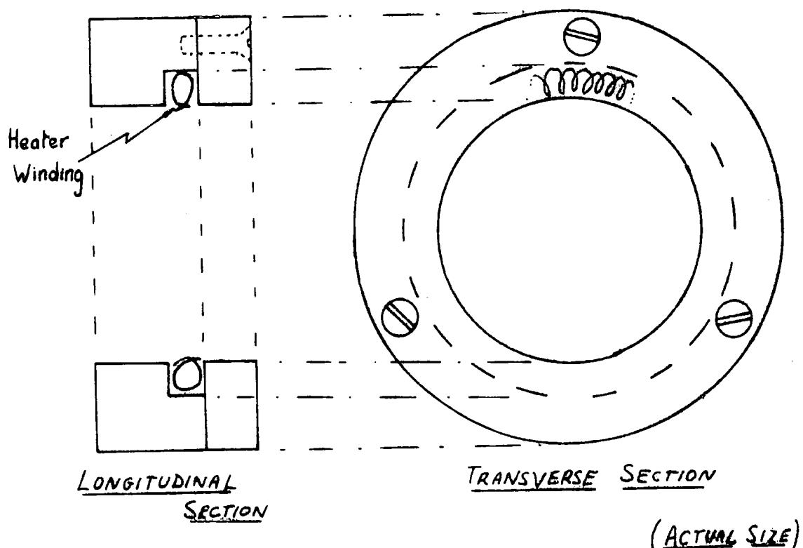
Figure 4.3 Details of the heater assembly.
