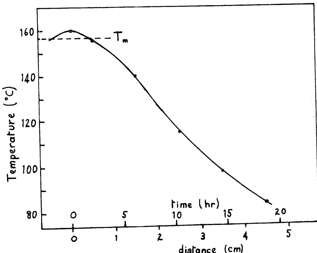
Figure 4.4 Temperature profile of the growth furnace (measured along the axis of the furnace before introduction of the boat and alloy).
