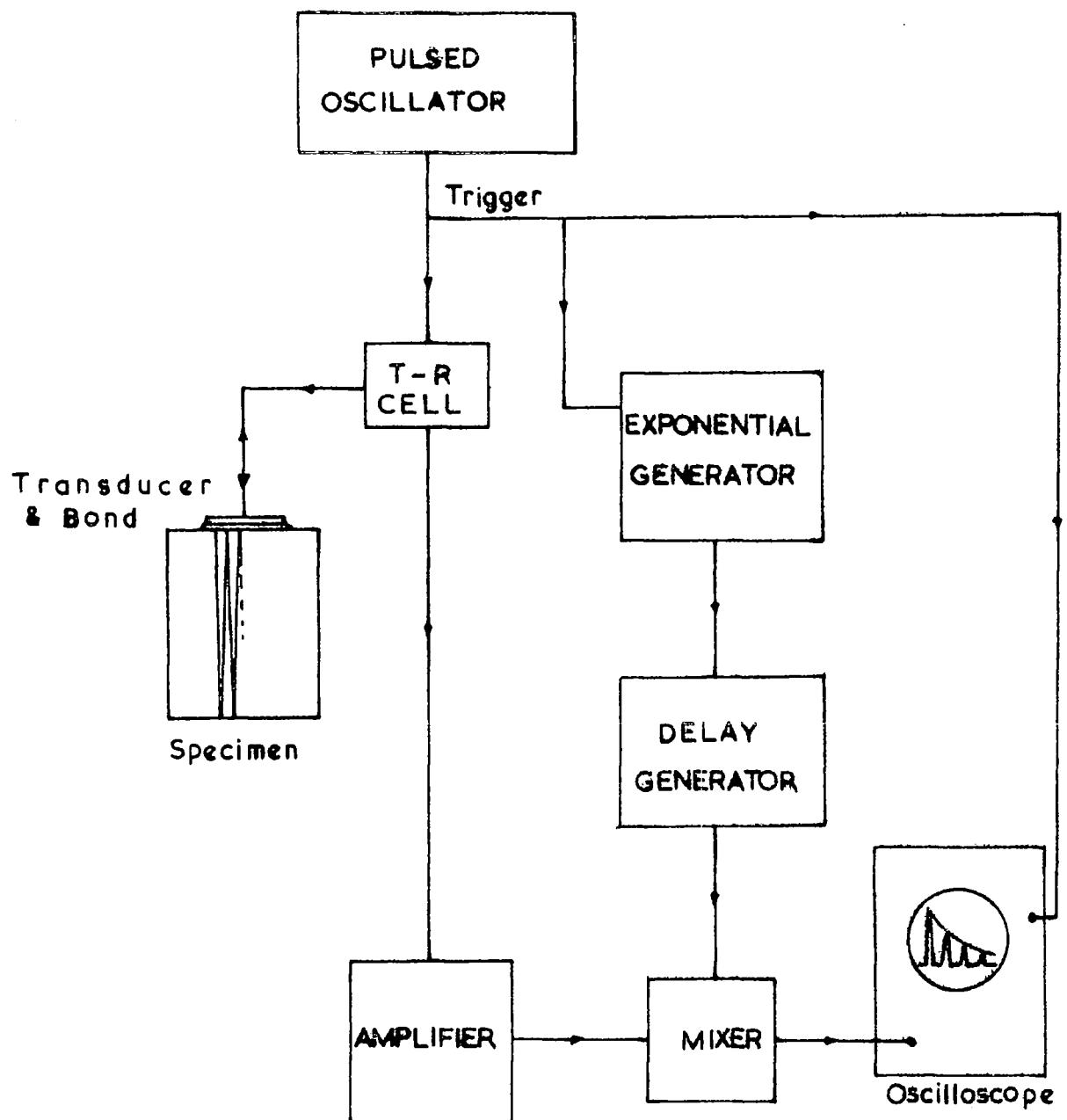
Figure 4.15 Block diagram of the instrumentation for the ultrasonic pulse-echo system.
