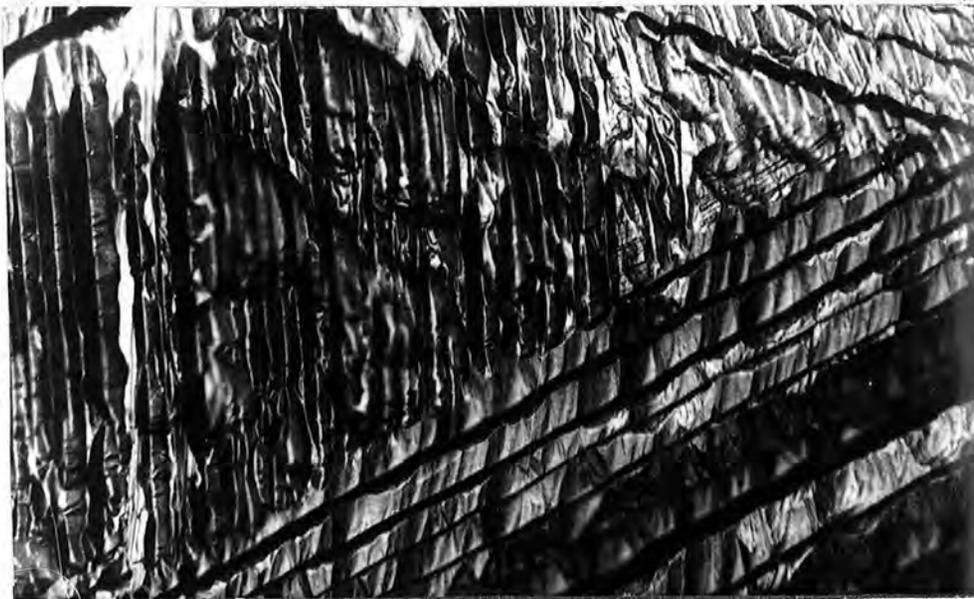
Figure 2.2(b) A region of an In-21 at.% Tl alloy in which main bands on three different  $\{110\}$  planes can be seen. Slight interpenetration of bands is occurring.
