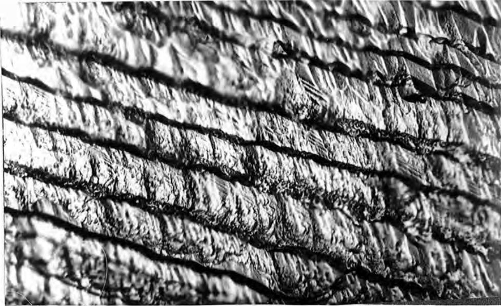
Figure 2.2(a) Transformation twins in an In-21 at.% Tl alloy. The main bands can be seen separated by the dark lines. Sub-bands are visible within them.
