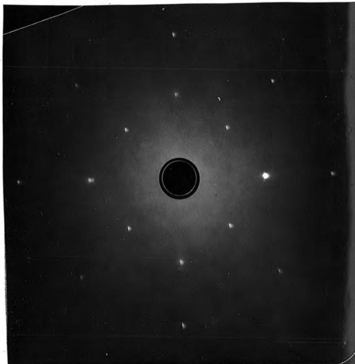
Figure 4.6 Laue back-reflection photograph of In-15 at.% Tl alloy. X-ray beam is directed along 4-fold axis.
