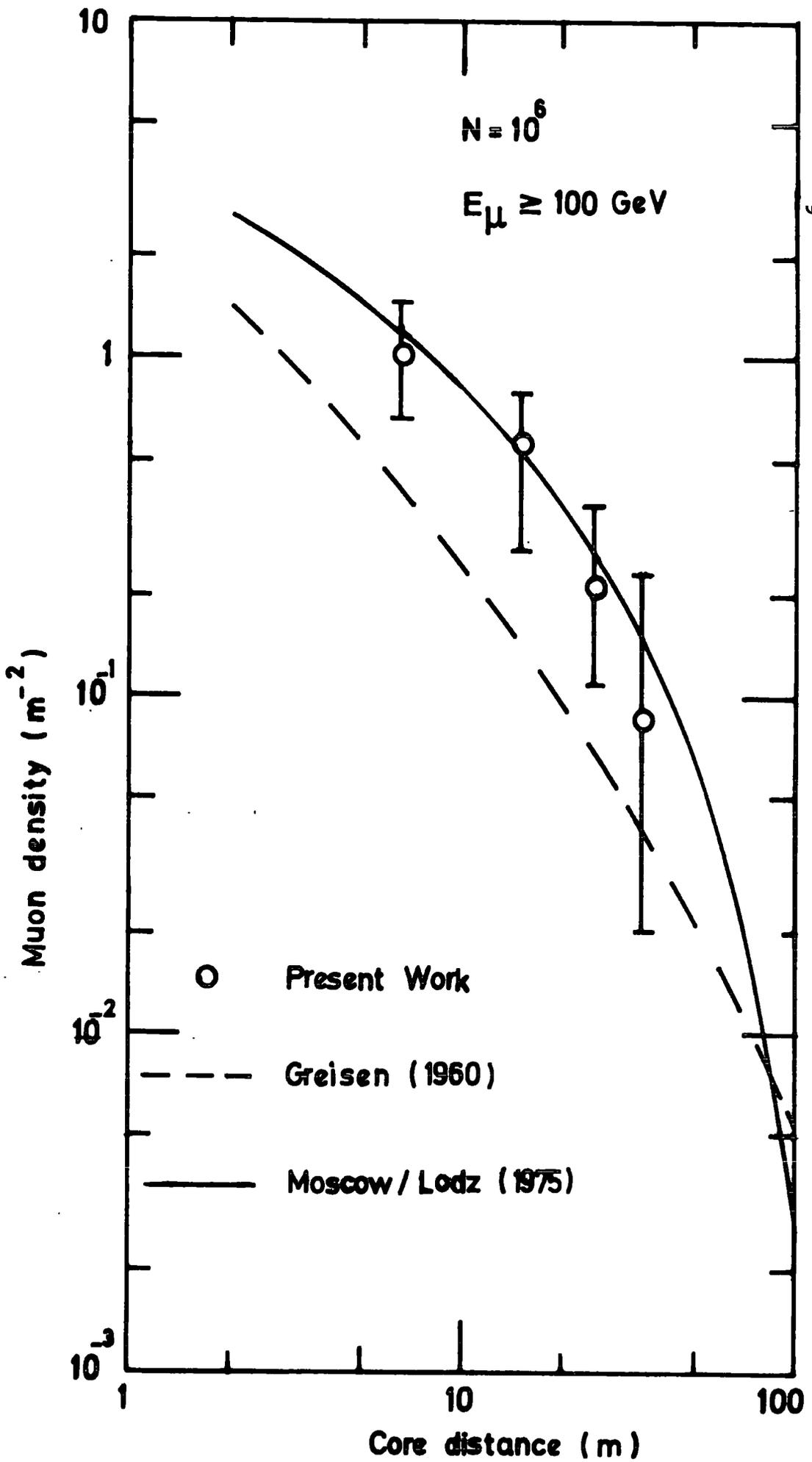
FIGURE 7.13 Comparison of the lateral distribution of muons ( $E_{\mu} \geq 100 \text{ GeV}$ ) in showers of size  $10^6$  particles with the extrapolations of the structure functions of Greisen (1960) and Moscow/Lodz collaboration, (Hawkes, 1977).
