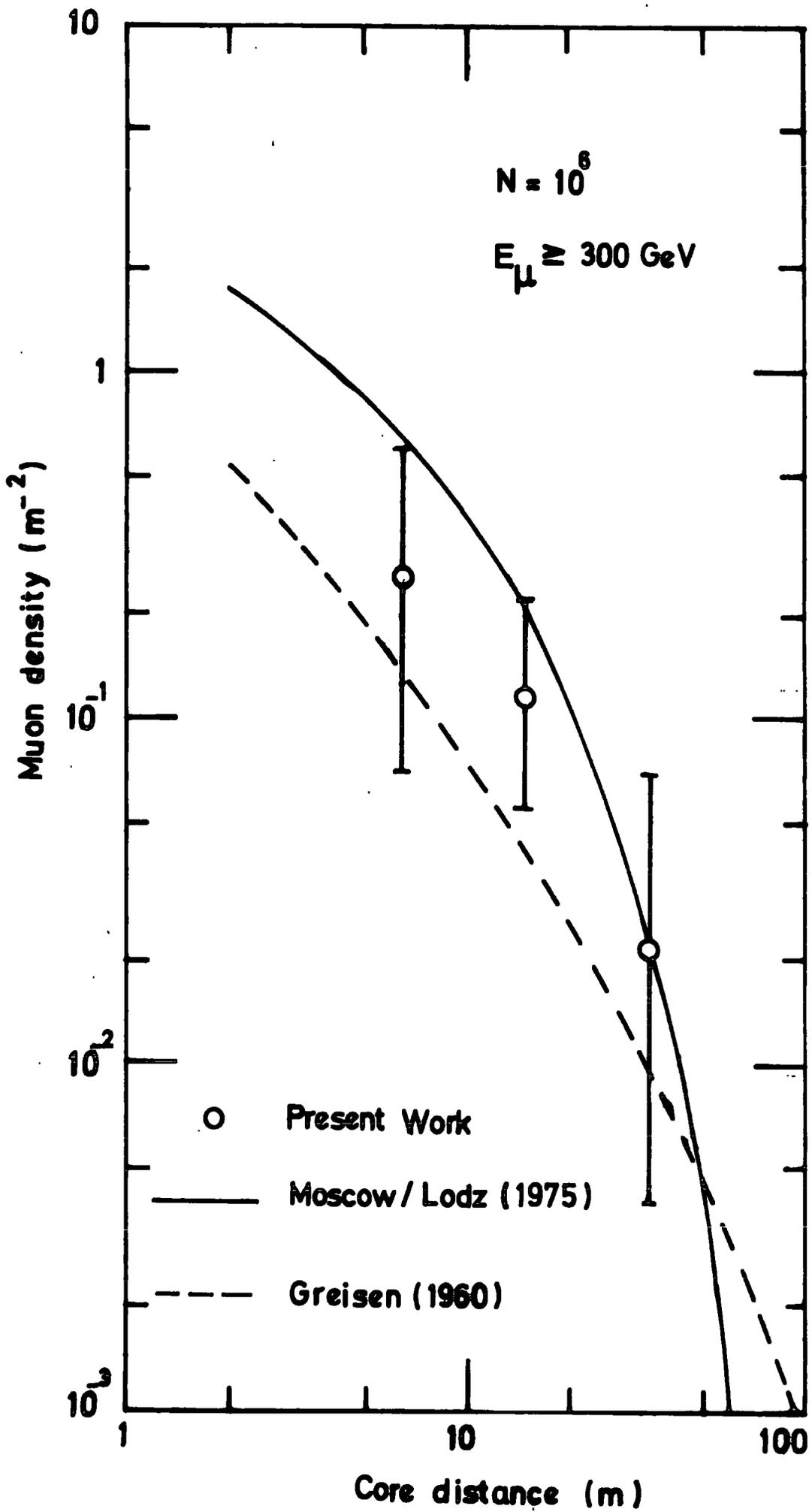
FIGURE 7.15 A comparison of the lateral distribution of muons having energies  $\geq 300$  GeV in showers of size  $10^6$  particles with the predictions of the muon structure function of Greisen (1960) and the Moscow/Lodz collaboration (Hawkes, 1977), both structure functions are extrapolated to  $E_{\mu} \geq 300$  GeV.
