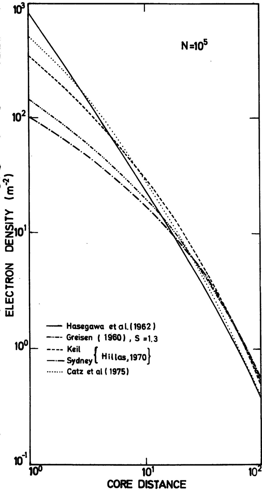
FIGURE 2.3 Measurements of the electrons lateral distribution obtained by different authors at sea level and normalised to a common shower size of  $10^5$  particles.
