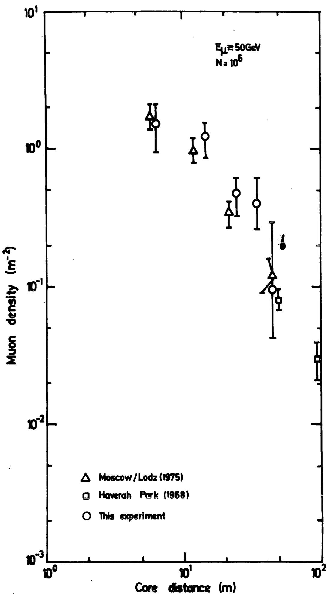
FIGURE 7.11 Comparison of the lateral distribution of muons ( $E \geq 50 \text{ GeV}$ ) with the measured distribution of the Moscow/Lodz  $\nu$  collaboration (Rozhdestvensky et al, 1975) and the Haverah Park measurement (Orford, 1968). The present data and Haverah Park data are normalised to a shower size of  $10^6$  particles.
