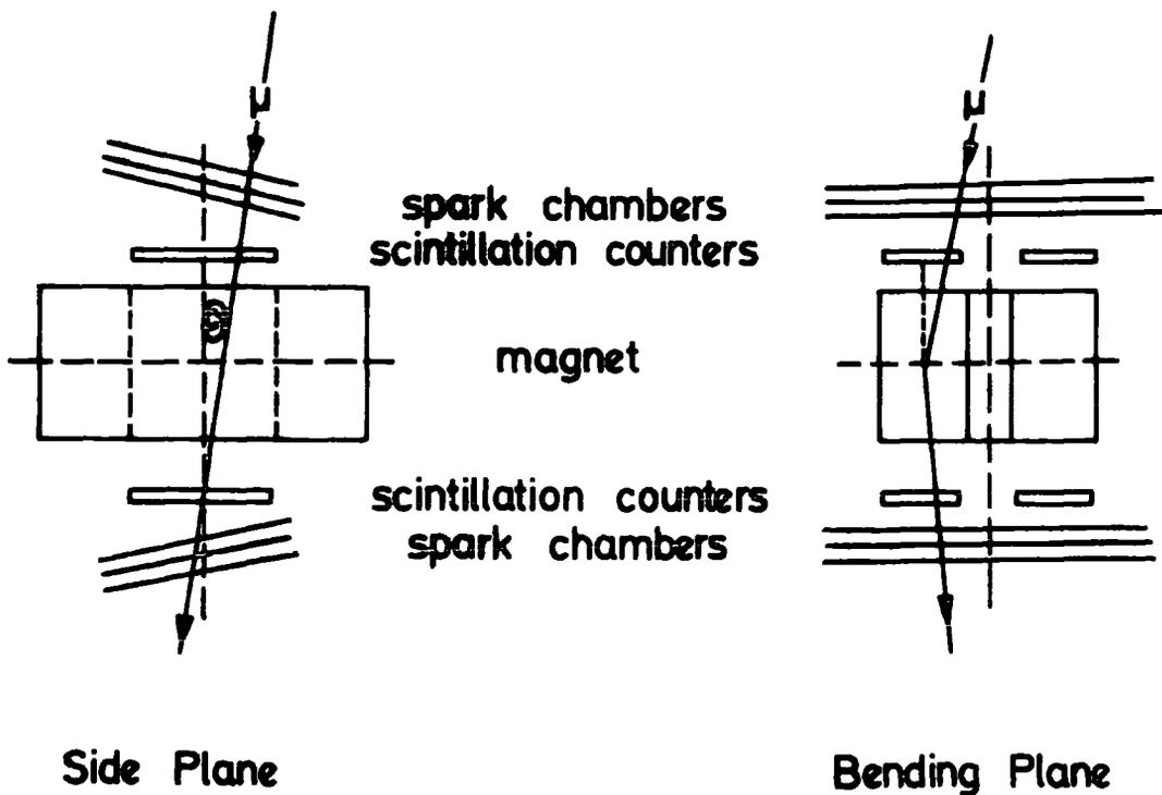
FIGURE 2.23b The magnetic spectrograph of the M.S.U. air shower array (After Abrozimov, et al, 1974).
