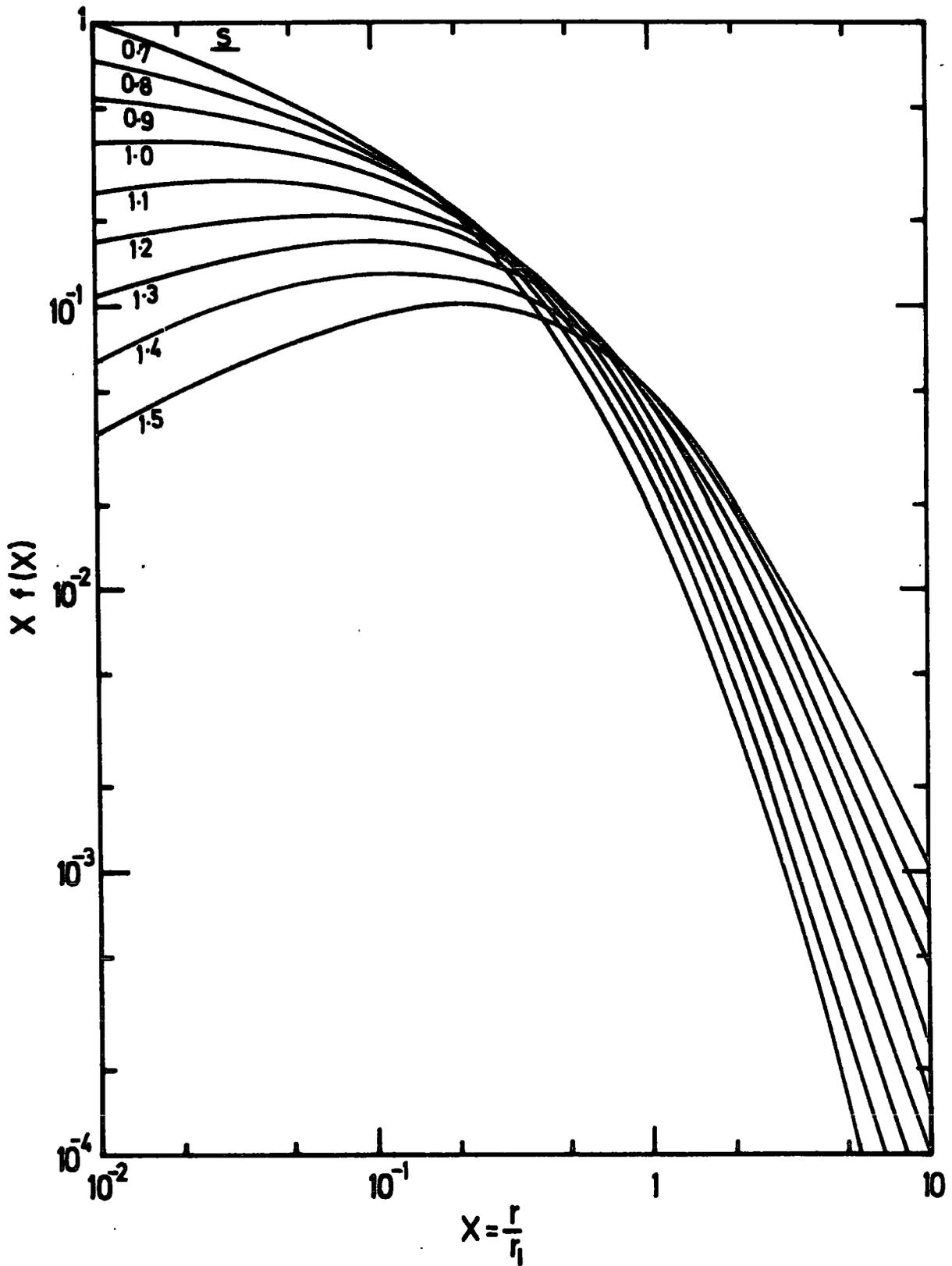
FIGURE 2.4 The dependence of the electron structure function on the age parameter for a fixed shower size, the curves are obtained by using the N.K.G. structure function.
