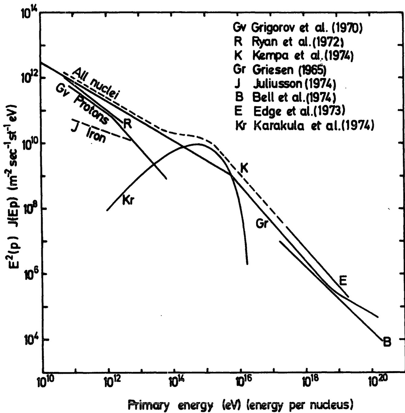
FIGURE 1.5 The differential energy spectrum of primary cosmic rays obtained from the results of various workers.
