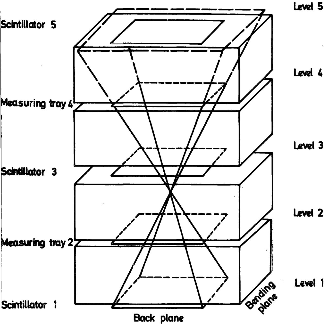
FIGURE 3.17a Illustration of the 1-4 tray category acceptance of the blue-side of M.A.R.S.
