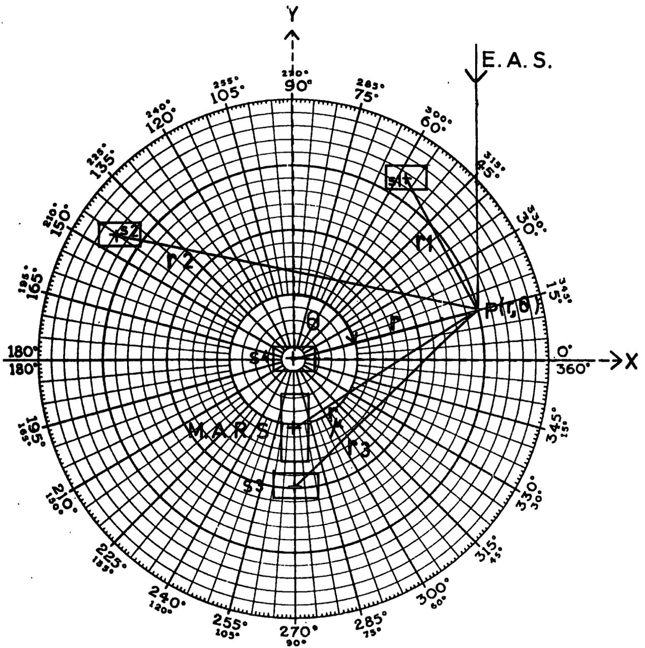
FIGURE 4.2 Determination of the core distances for various counters and the spectrograph in the plane polar co-ordinate system of the array.
