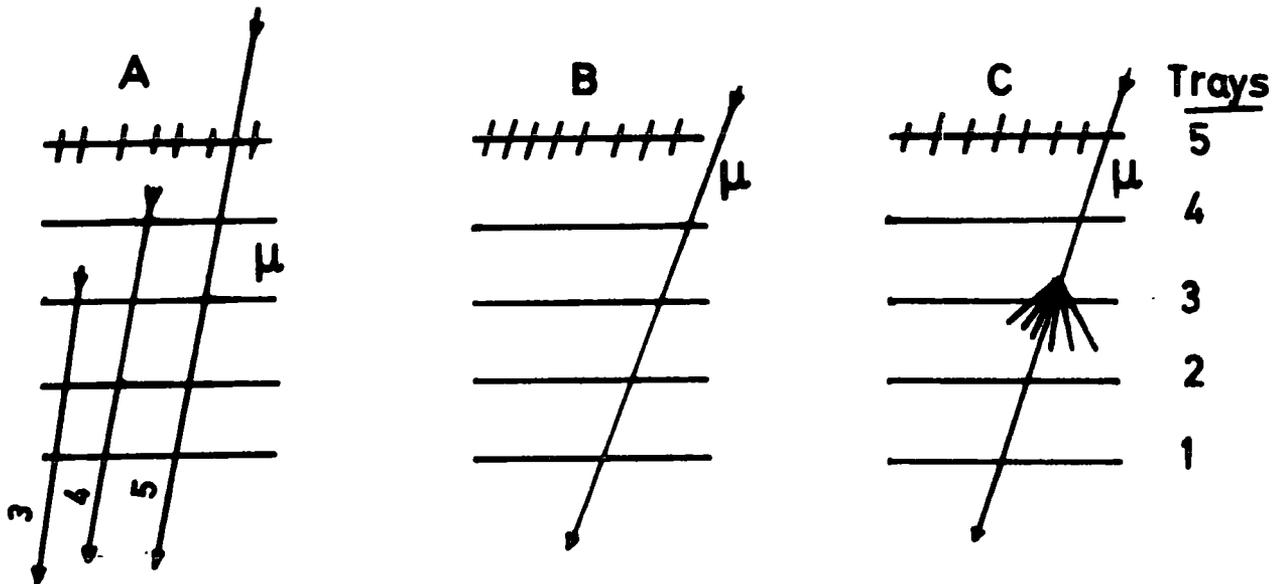
**A** - Muon trajectories are within 3 and 4 tray acceptance
