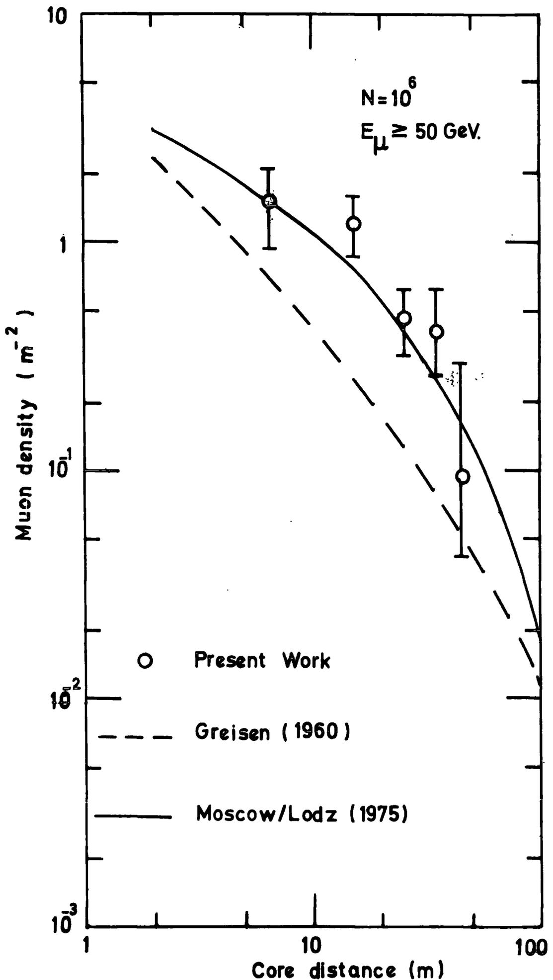
FIGURE 7.12 Comparison of lateral distribution of muons ( $E_{\mu} \geq 50 \text{ GeV}$ ) in showers of size  $10^6$  particles with the predictions of the Greisen's structure function extrapolated to  $E_{\mu} \geq 50 \text{ GeV}$ , and the muon structure function fitted to the Moscow/Lodz data.
