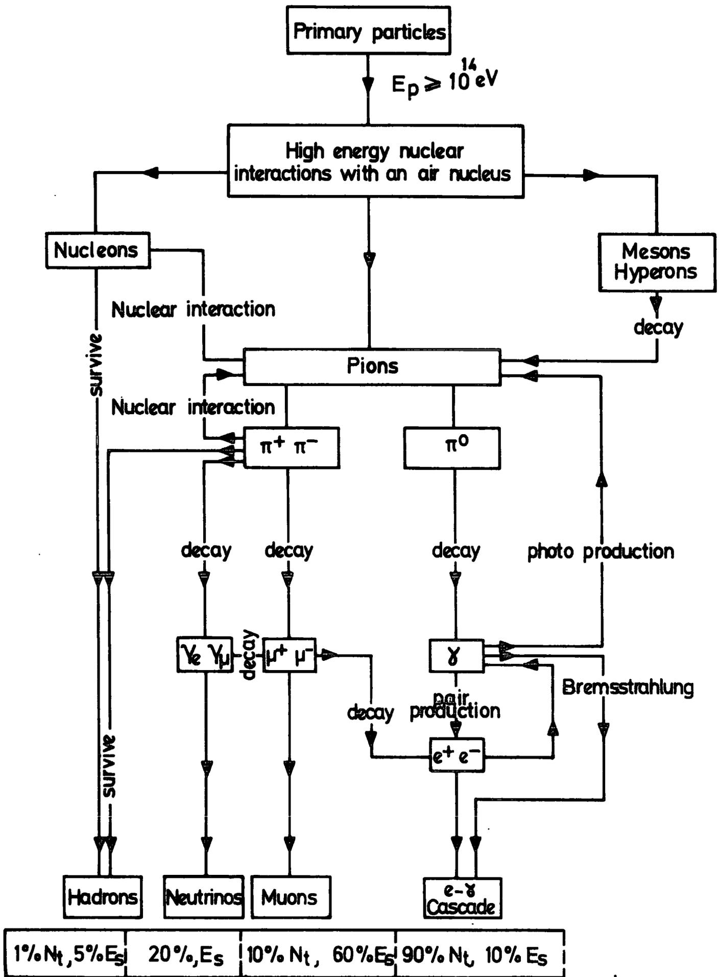
FIGURE 2.1 The development of an E.A.S. arriving at sea level,  $N_t$  is the number of particles in the shower at sea level and  $E_s$  is the total energy of the shower at the same level.
