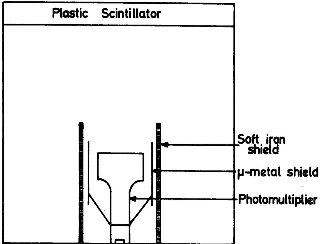
Figure 3.4 : Shielding system of a photomultiplier tube.
