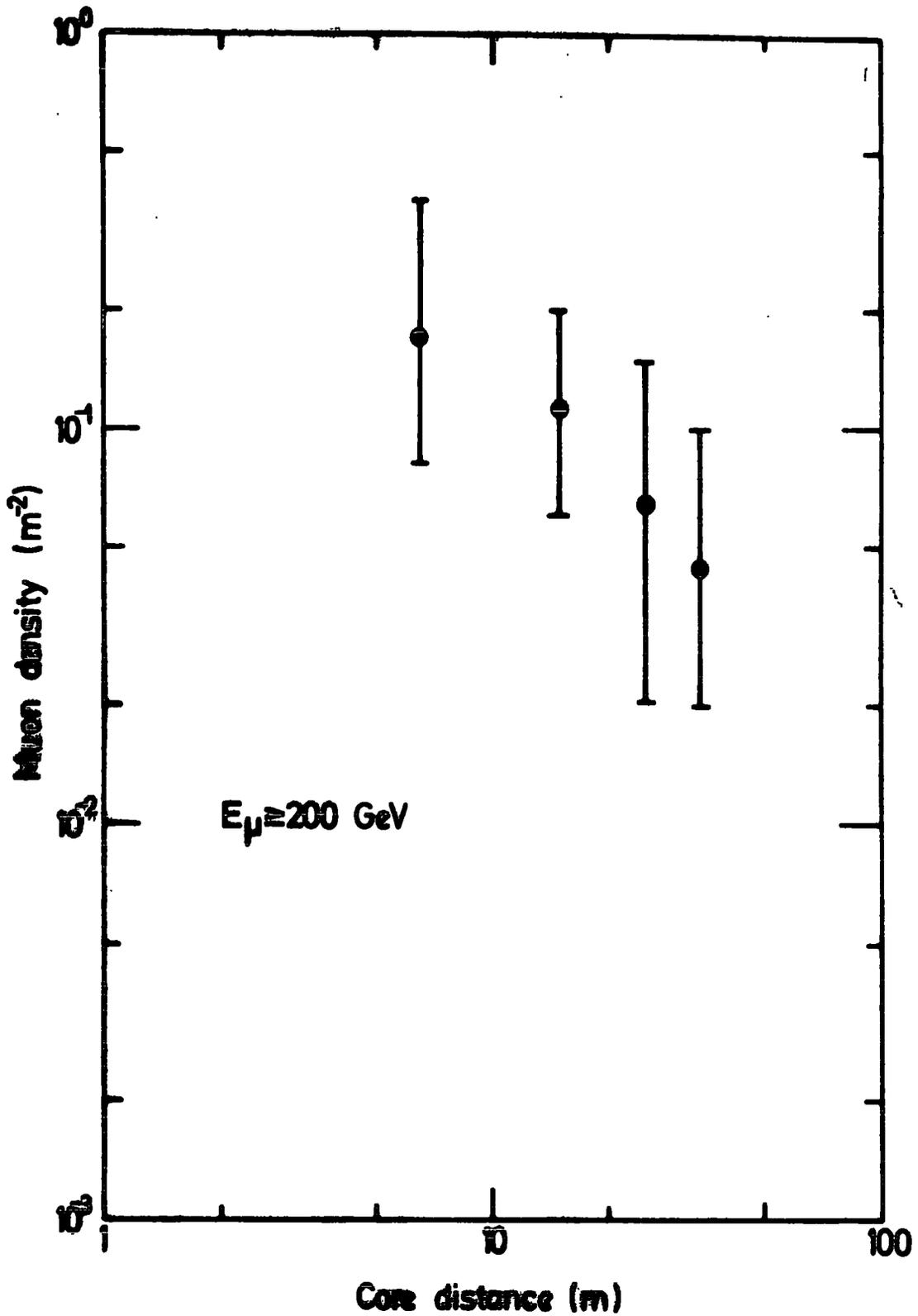
FIGURE 7.9 The measured lateral distribution of muons with energies  $> 200 \text{ GeV}$  in showers of various sizes as indicated in figure 7.2.
