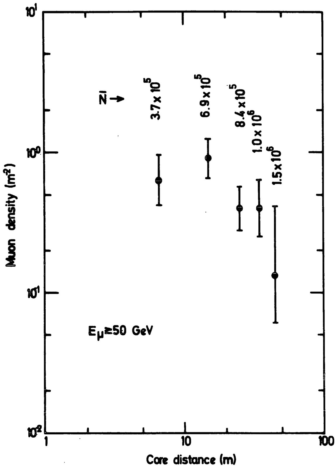
FIGURE 7.7 The measured lateral density distribution of muons having energies  $\geq 50 \text{ GeV}$  in selected showers (see text).
