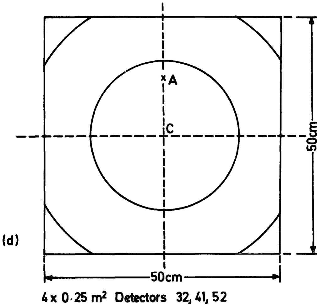
FIGURE 5.3d Pulse height contour map of one quarter of the 1m<sup>2</sup> density measuring detector. C represents the calibration point.
