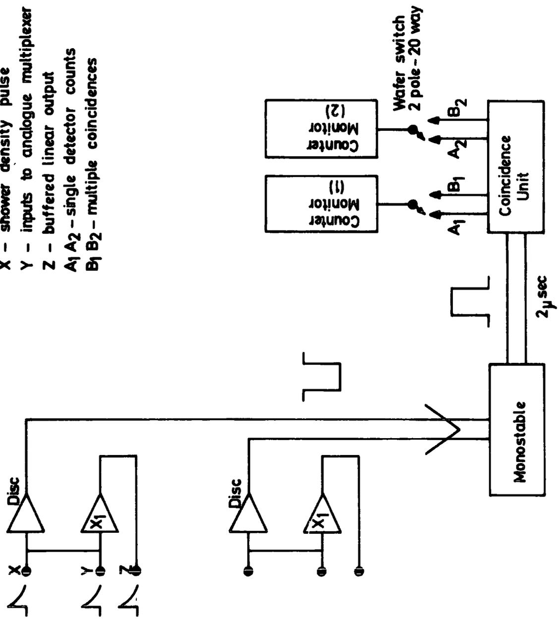
Figure 5-10 The array coincidence monitoring system.
