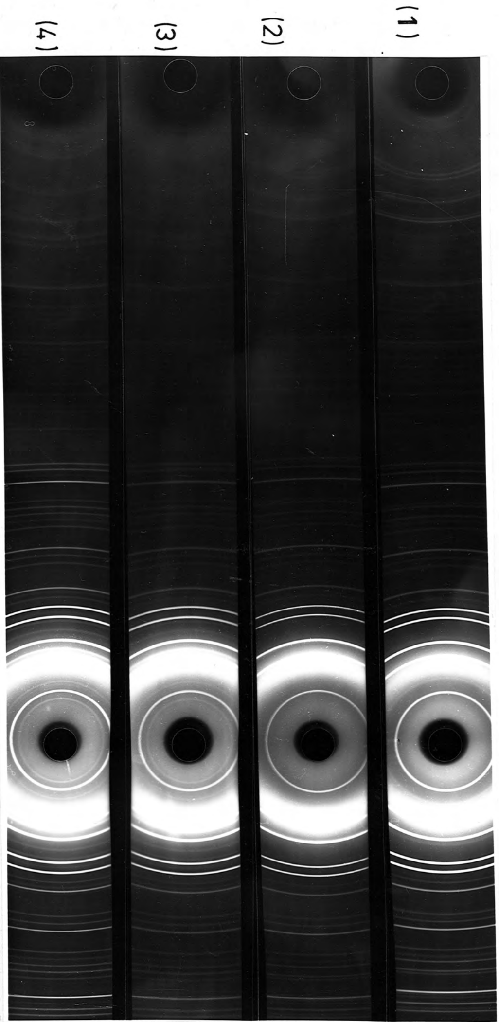
FIG. 1.9 X-ray diffraction patterns of (1) \text{Si}_3\text{N}_4 , (2) 5% MgO/ \text{Si}_3\text{N}_4 , (3) z = 3.2 sialon and (4) z = 4.0 sialon.
