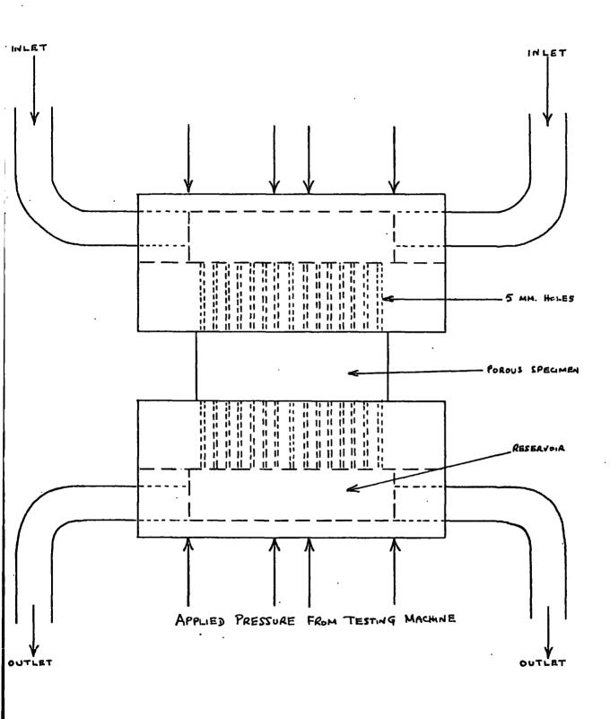
FIGURE 16: APPARATUS FOR MEASURING PERMEABILITY OF A MATERIAL UNDER STRAIN
