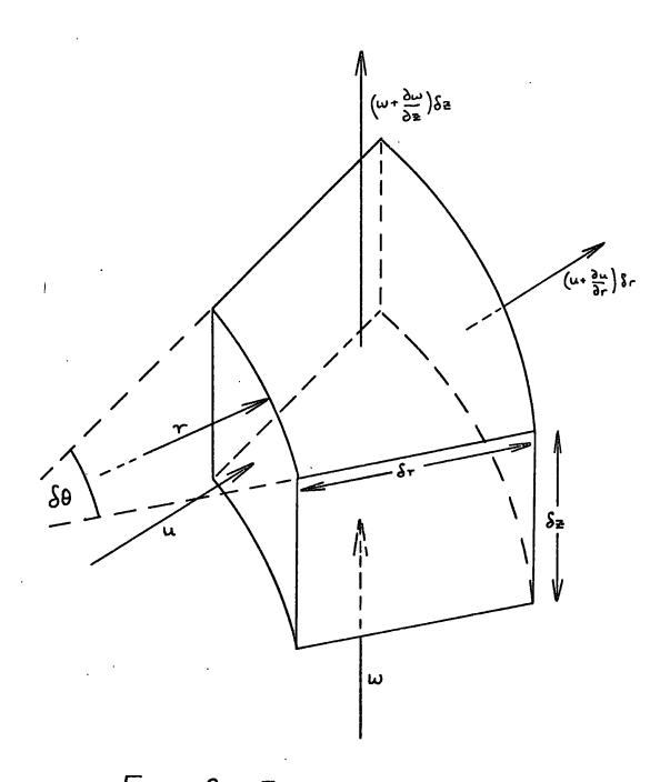
FIGURE 2 : FLOWS IN AN ELEMENT OF A MATERIAL WITH AXIAL SYMMETRY.
