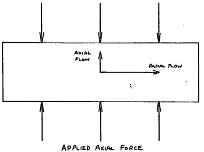
FIGURE 10 : DIRECTIONS OF AXAL AND RADIAL FLOW WITH APPLIED STRAIN
