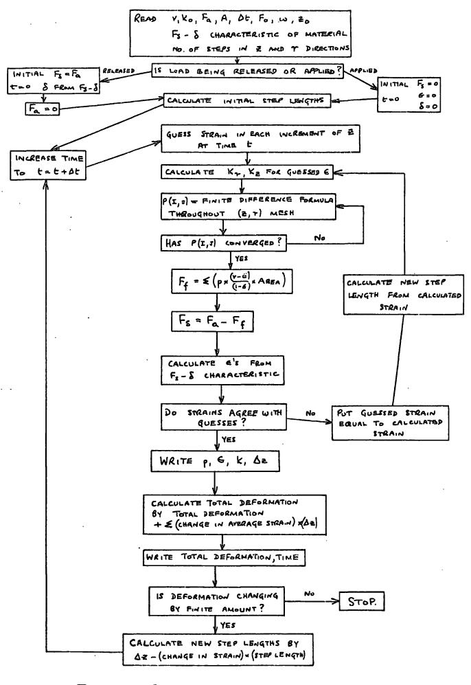
FIGURE 28: BLOCK DIAGRAM OF COMPUTER PROGRAM FOR AXIAL AND RADIAL FLOW.
