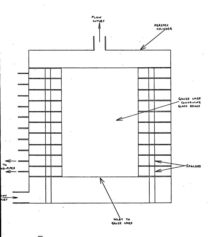
FIGURE 3 : APPARATUS FOR ONE-DIMENSIONAL FLOW
