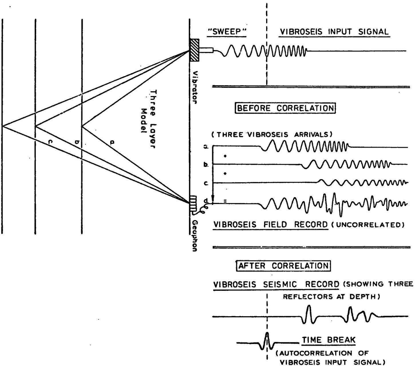
FIG. 1 - THE BASIC PRINCIPLES OF THE VIBROSEIS<sup>®</sup> SYSTEM
