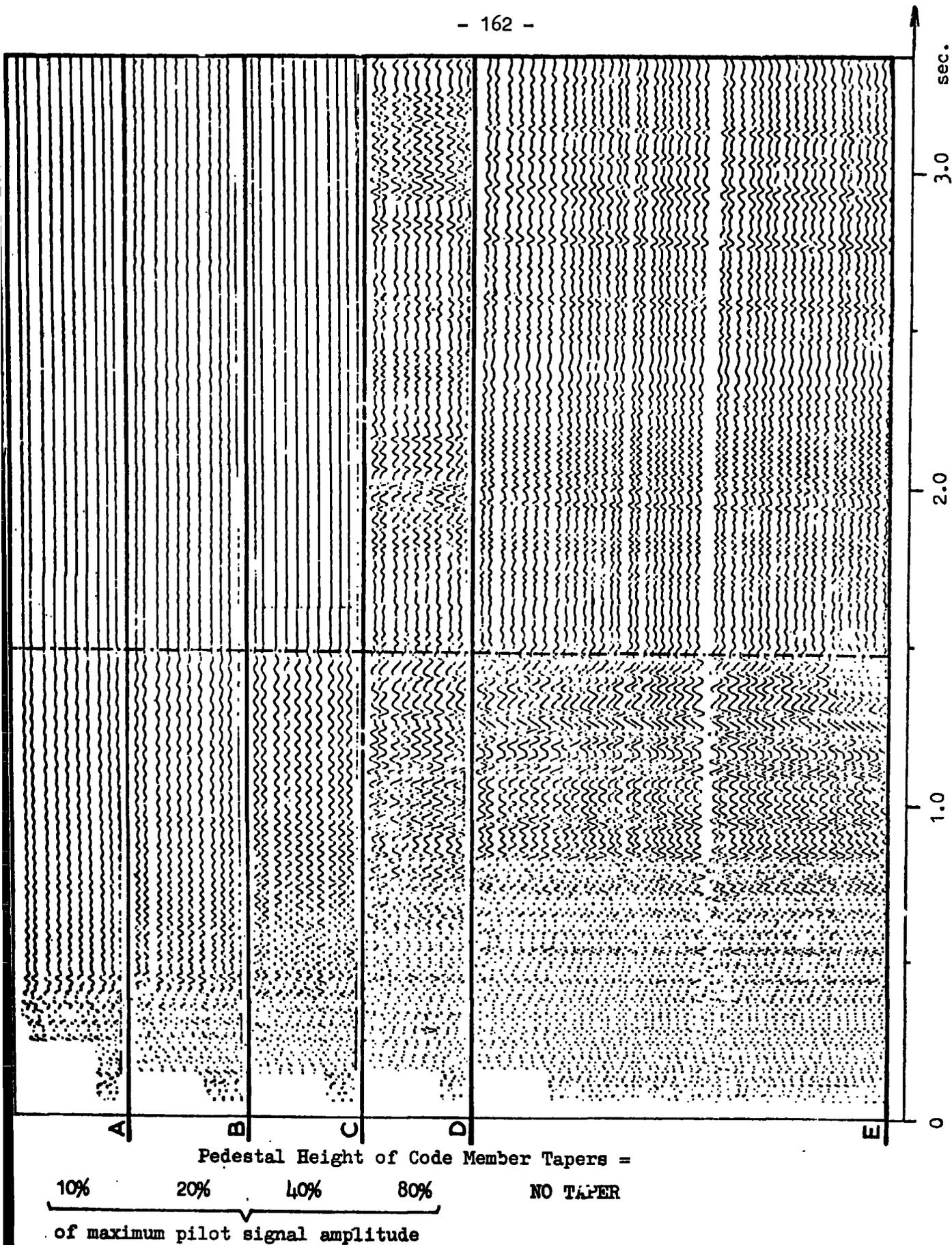
FIG. 62 - ONE-SIDED CROSSCORRELATION FUNCTIONS (PILOT SIGNAL/ACCELEROMETER OUTPUT)
