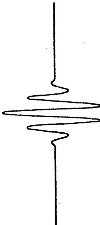
FIG. 17 - THE 'CHIRP' OR 'SWEEP' SIGNAL AND ITS AUTOCORRELATION
