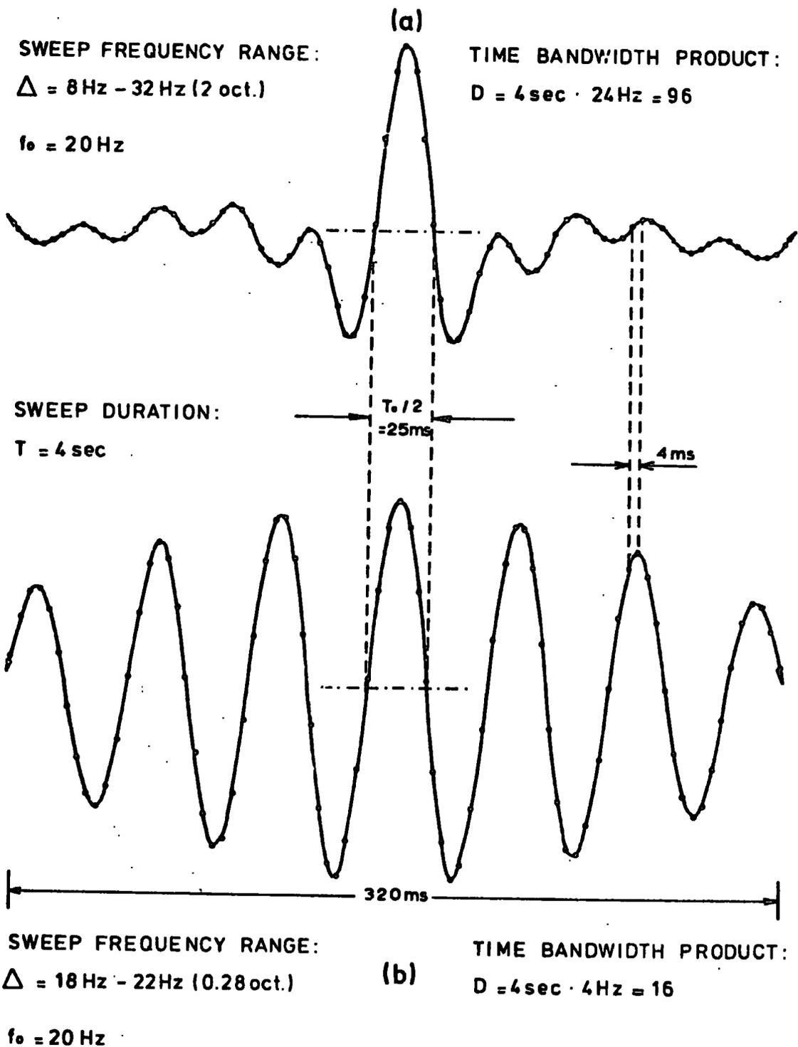
FIG. 7 - A/C-FUNCTION OF TWO DIFFERENT LINEAR SWEEPS
