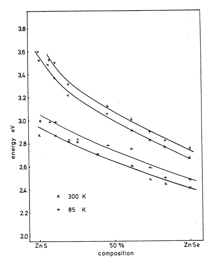
FIG 5.31 VARIATION OF PHOTOCONDUCTIVITY PEAK POSITION WITH COMPOSITION IN Zn (S,Se): I
