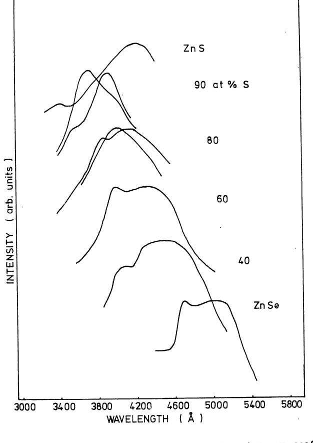
FIG 5.23 EXCITATION SPECTRA OF Zn(S,Se): I AT 300°K MONITORING S.A. EMISSION
