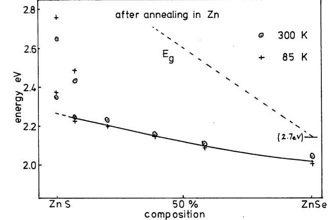
FIG 5.5 variation of photoluminescence peak position with composition before and after annealing in Zn
