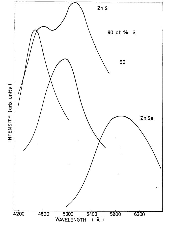
FIG 5.9 PHOTOLUMINESCENCE AT 85 K OF VERTICAL FURNACE CRYSTALS
