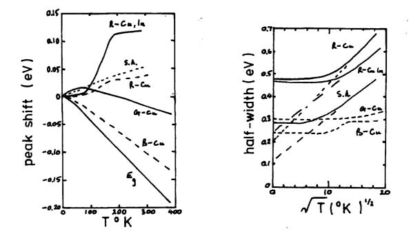
F1G 2.7 dependence of peak position and halfwidth of ZnS emissions on temperature
