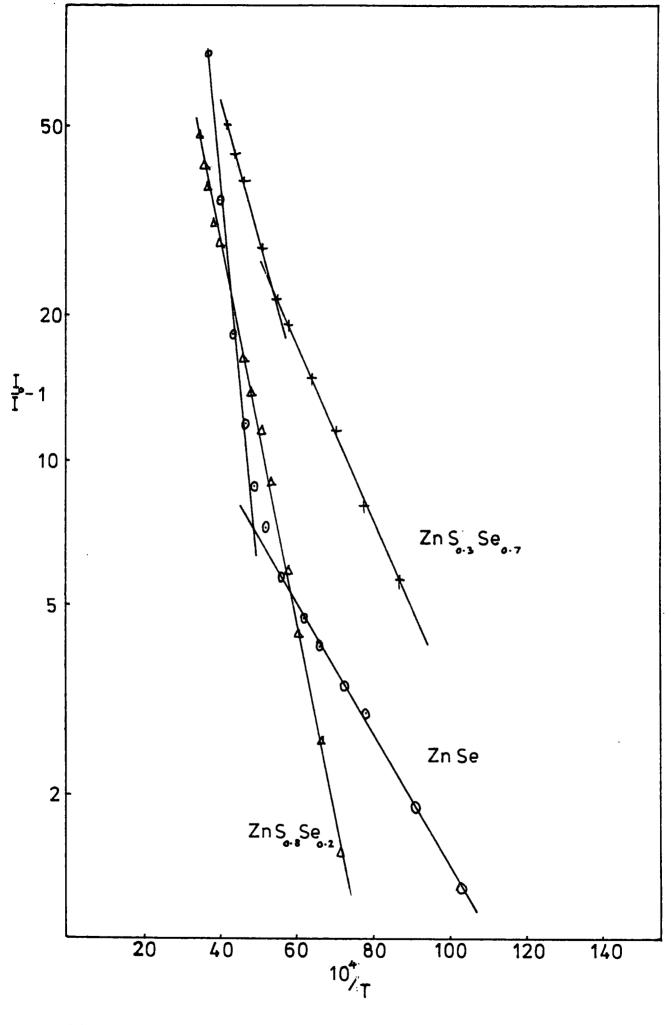
FIG 5.35 THERMAL QUENCHING OF Zn (S, Se): I
