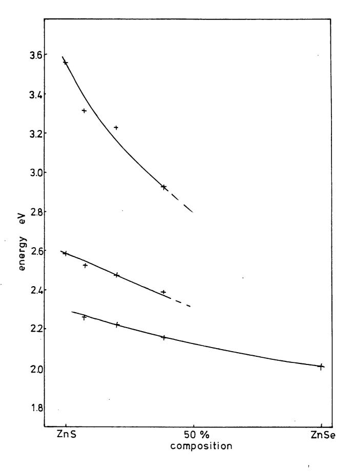
FIG 5.17 VARIATION OF CATHODOLUMINESCENCE PEAK POSITION WITH COMPOSITION IN Zn (S,Se): I,Zn
