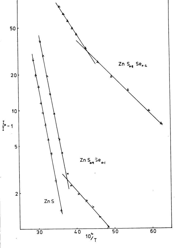
FIG 5.36 THERMAL QUENCHING OF Zn (S, Se): I
