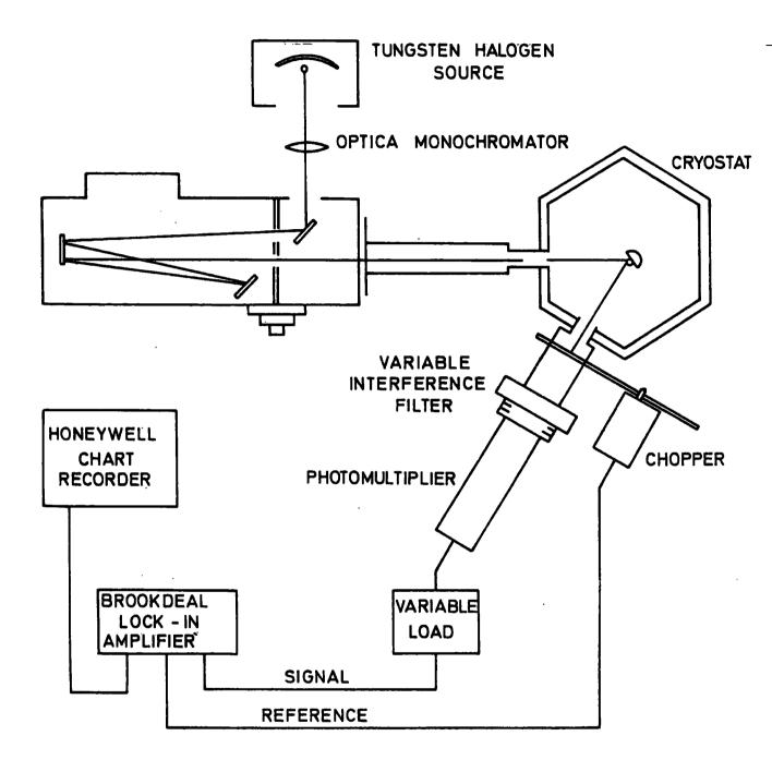
FIG. 4.5 EXPERIMENTAL ARRANGEMENT FOR MEASURING PHOTOLUMINESCENT EXCITATION SPECTRA.
