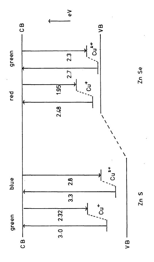
FIG 6.17 schematic representation of possible emission and excitation processes in Zn(S,Se): Cu
