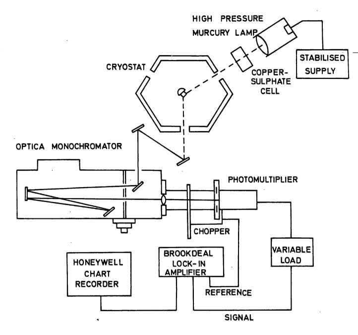
FIG. 4,4 EXPERIMENTAL ARRANGEMENT FOR MEASURING PHOTOLUMINESCENT EMISSION SPECTRA.
