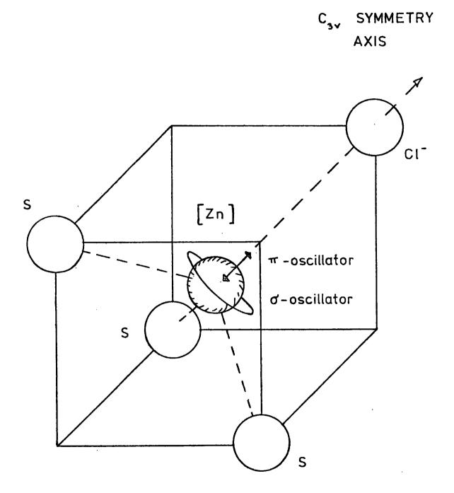
FIG 2.11 ASSOCIATION MODEL FOR SELF-ACTIVATED LUMINESCENCE CENTRE IN CUBIC ZnS:Cl
