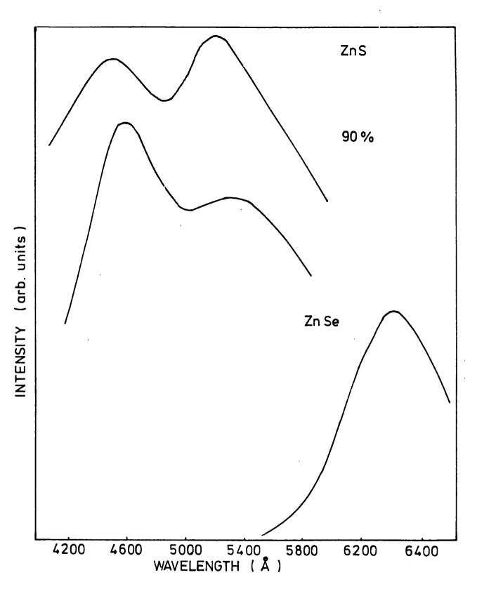
FIG 5.10 PHOTOLUMINESCENCE AT 300 °K OF VERTICAL FURNACE CRYSTALS ANNEALED IN Zn
