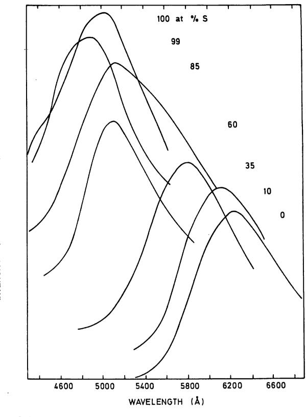
FIG. 6.1 Photoluminescence spectra of Zn(S,Se) : I, Cu crystals
