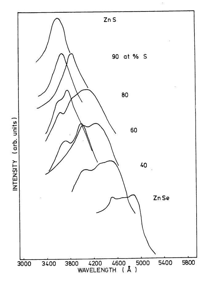
FIG 5.24 EXCITATION SPECTRA OF Zn (S, Se): I AT 85 ° K MONITORING S.A. EMISSION
