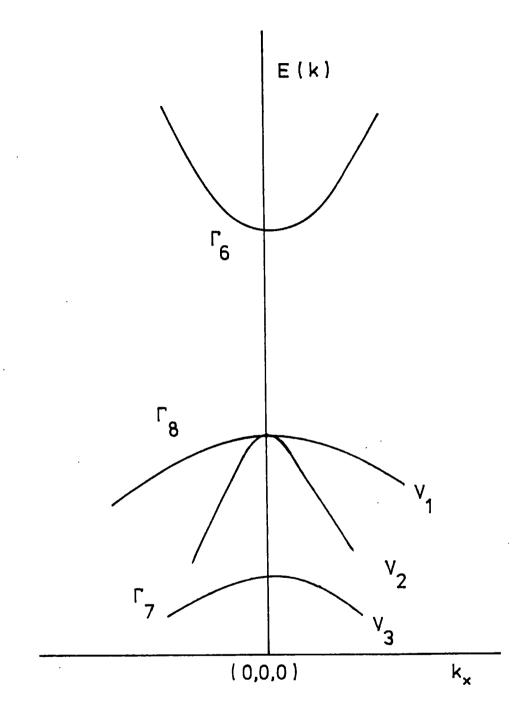
FIG 2.2a CONDUCTION AND SPIN-ORBIT SPLIT VALENCE BANDS OF A ZINC BLENDE CRYSTAL symmetry states, namely  $L_3$  and  $X_5$  shown in the energy band diagrams.
