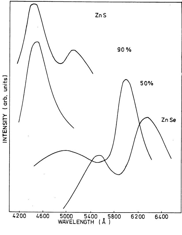
FIG 5.11 PHOTOLUMINESCENCE AT 85 °K OF VERTICAL FURNACE CRYSTALS ANNEALED IN Zn
