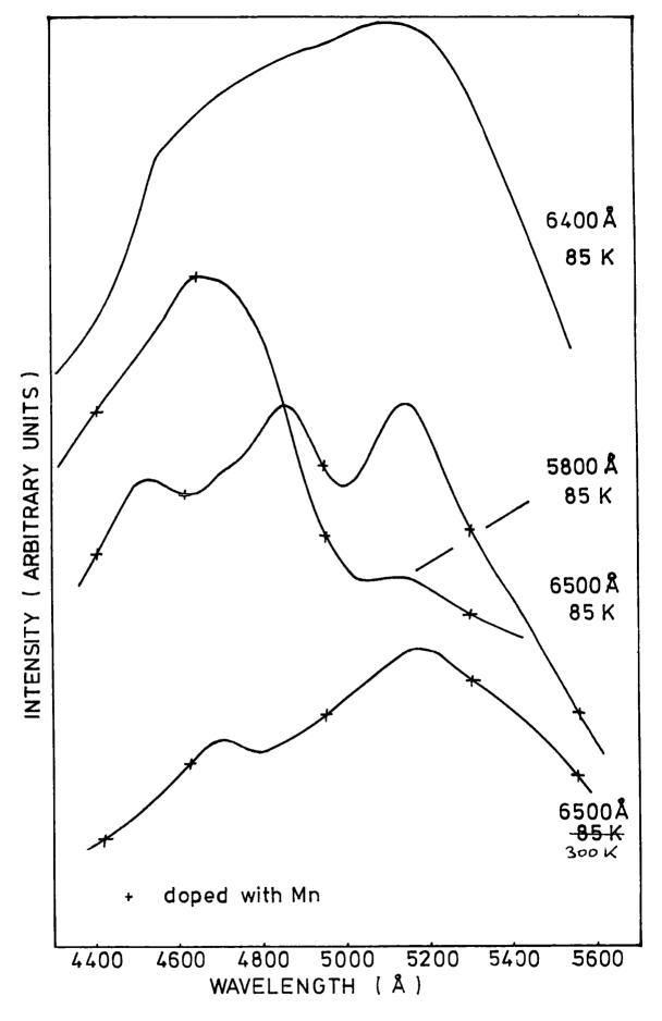
FIG 7.15 EXCITATION SPECTRA OF ZnSe:Cl,Mn,Cu,Zn AND ZnSe:Cl,Cu,Zn MONITORING 5800Å AND 6500Å.
