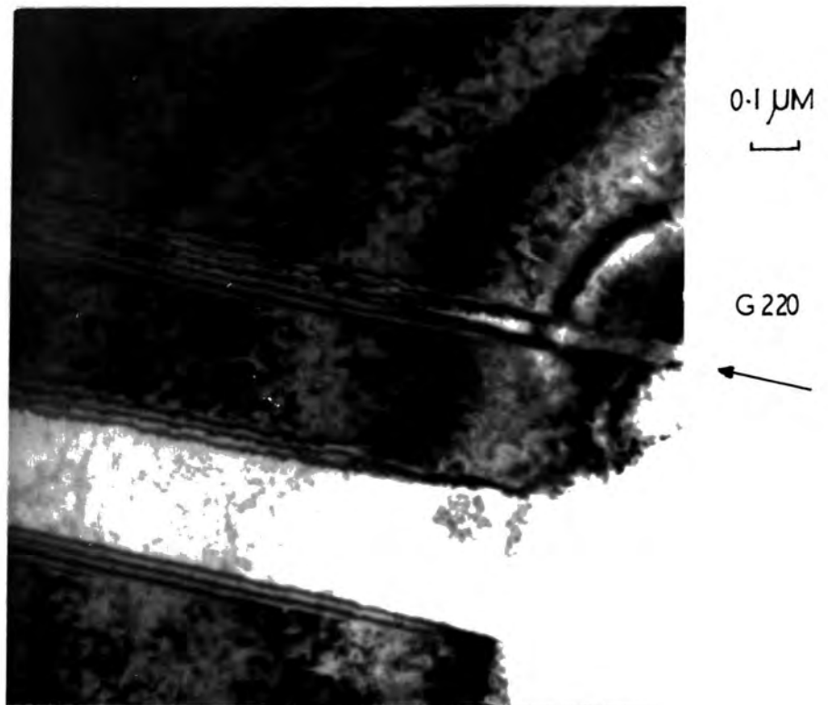
Figure 5.4.2: An irregularity in the specimen edge near a twin boundary
