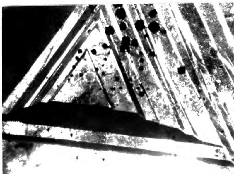
A. Triangular growth features on a facet. The dark spots are globules of selenium which sublimed from the tail reservoir as the crystal cooled (Mag. x 25)
