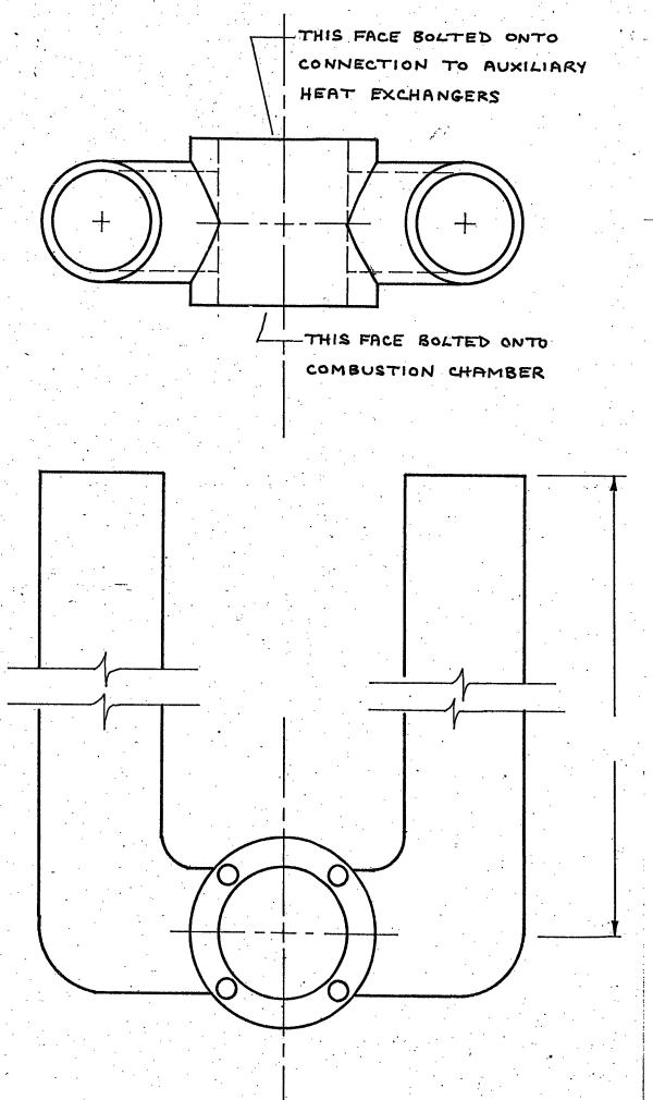
FIGURE 3.4: AIR INLET MANIFOLD
