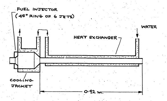
FIGURE 8.2 : FIRST COMBUSTION CHAMBER WITH
