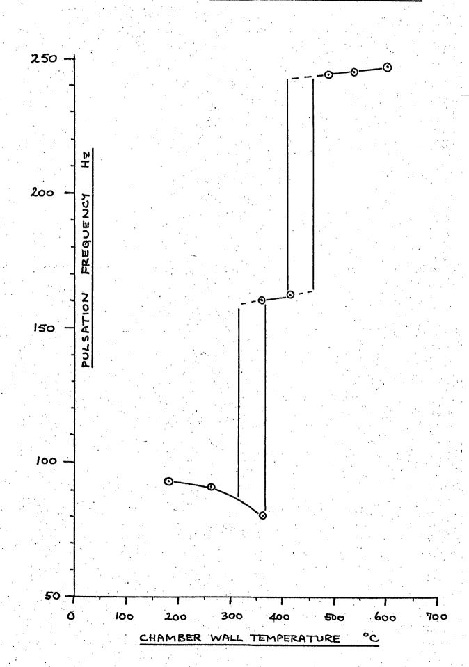
FIGURE B.11: VARIATION OF COMBUSTOR FREQUENCY
