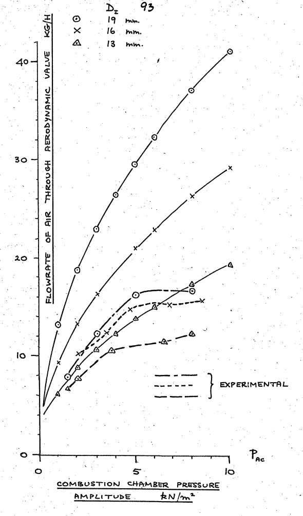
FIGURE 4.3: NET FLOW THROUGH AERODYNAMIC
