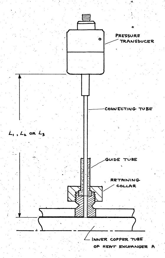
FIGURE 3.16: PRESSURE TRANSDUCER MOUNTING
