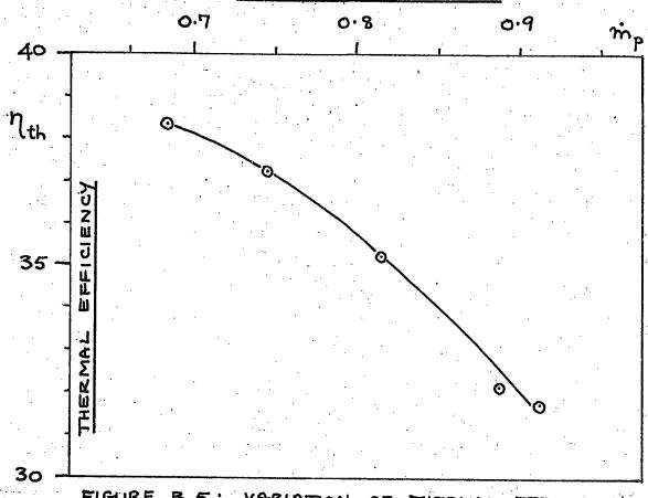
FIGURE B.5: VARIATION OF THERMAL EFFICIENCY
