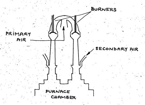
FIGURE 1.14: COUNTER- PHASE PULSATING COMBUSTER
