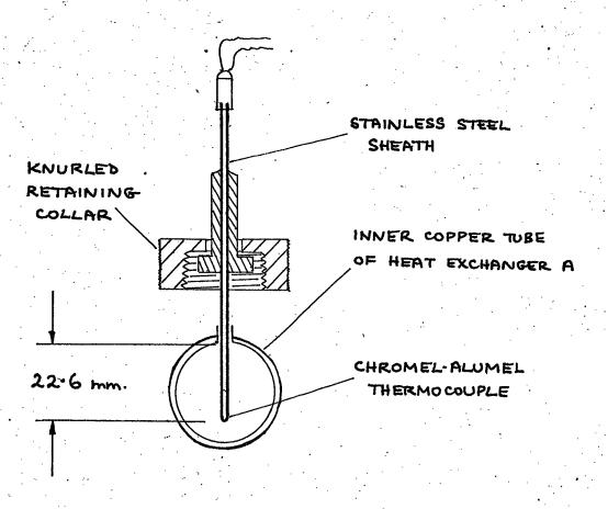
FIGURE 3.11: GAS TEMPERATURE THERMOCOUPLE
