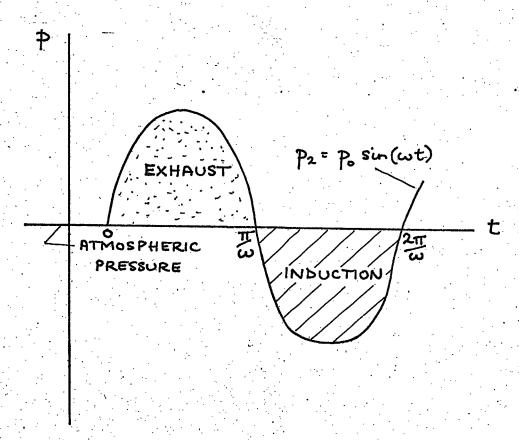
FIGURE 2.11: INDUCTION AND EXHAUST
