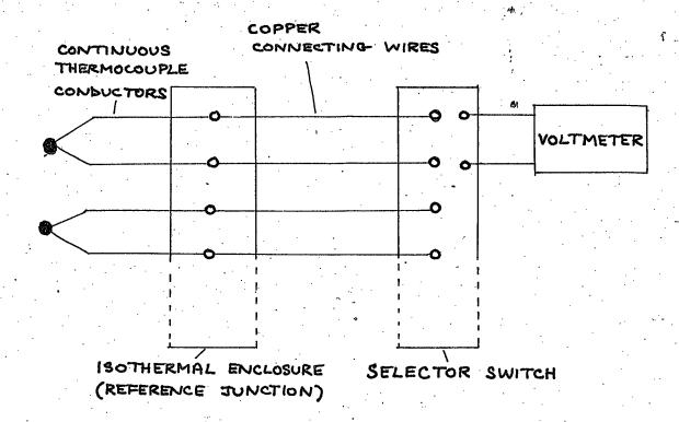
FIGURE 3.10 : THERMOCOUPLE CIRCUIT
