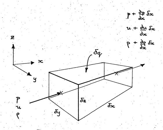
FIGURE 2.4! ELEMENTAL CONTROL VOLUME OF
