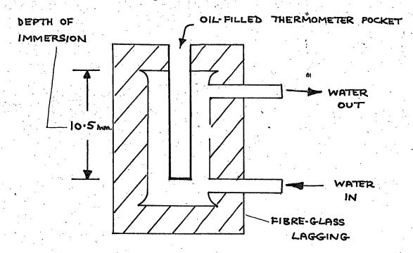
FIGURE 3.14: THERMOMETER POCKET
