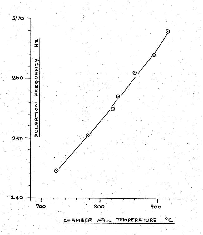
Figure B.11. shows that, having reached the 245 Hz mode, the combustor frequency rose at the rate of 0.25 Hz/°C but did not jump higher as the chamber reached its maximum temperature of approximately 920°C. The rise was attributed to the increasing velocity of sound in the gases.
