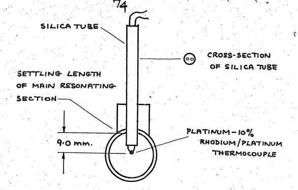
FIGURE 3.12: GAS TEMPERATURE THERMOCOUPLE
