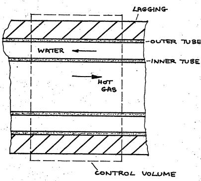
FIGURE 4.19 : TYPICAL SECTION OF HEAT EXCHANGER A
