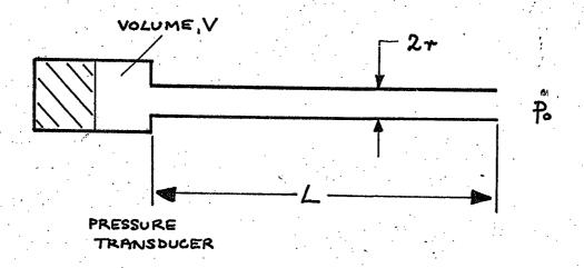
FIGURE 3.17 : IDEALISED PRESSURE MEASURING
