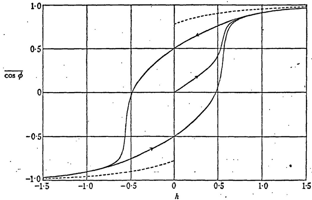
FIGURE 6.11 Magnetization curves for prolate (full curves) and oblate (broken curves) spheroids orientated at random. The curves refer to similar prolate (or oblate) spheroids orientated at random.  $\overline{\cos \phi}$  is proportional to the mean resolved magnetization per spheroid in the positive field direction, or to the resultant magnetization in this direction of the assembly.  $H = (|D_a - D_b|) I_0 h$ .
