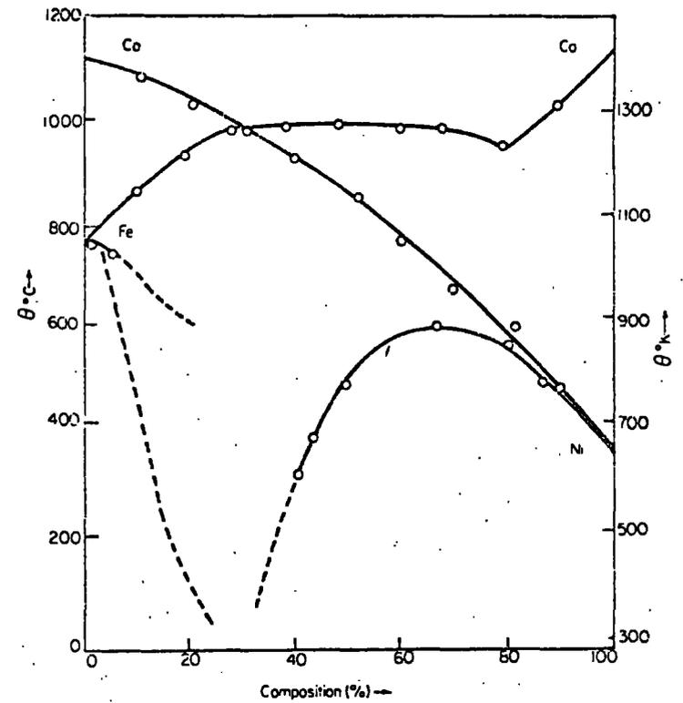
Figure 3.2 Magnetic transformation temperatures of Fe-Co, Fe-Ni and Co-Ni alloys
