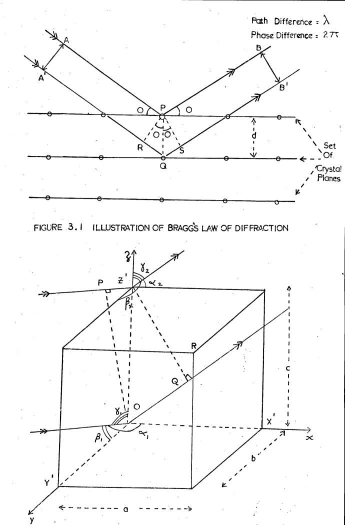
FIGURE 3.2 ILLUSTRATION OF THE DERIVATION OF THE LAUE EQUATIONS
