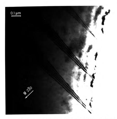
Figure 7.11: A group of long intrinsic stacking faults in  $2nSe_{0.4}S_{0.6}$
