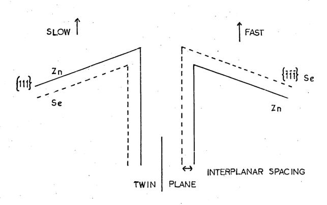
FIGURE 7.250 FAST AND SLOW GROWING FACES ON EITHER SIDE OF A TWIN BOUNDARY
