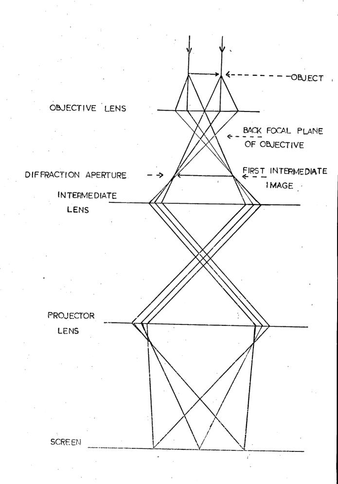
FIGURE 2.9 RAY PATHS UNDER DIFFRACTION CONDITIONS
