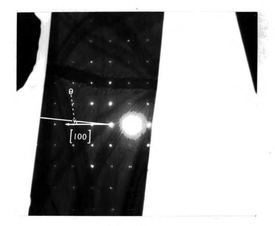
FIGURE 2.13 MICROGRAPH WITH SUPERIMPOSED DIFFRACTION PATTERN FROM MOOS CRYSTAL
