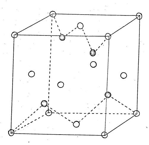
FIGURE 4.2 THE ZINCBLENDE STRUCTURE
