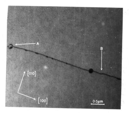
Figure 5.9: A precipitate at A exhibiting an unusual contrast effect
