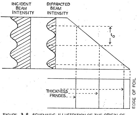
FIGURE 3.9 SCHEMATIC ILLUSTRATION OF THE ORIGIN OF THICKNESS FRINGE CONTRAST
