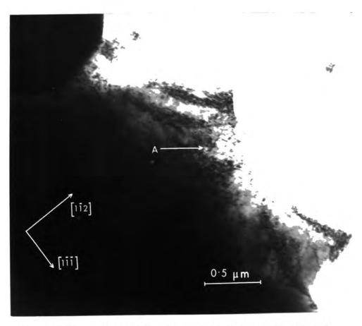
Figure 7.20: A bright field image of an ion beam thinned sample of ZnSe
