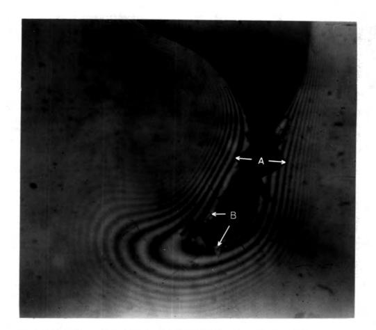
Figure 5.1: Photomicrograph of thinned MgO showing interference fringes x 200
