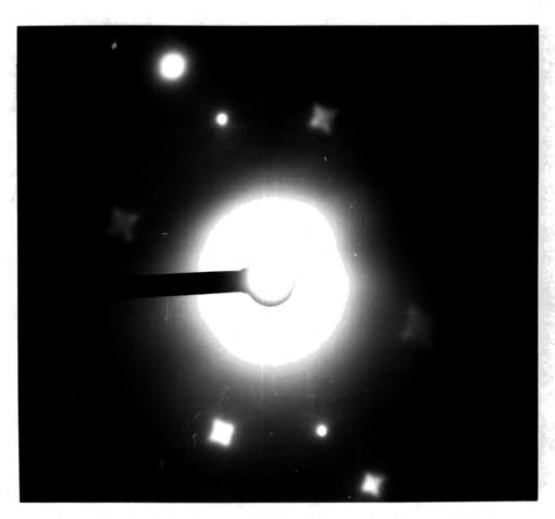
Figure 5.11: Diffraction from two overlapping crystals
