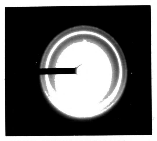
Figure 5.18: A diffraction pattern from extracted platelet shaped precipitates
