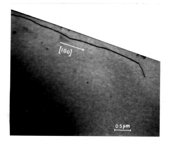
Figure 5.3: An edge dislocation lying parallel to a fractured edge of a specimen
