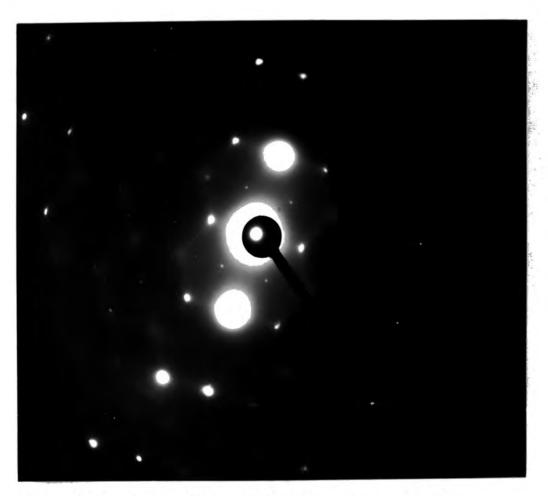
Figure 7.19: Selected area diffraction pattern from the region in Figure 7.18
