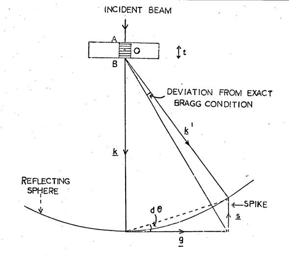
FIGURE 3.8 ILLUSTRATING REFLECTING SPHERE CONSTRUCTION FOR KINEMATICAL CONDITIONS (EXAGGERATED)
