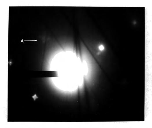
Figure 5.10: A <100> diffraction pattern containing spots showing 'fine structure'.
