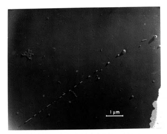
Figure 5.17: A shadowed extraction replica showing a linear array of precipitates
