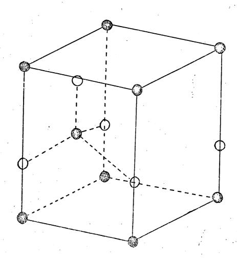
FIGURE 4.3 THE WURTZITE STRUCTURE
