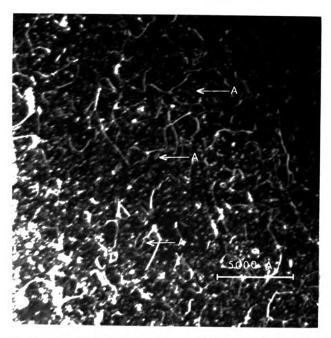
Figure 6.3: A dark field image of the region in Figure 6.2 taken using a {200} diffracted beam
