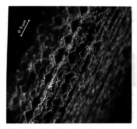
Figure 5.15: Reflection electron micrograph showing pyramidal etch hillocks
