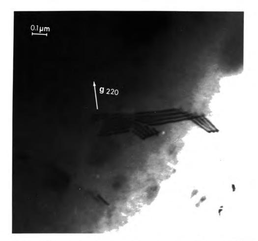
Figure 7.15: A stacking fault that has slipped from one {111} plane to another
