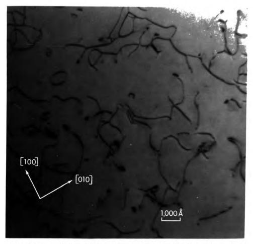
Figure 6.4: Dislocation tangles and loops in MgO irradiated with a dose of 3.66 x 10<sup>20</sup> nvt and annealed at 1450°C
