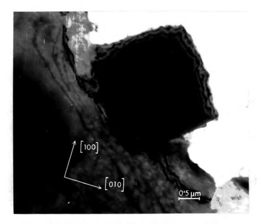
Figure 5.14: An etch hillock at the edge of a thin specimen
