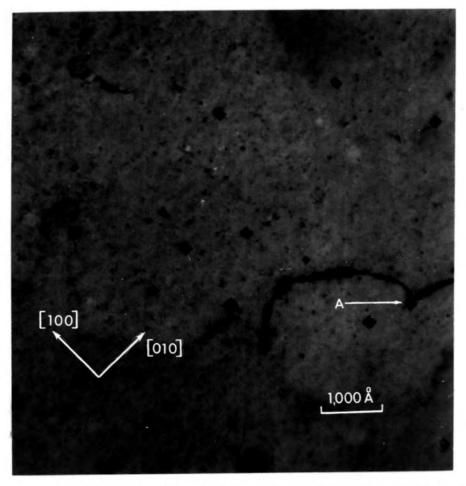
Figure 6.8: As in Figure 6.7, but in this case showing the location of a cavity at a cusp in a dislocation
