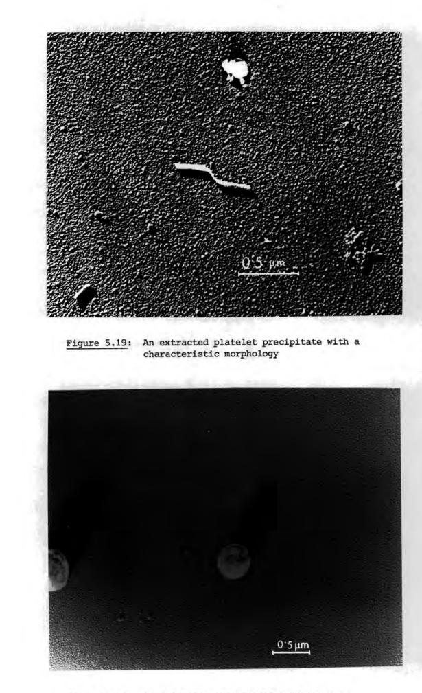
Figure 5.20: An extracted precipitate exhibiting an unusual contrast effect
