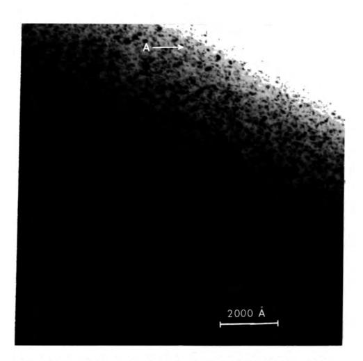
Figure 6.1: Defect clusters in MgO irradiated with a dose of 6.0 x  $10^{19}$  nvt
