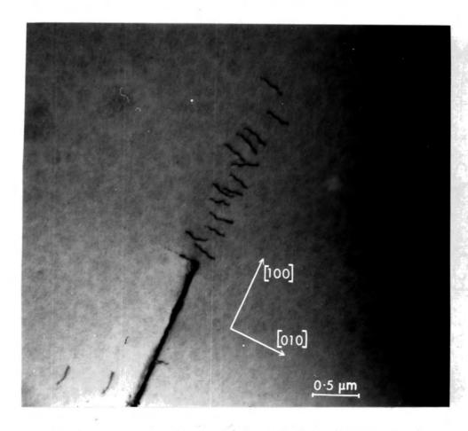
Figure 5.2: Dislocations at the end of a cleavage crack
