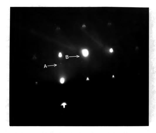
Figure 5.16: Reflection electron diffraction pattern taken from the region shown in Figure 5.15
