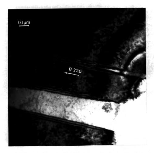
Figure 7.3: An irregularity in a specimen edge at a twin boundary
