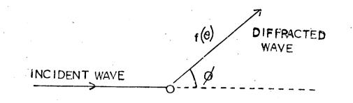
FIGURE 3.3 THE AMPLITUDE PHASE DIAGRAM FOR SCATTERING FROM A UNIT CELL CONTAINING ONE LATTICE POINT
