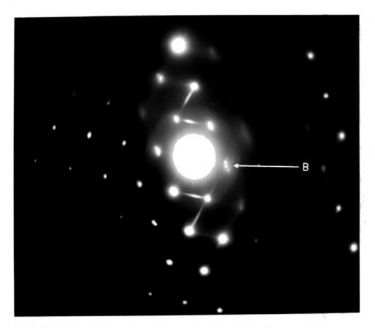
Figure 7.21 The selected area diffraction pattern from the region in Figure 7.20
