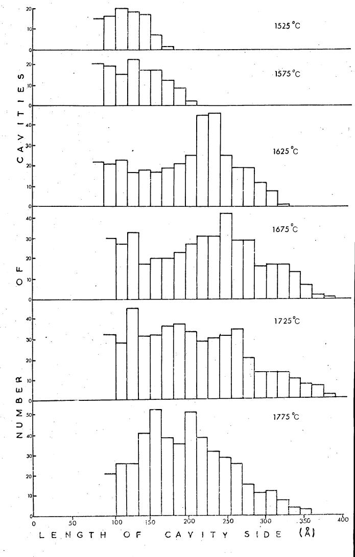
FIGURE 6.9 VARIATION OF CAVITY SIZE WITH ANNEALING TEMPERATURE
