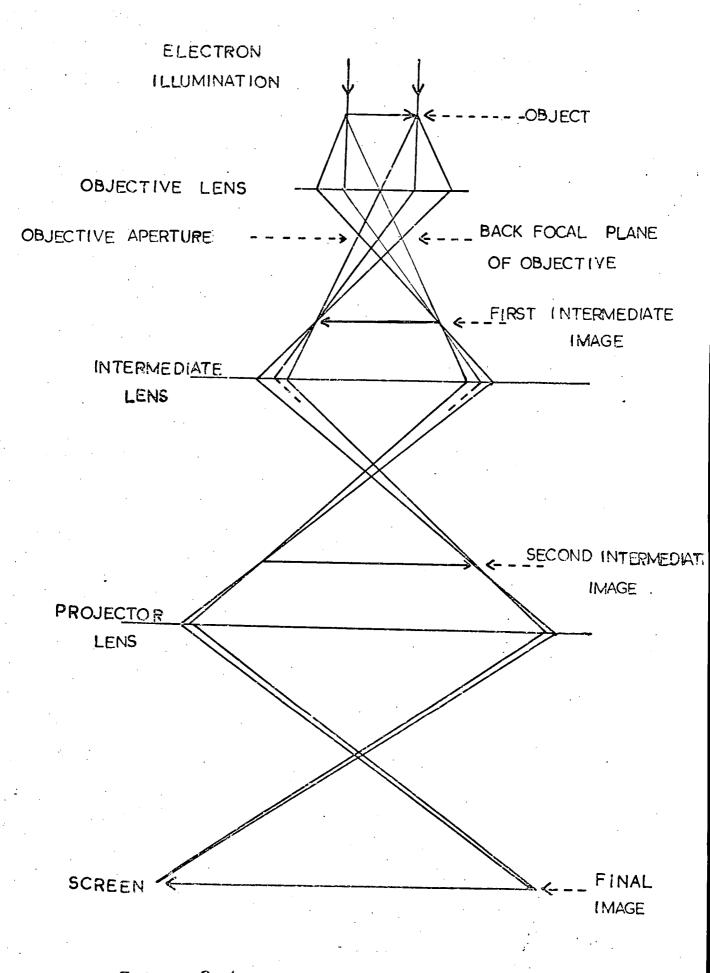
FIGURE 2.4 RAY PATHS UNDER MICROSCOPY CONDITIONS
