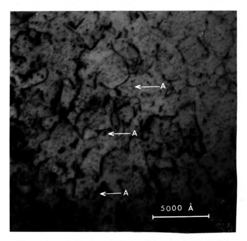
Figure 6.2: Dislocation tangles and small loops in MgO irradiated with a dose of 3.66 x 10<sup>20</sup> nvt and annealed at 1050°C
