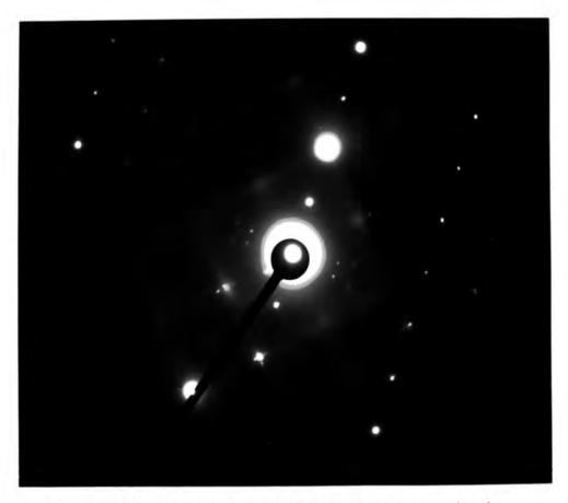
Figure 7.24: Selected area diffraction from a <100> zone axis of an ion beam thinned ZnSe specimen
