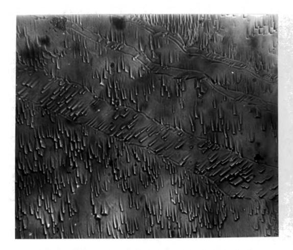
Figure 7.4: A photomicrograph of the Zn surface of an etched ZnSe sample demonstrating no change in polarity across twin boundaries x 200
