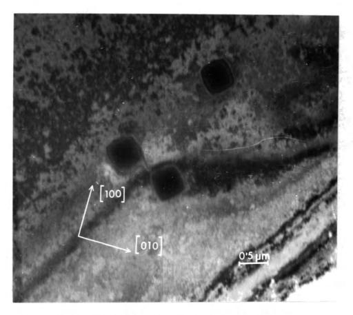
Figure 5.12: Etch hillocks revealed by absorption contrast
