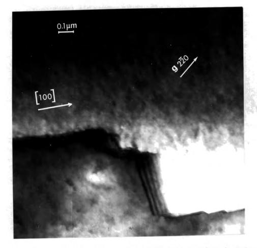
Figure 7.5: Fringe contrast at a <100> tilt boundary in ZnSe
