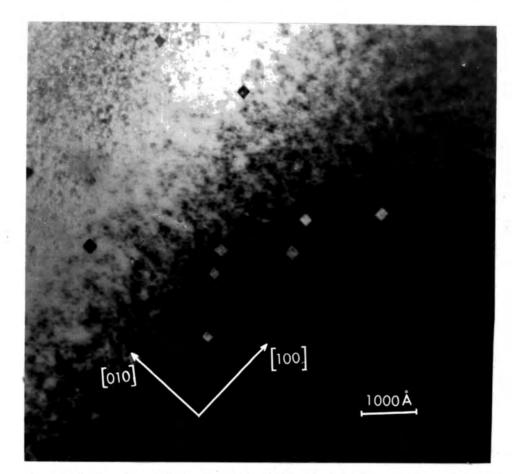
Figure 6.5: Cavities showing light and dark contrast in MgO irradiated with a dose of 3.66 x 10<sup>20</sup> nvt and annealed at 1525 °C
