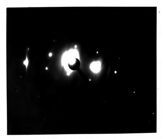
Figure 7.14: The selected area diffraction pattern illustrating the diffraction conditions operative when recording Figures 7.12 and 7.13
