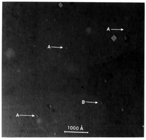
Figure 6.6: Cavities which are rectilinear rather than cuboidal in a sample treated similar to that shown in Figure 6.5
