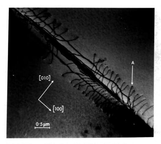
Figure 5.4: A cleavage crack showing edge and screw dislocations
