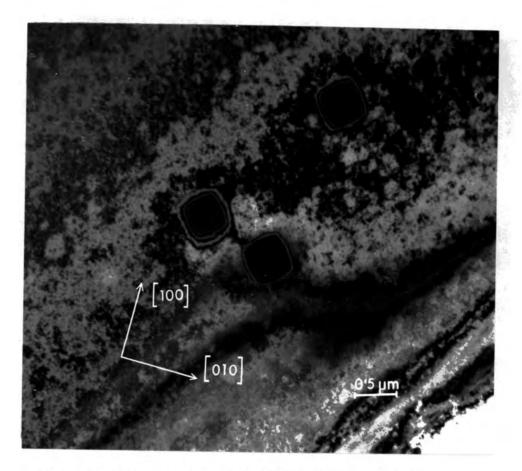
Figure 5.13: The same hillocks as in Figure 5.12 exhibiting diffraction contrast
