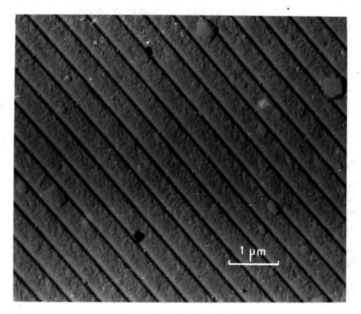
FIGURE 2.10 DIFFRACTION GRATING REPLICA HAVING 55000 LINES PER INCH
