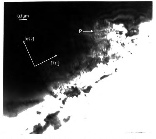
Figure 7.18: Overlapping layers of wurtzite and sphalerite structuresgiving rise to moiré fringe contrast in ZnSe<sub>0.4</sub>S<sub>0.6</sub>
