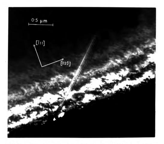
Figure 7.13: The dark field image of the stacking fault shown in Figure 7.12 recorded using the strong diffracted beam in Figure 7.14
