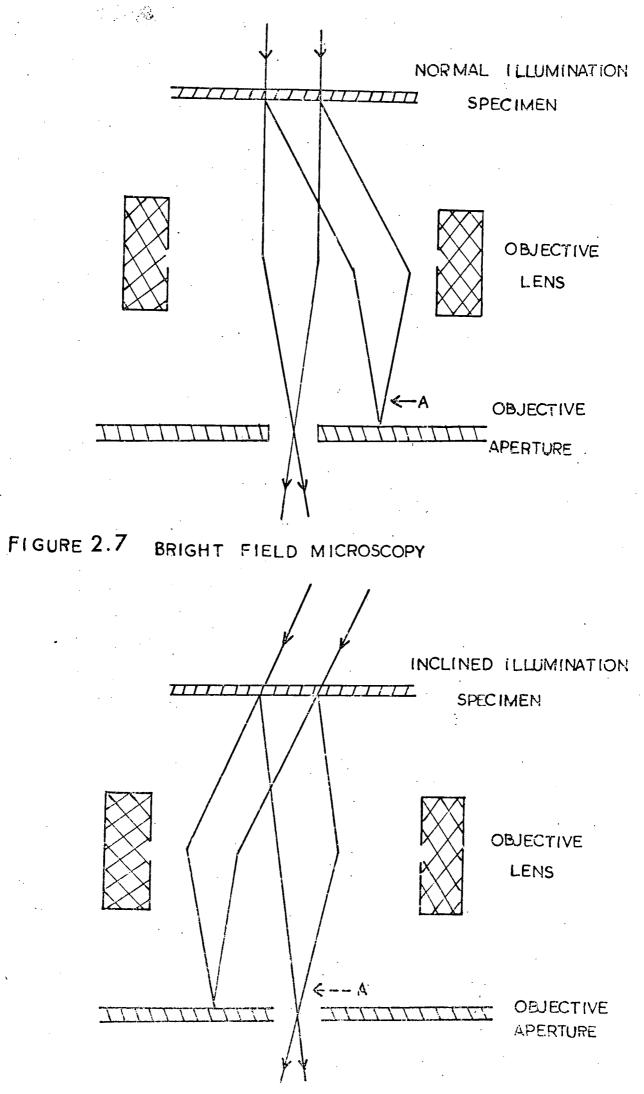
FIGURE 2.8 DARK FIELD MICROSCOPY
