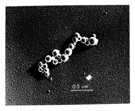
Figure 5.21: A cluster of extracted spherical precipitates
