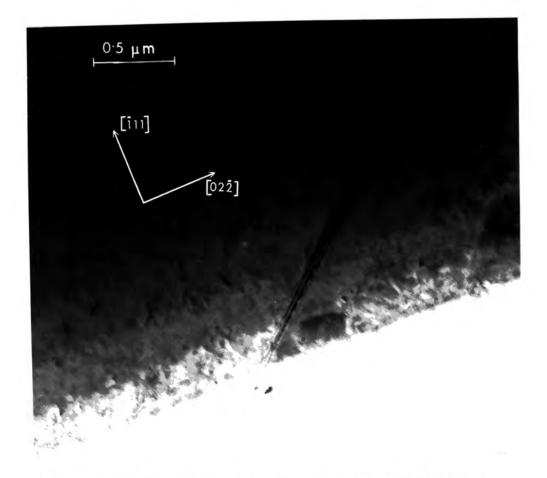
Figure 7.12: The bright field image of a single stacking fault in  $\text{ZnSe}_{0.4}\text{S}_{0.6}$
