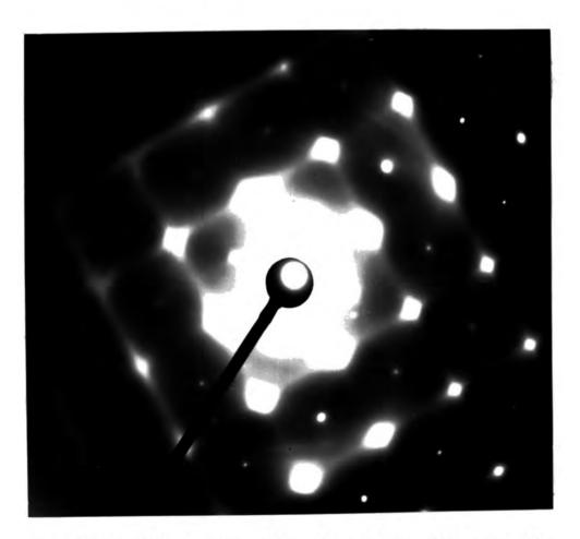
Figure 7.7: Selected area diffraction from a <100> zone axis of ZnSe using 100 KV electrons
