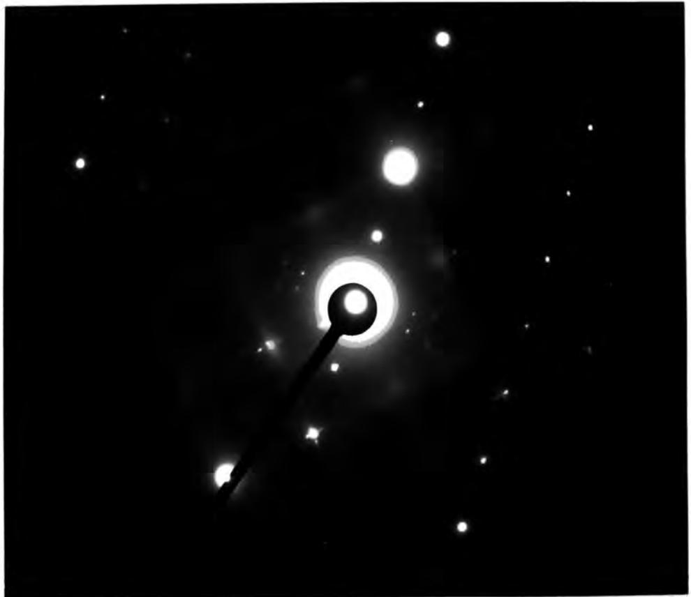
Figure 7.24: Selected area diffraction from a  $\langle 100 \rangle$  zone axis of an ion beam thinned ZnSe specimen
