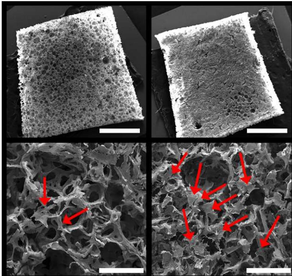
**Figure 5.18** SEM images of 7 day time points showing increased cell coverage on the wet plasma treated polyHIPE slice (RHS) as compared to the blank polyHIPE (LHS). Top scale bar is 1 mm, lower scale bar is 100  $\mu\text{m}$ . Red arrows indicate individual MG63 cells.
