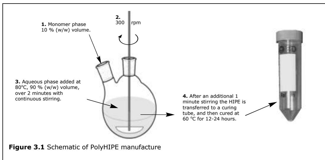
The polyHIPEs made with relation to this project were 90 % internal phase emulsions, unless stated otherwise. The material preparation was followed as set out in the paper by Carnachan et al.<sup>1</sup> with the aqueous phase temperature set at 80 °C. The monomer phase consisted of a styrene : divinylbenzene : 2-ethylhexyl
