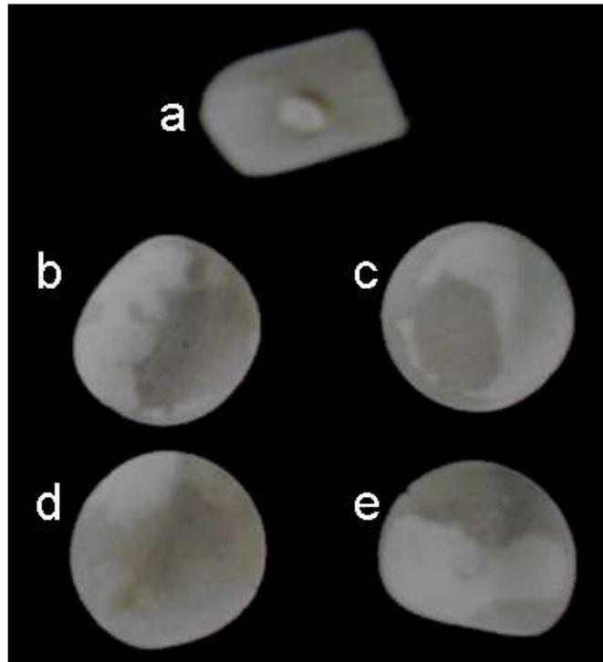
**Figure 5.2** Photograph of water droplet behaviour. All treated at 50 ml/min O<sub>2</sub>. a: untreated polyHIPE slice, b: 50 W, 1 minute plasma treatment, c: 50 W, 2 minutes plasma treatment, d: 50 W, 3 minutes plasma treatment, e: 75 W, 1 minute plasma treatment
