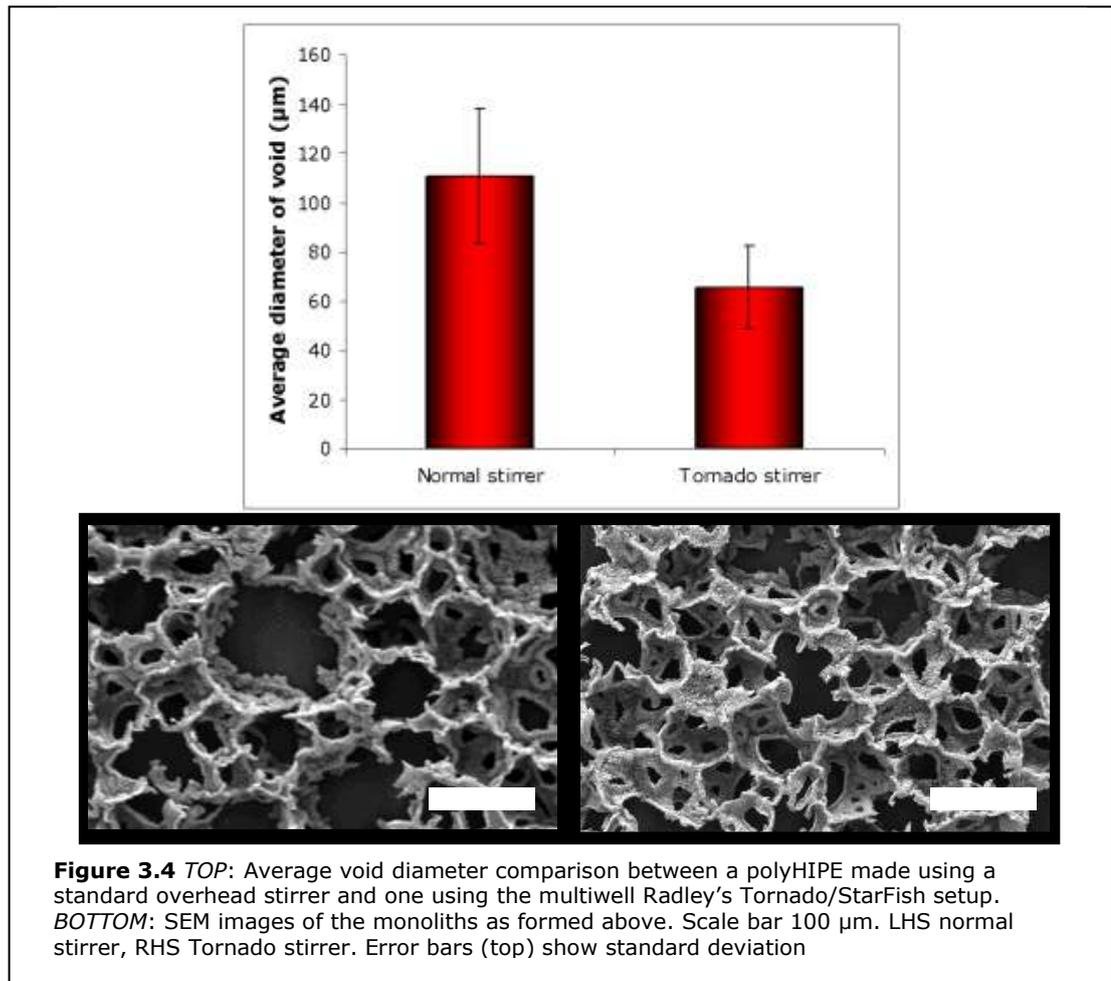
The interconnect diameter is significantly larger in the normal stirrer polyHIPE (nP) and has a larger standard deviation. The Tornado stirrer polyHIPE (tP) has a lower average interconnect diameter than the nP. This would indicate that the tP parent emulsion is more stable than the nP made emulsion. In most instances this would be advantageous, but in this case, where the void diameter has been optimised to a larger, specific diameter, it is a disadvantage. Although there are potential time
