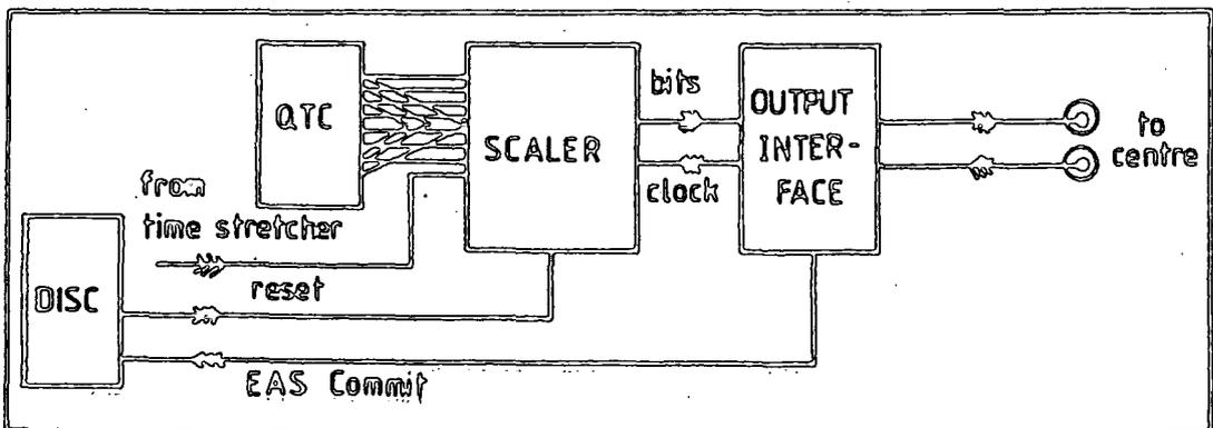
level was exceeded); and a pulse was sent to the EAS coincidence unit in the central recording station. If an EAS coincidence was not generated in the  $5\mu\text{s}$  following a detector trigger, the discrimination unit initiated the clearance of the digitisation system in readiness for another light pulse. The propagation time through the discriminator was 20 ns with a jitter of  $< 1$  ns, and a positive feedback system was employed to ensure the same delay for large and small pulses.
