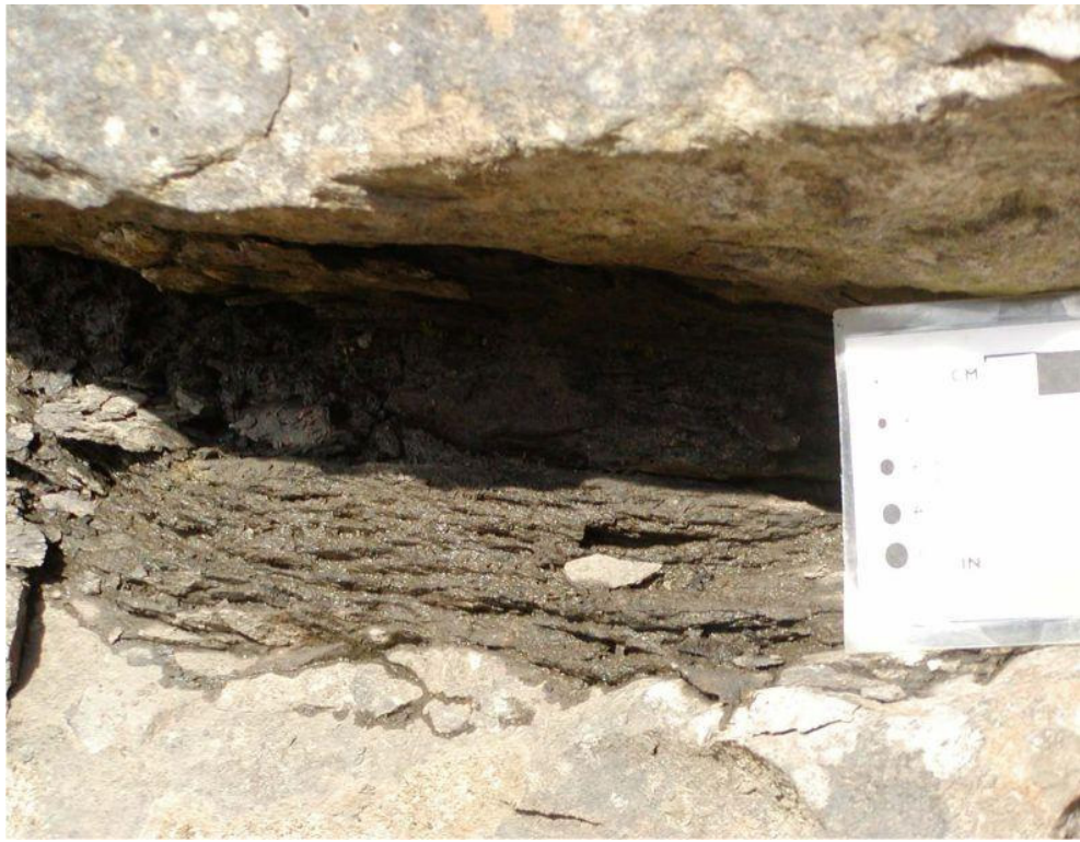
Figure 3.22. Planer bedded mudstone parting. Bedding plane approximately 60 millimetres thick. (Lanehead Quarry Weardale OS 39885 54052)
