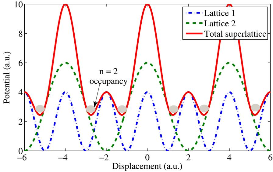
Figure 6.2: Schematic potential from an optical super-lattice created by overlapping two lattices (all units are arbitrary). Grey circles represent a loading of two atoms (or  $N/2$ ) in the ground state of each well. Our suggested scheme tunes the interactions to the desired value and then turns off the double frequency (dotted line) lattice leaving only the broader lattice (dot-dashed line), after which the atomic dimers collide.
