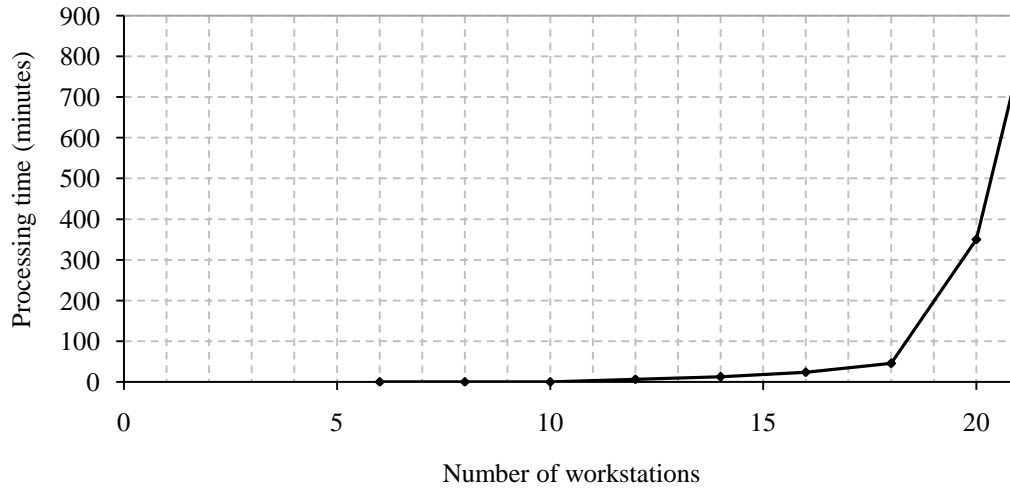
Figure 3.4: Schematic showing the duration of computational time against the number of workstations.
