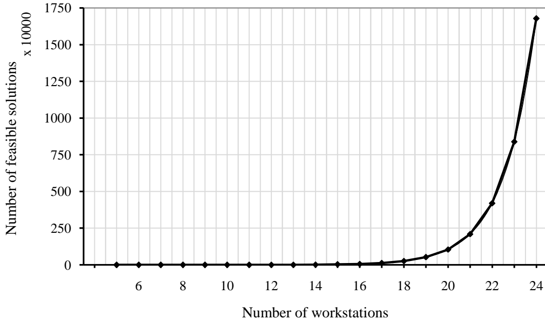
Figure 1.2: Growth of allocation of inspection stations problem search space. The horizontal axis is the number of workstations in an allocation problem. The vertical axis is the number of feasible solutions that have to be considered. The figure shows an exponential growth in search space size against problem size.
