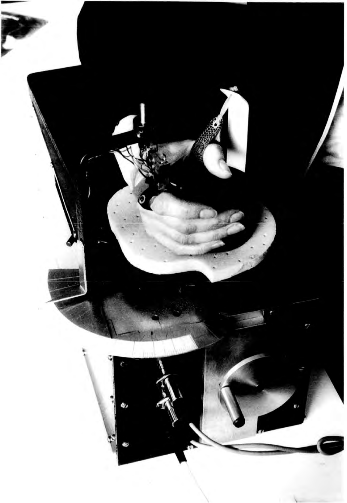
FIGURE 3•6. ARTHROGRAPH WITH THE HAND IN POSITION SHOWING THUMB SUPPORT AND FINGER GRIP.
