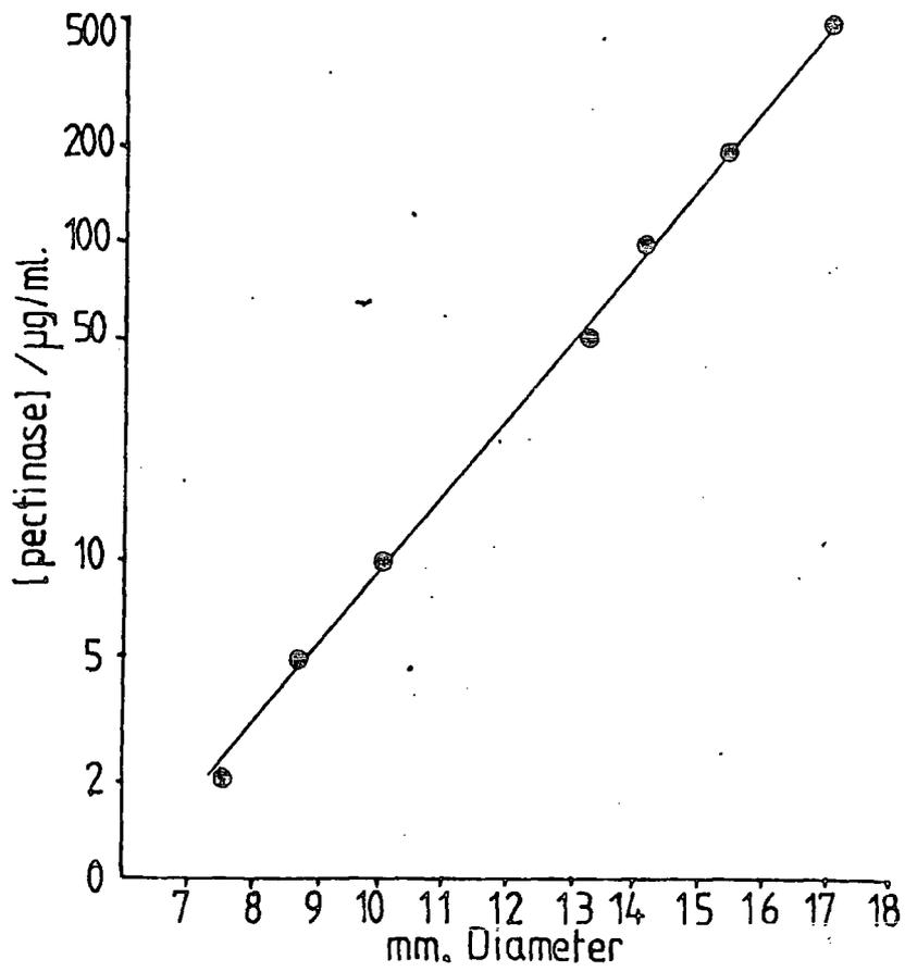
Figure 5.9: Standard curve for pectinase assay. Standard errors are denoted by a bar.
