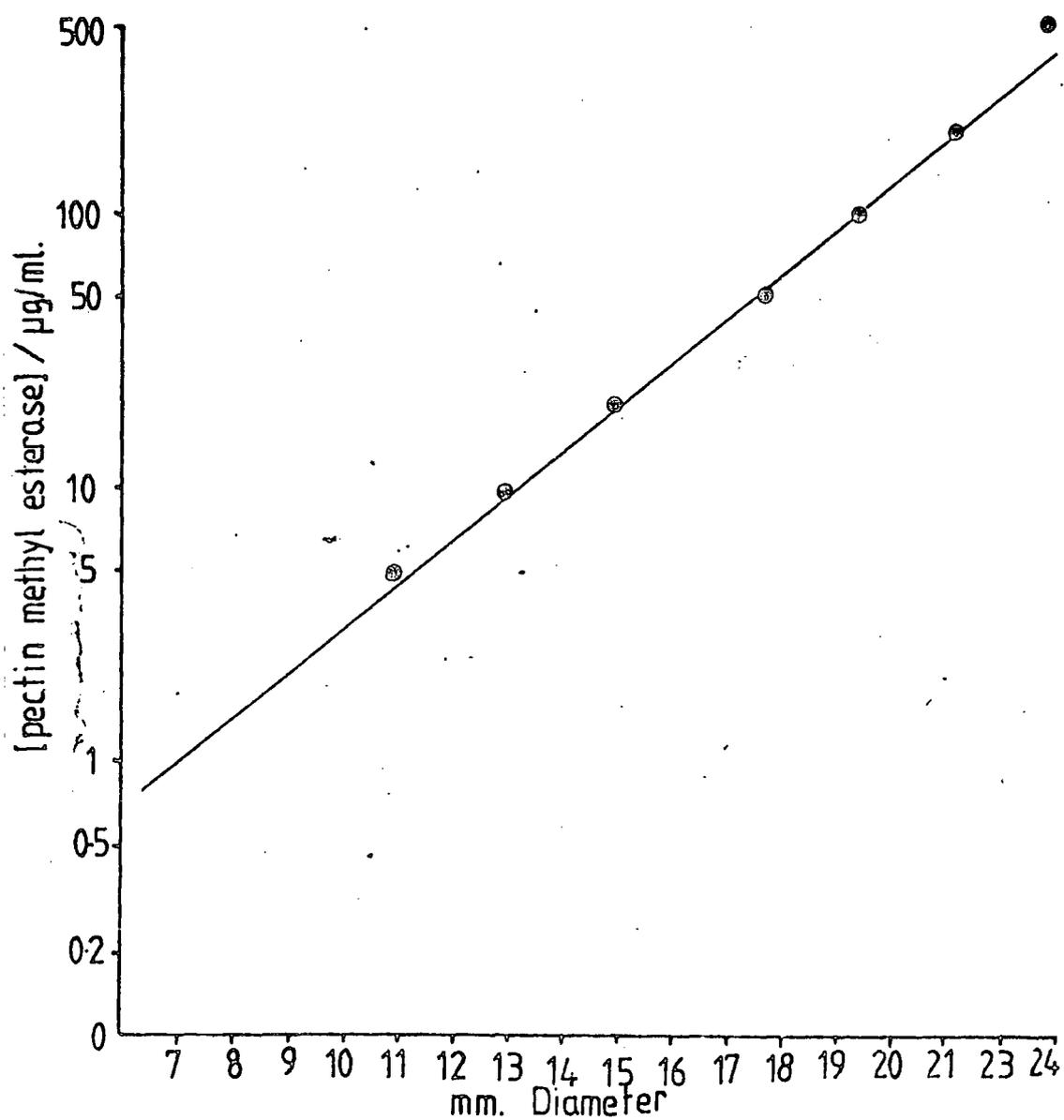
Figure 5.8: Standard curve for pectin methyl esterase. Standard errors are denoted by a bar.
