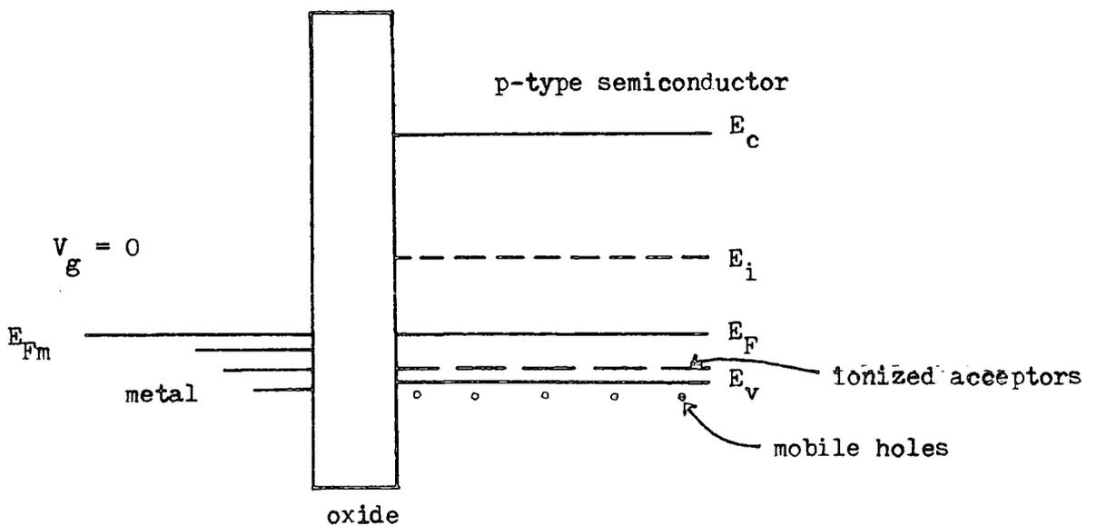
Fig. 2.2 : Ideal energy band diagram at  $V_g = 0$ .
