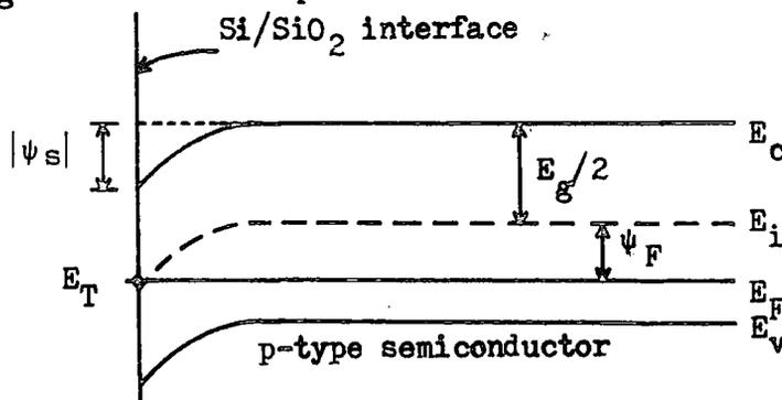
Fig 2.9 : Position of a single discrete interface-state level within the band gap as a function of surface potential.
