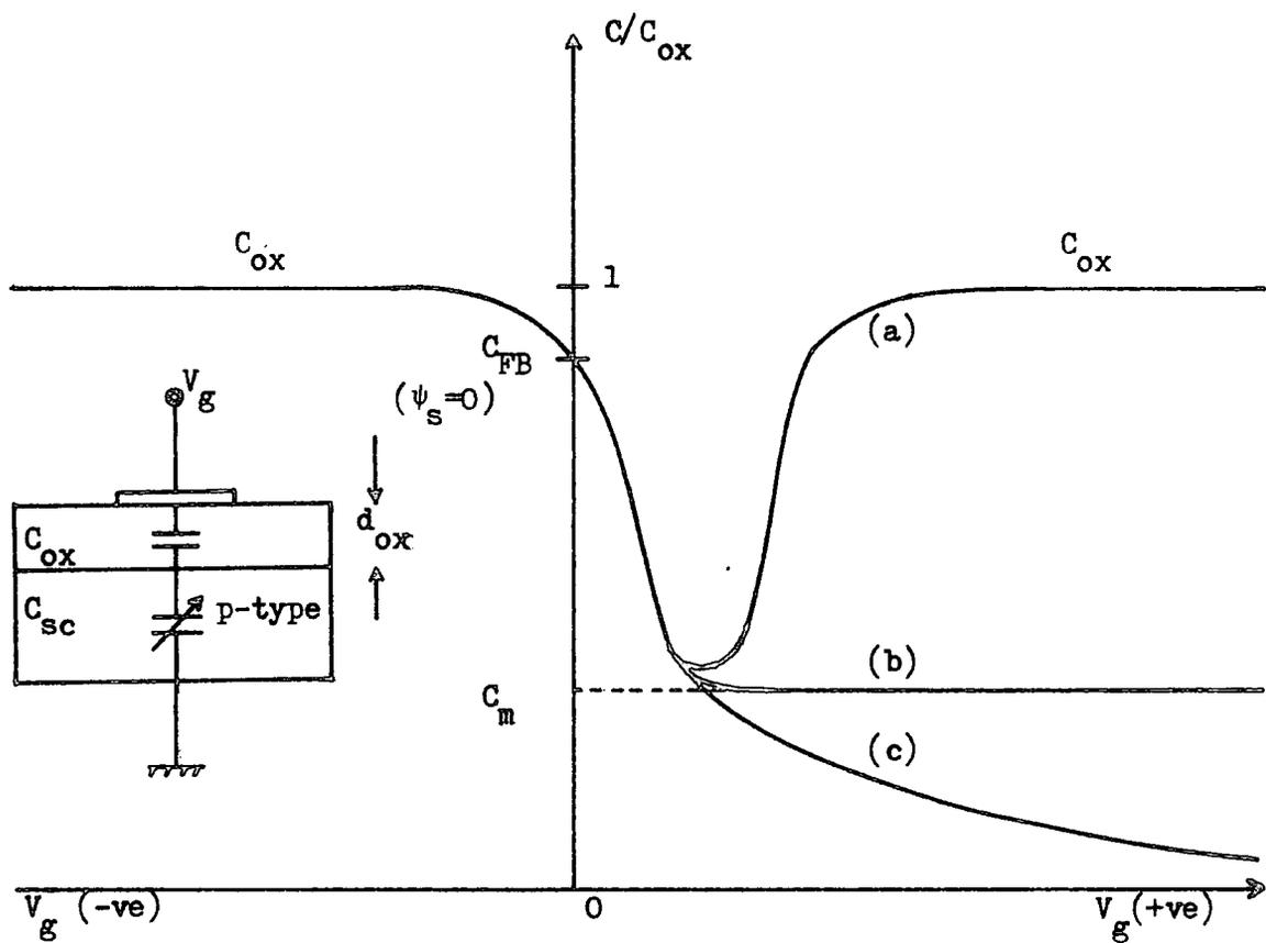
Fig 2.5 : Ideal MOS Capacitance-voltage curves (30)
