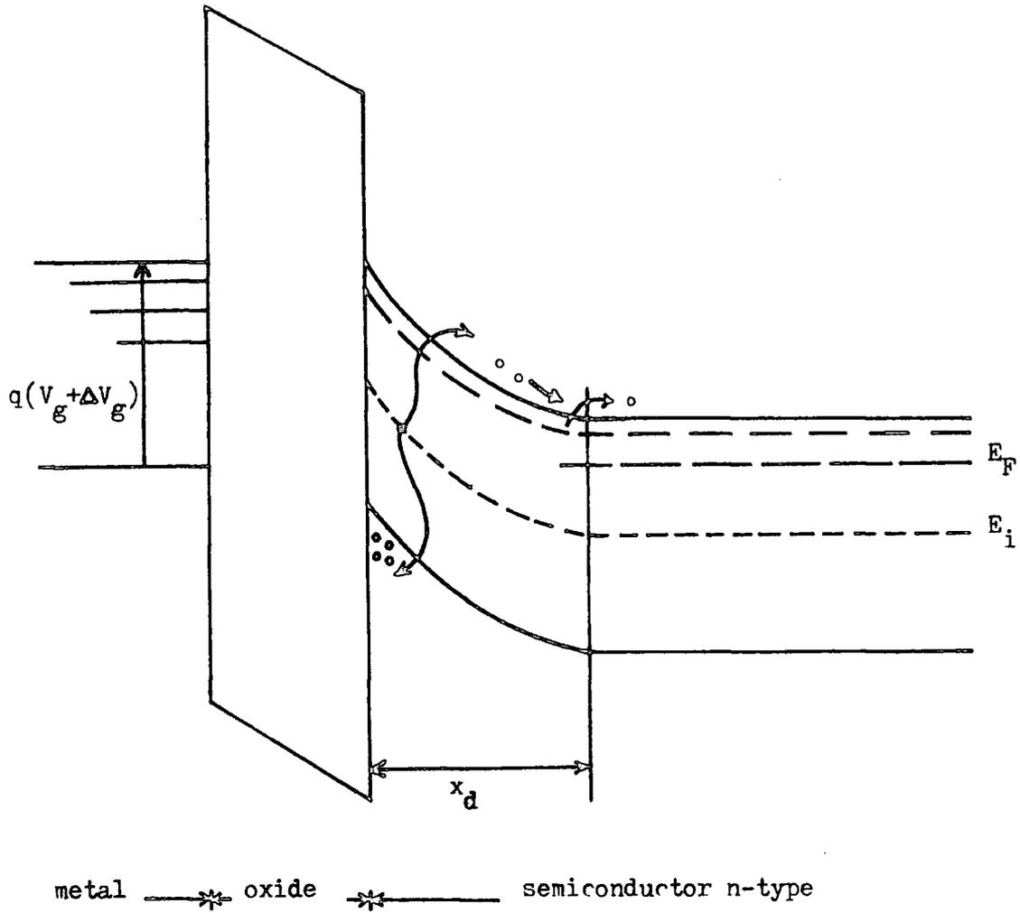
Fig 4.1 : Relaxation of depletion region due to generation of electron-hole pairs in the depletion region of an MOS capacitor.
