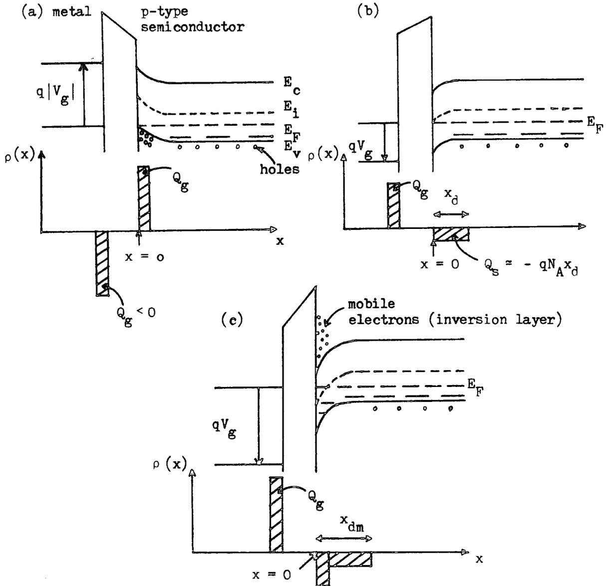
Fig 2.3 : Energy band diagram and charge distribution in an MOS structure upon applying external bias.
