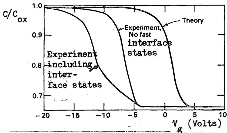
Fig 2.7 : The effect of interface-states on the h.f. capacitance-voltage characteristics of an MOS capacitor.
