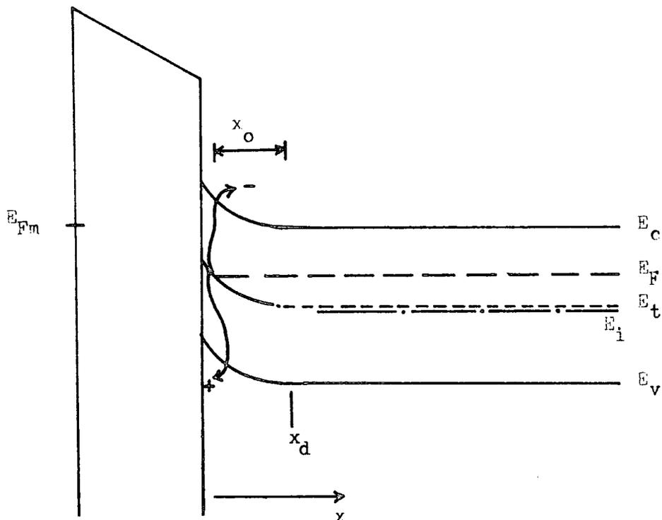
Fig 3.1 : Band diagram of n-type MOS structure with a discrete bulk trap at energy  $E_t$  biased into inversion.
