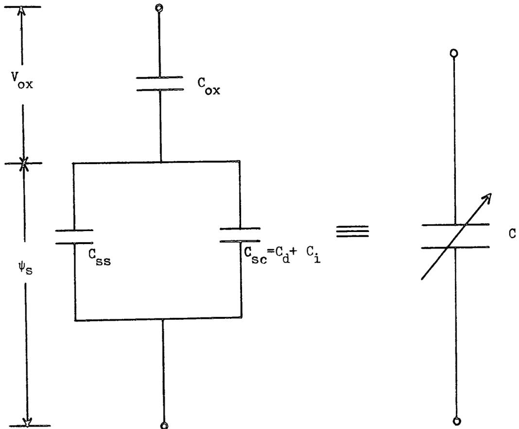
Fig 2.8 : Simplified equivalent circuit of the MOS capacitor showing the capacitance due to interface-states,  $C_{ss}$ .
