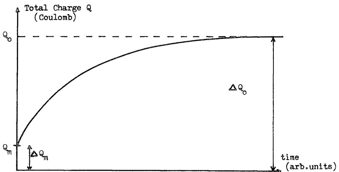
Fig. 4.3 : Schematic diagram of the transient characteristic of the total charge in an MOS capacitor after a small depleting voltage step.
