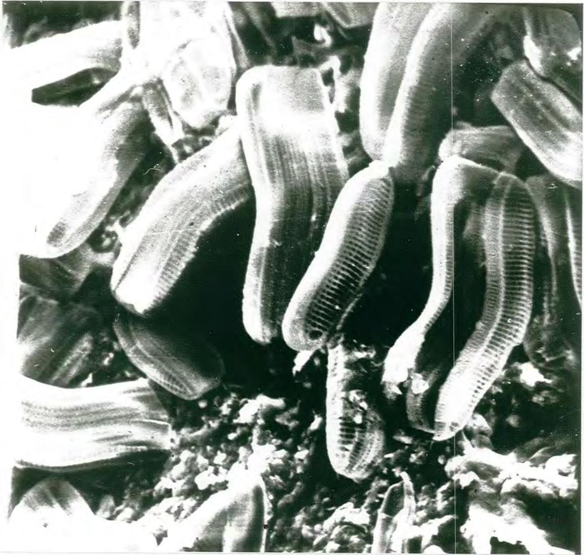
Figure 1.1 Diatom colony on hull surface.
