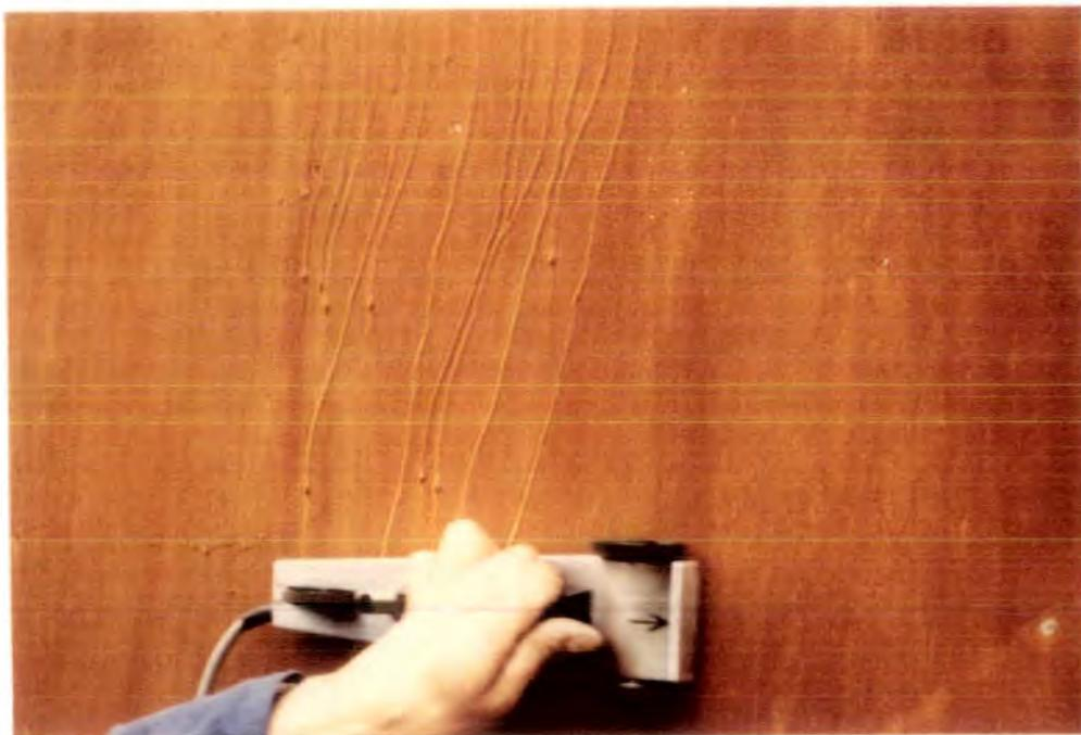
Figure 1.19 B.S.R.A. Roughness Gauge in use
