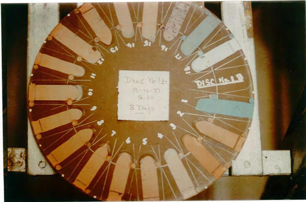
Figure 4.3 A Camrex Disc after sea water Trials
