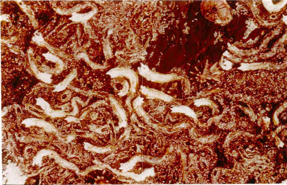
Figure 1.9 Typical calcareous growth resulting from tube-worm fouling
