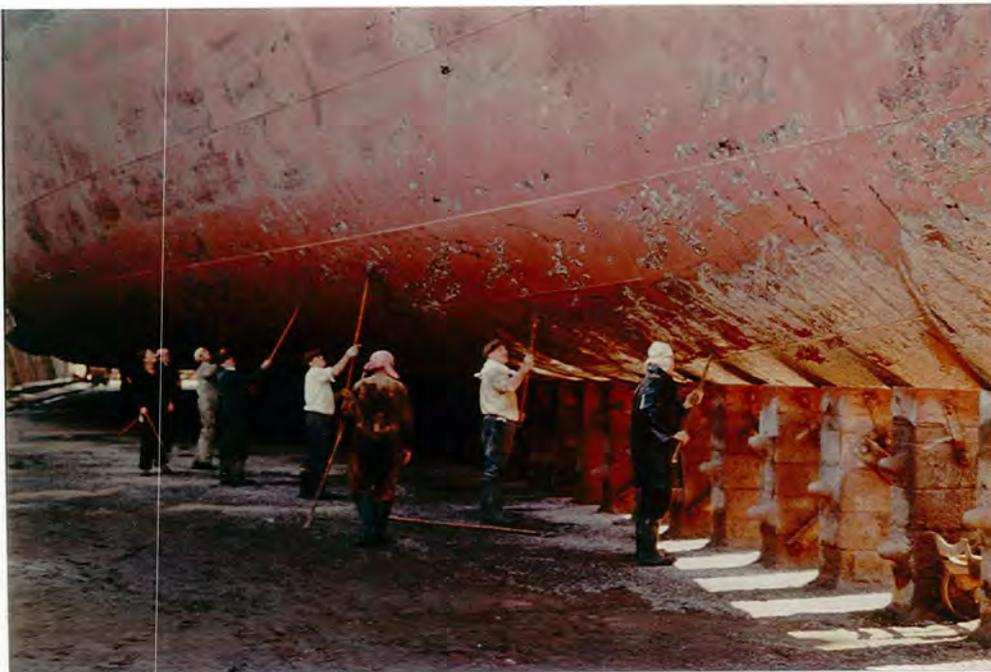
Figure 1.23 Removal of fouling using scrapers
