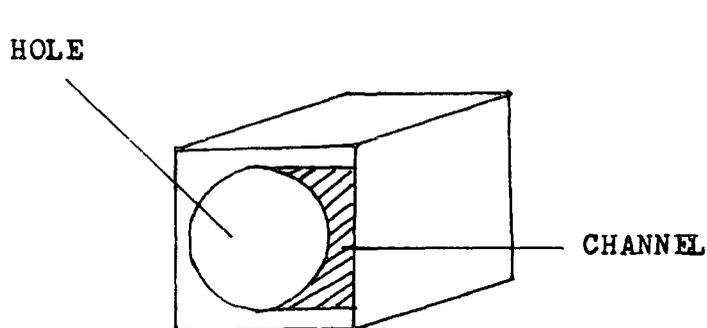
With the block standing on the front face, the hole is filled with lacquer and then drawn down the polyethylene sheet in the opposite direction to the channel, thus, leaving a film of lacquer of given width and depth. By measuring the width after cure, one can assess the spreading of the film (if any) by comparison with the width of the channel and, if necessary, calculate the resulting change in depth.
