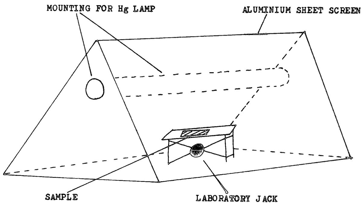
lamp. In the work carried out, the distance was maintained constant at 18cm and the lamp output was unfiltered, the only variables being the time of irradiation and the age of the lamp.
