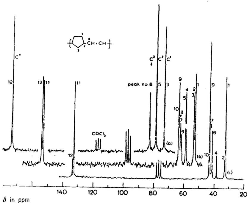
Fig. 4.2.  $^{13}\text{C}$  nmr spectra of three samples (a), (b), (c) of poly(1,3-cyclopentylene vinylene) in  $\text{CDCl}_3$ . Polymers prepared using (a)  $\text{ReCl}_5$ , (b)  $\text{WCl}_6/\text{C}_2\text{H}_5\text{AlCl}_2$ , (c) ruthenium complex, as initiators. The scale refers to spectrum (c). Spectra (b) and (a) are offset by 20 p.p.m. and 40 p.p.m., respectively.
