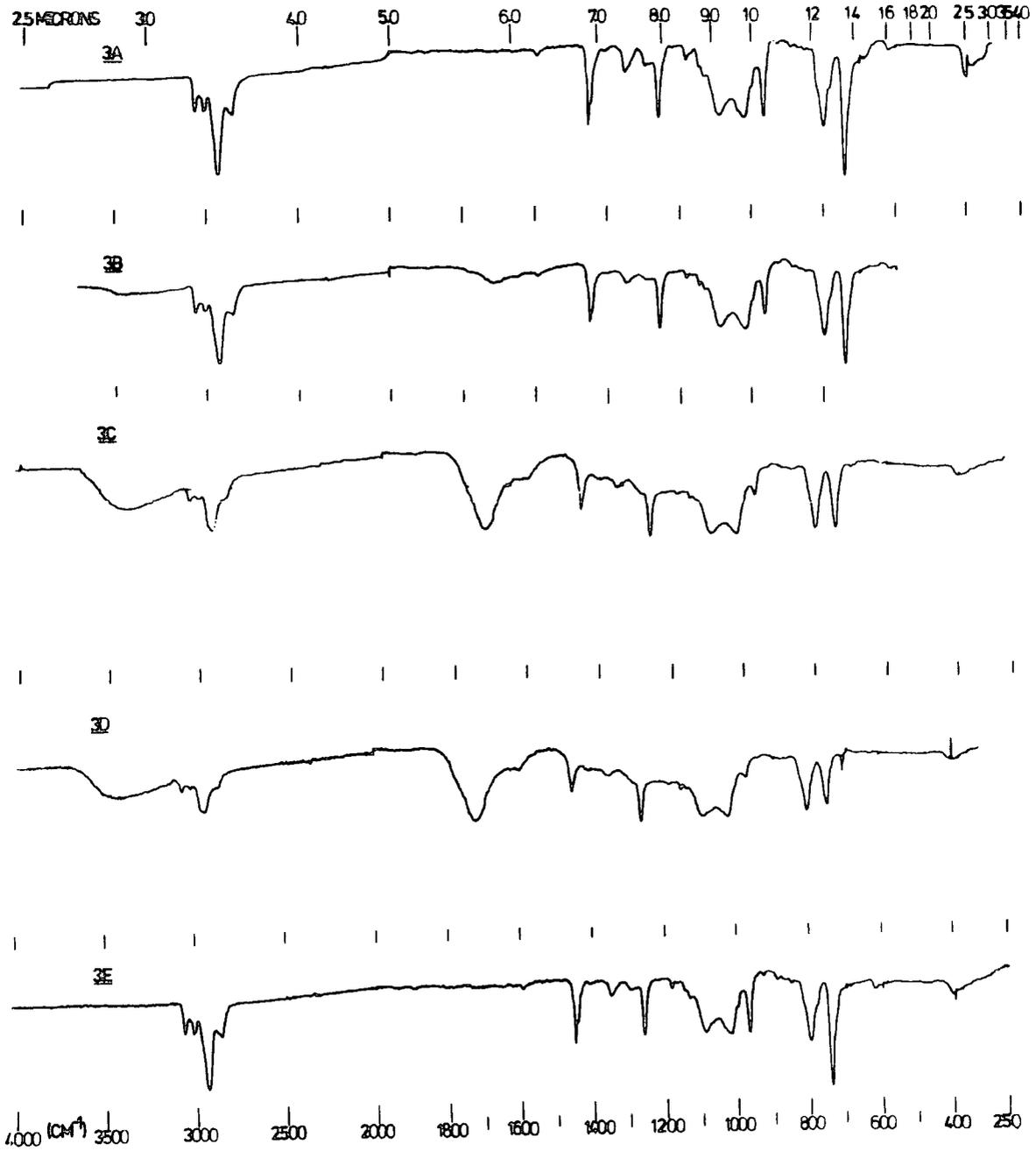
Figure 4.12. I.R. spectra of poly(19-12), film no. 4 exposed to light and air
