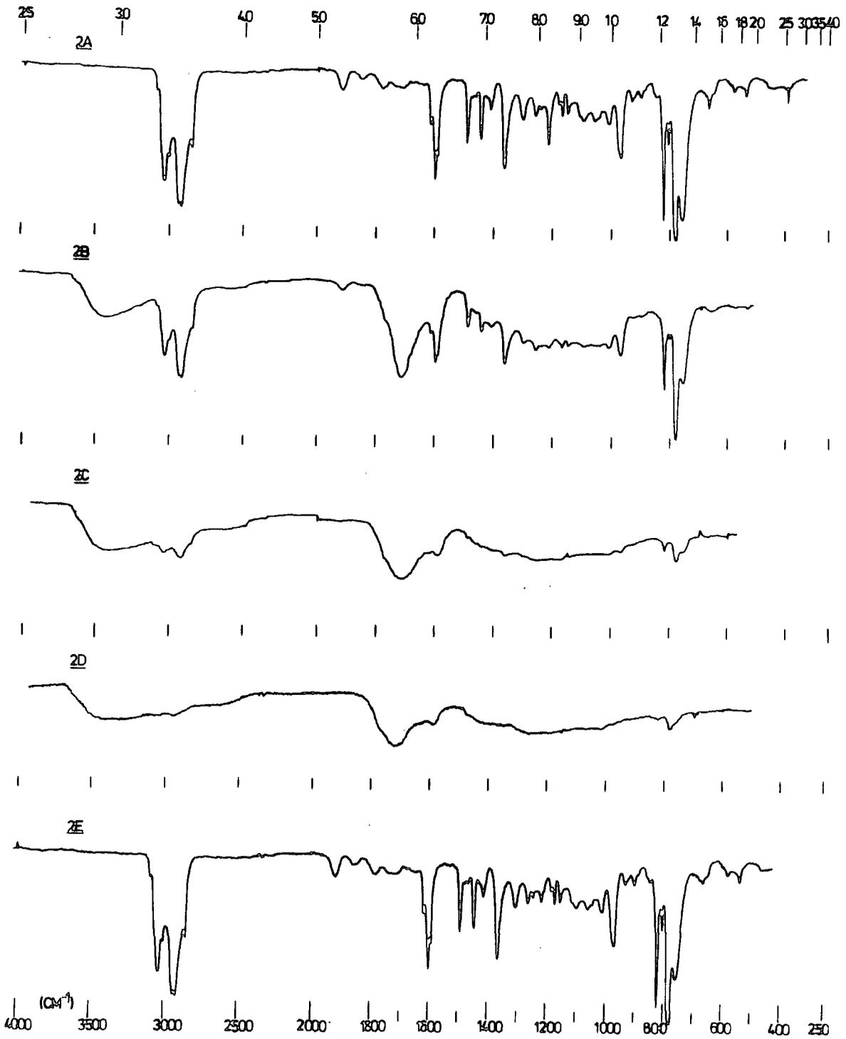
Figure 4.10. I.R. spectra of poly(15-2), film no. 5 exposed to light and air
