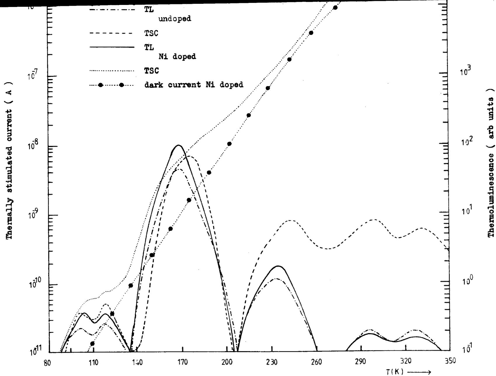
Figure 9.9.2 TSC and TL spectra for the  $\text{TiO}_2.\text{Ni}$  crystal NI(NL) before and after nickel diffusion.
