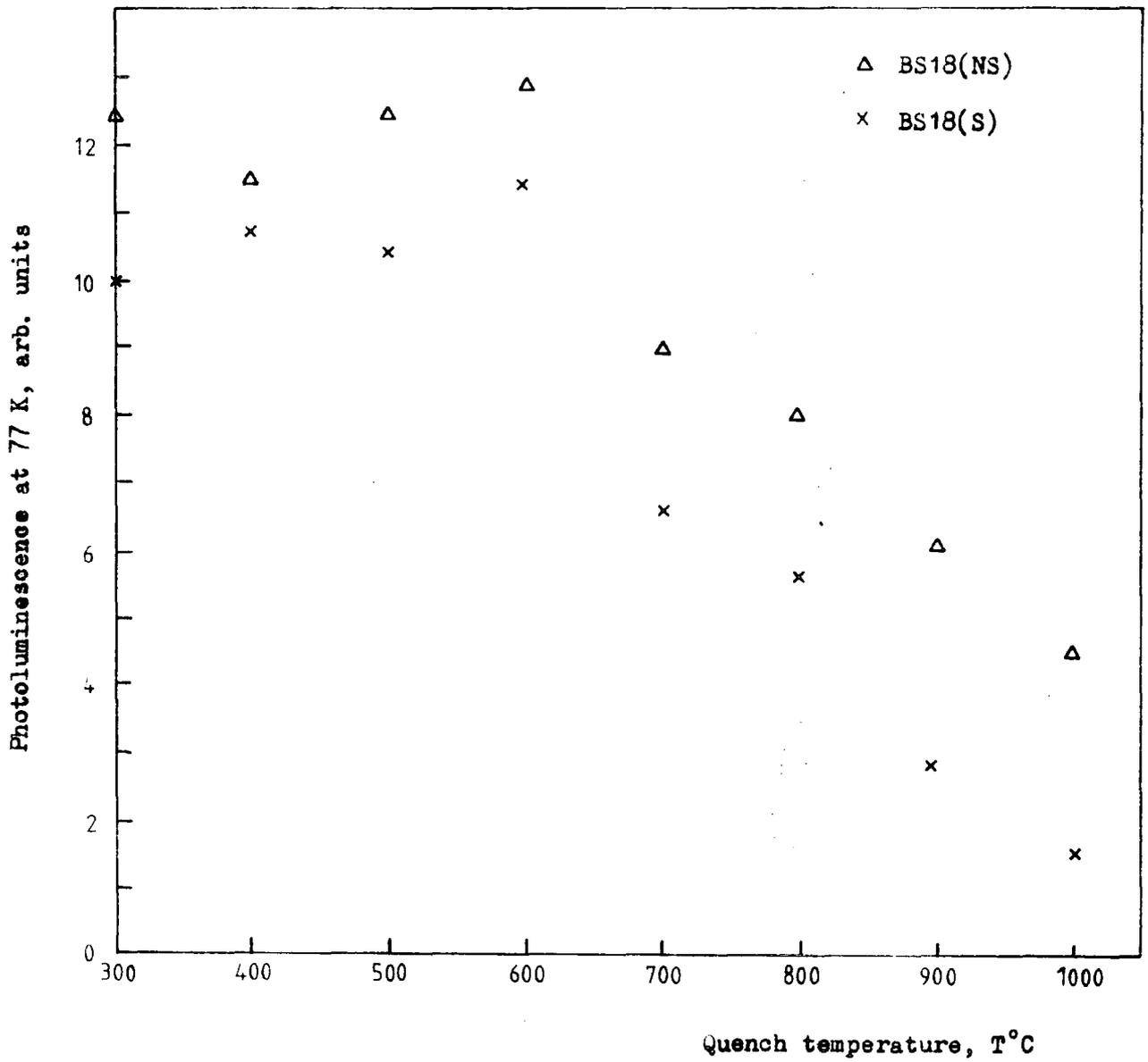
Figure 6.7.1 The photoluminescence intensity in the non-stoichiometric as grown crystal BS18(NS) and the stoichiometric as grown crystal BS18(S) after quenching from a temperature T°C.
