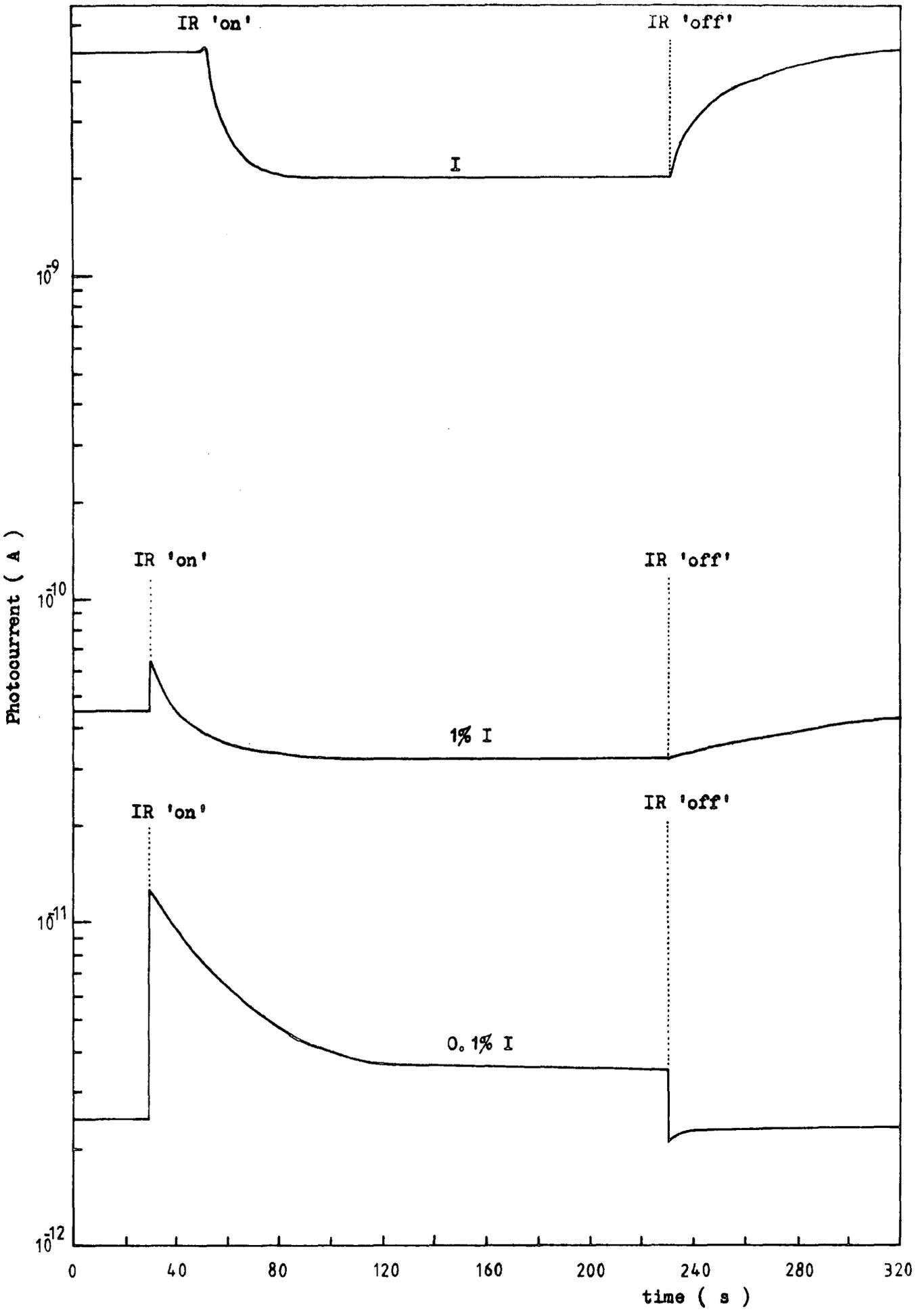
Figure 5.6.3 Photoconductivity quenching and stimulation due to infra red light as a function of 400 nm light intensity at 77 K for a quenched CA<sub>3</sub>(NL) crystal .
