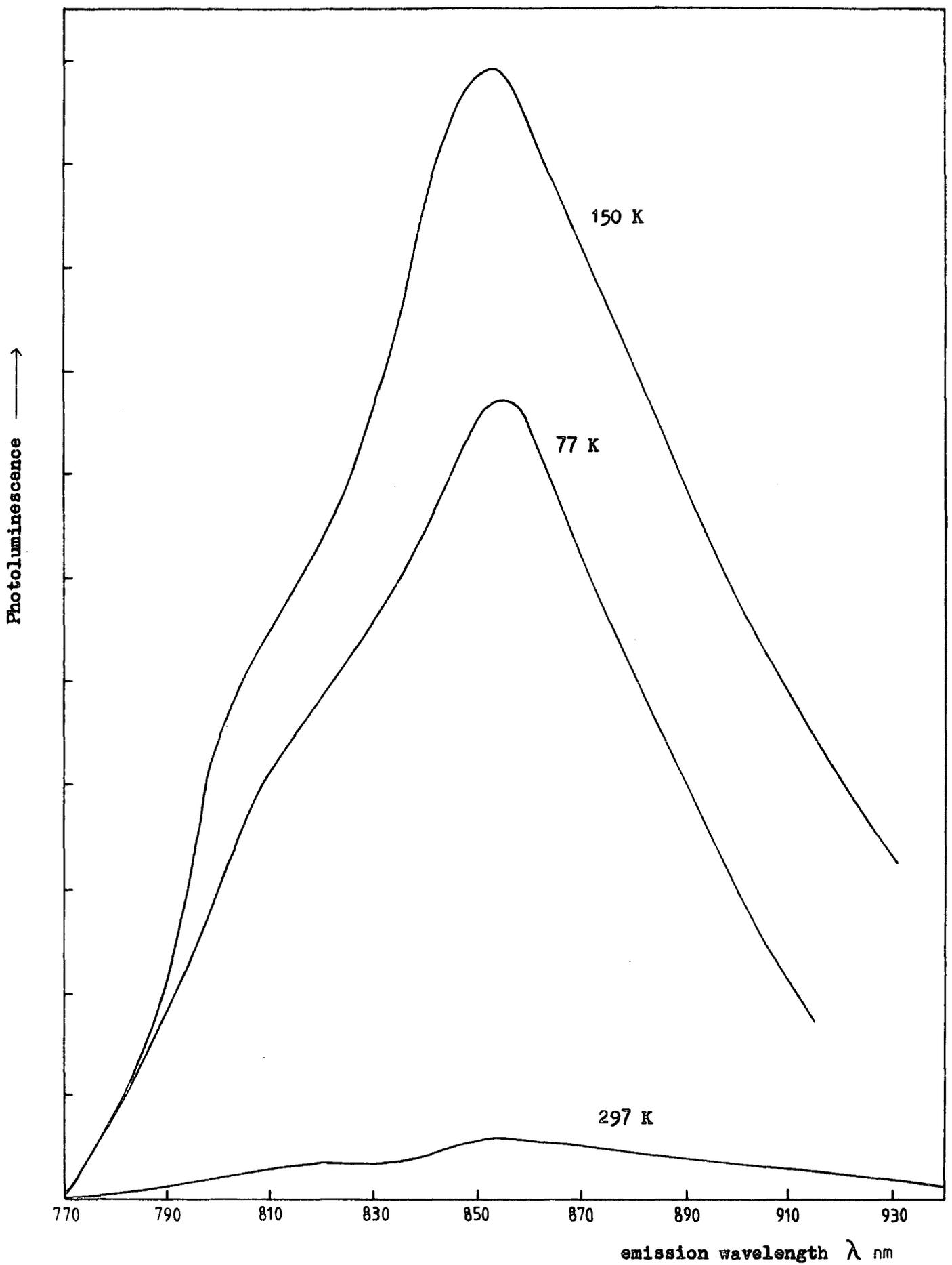
Figure 6.2.3 The temperature dependence of the photoluminescence emission spectrum for the crystal CA<sub>3</sub>(NL).
