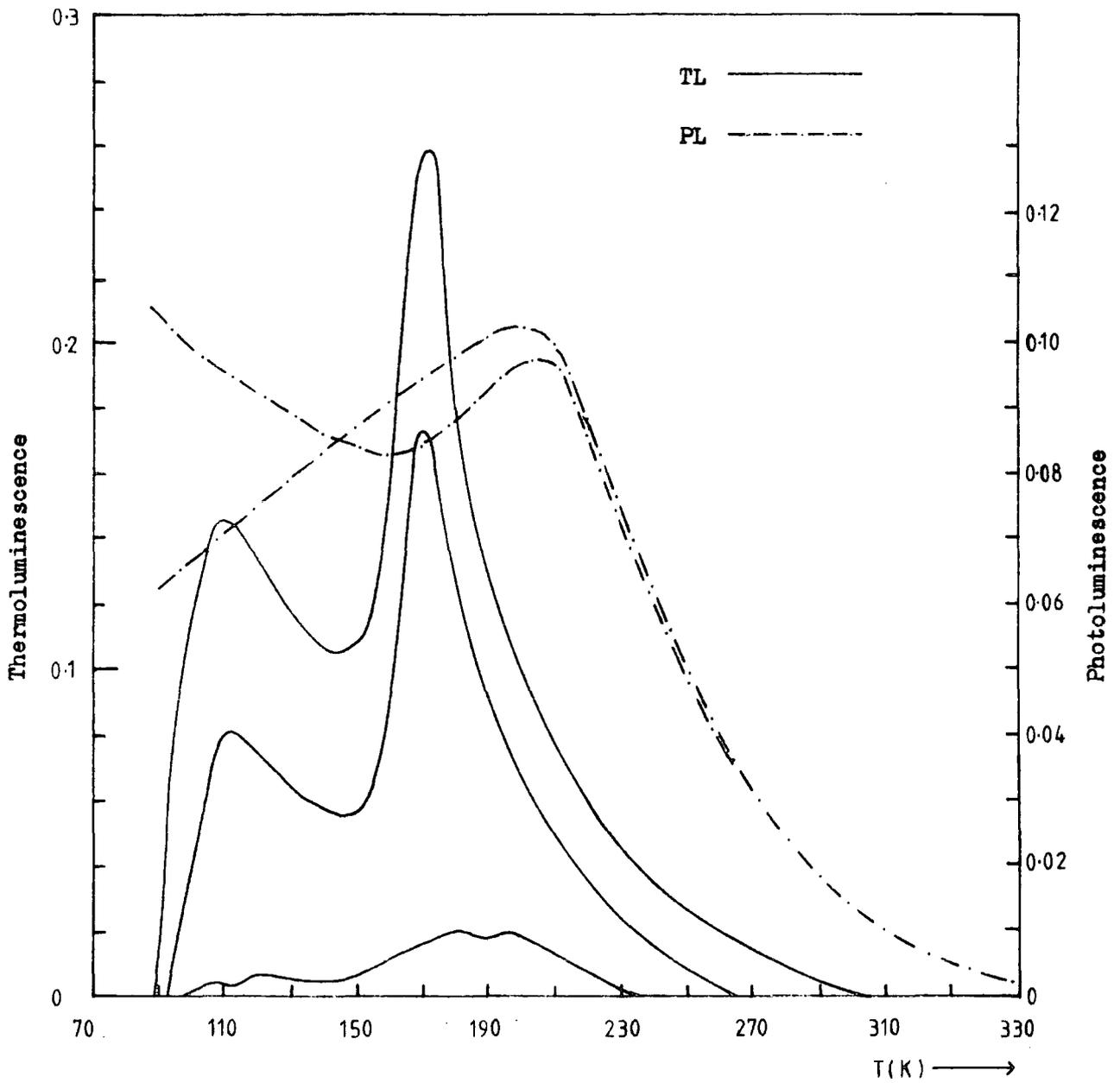
Figure 10.2.1 Photoluminescence and thermoluminescence spectra for the 'sandy' rutile powder DN5 (a) as-prepared (b) quenched from 500°C (c) quenched from 1000°C.
