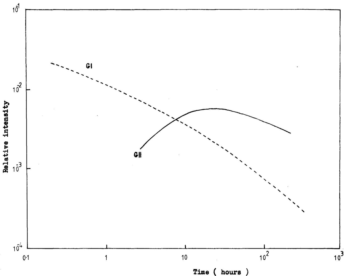
Figure 9.12.1 The change of the ESR absorption intensity for GII compared with the substitutional  $\text{Co}^{2+}$  line as a function of the times of annealing ( oxidation ) for the sample which was reduced in the vacuum of  $10^{-2} \sim 10^{-3}$  torr at  $800^\circ\text{C}$  for 30 minutes ( after Miyako 1971 ) .
