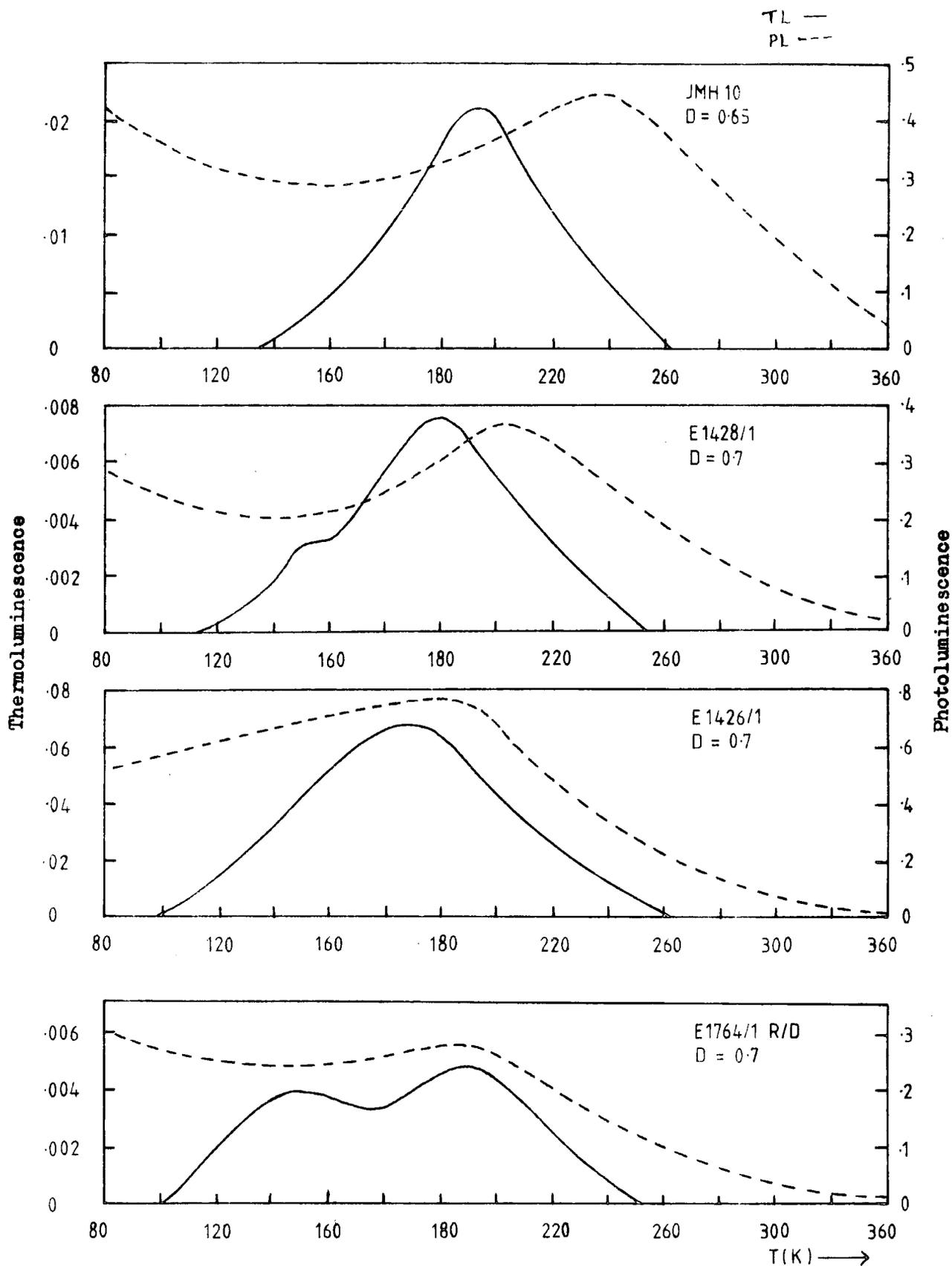
Figure 10.5.1 TL and PL spectra for the four rutile pigments JMH10, E1428/1, E1426/1 and E1764/1 R/D .
