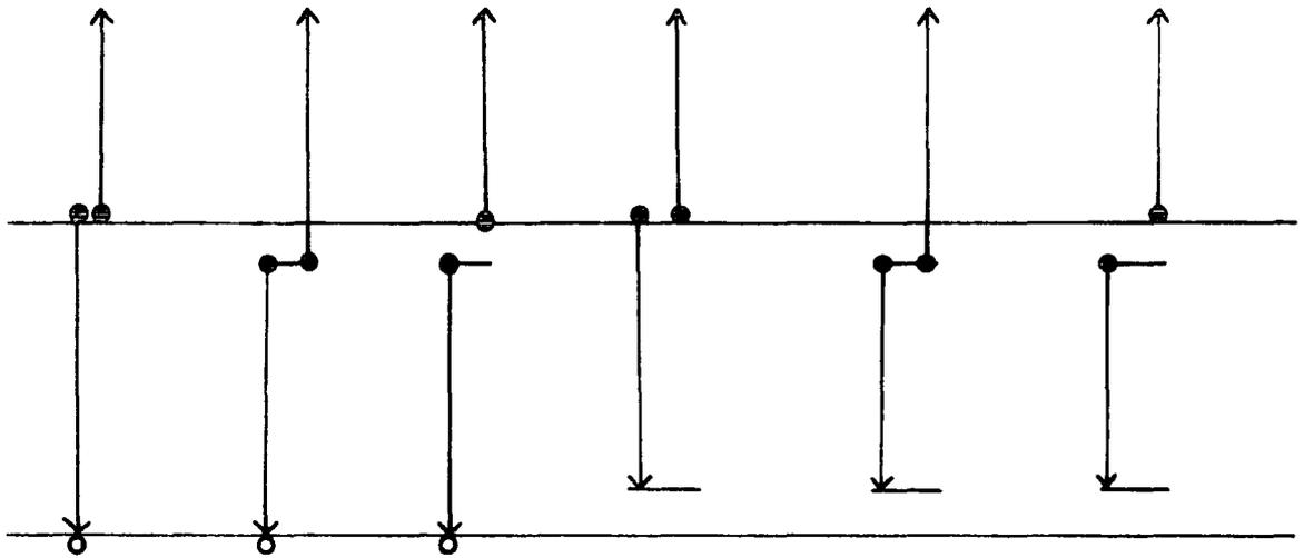
Figure 6.6.6 Diagram of some Auger processes in a n-type semiconductor.
