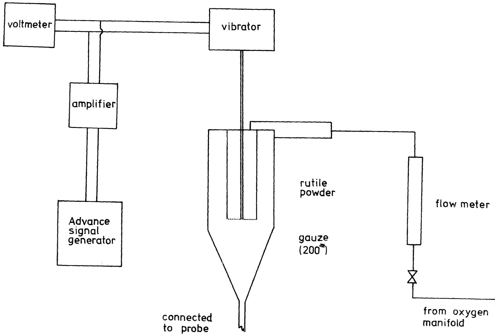
Figure 3.3 Schematic of the hopper feed system
