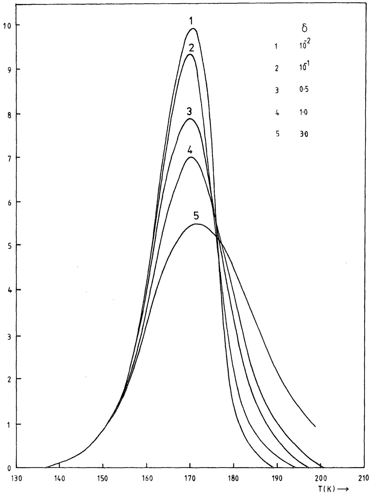
Figure 8.4.3 Variation of TSL with the retrapping ratio  $\delta$ .
