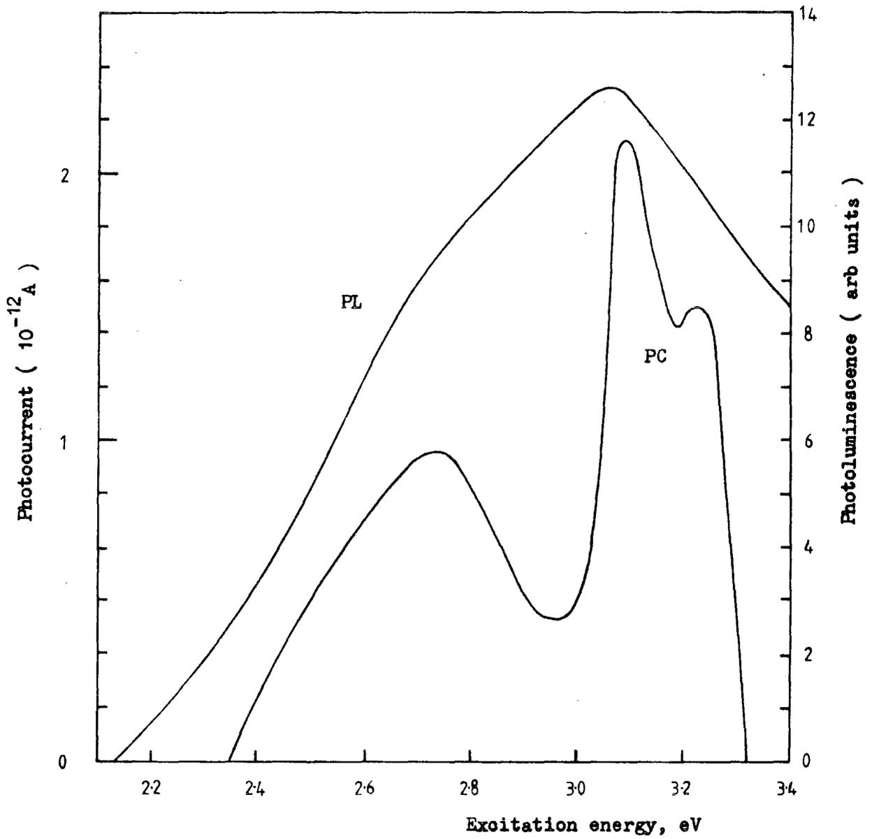
Figure 9.11.1 PC spectral response and PL excitation spectrum for cobalt doped crystal CO(NL) at 77K ( after spectral correction ).
