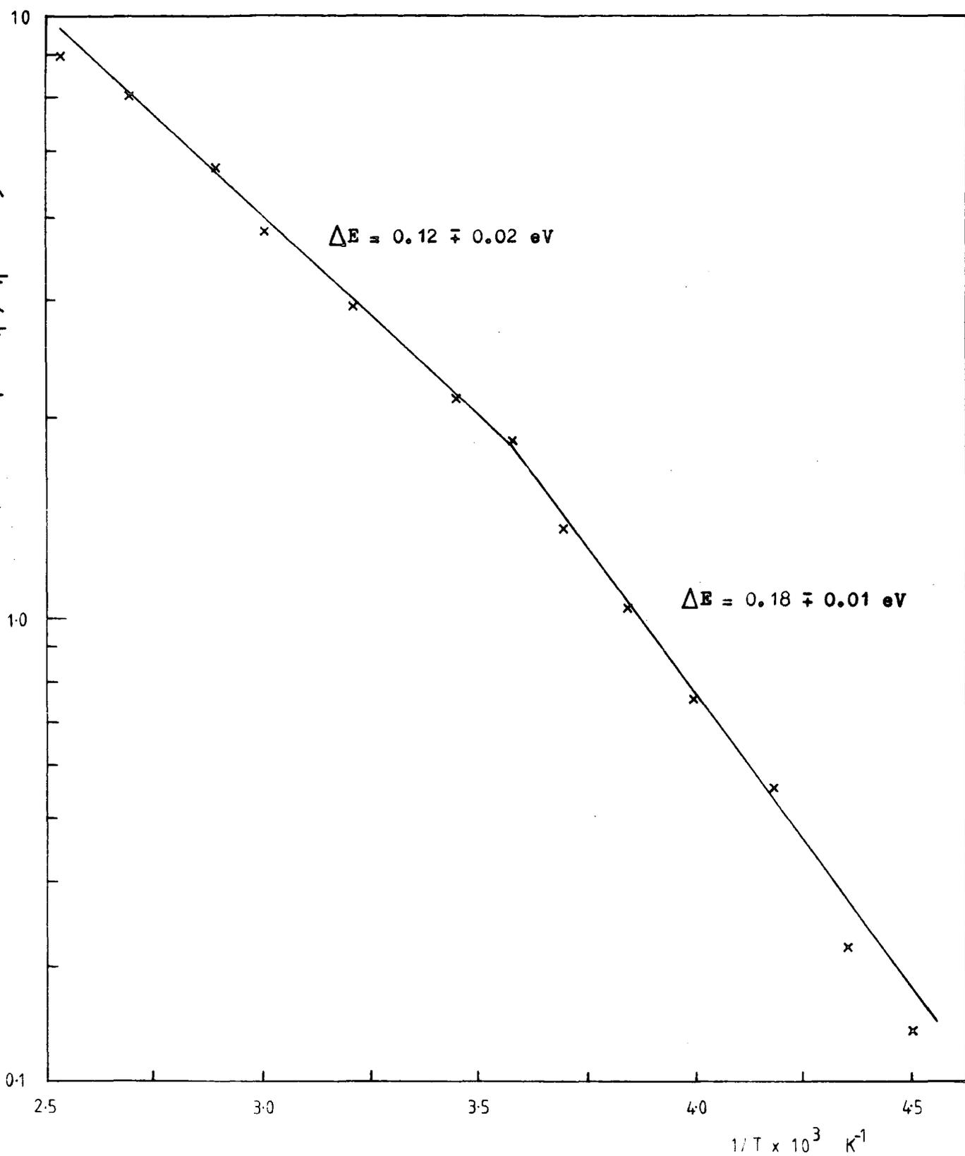
Figure 6.6.2 Activation energy plot for the thermal quenching of photoluminescence in the crystal CA<sub>3</sub>(NL).
