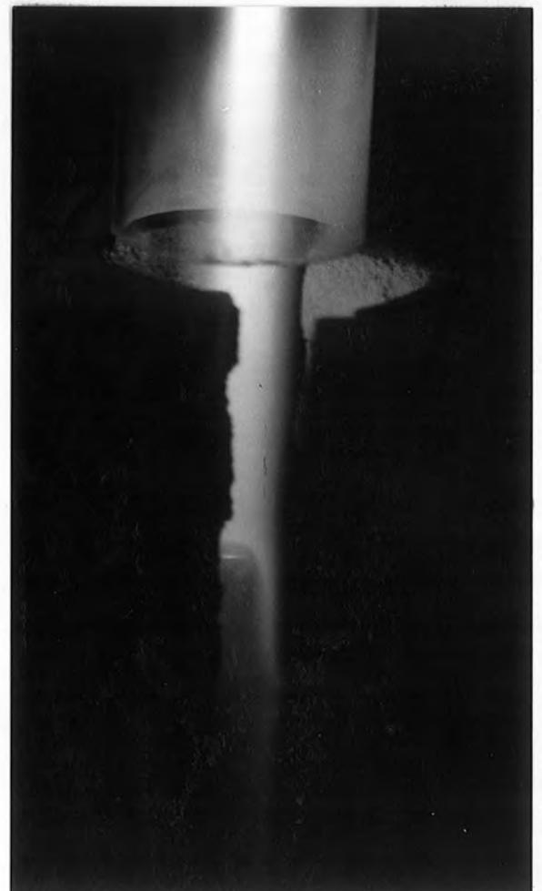
to provide a constant flow of feed material to the probe. A flow of 1 litre/min was used for the growth of single crystal rutile.
