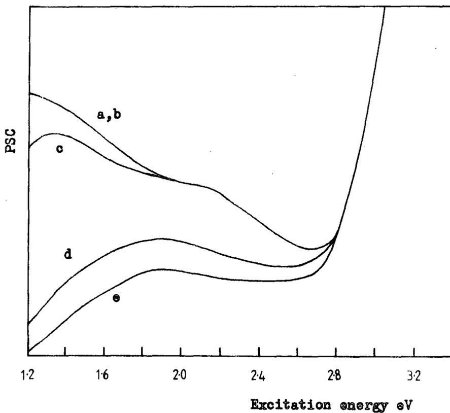
Figure 9.5.2 PSC spectra for crystal C1(NL) after chromium doping
