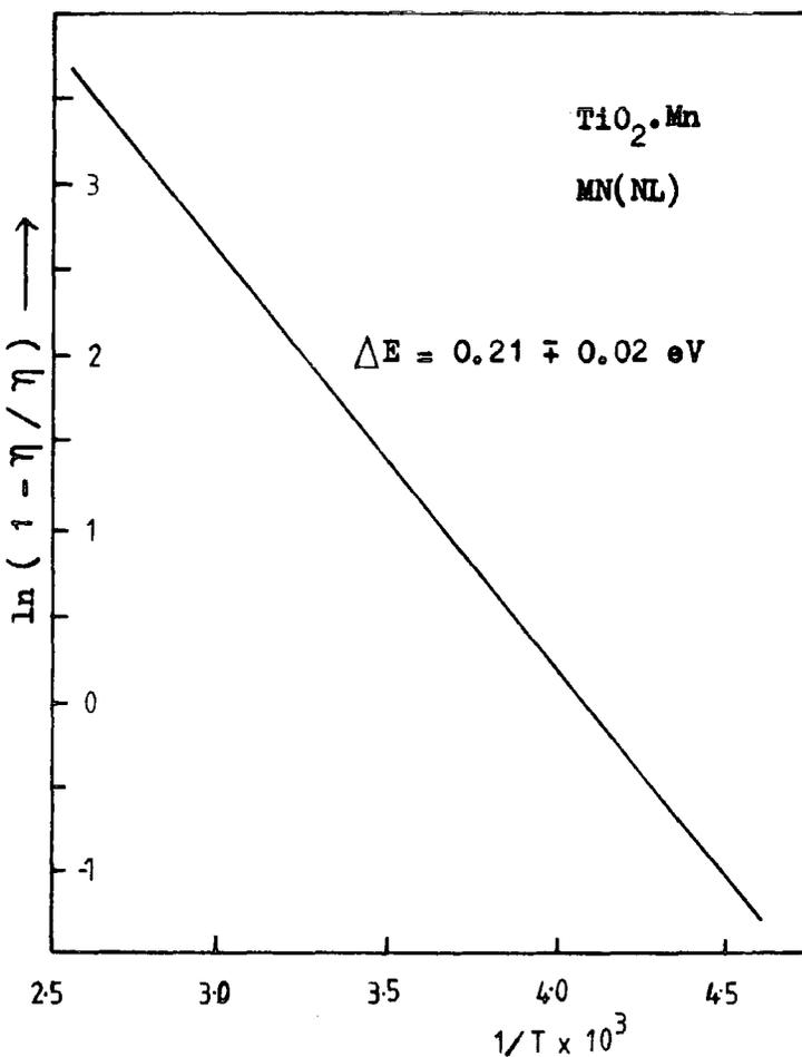
Figure 9.2.8 The temperature dependence of the photoluminescence emission intensity for the crystals NI(NL) and MN(NL).
