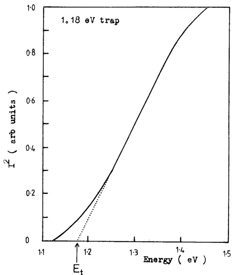
Figure 5.9.2  $I^2$  versus E plot for the 1.18 eV trap in crystal CA3(NL).
