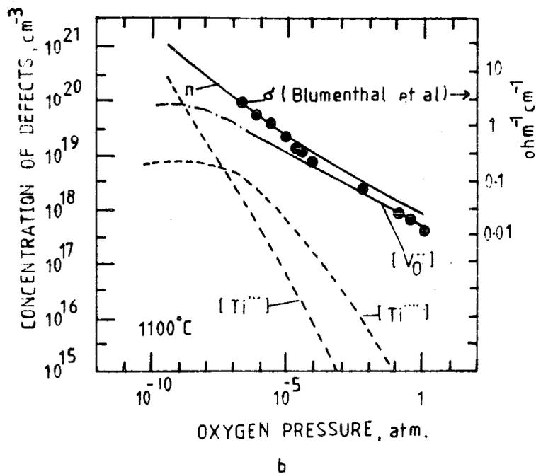
Figure 1.5.1 The concentrations of point defects and electrons in  $\text{TiO}_{2-x}$  as a function of the partial pressure of oxygen ( After Kofstad 1972). Results of electrical conductivity after Blumenthal et al (1966) (a)  $1500^\circ\text{C}$  (b)  $1100^\circ\text{C}$ .
