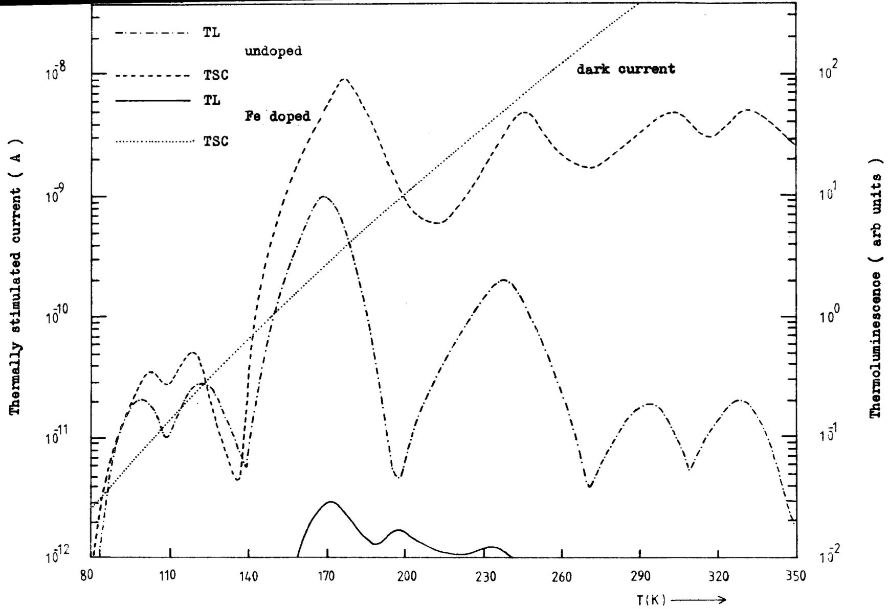
Figure 9.7.1 Comparison of the TSC and TL spectra for crystal FE(NL) before and after Fe doping .
