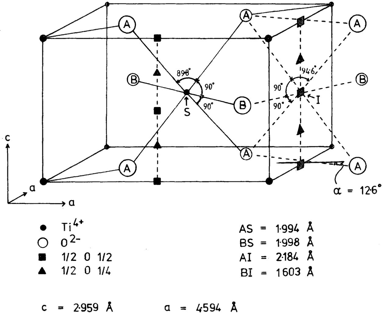
Figure 1.2.1 Crystal structure of rutile showing a unit cell and some  $\frac{1}{2}0\frac{1}{2}$  (■) and  $\frac{1}{2}0\frac{1}{4}$  (▲) type interstitial sites. The positions of the oxygen ions around the octahedrally coordinated substitutional ion S and around the interstitial site I are indicated
