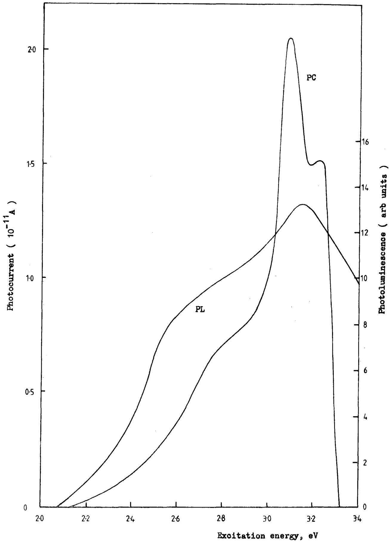
Figure 9.9.1 PC spectral response and PL excitation spectra for the TiO<sub>2</sub>.Ni crystal NI(NL) at 77K .
