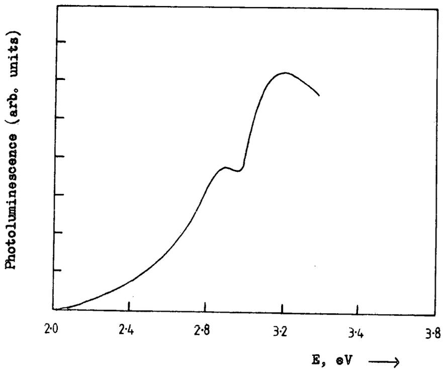
Figure 9.5.3 Photoluminescence excitation spectra for crystal C1(NL) at 77 K ( after spectral correction ).
