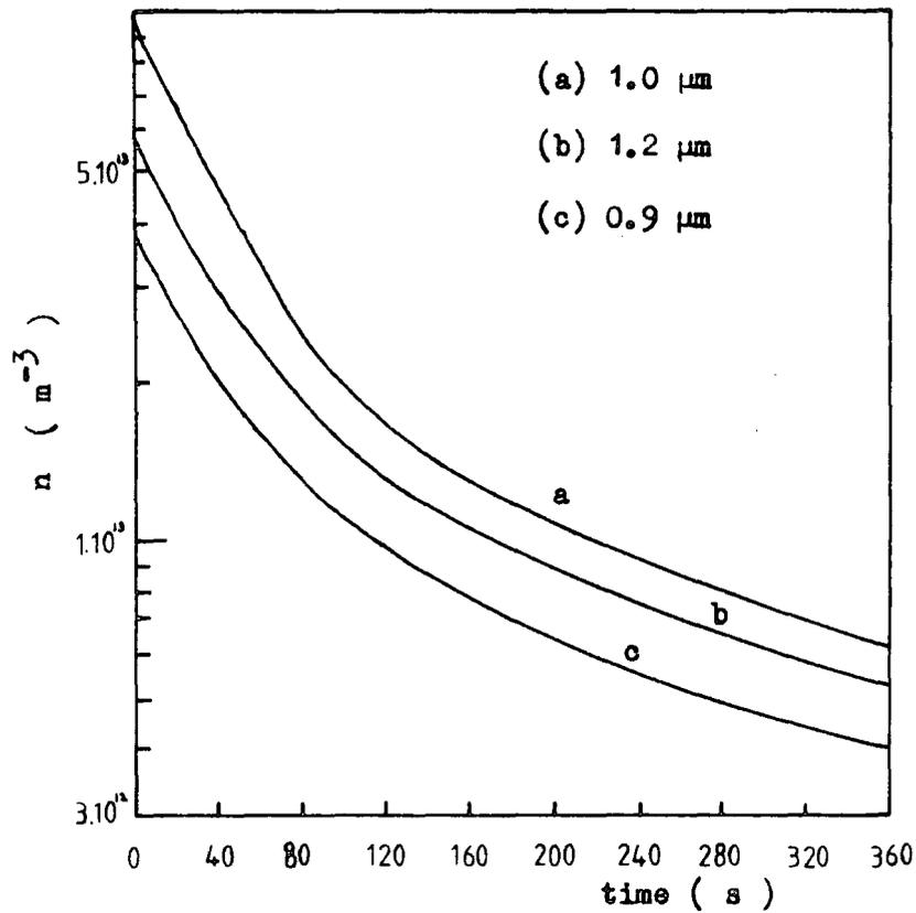
Figure 5.11.2 The emptying of the 0.86 eV trap in crystal CA3(NL) after excitation with light of wavelength  $1.2 \mu\text{m}$ ,  $1.0 \mu\text{m}$  and  $0.9 \mu\text{m}$  .
