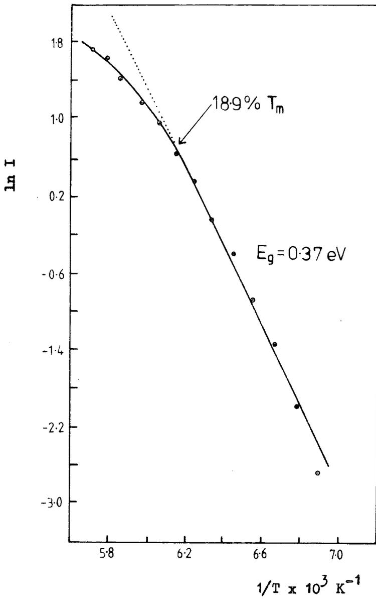
Figure 7.5.3 Garlick and Gibson plot for the NL crystal CA3(NL) .
