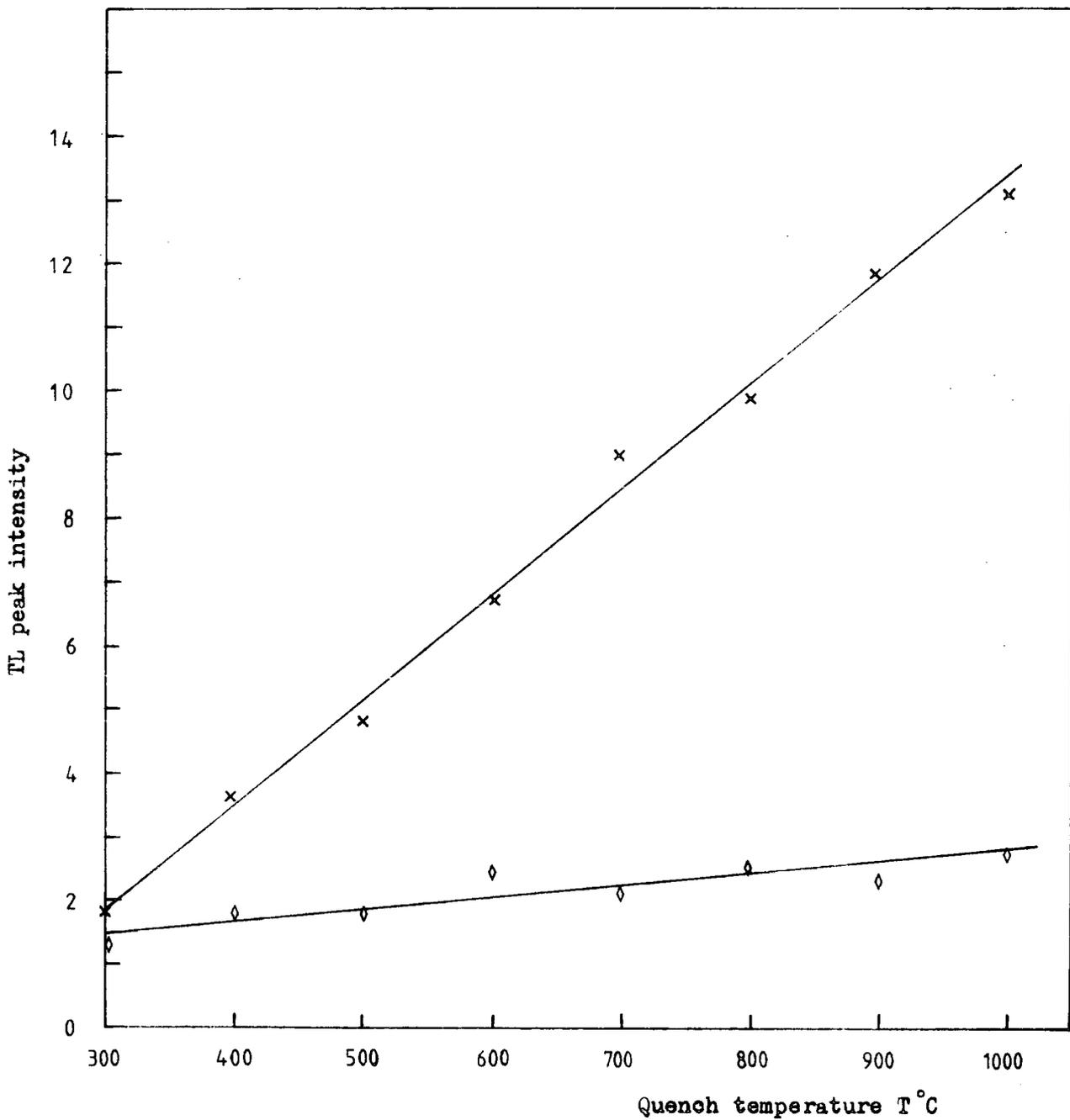
Figure 10.3.4 Variation of the TL peak height for pigment SPF552 after quenching from  $T^{\circ}\text{C}$ .  $\times$  175 K peak  $\diamond$  130 K peak
