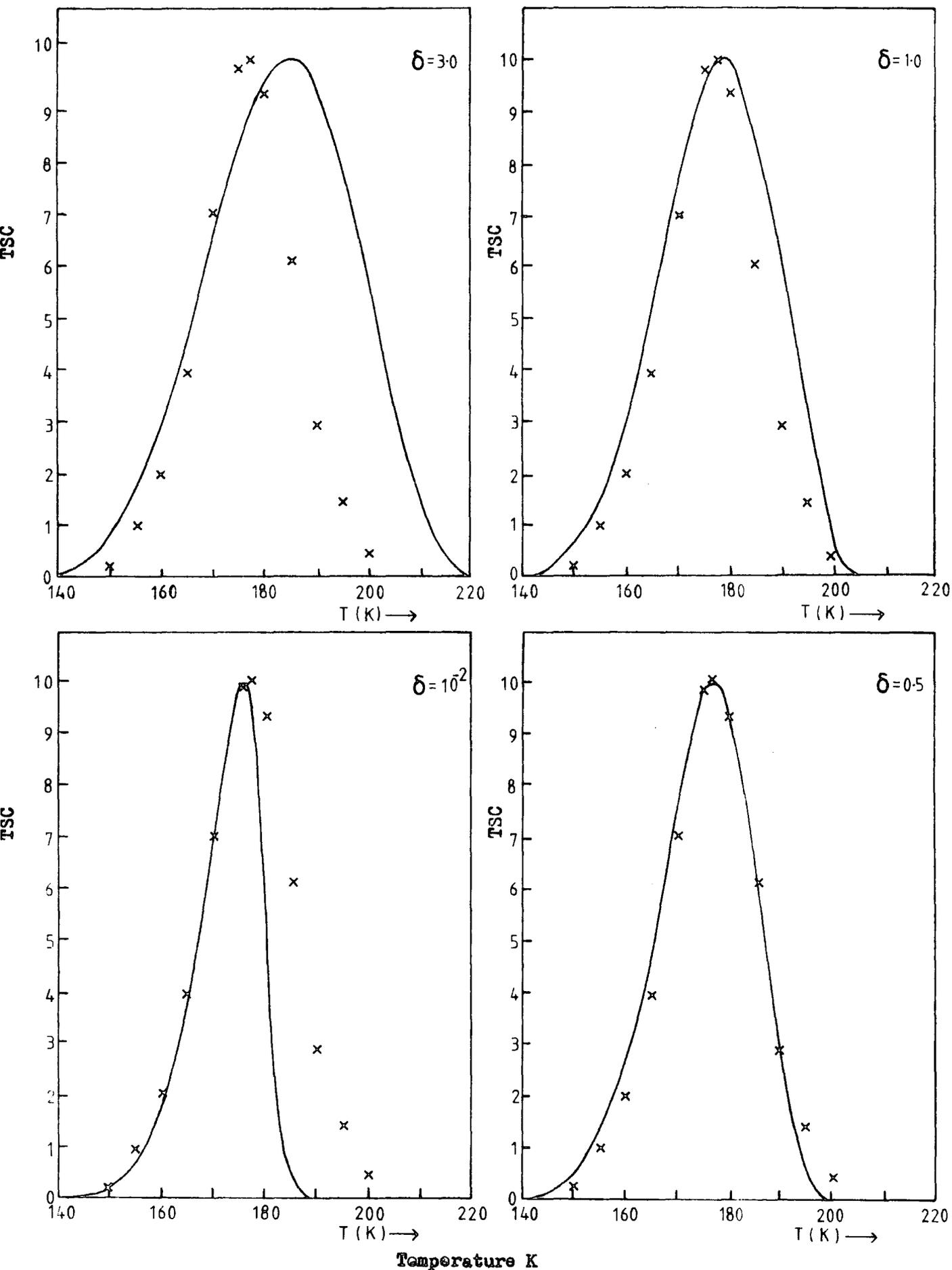
Figure 7.5.2 Comparison of the geometrical shapes of TSC curves for different retrapping ratios.  $E = 0.37 \text{ eV}$ ;  $h_s = 2.0 \cdot 10^{17} \text{ cm}^{-3}$ ;  $h_d = 1.7 \cdot 10^{16} \text{ cm}^{-3}$ ;  $\tau = 10^{-8} \text{ s}$ ;  $\text{FREQ} = 7.39 \cdot 10^9 \text{ s}^{-1}$ ;  $\beta = 0.5 \text{ }^\circ\text{s}^{-1}$ .
