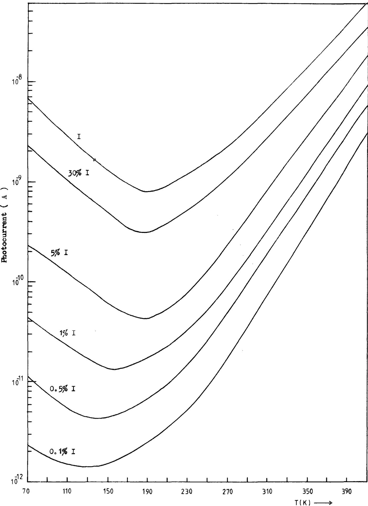
Figure 5.6.4 Temperature dependence of the photoconductivity at various excitation intensities for the quenched CA<sub>3</sub>(NL) crystal.
