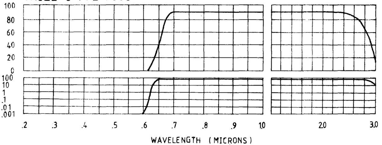
Figure 4.5.3 Spectral transmission of the order sorter filters.
