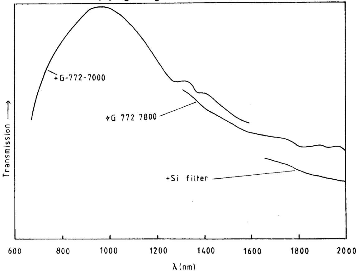
Figure 4.5.2 Throughput of the optical system for the 1  $\mu\text{m}$  grating.
