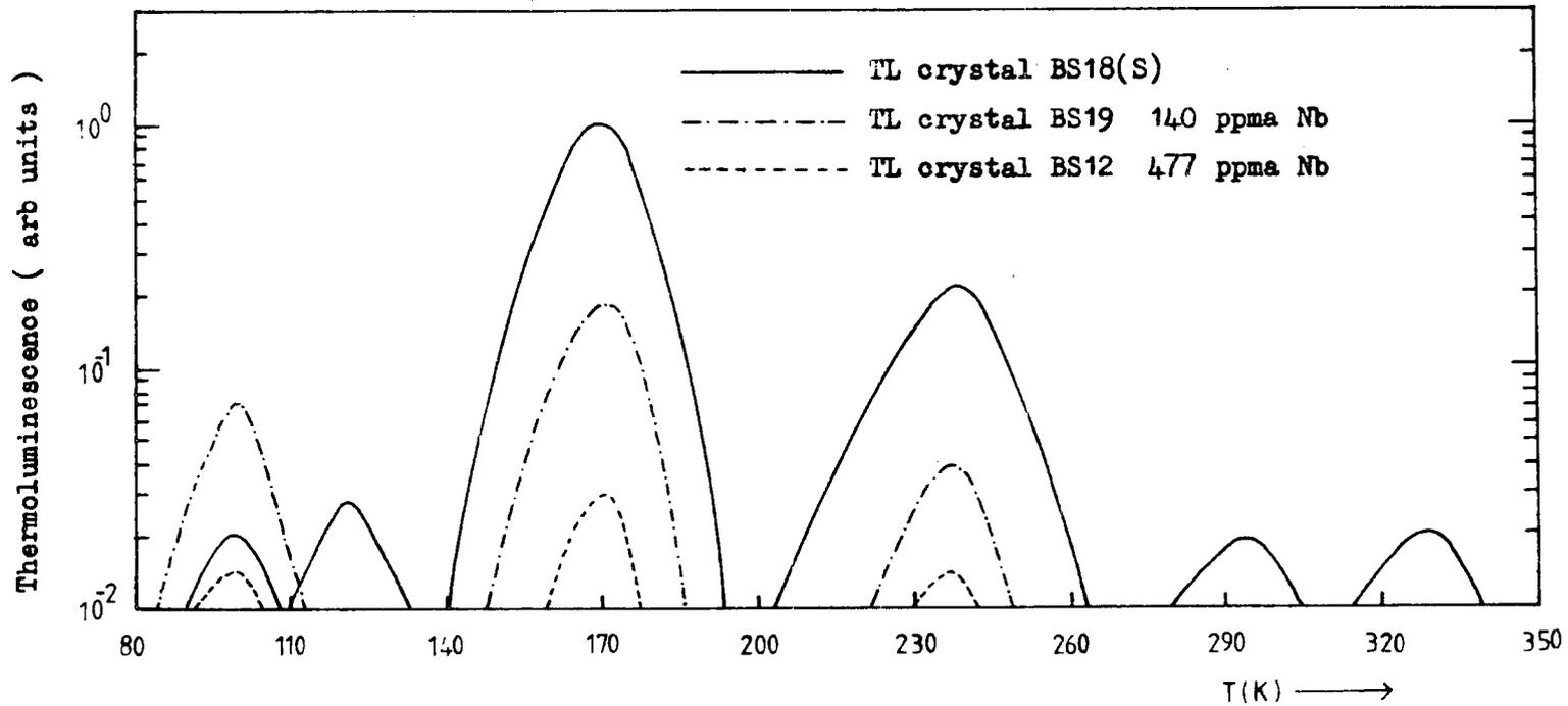
Figure 9.15.2 Comparison of TL spectra for the niobium doped crystals BS12 and BS19 and the 'undoped' crystal BS18(S) .
