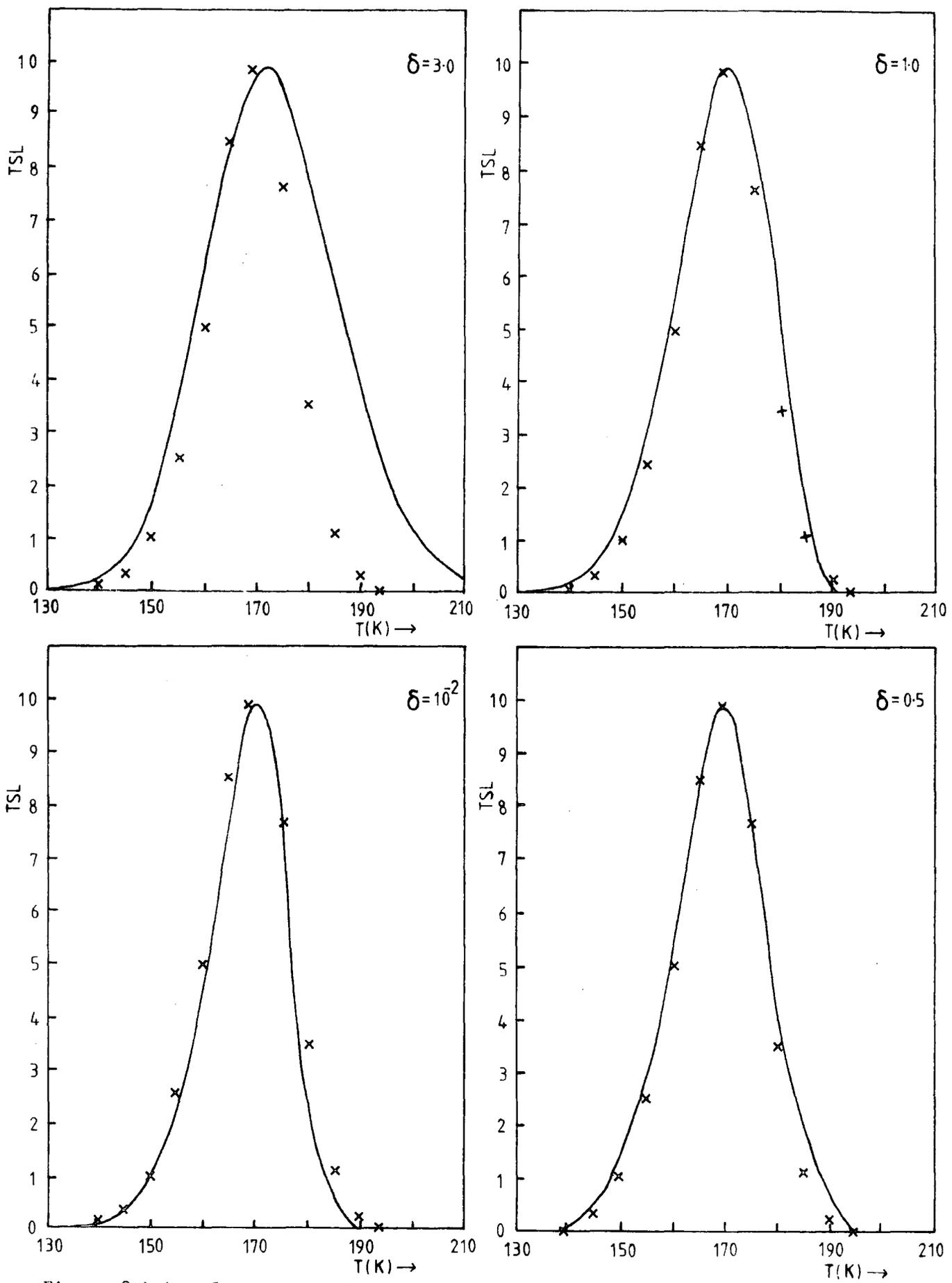
Figure 8.4.4 Comparison of the geometrical shapes of TSL curves for different retrapping ratios,  $\delta$ .  $E = 0.37 \text{ eV}$  ;  $h_s = 2.0 \cdot 10^{17} / \text{cm}^3$  ;  $h_d = 1.70 \cdot 10^{16} / \text{cm}^3$  ;  $\tau = 10^{-8} \text{ s}$  ;  $s = 7.39 \cdot 10^9 / \text{s}$  ;  $\beta = 0.5 \text{ } ^\circ/\text{s}$  .
