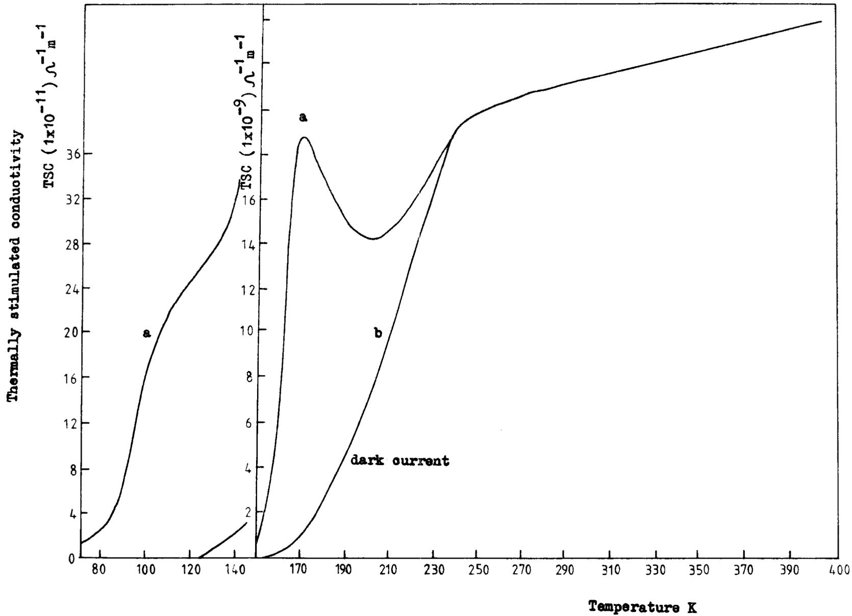
Figure 7.7.1 Thermally stimulated conductivity of a crystal reduced by heating in a vacuum at  $600^{\circ}\text{C}$  for 2 hrs .
