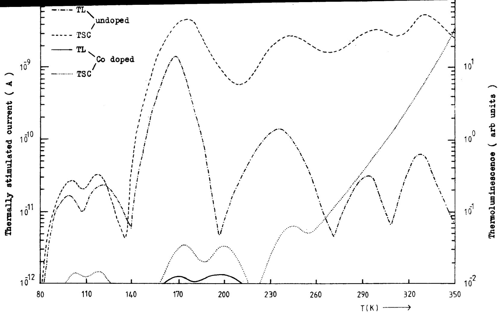
Figure 9.11.2 Comparison of the TSC and TL spectra for crystal CO(NL) before and after cobalt diffusion .
