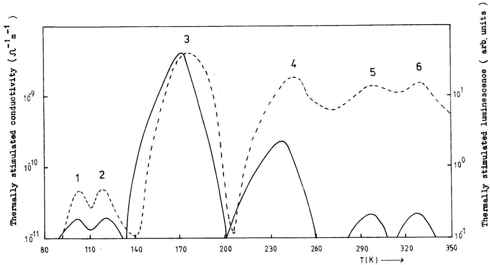
Figure 8.2.3 Comparison of the TSC and TL spectra for the NL crystal CA3(NL) .
