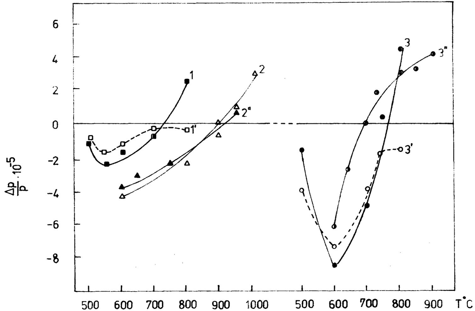
Figure 1.5.2 Dependences of the relative changes in the density (continuous curves) and weight (dashed curves) on the reduction temperature. Reduction duration (hrs) : 1, 1, 3, 3 ; (2) : 2, 2, 3, ; (0.5). Vacuum ( mm Hg ) 1, 1, 3, 3, 3 (  $1 \cdot 10^{-3}$  ) ; 2 (  $1 \cdot 10^{-4}$  ) ; 1 (  $10^{-2}$  ).
