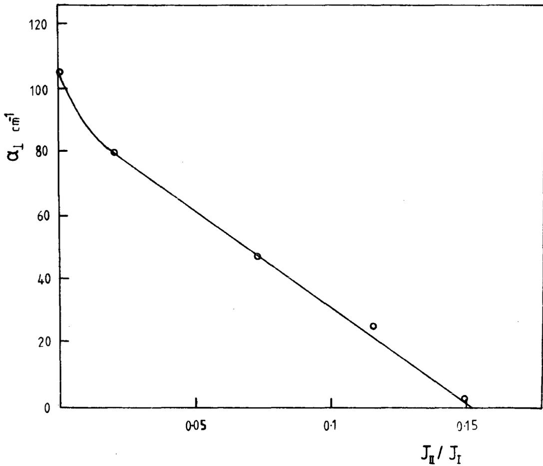
Figure 9.6.2 Relative intensity of EPR spectrum  $\Pi$  versus the optical absorption coefficient  $\alpha_I$  at the maximum of the 1.1 eV band for a  $\text{TiO}_2 \cdot \text{Cr}$  crystal ( after Sochava et al 1969 ) .
