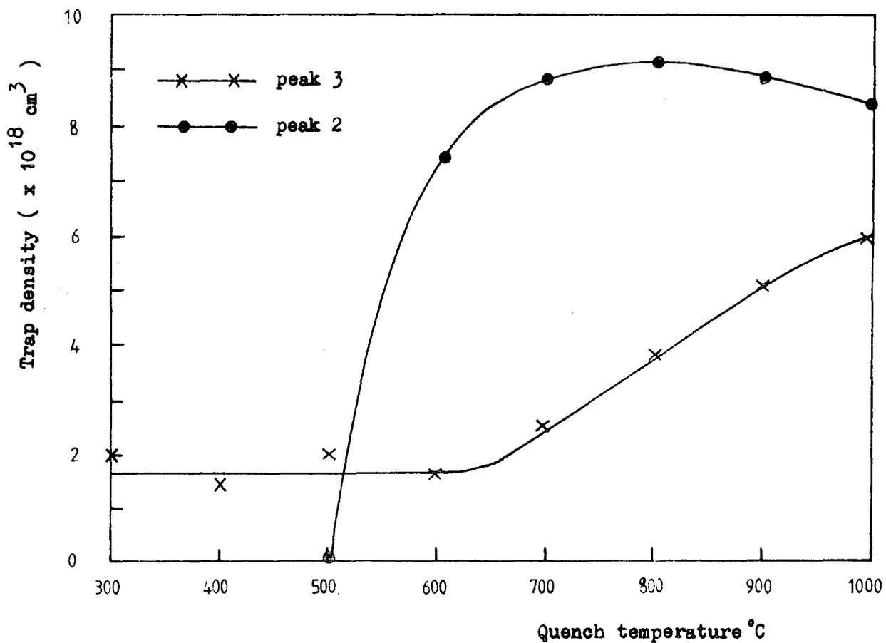
Figure 9.4.7 Densities of the shallow traps in the chromium doped crystal C1(NL) after quenching from  $T^{\circ}\text{C}$ .
