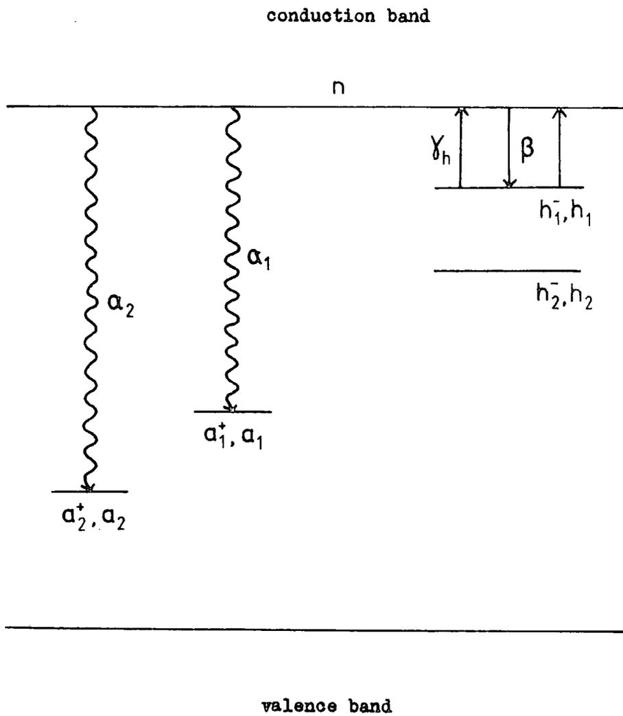
Figure 8.6.1 Energy level scheme with two acceptor centres involved in the recombination process .
