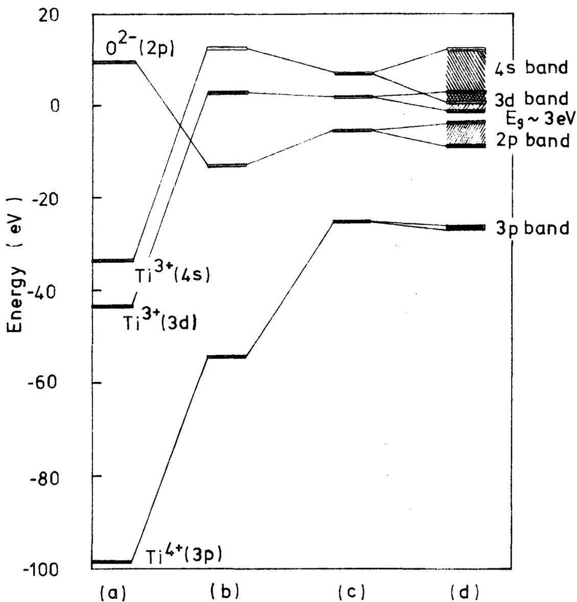
Figure 1.7.1 Sketch of the energy band structure of pure, stoichiometric  $\text{TiO}_2$ , based on a tight binding approximation; (a) free ion energies, (b) effects of Madelung potential, (c) screening and covalency effects, (d) bandwidth effects. After Adler 1970.
