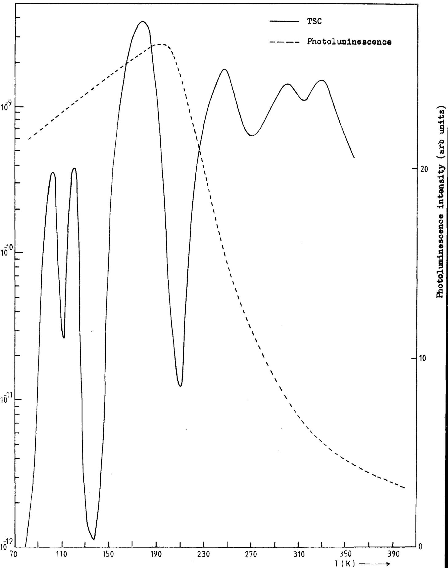
Figure 6.6.1 The thermal quenching of the photoluminescence in crystal CA<sub>3</sub>(NL).
