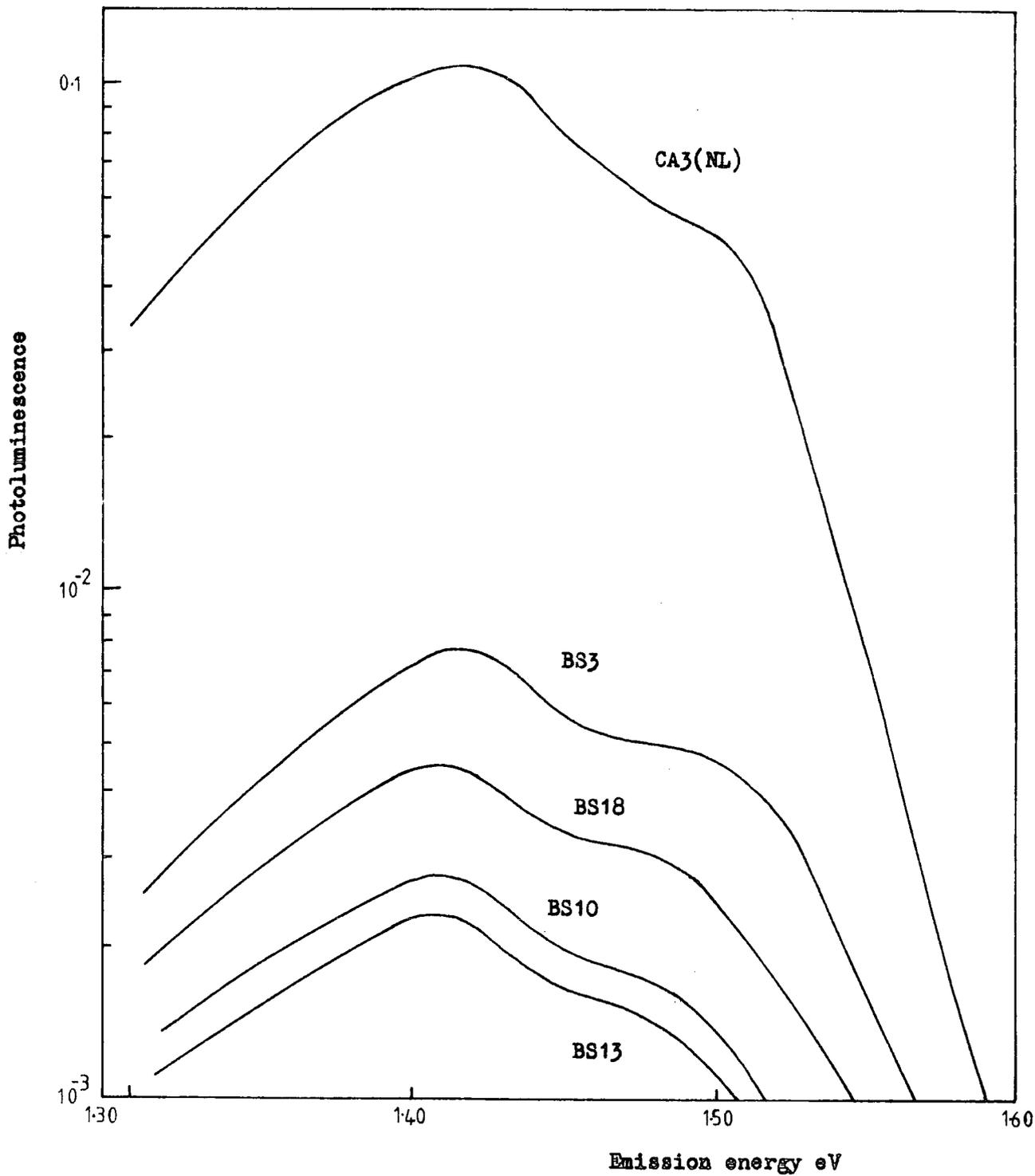
Figure 6.2.2 Comparison of the photoluminescence emission spectra for the flame fusion and plasma grown crystals.
