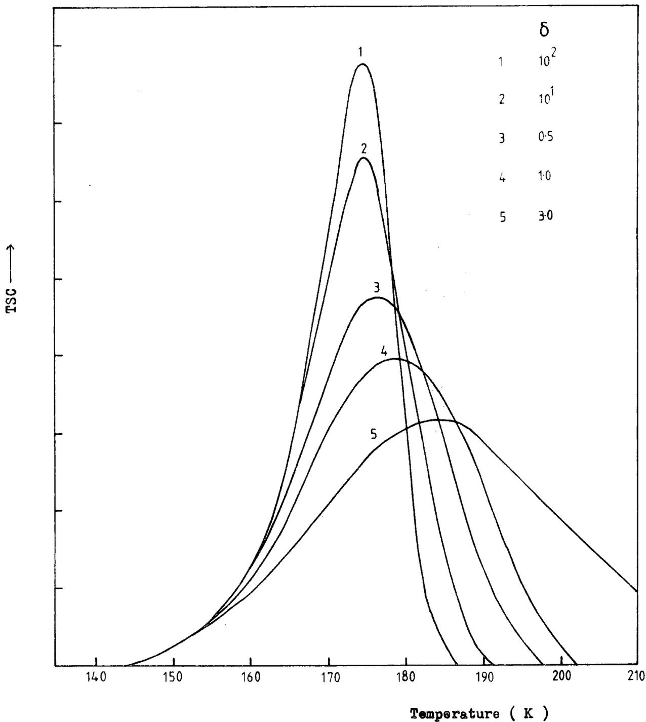
Figure 7.5.1 Variation of TSC curves with retrapping ratio  $\delta$  .
