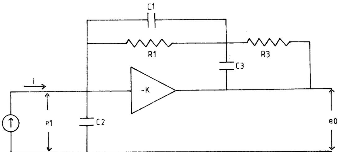
Figure 4.4.3 Circuit using compensated feedback ( Presley 1966 ).
