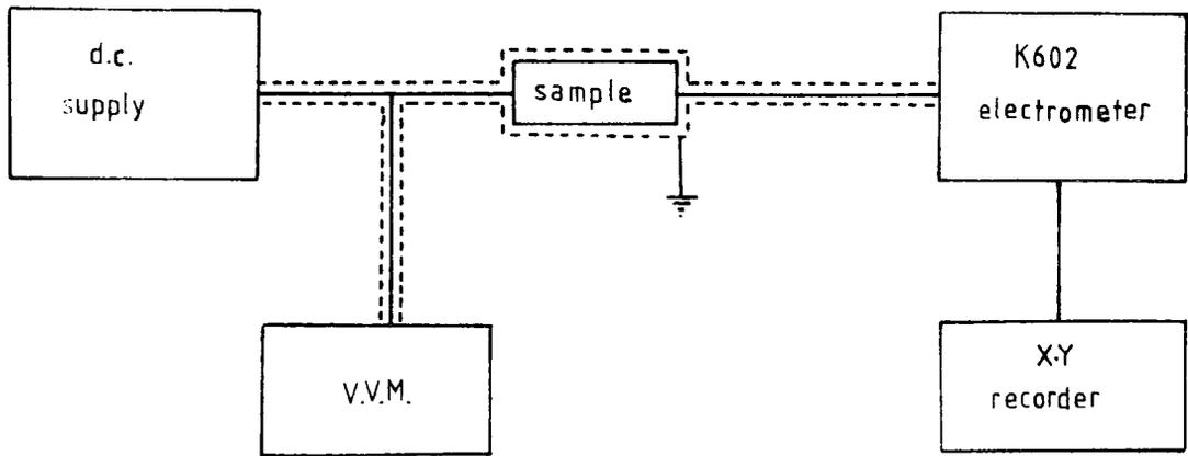
Figure 4.4.1 Electrical circuit for low current measurement.
