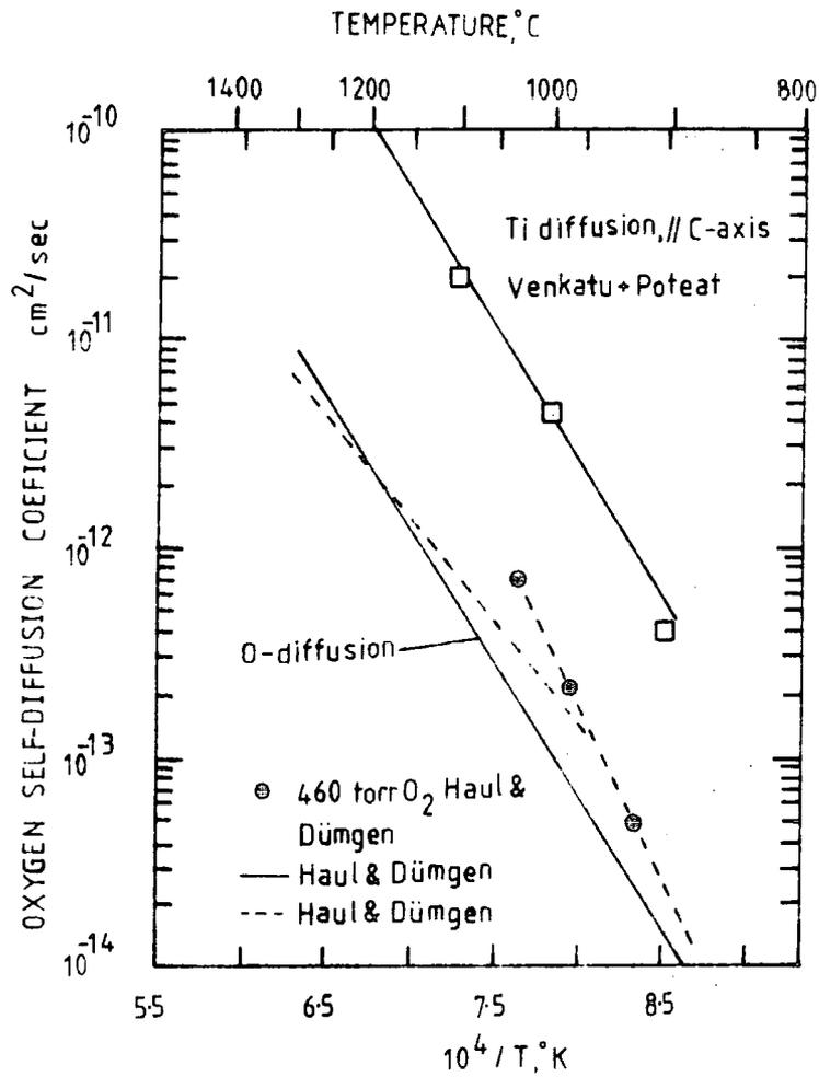
Figure 1.6.1 Self diffusion coefficients in rutile near atmospheric pressure as a function of the reciprocal temperature. After Haul and Dümgen (1962,1965) and Venkatu and Poteat (1970).
