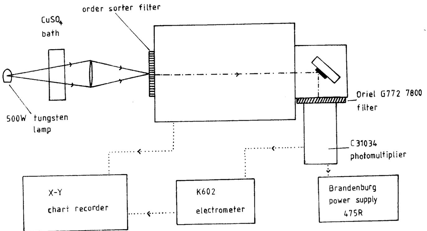
Figure 4.6.2 The experimental arrangement for observation of photoluminescence excitation spectra.
