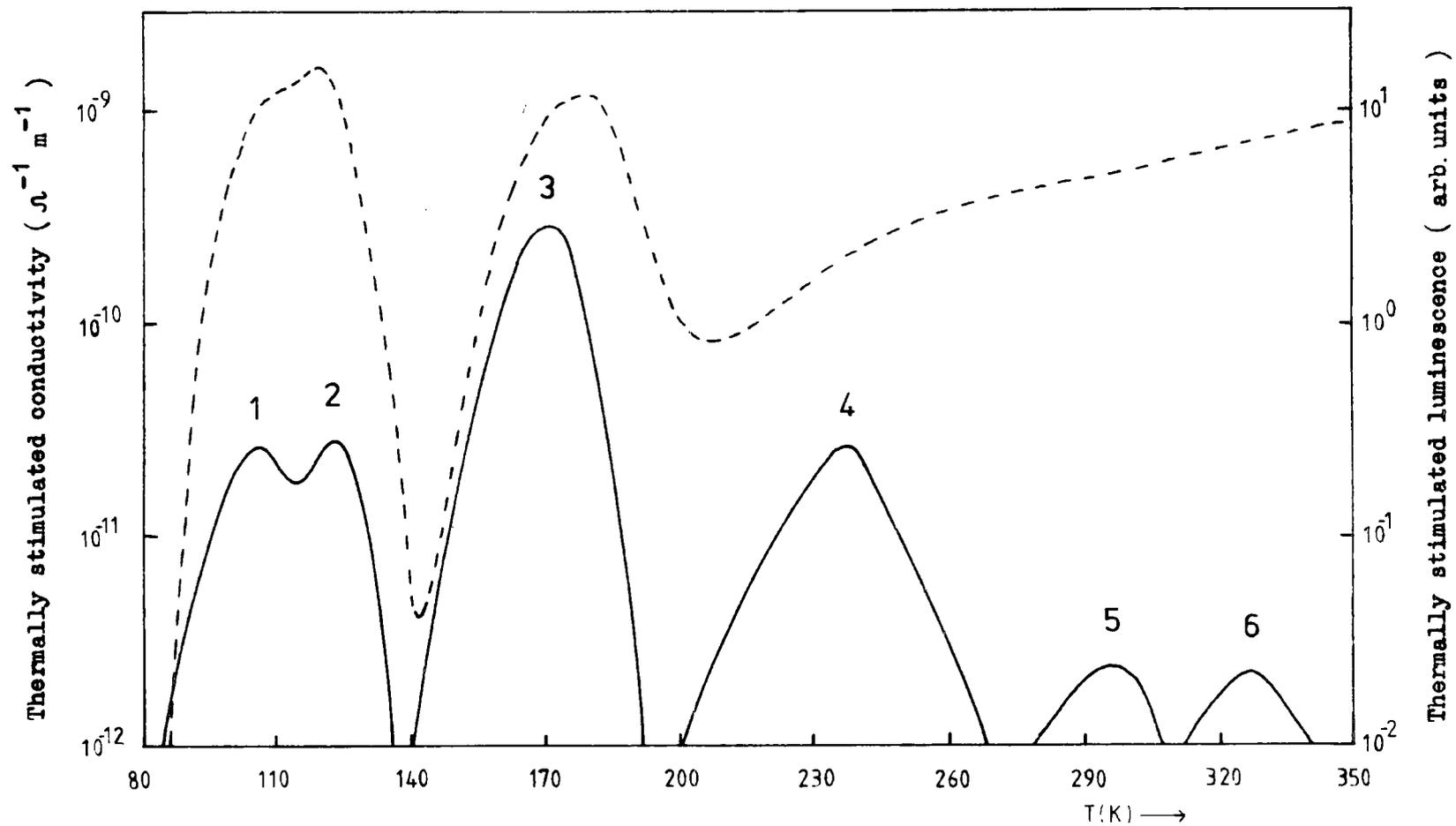
Figure 8.2.5 Comparison of the TSC and TL spectra for the crystal BS18(S) after quenching from  $600^{\circ}\text{C}$  .
