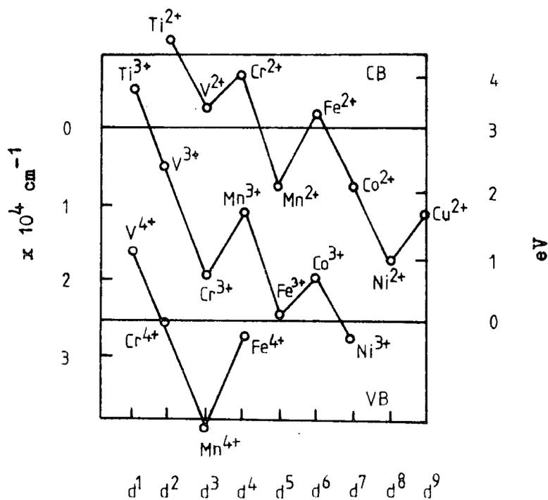
Figure 9.16.5 Calculated energy levels of the transition metal ions in  $\text{TiO}_2$ . The levels  $M^{+j}$  and  $M^{+(j-1)}$  which are near mutually are enclosed with dotted lines ( Tanaka et al 1972 ).
