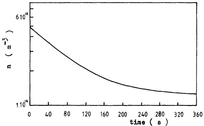
Figure 5.11.4 The emptying of the 0.68 eV trap in crystal CA3(NL) after excitation with light of wavelength 1.5  $\mu\text{m}$  .
