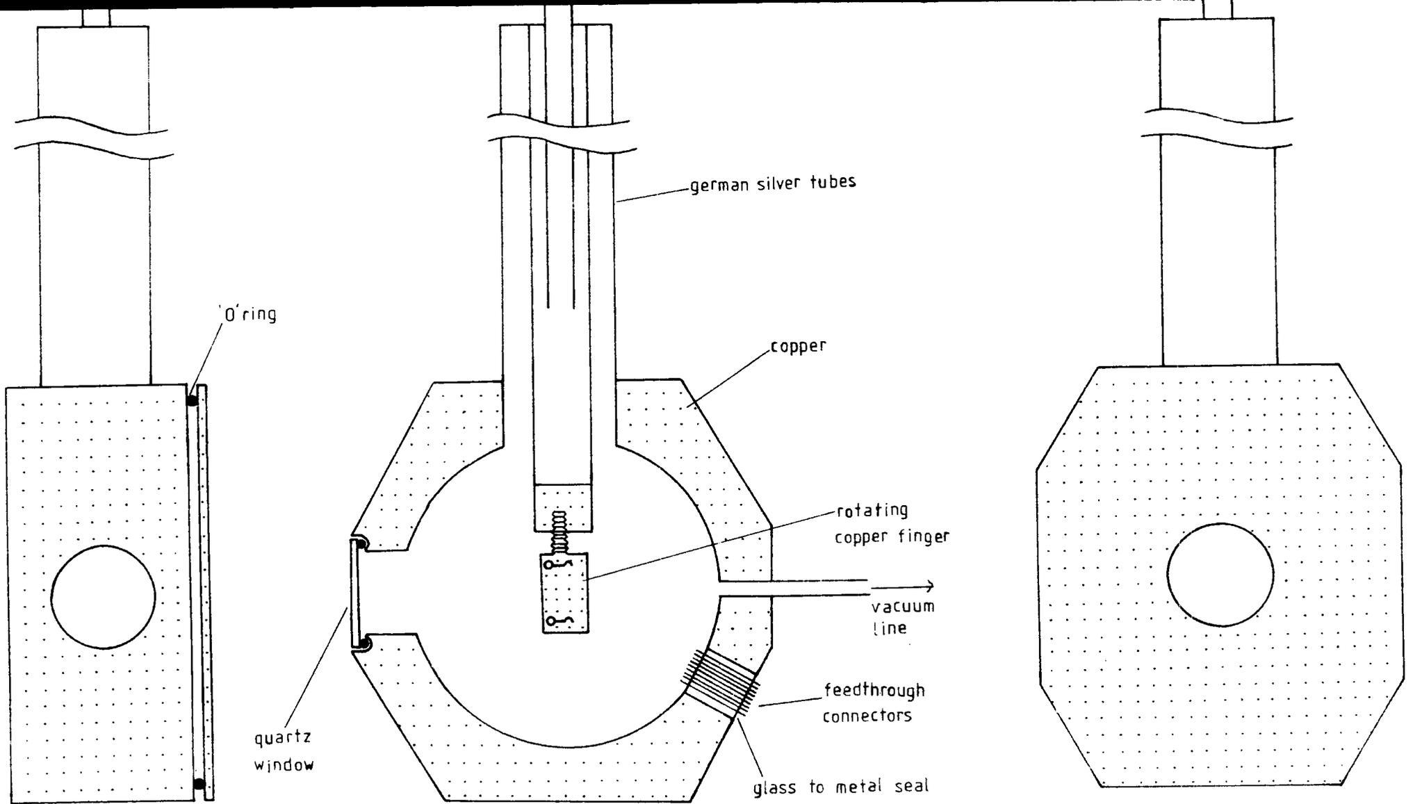
Figure 4.3.1 Liquid nitrogen cryostat.
