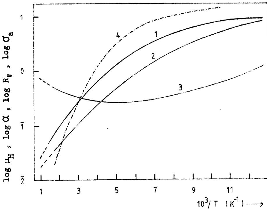
Figure 1.8.2 Temperature dependence of the Hall constant  $R_H$  (1), Hall mobility  $\mu_H = R_H \sigma_a$  (2), electrical conductivity  $\sigma_a$  (3) and the ratio of Hall mobility to the drift mobility (4).
