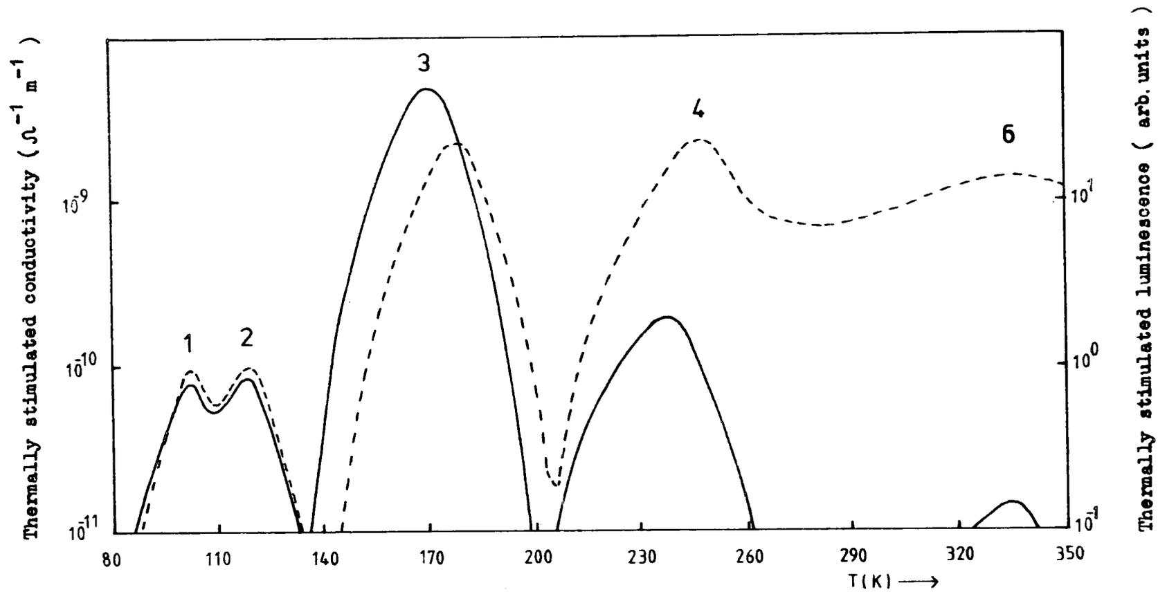
Figure 8.2.2 Comparison of the TSC and TL spectra for the non-stoichiometric as-grown crystal BS18(NS) .
