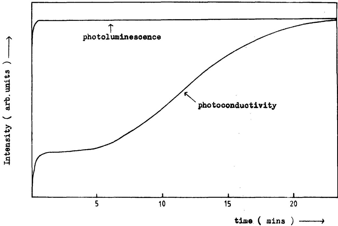
Figure 6.9.1 Kinetic response of PL and PC due to excitation with 410 nm light at 77 K.
