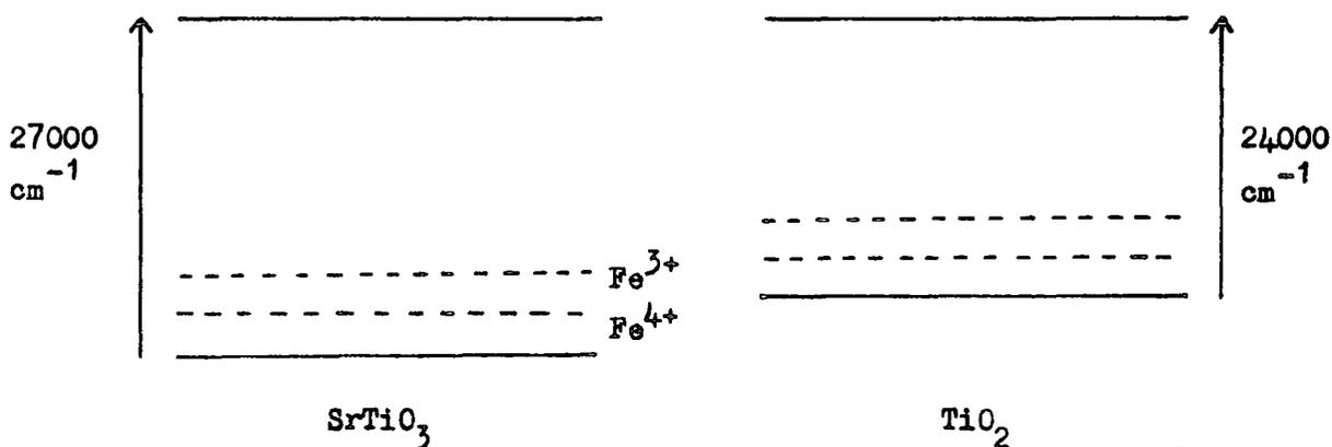
Before irradiation (  $0.39-0.43 \mu m$  ) the ions are present as  $Fe^{3+}$  and  $Mo^{6+}$ . After irradiation with blue light charge transfer takes place through either valence or conduction band, and  $Fe^{4+}$  and  $Mo^{5+}$  are created. When a photon is absorbed and an electron in an  $Fe^{3+}$  ion is expelled it is converted to  $Fe^{4+}$
