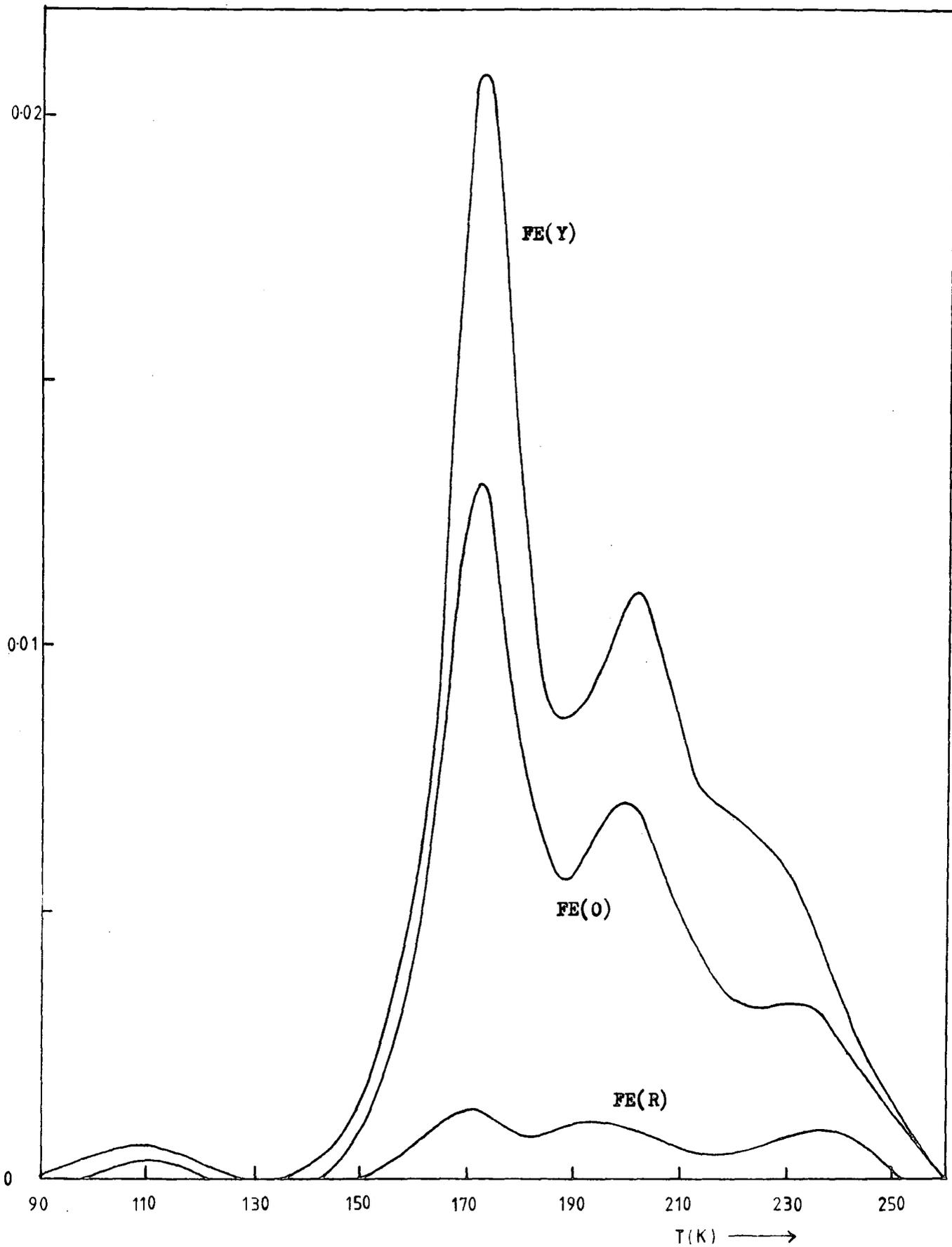
Figure 9.7.2 Thermoluminescence spectra for three samples cut from the iron doped plasma grown boule BS15 .
