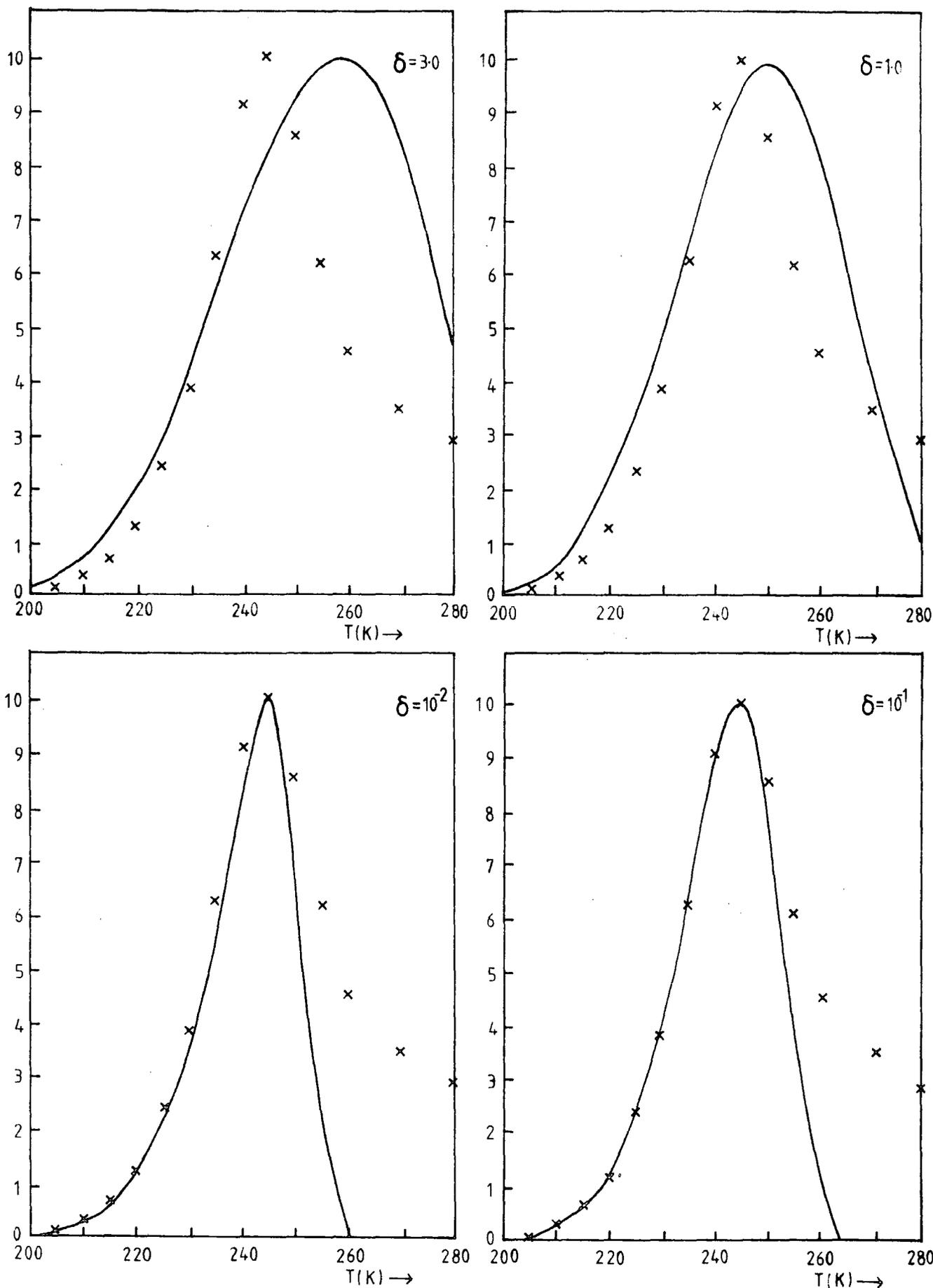
Figure 8.5.2 Comparison of the geometrical shapes of the TSC curves for different re trapping ratios,  $\delta$ .  $E = 0.51 \text{ eV}$  ;  $h_s = 9 \cdot 10^{15} / \text{cm}^3$  ;  $h_d = 8.0 \cdot 10^{14} / \text{cm}^3$  ;  $\tau = 10^{-8} \text{ s}$  ;  $\text{FREQ} = 3.5 \cdot 10^9 / \text{s}$  ;  $\beta = 0.5 \text{ } ^\circ/\text{s}$  .
