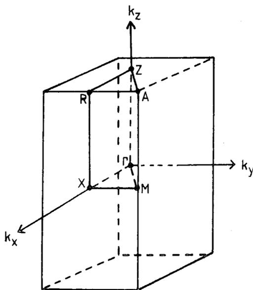
Figure 5.3.2 Schematic of rutile band structure and Brillouin zone with points of high symmetry .
