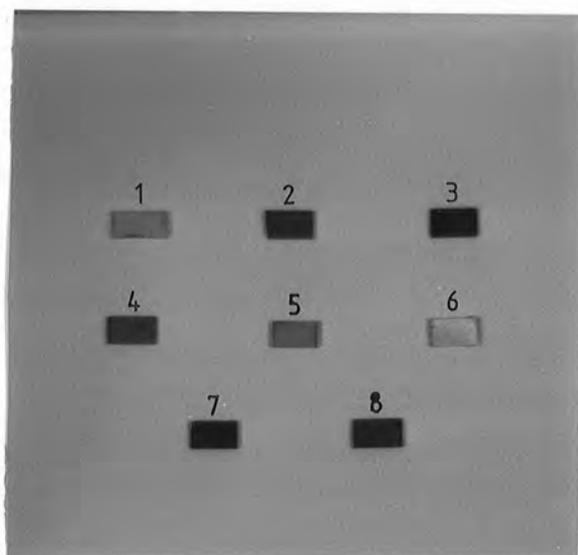
Figure 3.7.2 Photograph of the doped rutile crystals.
