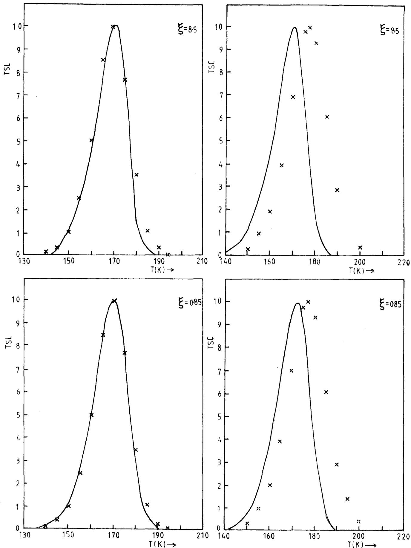
Figure 8.4.5 Comparison of the TSC and TSL curves for  $\xi = 8.5$  and  $\xi = 0.85$ .
