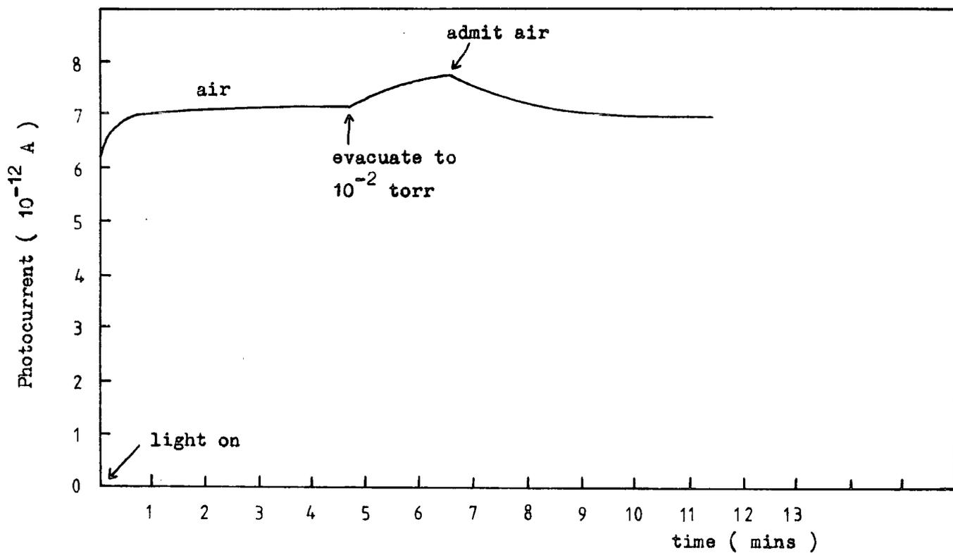
Figure 5.4.2 Photocurrent changes in crystal BS18(S) caused by changing ambient gases during excitation at 300 K (  $\lambda = 400$  nm ).
