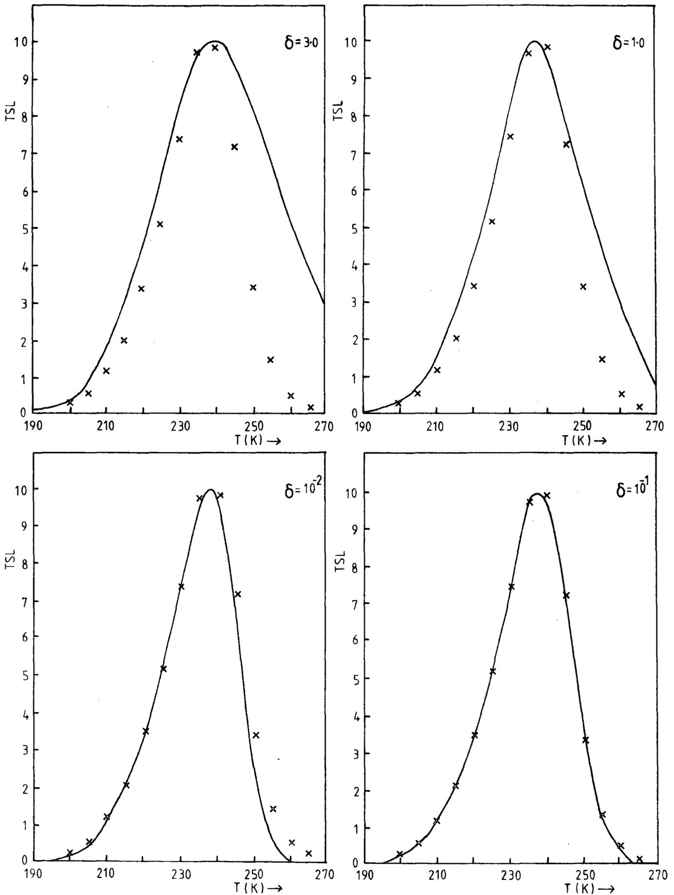
Figure 8.5.1 Comparison of the geometrical shapes of TSL curves for different retrapping ratios,  $\delta$ .  $E = 0.51 \text{ eV}$  ;  $h_s = 9 \cdot 10^{15} / \text{cm}^3$  ;  $h_d = 8.0 \cdot 10^{14} / \text{cm}^3$  ;  $\tau = 10^{-8} \text{ s}$  ;  $\text{FREQ} = 3.5 \cdot 10^9 / \text{s}$  ;  $\beta = 0.5 \text{ }^\circ/\text{s}$  .
