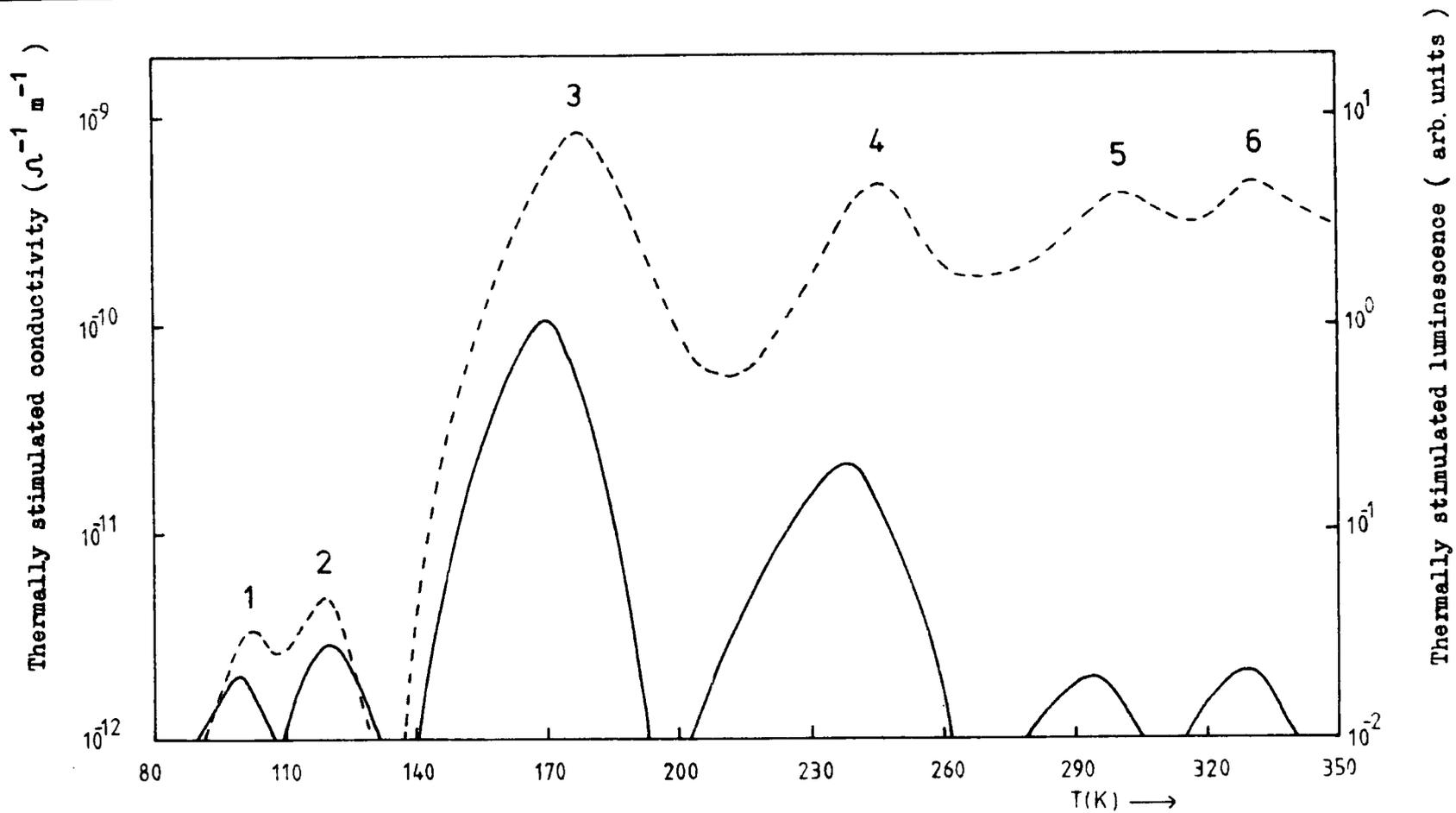
Figure 8.2.4 Comparison of the TSC and TL spectra for the stoichiometric as-grown crystal BS18(S) .
