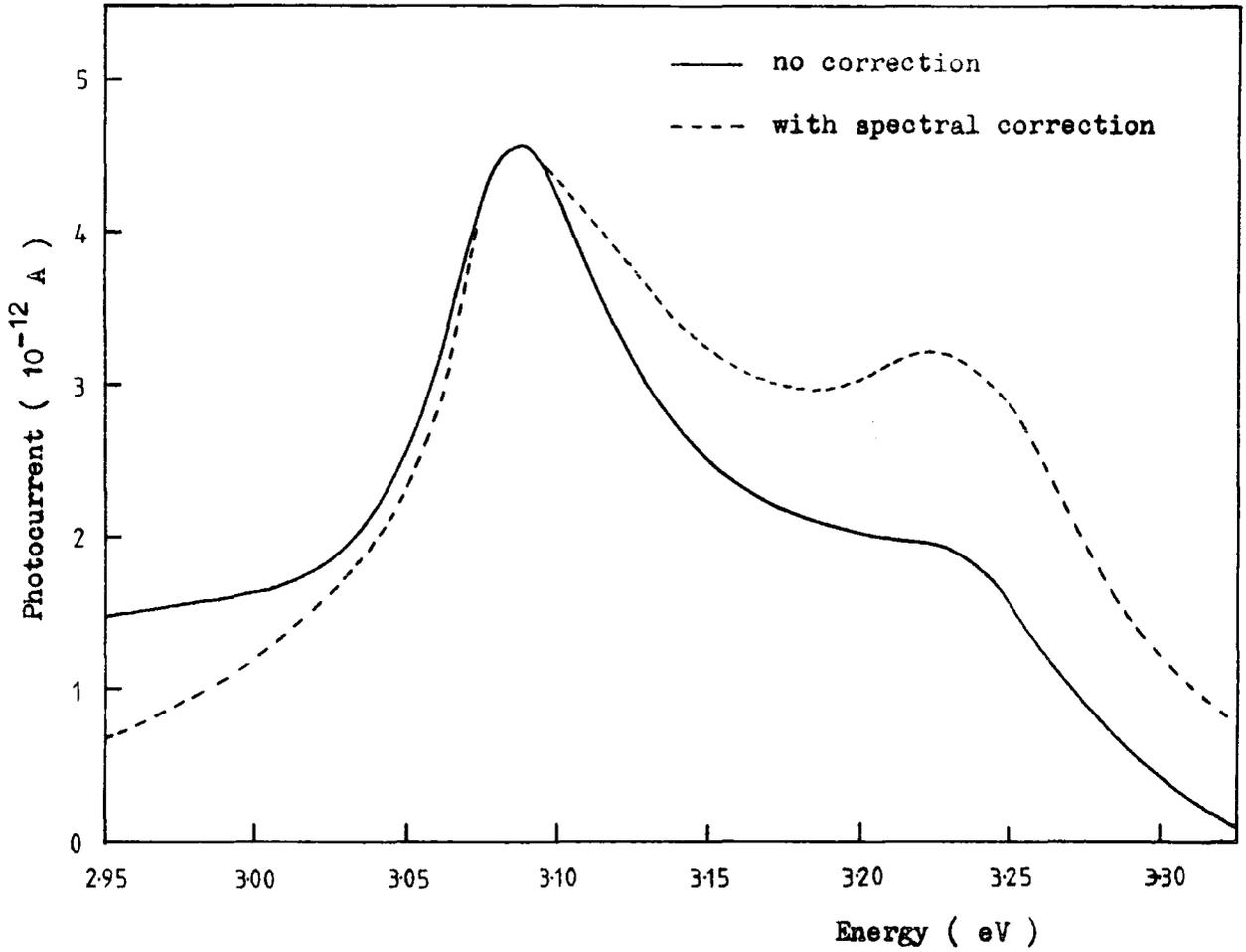
Figure 5.2.1 Spectral response of photoconductivity in crystal CA3(NL) at 77 K.
