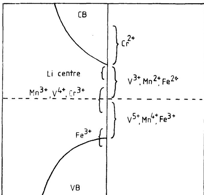
Figure 9.16.4(c) Proposed energy level schemes of the transition metal ions in  $\text{TiO}_2$  ( Mizushima 1973 ).
