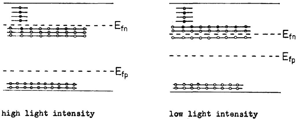
Figure 5.7.3 Model for IR quenching in quenched oxidised crystals.
