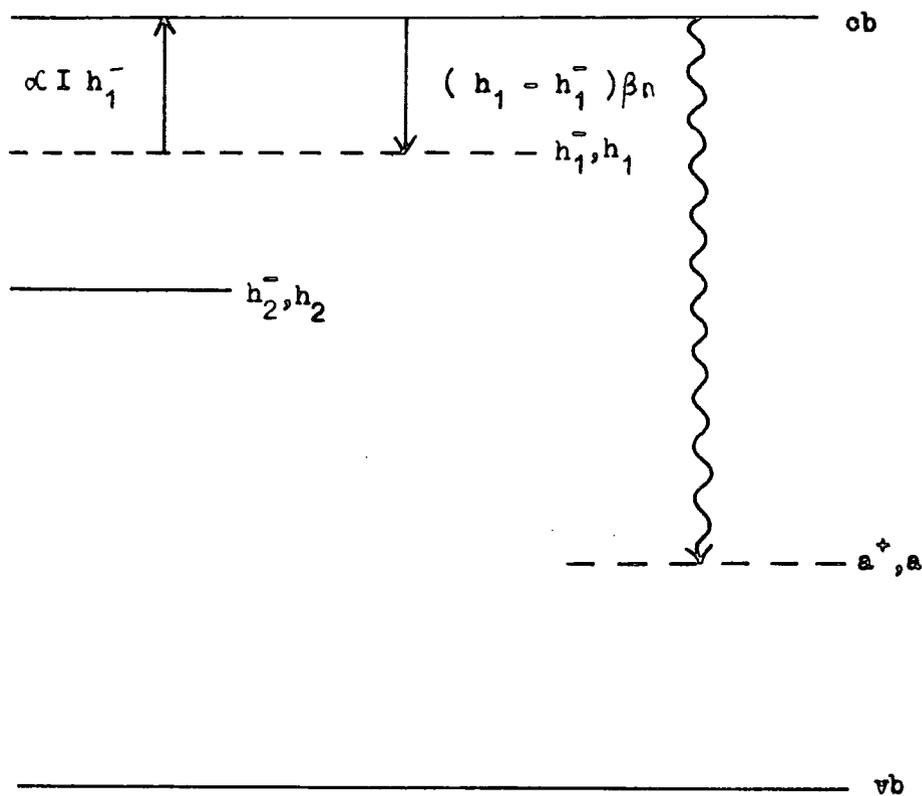
Figure 5.10.1 Simple insulator model used to describe the PSC spectra .
