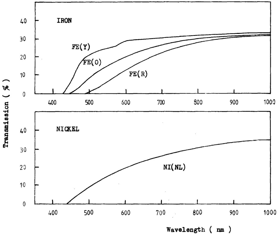
Figure 9.2.3 The optical transmission spectra of the iron and nickel doped crystals at 300 K.
